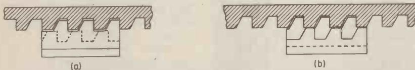
Fig. 6. Mechanical detenting. Detent pawl is split and has two sets of teeth at 180° to each other. At (a), the carriage is detented to an odd numbered cylinder and the upper pawl teeth are engaged. The lower pawl, represented by the broken line, rests against the tops of the rack teeth. In (b), the carriage is detented at an even cylinder and the lower pawl is engaged. Tooth pitch on the rack is twice the cylinder spacing.
