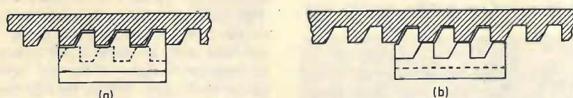
Fig. 6. Mechanical detenting. Detent pawl is split and has two sets of teeth at 180° to each other. At (a), the carriage is detented to an odd numbered cylinder and the upper pawl teeth are engaged. The lower pawl, represented by the broken line, rests against the tops of the rack teeth. In (b), the carriage is detented at an even cylinder and the lower pawl is engaged. Tooth pitch on the rack is twice the cylinder spacing.
