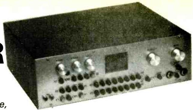
*A matching unit to the 80-100W power amplifier described in the June, July and August issues of Wireless World. Each circuit in the design is separate, and can be included or omitted, as desired, or switched in and out from the front panel. The design includes a noise blanker and image-width control*
