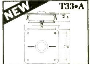
Low colouration dome high frequency unit with extended frequency response.
