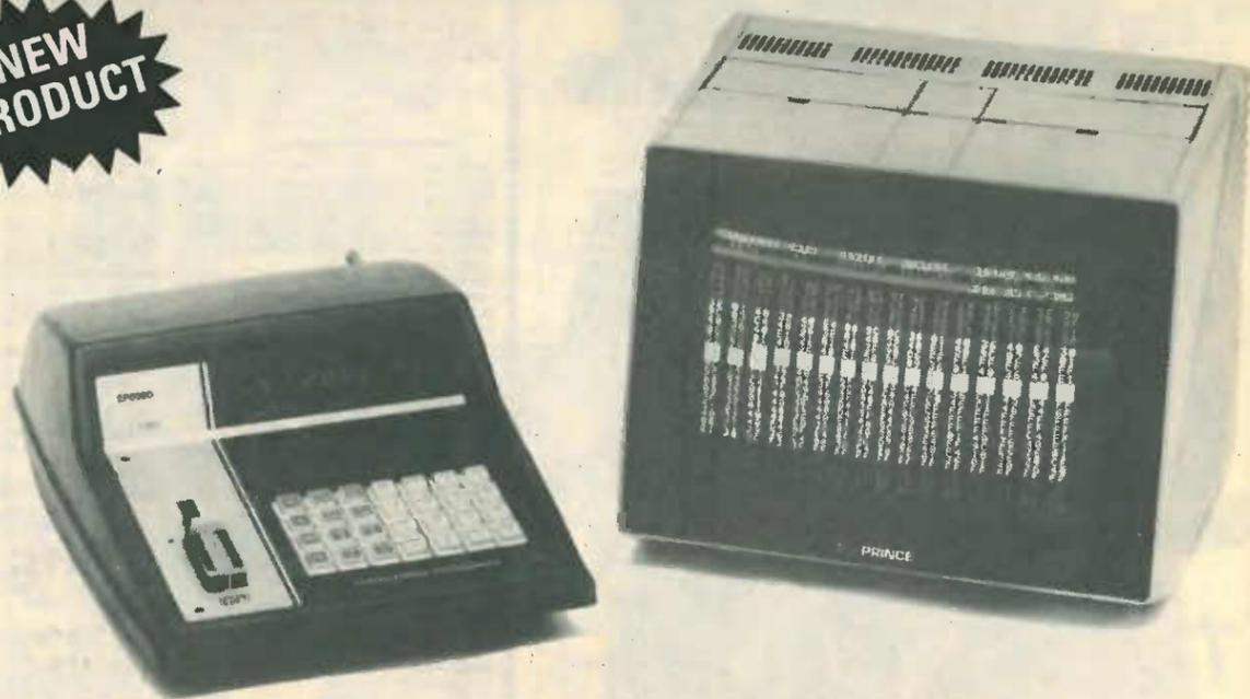
The new microprocessor controlled EP8000 Emulator Programmer will program and emulate all EPROMs up to 8k x 8 sizes, and can be extended to program other devices such as 16k x 8 EPROMs, Bipolar PROMs, single chip microprocessors with external modules. Personality cards and hardware changes are not required as the machine configures itself for the different devices. The EP4000 with 4k x 8 static RAM is still available with EPROM programming and emulation capacity up to 4k x 8 sizes.
