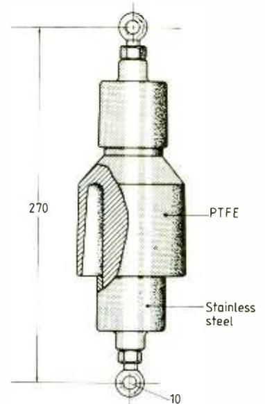
**Fig. 10.** Tough German aerial strain insulator using skirt principle. Rated at 50kV (dry) at 500kHz. 700kg tensile load, mass 1.5 kg. (Dieckmann & Klapper.)
