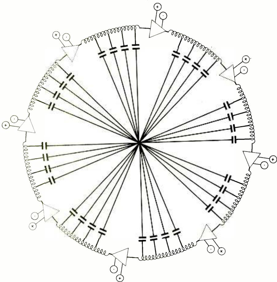
**Fig. 3.** Artificial delay line whose construction is described in the text in which a wave runs in the clockwise direction. Rotation of the system in an anticlockwise direction at the same angular frequency as that of the wave produces a static field. Red and green light-emitting diodes, connected at the points marked + and -, indicate the stationary wave, as on the cover photograph.
