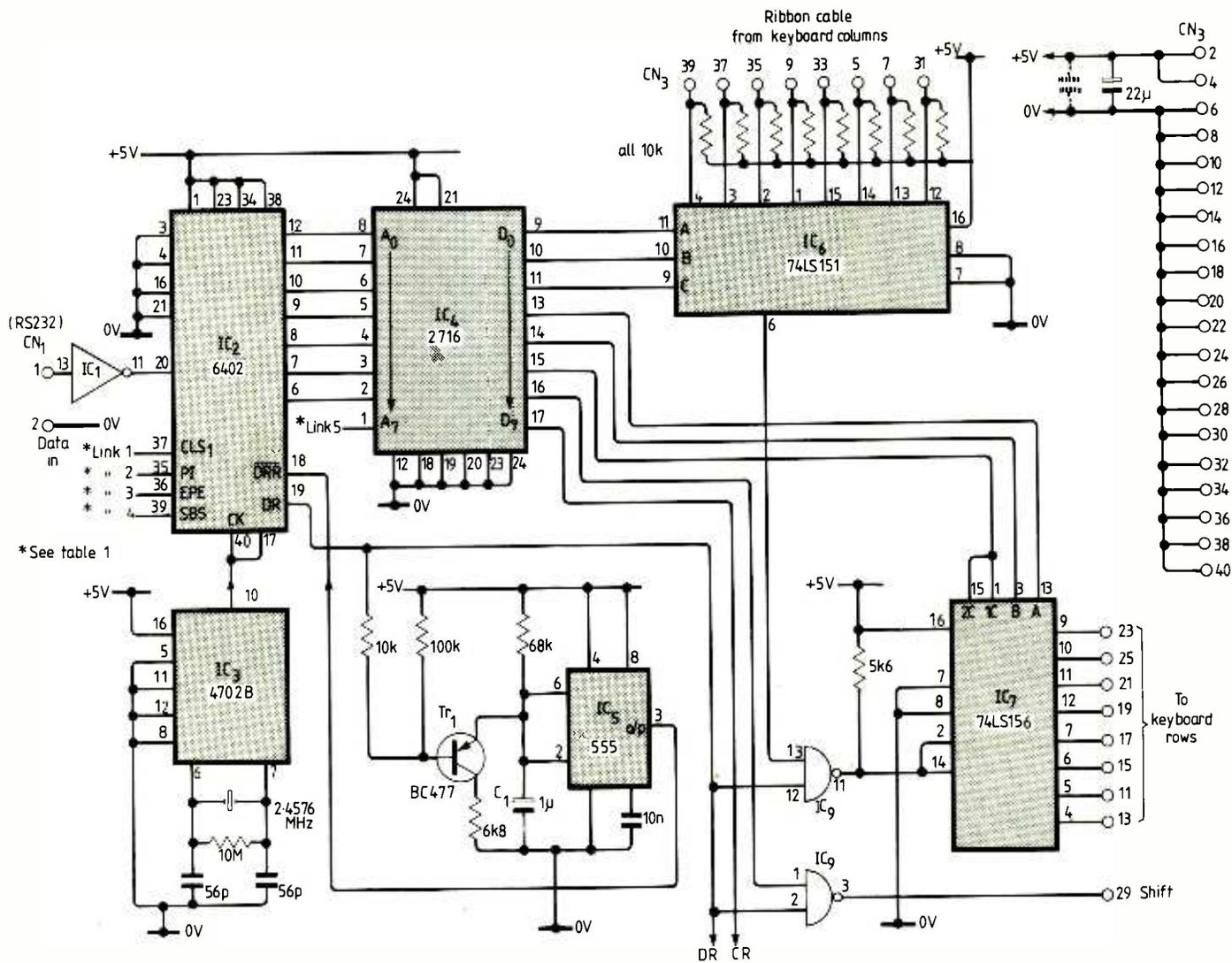
**Fig. 2.** Incoming serial data from the computer is converted by the interface into parallel data in a form suitable for connection to the keyboard matrix of the typewriter. IC<sub>1</sub> is a section of an MC1489 line-receiver device.
