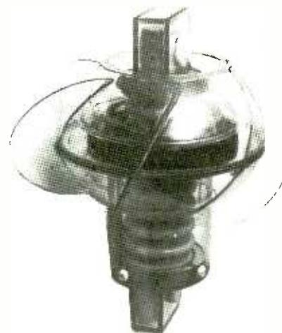
**Fig. 14.** British invented link/strain insulator assembly with protective shrouding. Wind-driven rotating outer dome expels water by centrifugal action. (P. F. Barber, Scarborough.)
