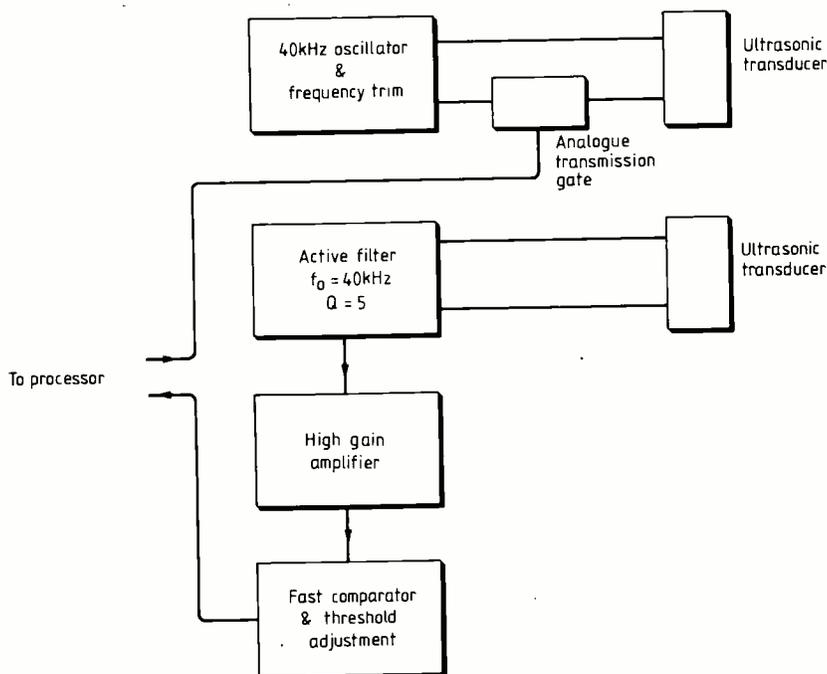
Block diagram of the ultrasonic frequency ranging system.
