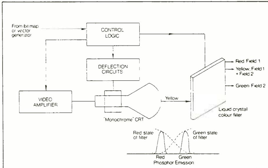
and green. In any field, information written on the screen appears in the colour selected by the electronic switch. Each colour is repeated at 60Hz, requiring the two-field system to run at 120Hz. This field-sequential system provides all possible mixtures of the two primary colours emitted by the phosphor and research is continuing to extend the concept to three fields to produce the full colour spectrum.
