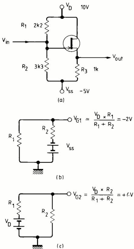
Fig. 5. Using superposition to find the dc bias on the gate of a j-fet amplifier. Original circuit (a), determining the effect of  $V_{SS}$  (b), and determining the effect of  $V_D$  (c).
