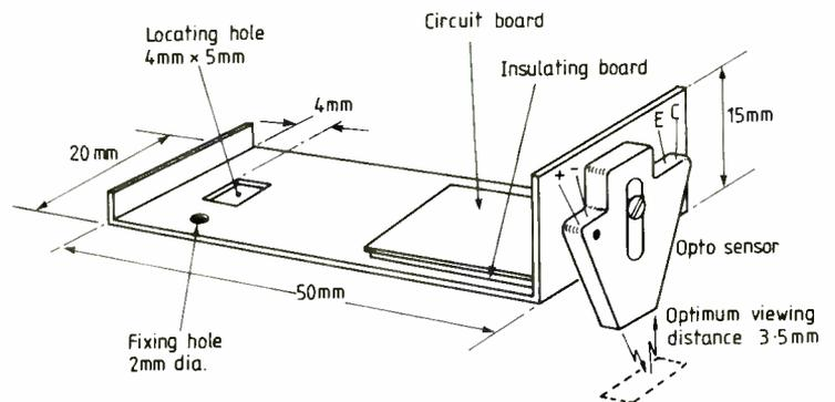
**Fig. 7.** Opto-sensor mounted underneath the platen roller views the paper through a hole cut in the paper guide roller carrier (Fig. 6).
