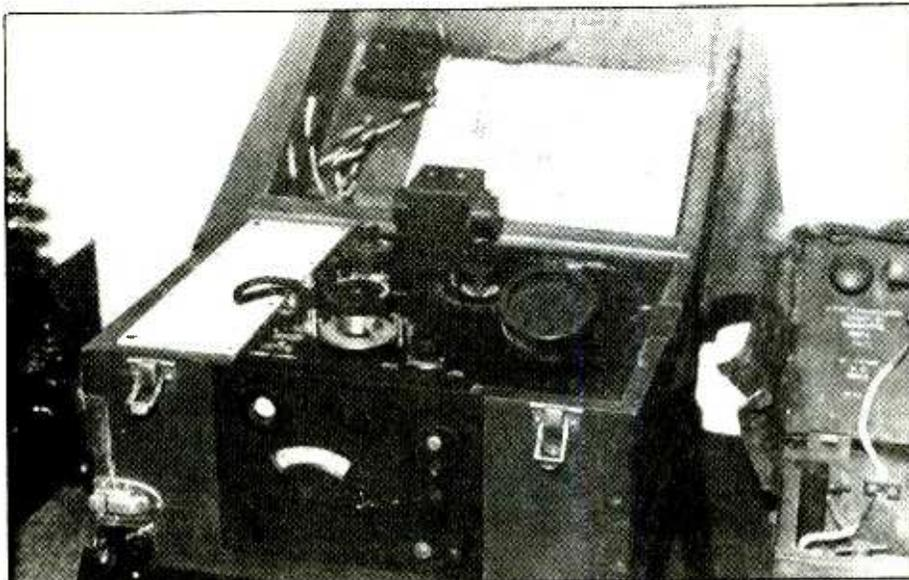
**Fig. 1.** This l.f. trench transmitter operated into an aerial only a metre above ground, but others worked from aerials inside the trench. (20watt Mk 3 transmitter, 1917, has single-valve tuned-anode oscillator, but a second valve could be switched in parallel for maximum power. HT supplied by 1,000-volt battery or induction coil.)
