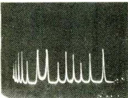
If the oscilloscope sweep speed is too fast, as it is here, the tuner frequency may still be dropping when the next sweep begins. This can arise because voltage-controlled tuning circuits usually incorporate some capacitance for stability, for example,  $C_x$  in Fig. 1.
