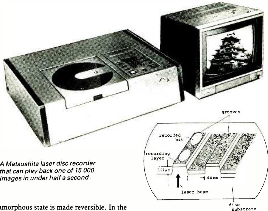
*An erasable optical storage disc for video images and data developed by Matsushita uses two separate lasers for recording and erasing through a common optical system. The one gigabyte disc can record broadcast pictures in real time and be erased over one million times but when the disc might be available is not yet certain.*
