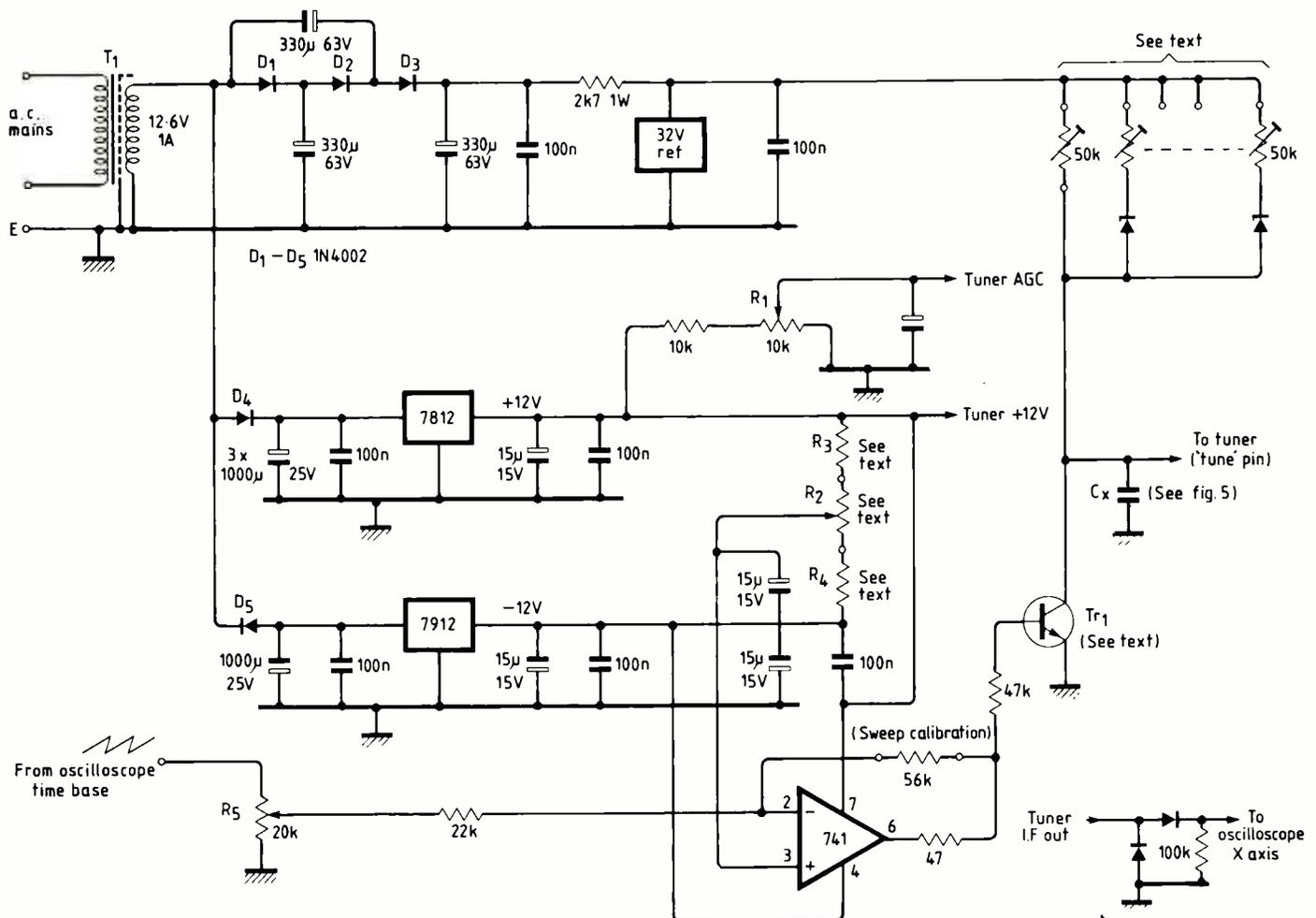
viewing frequencies of hundreds of megahertz the oscilloscope is coping only with rectified a.c. and the sweep should be as slow as possible. About 25 sweeps per second will be fast enough to avoid too much flicker.
