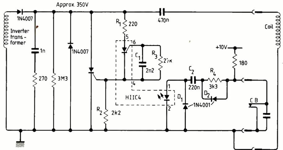
crease the light drive required for operation at low temperatures. If the unit is to be potted C<sub>1</sub> should be increased in value to cope with the increased coupled dV/dt due to the μ<sub>r</sub> of the potting compound. The drive circuit is basically that used by Cooper with revised differentiator values
