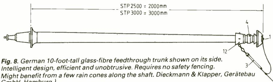
**Fig. 8.** German 10-foot-tall glass-fibre feedthrough trunk shown on its side. Intelligent design, efficient and unobtrusive. Requires no safety fencing. Might benefit from a few rain cones along the shaft. Dieckmann & Klapper, Gerätebau GmbH, Hamburg.)
