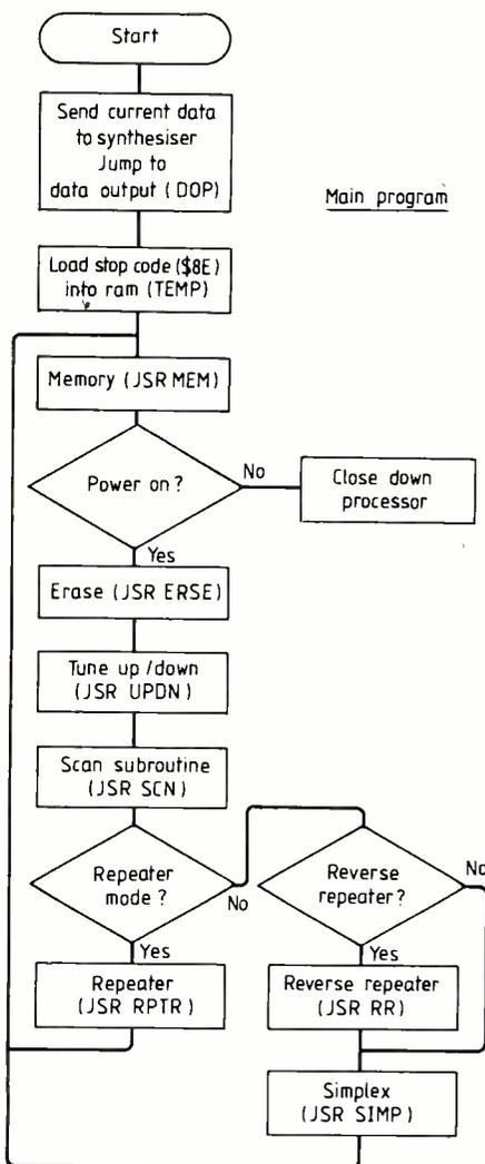
Eprom starts at 1800 hexadecimal and software breaks down into these main routines. Erase and up/down routines were covered in the April issue
