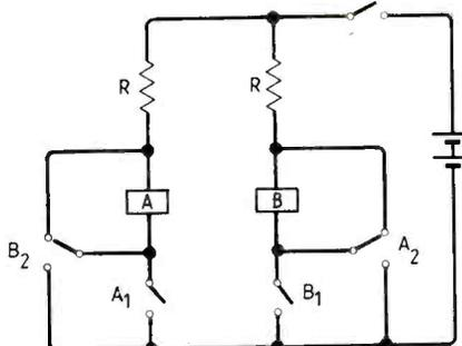
This arrangement cannot act like a buzzer, because of the toggle action. Thus relay A cannot cancel its instruction to relay B at once, but instead its changeover contact must move right across its gap. Output can be taken from a further contact. Frequency is 3-10Hz, depending on obvious factors.
