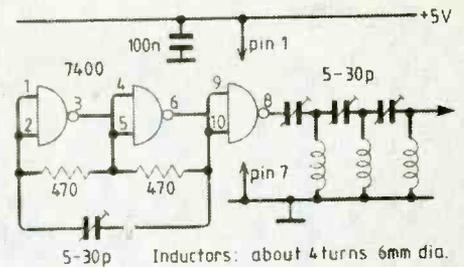
Electrically the comb generator is just an oscillator. But where normally we try to get a clean signal and suppress the harmonics here we try to produce as many as possible. We make a high pass filter by feeding the output through two or three (or more) small capacitors in series with inductors. Choose a convenient frequency for the oscillator (e.g. 10, 20, 25 or 50MHz) and fiddle both the capacitors and inductors while watching the result on the screen.
