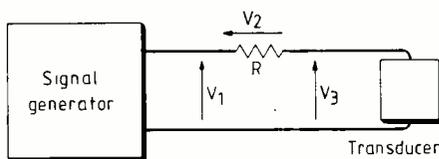
**Fig. 3.** In the absence of a bridge the input impedance of a transducer may be determined by measuring the voltage drop across a series resistor.
