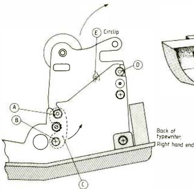
**Fig. 5.** Platen roller must be swung upwards to allow access for fitting the paper-out detector. Remove screw B on the right-hand roller support bracket. Swing plate C clear on the right-hand bracket and swing the platen roller assembly upwards, pivoting it about nut D.
