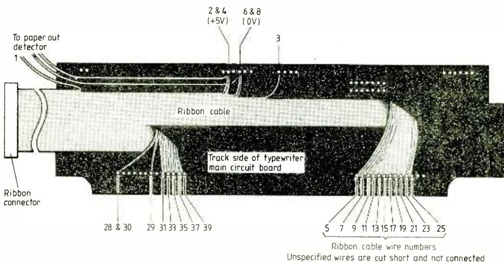
**Fig. 4.** 40-way ribbon cable connects the interface to the underside of the typewriter main circuit board. Alternate wires in the ribbon are connected to +5 or to 0V either at the interface end or the typewriter end. This helps to prevent crosstalk between the signal wires.
