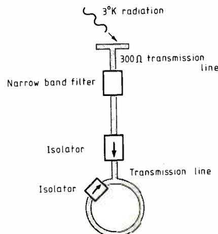
**Fig. 2.** More practical arrangement for putting the wave into the circular line.
