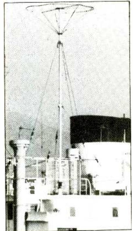
**Fig. 3.** Top-loaded unipole aerial of Scandinavian origin. The stays add to the top capacitance, also to the leakage. Has little height. (Photographed at Eleusis, Greece, 1982)
