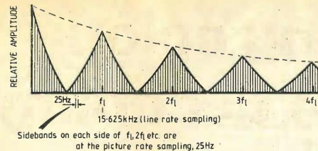
Fig. 2. Spectrum of luminance component of a television signal with  $15.625\text{kHz}$  sequential scanning of a stationary picture. Scene is sampled at  $15.625\text{kHz}$  for 625 lines and 25 pictures per second are constructed. The spectral energy centres are therefore at line frequency  $f_L$  and at  $2f_L$ ,  $3f_L$ , etc. Spacing of sidebands about the multiples of  $f_L$  is  $25\text{Hz}$ , which is the picture rate.
