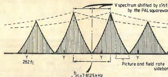
Fig. 4. V-axis spectral energy groups are alternatively reversed about the centre of subcarrier frequency at half the line frequency ( $7.8\text{kHz}$ ).
