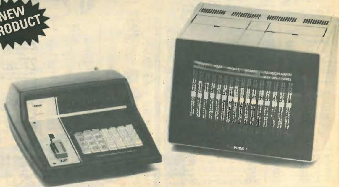
The new microprocessor controlled EP8000 Emulator Programmer will program and emulate all EPROMs up to 8k x 8 sizes, and can be extended to program other devices such as 16k x 8 EPROMs, Bipolar PROMs, single chip microprocessors with external modules.
