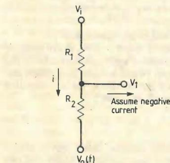
plied at time  $t$  the system will not respond until  $t + \tau$ . At  $t$  the voltages  $v_i$  and  $v_0$  on the resistor network interact instantaneously and define the value for  $v_1$  at the amplifier input, Fig. 3
