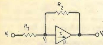
The resistance chain is an instantaneous voltage dividing system, and in particular, for negative feedback ( $\mu < 0$ ) it can be regarded as forming a 'voltage lever' pivoted at the amplifier input  $v_1$ .
