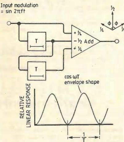
Fig. 11(c). Derivation of comb filter characteristic using algebra and vector diagram. Output is vector sum of the three contributions. Phase angle ( $\phi = 2\pi ft$ ) swings between 0° and 180° as the modulation, representing the tv signal, swings between 0-5MHz. When  $\phi = 0^\circ$  signal doubles,  $\phi = 180^\circ$  signal cancels. Output signal is
