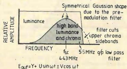
Fig. 8. PAL encoder output signal showing the shaping y chroma pre-modulator filters and the output filter. Output signal is as shown, where Y is the luminance component,  $U \sin \omega t$  is the B-Y colour component, and  $V \cos \omega t$  is the R-Y colour component both modulated onto the 4.43MHz subcarrier. The  $\cos$  term shows quadrature phase relationship between U and V.  $\pm$  indicates the alternating V axis.
