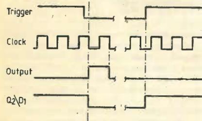
Note that in both circuits the trigger pulse must be a minimum (for worst case phasing w.r.t. the clock) of two clock periods wide.
