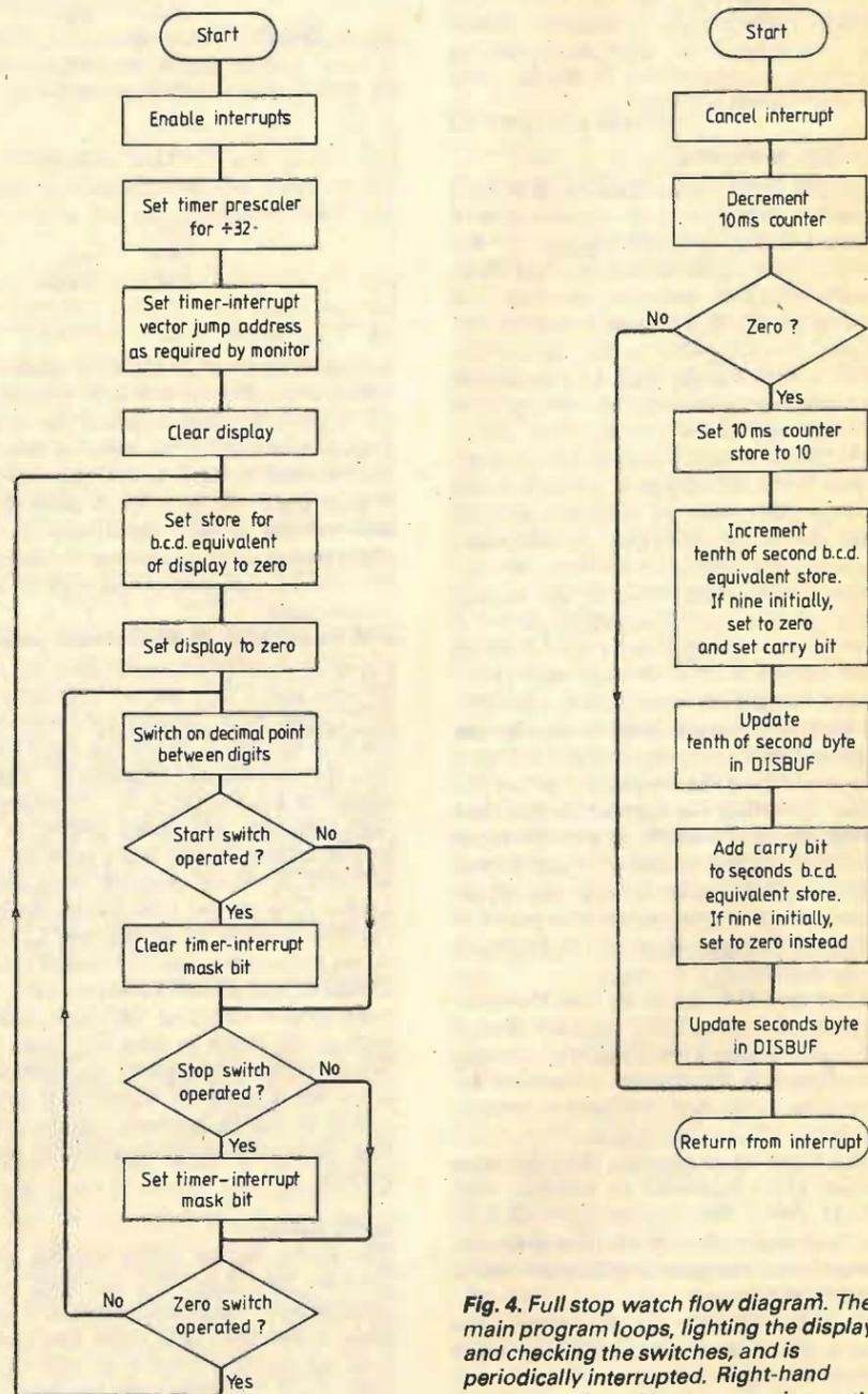
Fig. 4. Full stopwatch flow diagram. The main program loops, lighting the display and checking the switches, and is periodically interrupted. Right-hand diagram is timer-interrupt service routine.
