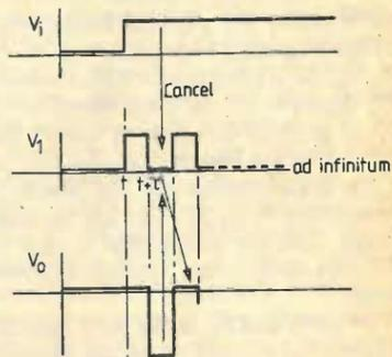
In the second case  $k_1 > 0$  we can obtain finite regenerative amplification under the condition  $0 < k_1 < 1$  i.e.  $R_2/R_1 > \mu - 1$ . The diagrams for the graphical analysis are easier to construct using equation 9:
