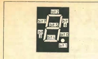
Fig. 1. Bit/segment allocations of Picotutor display.
