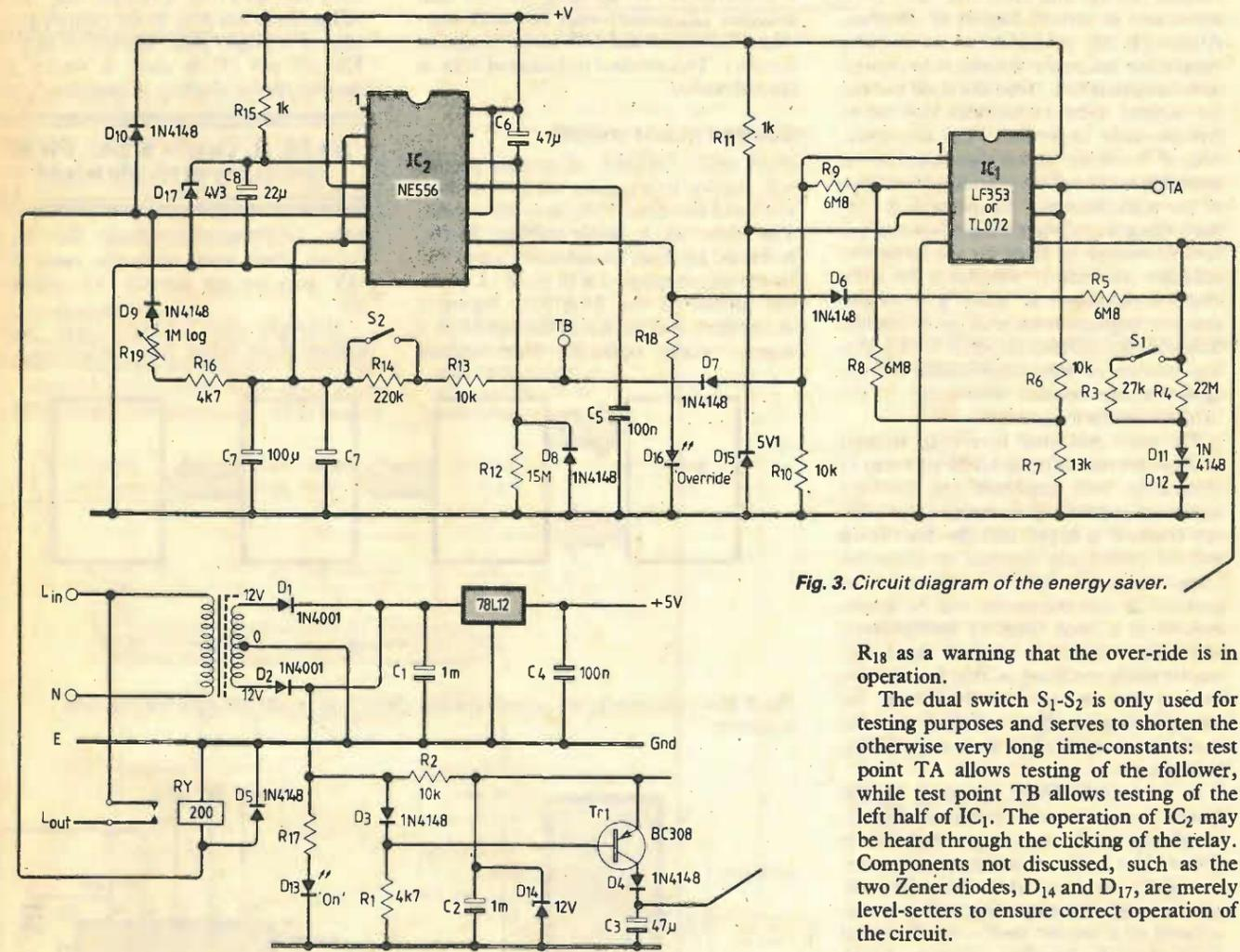
Fig. 3. Circuit diagram of the energy saver.
