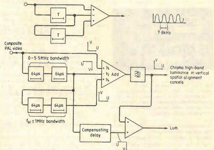
Fig. 11(b). Block diagram of a filter operating over a three-line period with 1/4:1/2:1/4 contribution from the outer lines (top) or across five lines in the ratio 1/4:1/2:1/4 i.e. lines N, N+2, N+4, (bottom).
