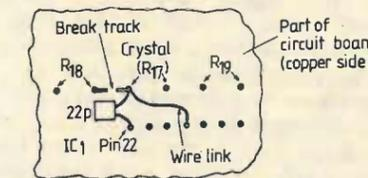
Fig. 6. Hardware modifications to Picotutor to allow more accurate timing using a crystal reference. Some reprogramming is necessary, see text.
