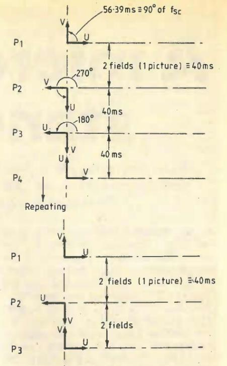
Fig. 14. By raising colour subcarrier by 6.25Hz, perfect decoding of still pictures free of cross-luminance and cross-colour can be obtained using one 625line picture store.
