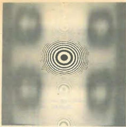
Fig. 12(c). Using a zone plate test signal the display shows luminance comb operating across three lines in one field, illustrating loss of diagonal resolution. The 'returned' resolution within the boxes is inverted, but is not significant on pictures.
