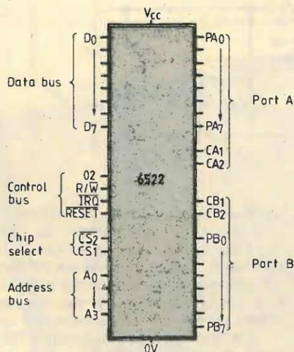
Fig. 2. Rockwell 6522 versatile interface adaptor. Only port A is used in this application.
