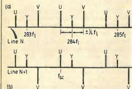
Fig. 5. Y, U and V spectra combined and simplified. Bringing these U and V spectrum diagrams together, but simplifying them by not showing the decaying picture-rate sidebands, results in (a). U has a quarter-line offset (low) with respect to the Y signal spaced at multiples of line frequency. V has a quarter-line offset above the multiples of line frequency. Note, there is no spectral peak component dominant at the half line frequencies.
