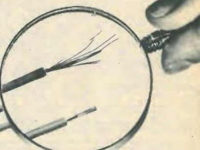
Stripping small cable with anything but the correct tool can cause unseen damage, and a damaged conductor can be a hidden hazard.
