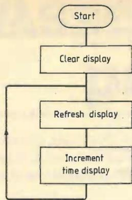
Fig. 2. Flow diagram for a software timer.
