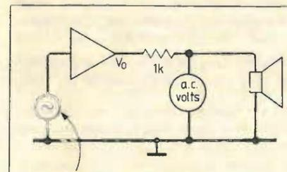
Variable frequency sinusoidal signal source, adjust so  $V_0 = 10V$
