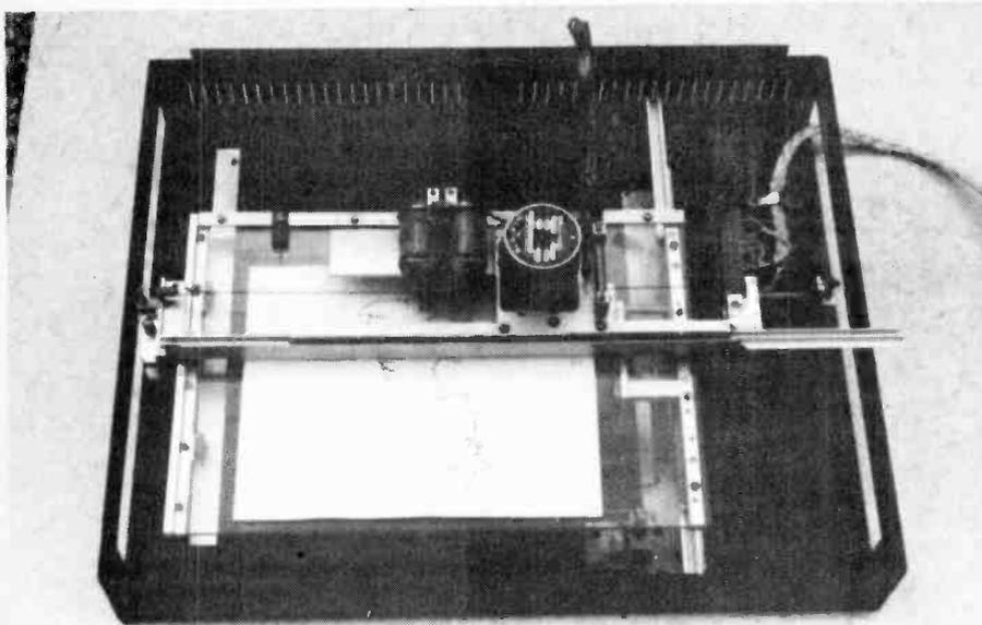
Fig. 12. Shows the completed plotter with a map of a well known country drawn on the machine earlier.
