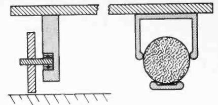
Fig. 11. Slider mechanism. Two ball-bearings are used in each slider.
