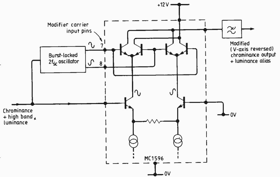
Fig. 18. Pal chrominance modifier with  $2f_{sc}$  oscillator locked to incoming burst using MC1596 i.c.
