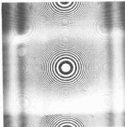
(e) 5.25MHz system b.w. limit Notch at  $f_{sc}$
