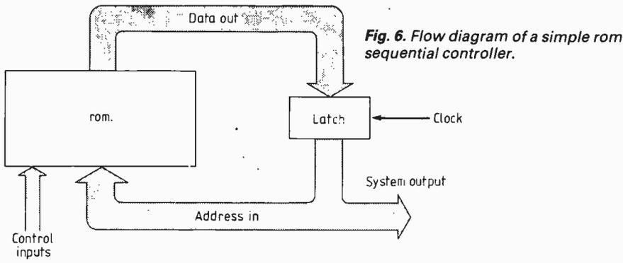
Fig. 6. Flow diagram of a simple rom sequential controller.
