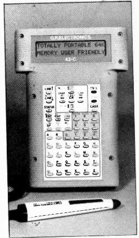
Nominally a hand-held terminal, the 42-C from G.R. Electronics has many inbuilt functions associated with a portable computer.
