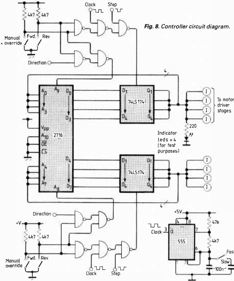
Fig. 8. Controller circuit diagram.
