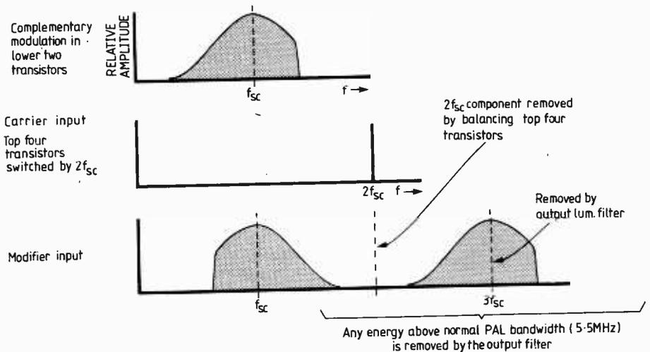
Fig. 19. Modifier chrominance signal envelopes show reversing of the sidebands as the carrier input is high w.r.t. the video signal.
