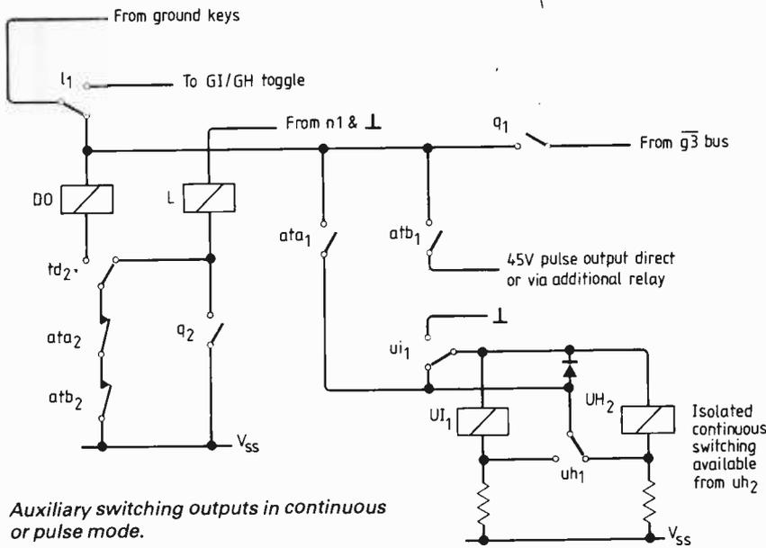
Auxiliary switching outputs in continuous or pulse mode.
