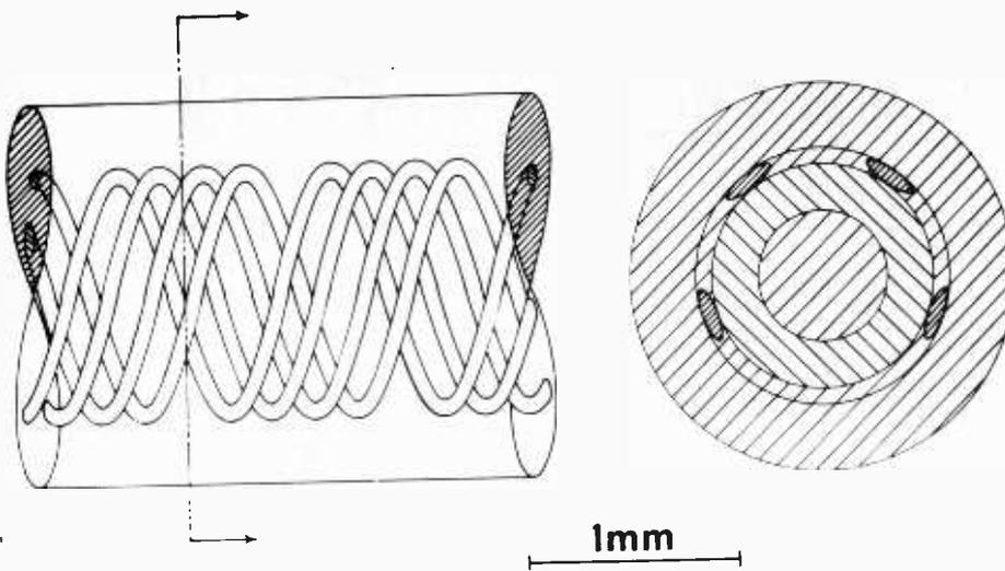
Fig. 7. Construction of connecting cable. The insulated helical conductors are wound on a silicone rubber tube and covered with an outer layer of silicone rubber adhesive.
