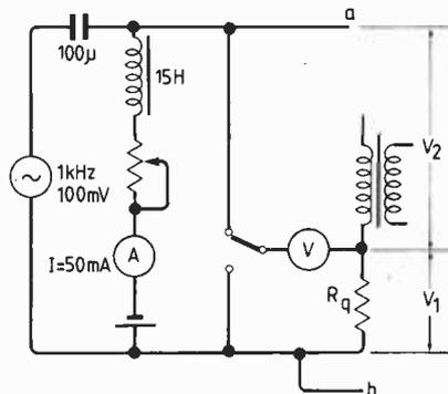
*Test circuit for determination of  $rg$  value. Connect to line interface and select  $rg$  for  $V_1 = V_2$ . Impedance is 600 ohms  $\pm 20\%$ .*
