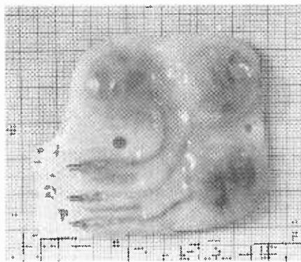
**Fig. 3.** (a) Complete three-receiver implant after encapsulation in silicone rubber. The three plugs mate with sockets on the implanted cable. (b) The corresponding oscillator block as used by the patient.
