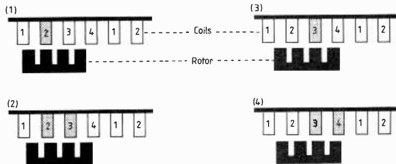
Fig. 1. Internal configuration of a typical four-pole stepper motor. The sequence shows how the half stepping is achieved.
