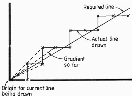
Fig. 16. Plotting a straight line by approximation of the gradient.
