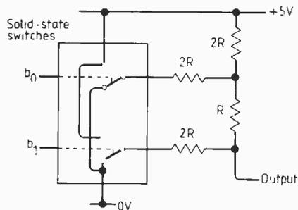
Fig. 1. Basic digital-to-analogue converter circuit. Two digital input bits,  $b_0$  and  $b_1$ , are converted to one of four output levels using an R-2R network. Bit  $b_0$  is the least-significant digit of a binary word and  $b_1$  is the most significant.
