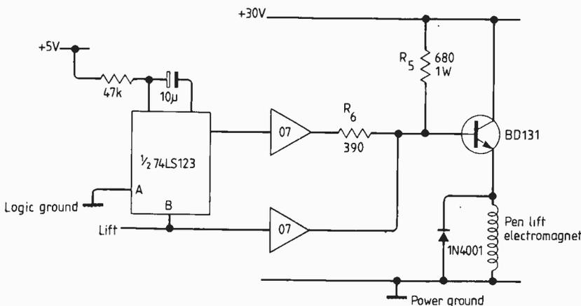
Fig. 9. Pen lift control electronics.
