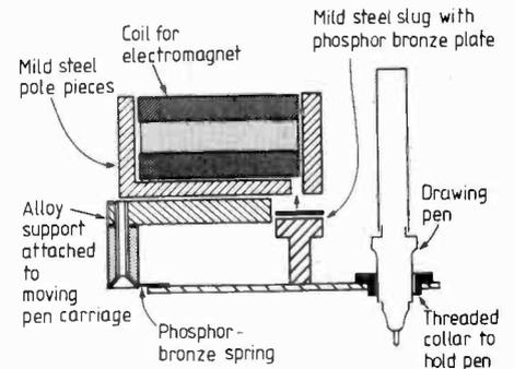
Fig. 14. Cross-section of pen lifting mechanism. More than one can be used to provide different coloured pens.
