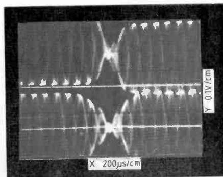
bands generated are large. Residual error is shown in the bottom trace, Y-out, (b). Some is also due to the changed rise times of the subtracting chroma transitions due to the reduced bandwidth of the chrominance signal. Comparison of the two traces at (a) shows this rise time difference. Colour print 5 shows the effect of the reduced rise time on the chroma-only display.
