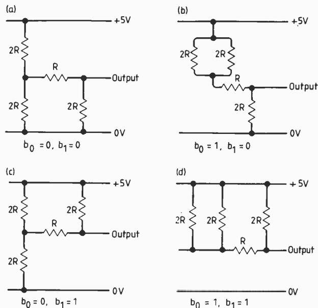
Fig. 2. Equivalent circuits of the network shown in Fig. 1 for the four input permutations.
