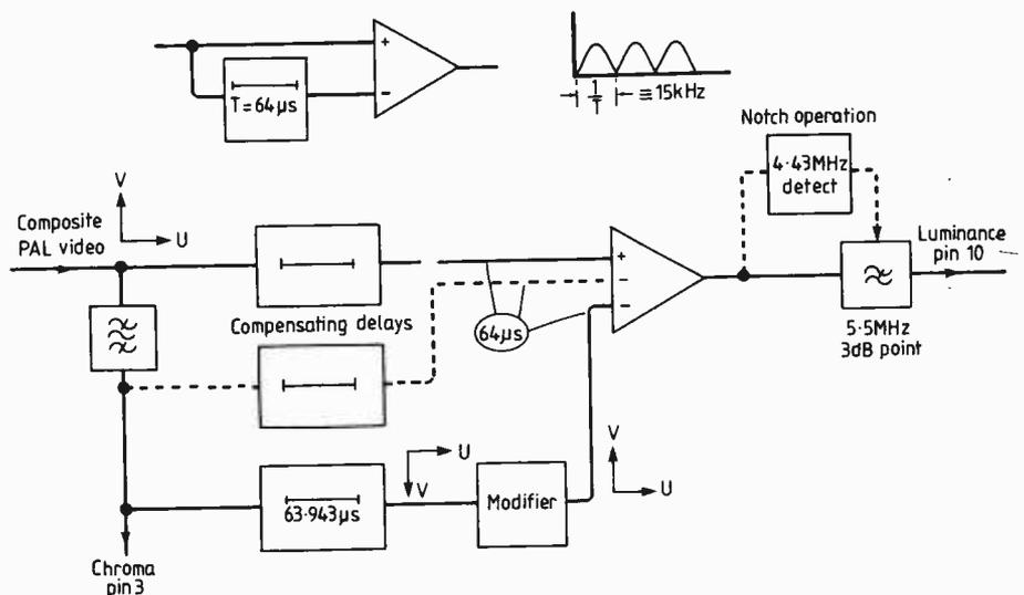
**Fig. 20.** Combing across adjacent lines with the aid of the PAL decoder (page 54, bottom). Block diagram of the PAL decoder is for Mullard one-chip decoder TDA3561A (or 3560). Components within broken-line area are replaced by diagram on p.54; pin 10 is luminance input, pin 3 chroma input.
