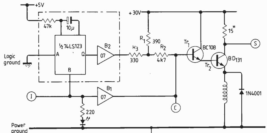
Fig. 2. Motor driver circuit. The enclosed section is required only once for each motor.
