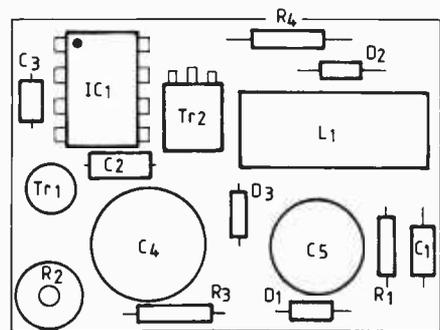
of 0.5mm wire wound on a Neosid 14mm powdered-iron toroid was used for the prototype output choke. Copper on the top surface of the p.c.b. is soldered to the fet drain terminals to act as a heat sink.
