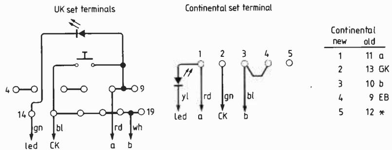
*Modifications for connection of UK or Connection to public network for UK (left) and Continental sets. For UK sets, remove straps 5, 6, 17 and 18 in telephone. Change around green/white strap in terminal block and connect blue wire to tag five in telephone. In Continental telephones, change green wire from point two to point five and connect 'a' to the socket ground strap.*
