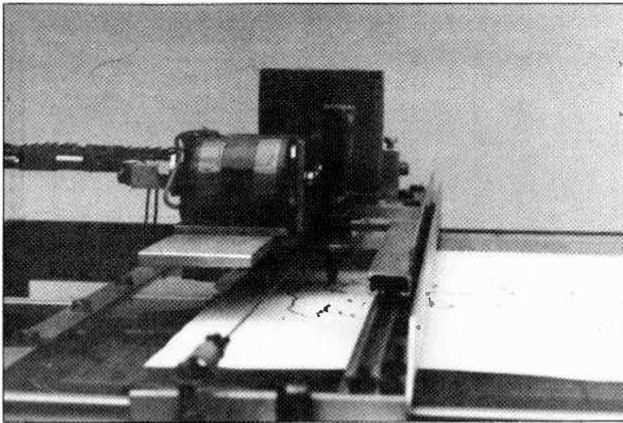
Fig. 15. The pen carriage with the lifting mechanism. The stepper motor is visible behind the pens.
