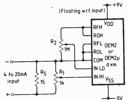
d.v.m. As shown in the modified circuit  $R_S$  converts the 4-20mA signal into an input voltage of between 60 and 300mV.  $R_1$  provides full-scale calibration control and is adjusted to give a 40 to 200mV input. A 40mV offset derived through  $R_2$  from the stable 100mV reference at ROH is injected between COM and INLO. The differential voltage between INLO and INHI now gives the desired display range of 0rev/min at 4mA/40mV rising to 1600rev/min at 20mA/160mV input.
