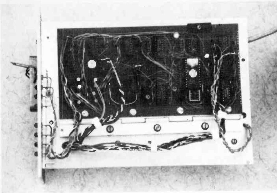
Fig. 10. Controller p.c.b. Interconnections are made with wire-wrap wire from pins on the component side.
