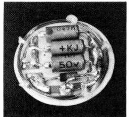
Fig. 2. Circuit (a) and construction (b) of one of the three receivers in the chest implant.
