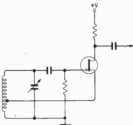
Fig. 1. Output level of this simple oscillator varies with frequency and the tapped coil makes range-switching complicated.
