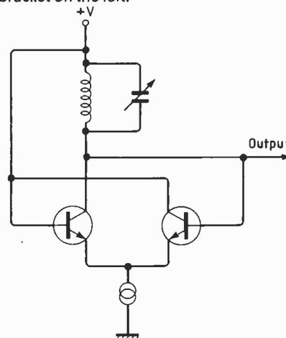
Fig. 2. This more complex design is similar to the oscillator in the TDA1072 i.c.
