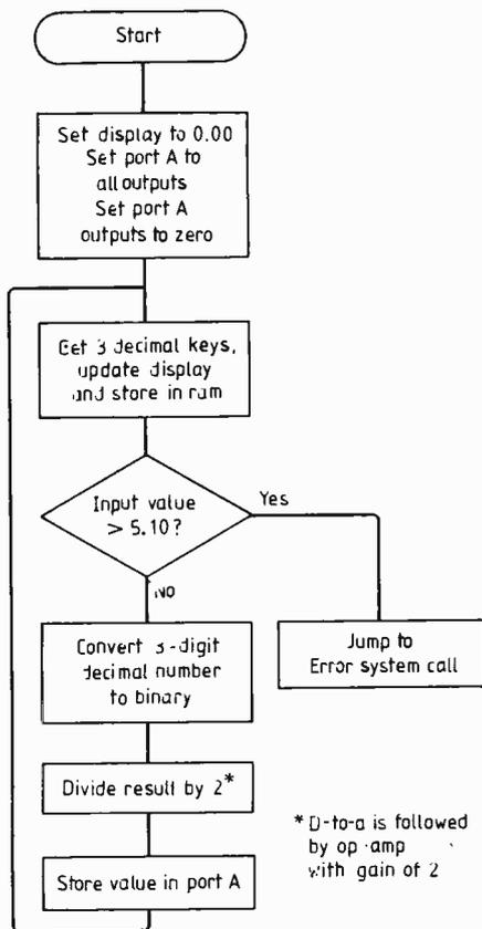
Fig. 3. Picotutor contains a program for converting three decimal digits entered on the keypad to binary form. This binary value is sent to the digital-to-analogue converter board through port A.
