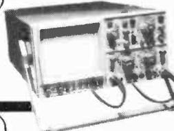
**Hameg HM 204 20MHz Oscilloscope £365** High performance instrument with sweep delay. Versatile triggering to 50MHz, variable hold off control, Z modulation and internal illuminated graticule.
