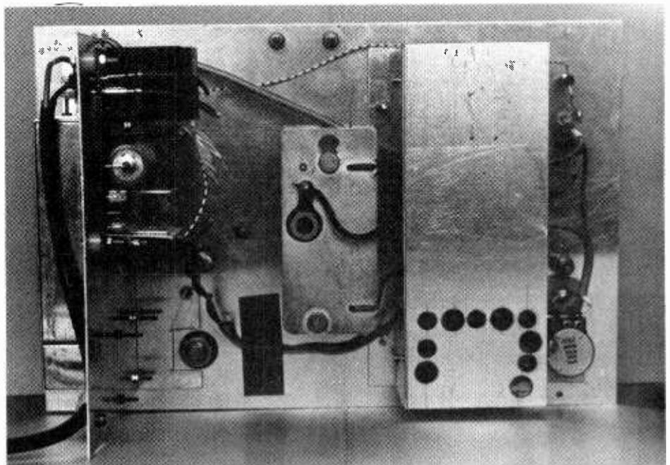
Rear view of the assembly: the r.f. generator board is enclosed in a screening box and the power supply is fixed to a bracket on the left.
