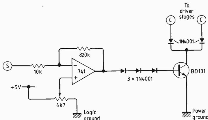
Fig. 4. Driver protection circuitry.  $RV_1$  sets maximum output current.
