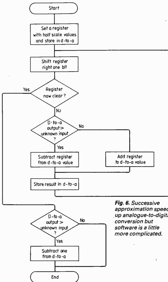
Fig. 6. Successive approximation speeds up analogue-to-digital conversion but software is a little more complicated.
