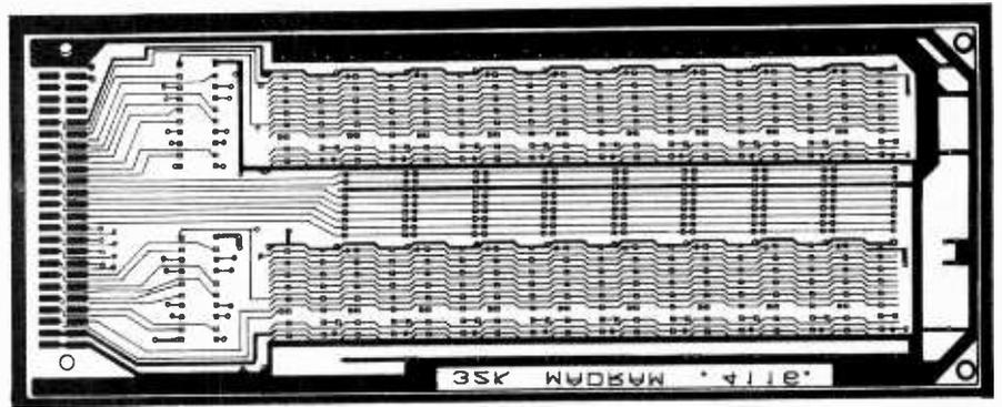
Fig. 21. Artwork for a memory board. All bus interconnections were drawn by the plotter.
