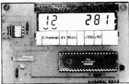
**Fig. 2.** Contents of channel 12: input has spent 281 units of ten seconds in the range of channel 12 - 36,000-38,999 in this case. Channel contents rise from 0 to 99,999, after which 10,000 is displayed, with the arrowed annunciator pointing to  $\times 10$ , etc.
