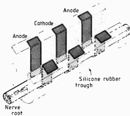
**Fig. 5.** Construction of electrodes for one nerve root. The middle platinum foil electrode is a cathode while the outer ones (connected together) form an anode.
