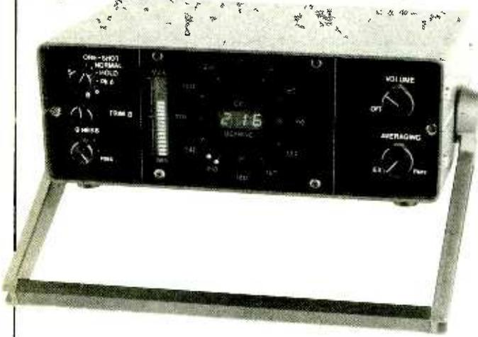
calculation to the bearing is handled by a Z80 processor, which is also used to drive the display. The phase-shift caused by signal delay through the receiver is automatically compensated for to give a superior performance than that in most Doppler-shift direction finders, according to the maker.
