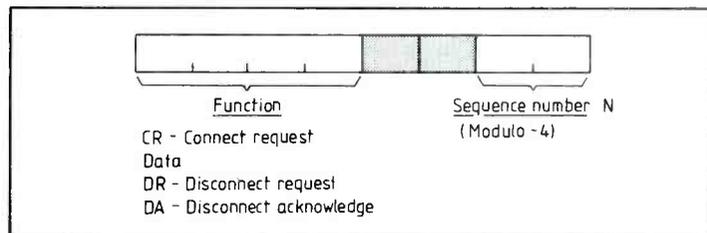
Fig.6. Link control byte. This byte in each packet contains one of the function codes shown and a two-bit sequence number field which is only used in data packets.
