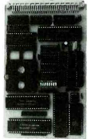
The CARDMASTER CPU1 card is equally suitable as a Single Board Controller or the heart of the CARDMASTER system. The CARDMASTER CPU1 is supplied with a powerful three way operating system.
