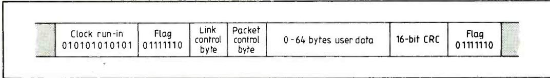
**Fig. 3. Packet format. High-level synchronous data link communication, HDLC, is a bit-oriented serial communication protocol. A transmission packet is recognized by a flag at its start.**
