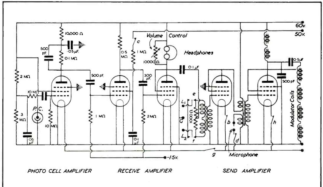
Fig.4. Circuit diagram of the amplifiers.
