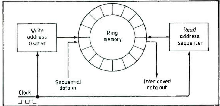
Fig. 3. De-interleave is achieved by the use of a ring memory which is addressed linearly on one side and by a sequencer at the other side. Timebase correction may also be performed by the same unit.
