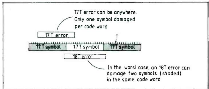
Fig. 4. The odd-even symbol interleave ensures that a 17T error causes no more than one symbol in error in each of two code words, wherever the error is. The worst case for an 18T error is that two symbols are damaged in one code word. Thus errors in excess of 17T must be regarded as burst errors.
