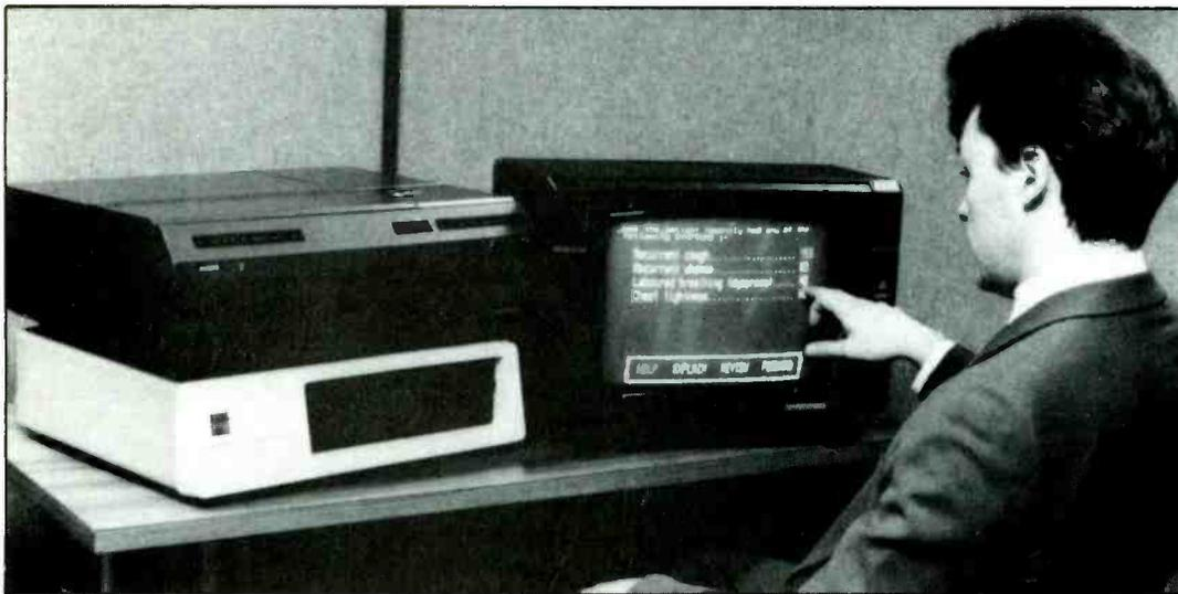
Expert systems are a compilation of the knowledge of specialists in a particular field. Under computer control, they can offer diagnosis, analysis and can offer remedial action. Adept, developed by Marconi Instruments and Allen & Hanbury, is used to diagnose sufferers from asthma. It has a touch-sensitive screen for input.
