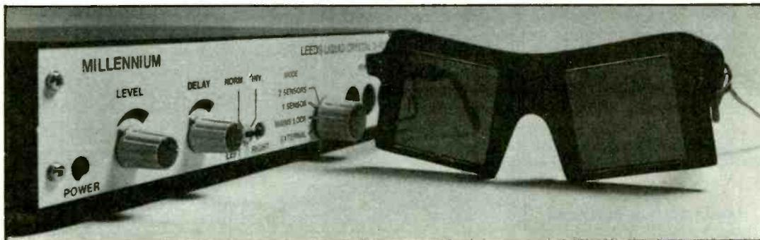
long axes of molecules perpendicular to the field with an h.f. pulse applied at a suitable time. This is made possible by choosing a material having a permittivity in the direction perpendicular to the molecule greater than that in the parallel direction. (The material actually used, supplied by RSRE, had a  $\Delta\epsilon$  of 2.95 at 200kHz and -1.8 at 100kHz, crossing over at 5kHz.)
