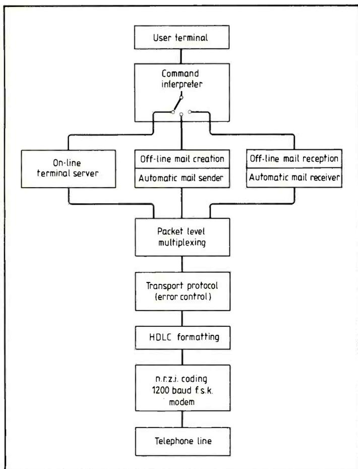
**Fig. 2. System hierarchy. The 1200 baud modem is an integral part of the mailbox. Careful choice of protocols and error-checking methods results in efficient and reliable communication.**
