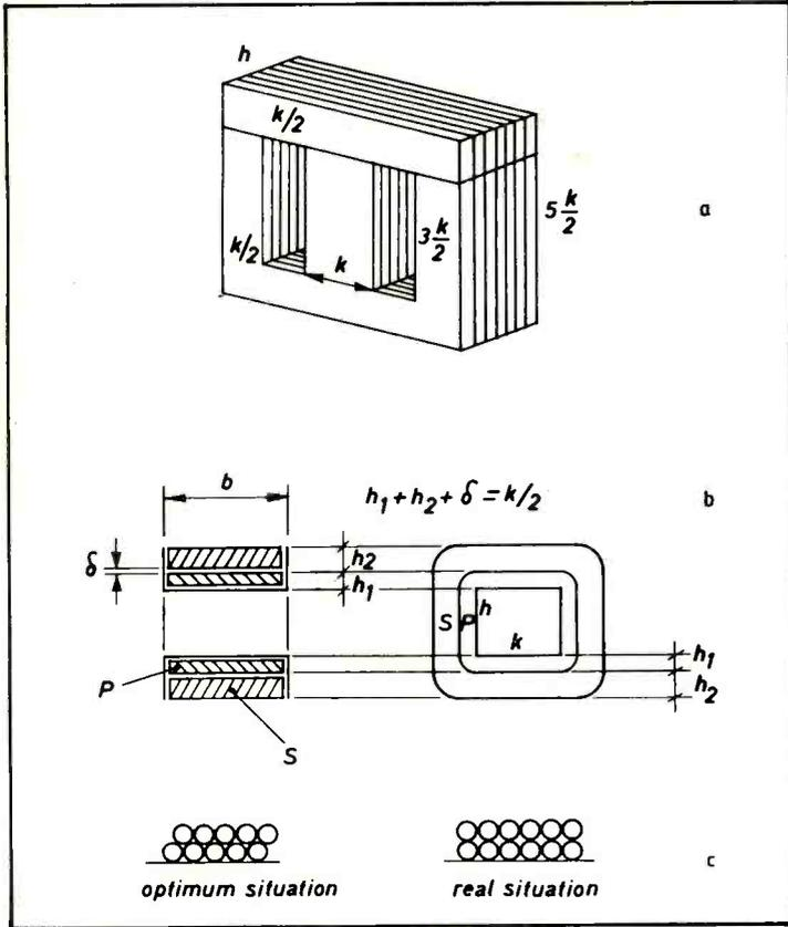
Fig. 1. Typical E-I stack of laminations at (a). Calculating mean turn lengths shown at (b), and at (c) are the ideal and practical lays of turns.
