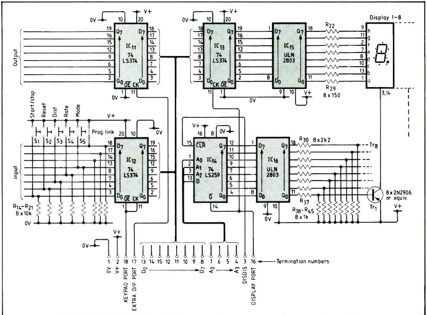
Fig. 1. Display board. Details of the processor board were given in last month's article.
