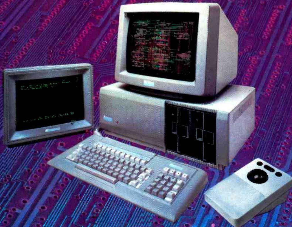
CAD-8 is a low cost easy to operate system specifically designed for creating accurate two dimensional multilayered P.C.B.'s using high-resolution colour graphics.
