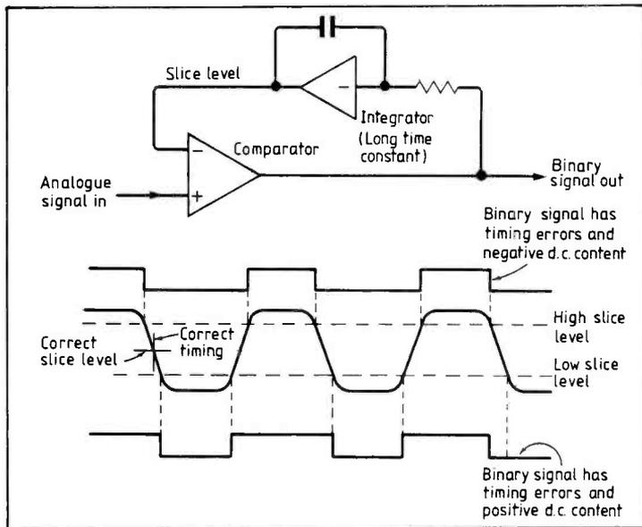
Fig. 2. Self-slicing a d.c.-free channel code. Since the channel code signal from the disc is bank limited, it has finite rise times and slicing at the wrong level as shown here results in timing errors, which cause the data separator to be less reliable. As the channel code is d.c. free, the binary signal when correctly sliced should integrate to zero. An incorrect slice level gives the binary output d.c. content and, as shown here, this can be fed back to modify the slice level automatically.
