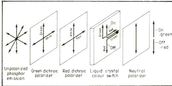
manufacturing tolerances. The technique is still only used in the model 5116 colour display oscilloscope and could clearly be applied in other traditionally 'mono' display situations; however Tektronix say their shutter is not available for use outside the USA.
