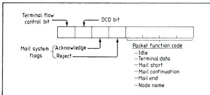
Fig.7. Packet control byte. The second byte after the flag in each data packet contains higher-level information about the data following.
