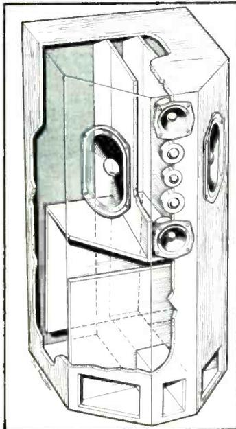
transmission-line system in the light of new materials and manufacturing procedures. TDL Electronics, Unit 11, Hampton Lovett Industrial Estate, Droitwich, Worcs WR9 0NX. EWW206
