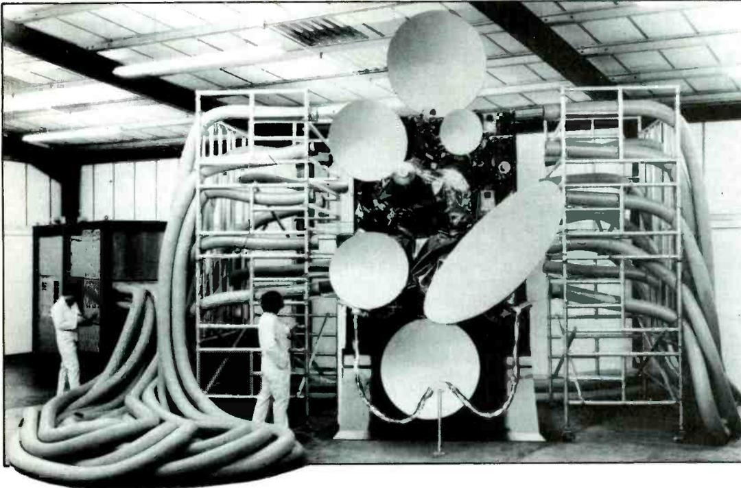
Medusa is a complex of heaters and coolers which can offer a satellite under test all the temperature changes that it is likely to encounter in space. It is shown here with a mock-up of the Olympus communications satellite from BAe which will be tested in this way. Medusa comes from Dynam Engineering in Blackburn.
