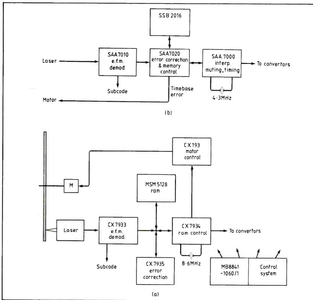
Fig. 5. Shows the l.s.i. chip arrangement of Sony's first generation CD player, contrasted with the Philips equivalent.
