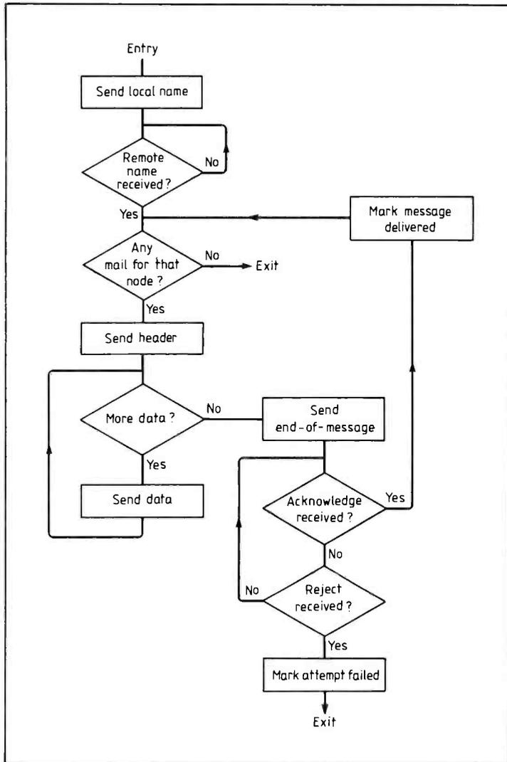
Fig.8. Simplified flow diagram of the mail sender, which is activated each time that the system is ready to send a new packet and has no terminal information to send.
