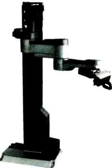
RTX arm displays the SCARA principle with vertical axes and horizontal movement.
