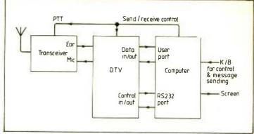
Fig. 9. How the d.t.u. interfaces with two transceiver and computer.
