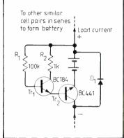
In a battery, the cells are grouped in pairs as shown. Normally the combined cell voltage keeps  ${\rm Tr}_2$  switched on. If voltage falls below  $1.3{\rm V}$  — which is equal to two diode voltage drops and one cell voltage — then  ${\rm Tr}_2$  turns off. The voltage across one cell cannot become negative. Optional diode  ${\rm D}_1$  allows other cells in the battery to function when this cell pair has cut out.
