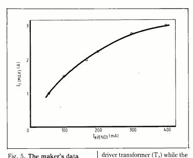
Fig. 5. The maker's data regarding base current requirement, given graphically.
