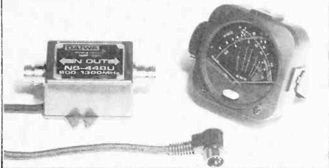
Frequency range 900 to 1300 MHz, impedance 50 ohms, power range forward 5/20W, reflected 1.6/6.6W, connections N type.
