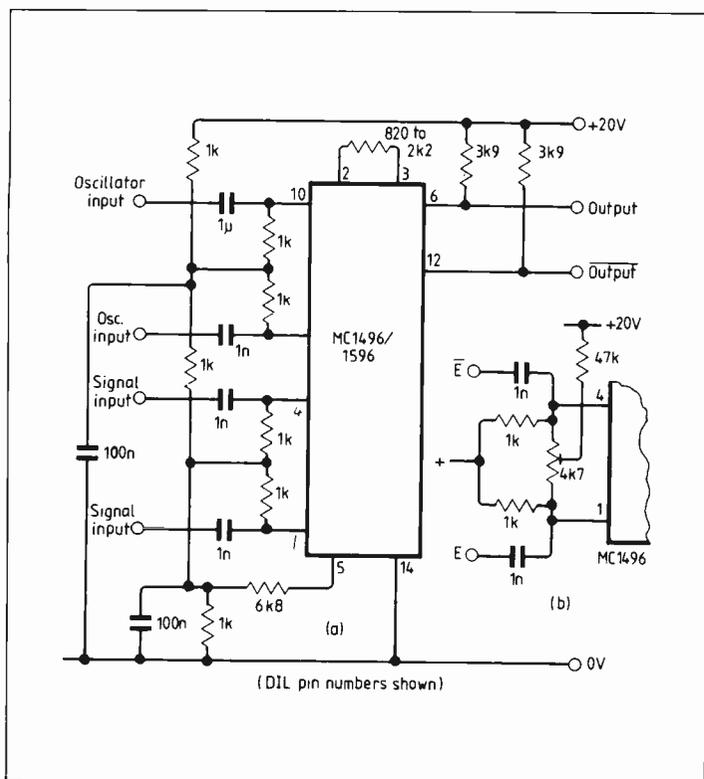
**Fig. 8. Use of MC 1496/1596 as double balanced demodulator, with single-supply operation is shown at (a). Method of nulling spurious responses is at (b).**
