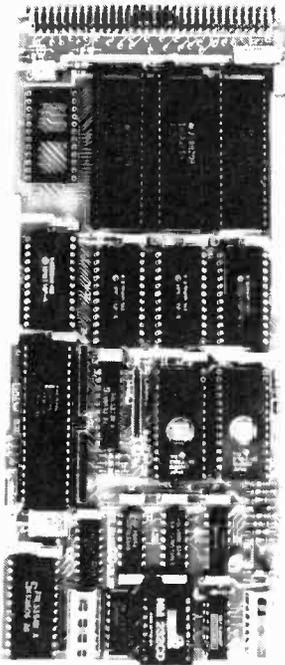
Based on the Intel 8052AH single component Microcontroller the CPU comes complete with a unique implementation of the BASIC language enabling direct access to the special function registers, timers and interrupts available on the 8051 device.
