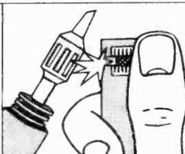
Flint ignition system built into the cap.
