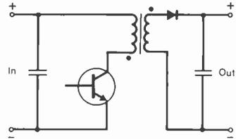
A transformer with a specific inductance stores energy while the transistor is on. The energy cannot be passed to the secondary output as it is blocked by the diode. When the transistor is cut off, the stored energy is
