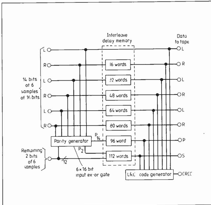
**Fig. 6. In 16bit mode, 14 of the bits of each sample are stored as words (L, R) and the extra two bits of each sample stored as 12bits of another word. Parity is generated on the 16bit data, and 14 of the parity bits are stored in the P-word. Remaining two bits are added to the 12bits of sample data to complete the S-word.**
