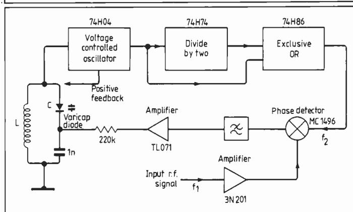
Fig. 2. Phase-locked loop using practical devices
