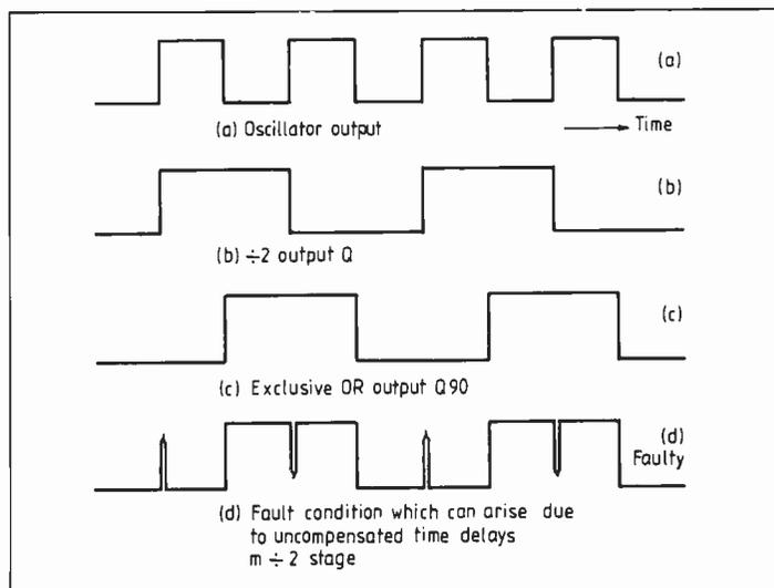
Fig. 3. Time and phase relationships of quadrature generator
