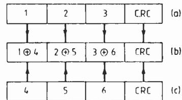
**Fig. 5. In this one 35-line interleave block of 1610/1630 format, block is divided into three sections of  $11 \frac{2}{3}$  lines each, two data, one parity. Three passes through the interleave memory are needed to create the signal structure (1, 2, 3). Large L/R interleave allows interpolation if dropout exceeds  $11 \frac{2}{3}$  lines.**
