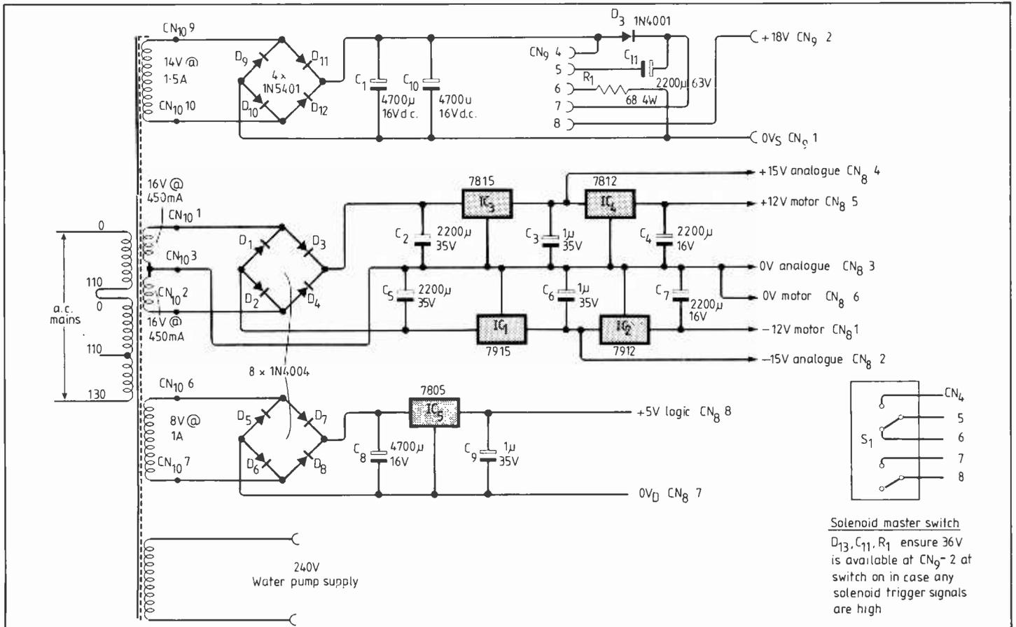
provides regulated supply rails of +5V, +15V, -15V for the computer interface board, +18V unregulated for the solenoid driver board and 240V for the pump.
