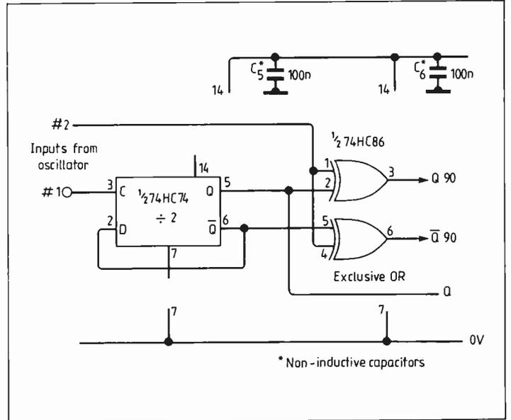
Fig. 5. Quadrature waveforms generator
