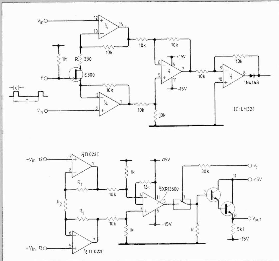
the transconductance of the op-amp where  $g$  is  $I_c/2V_T$  which is  $19.23I_c$ ; control current  $I_c \leq 2mA$ .
