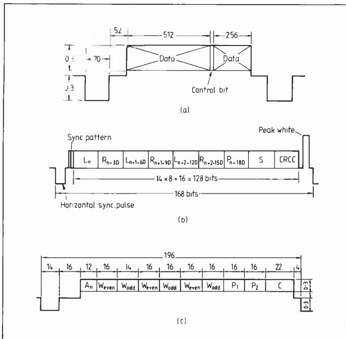
**Fig. 3. Video line from PCM1610 has control bit that determines the use of pre-emphasis and selection of 44.1 or 44.0559kHz (a). Note peak white ref. In video line from PCM-F1 in 16bit mode (b) and address at beginning of video line from JVC unit (c).**
