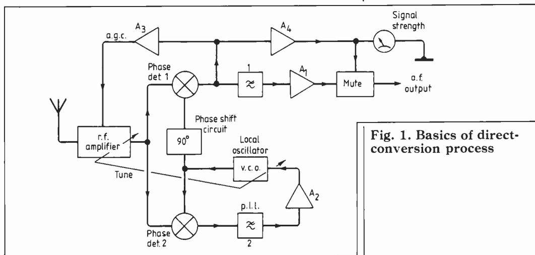
Fig. 1. Basics of direct-conversion process
