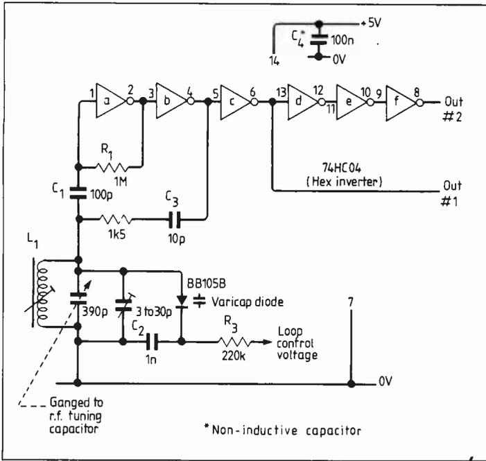
**Fig. 4. Phase-locked local oscillator**
