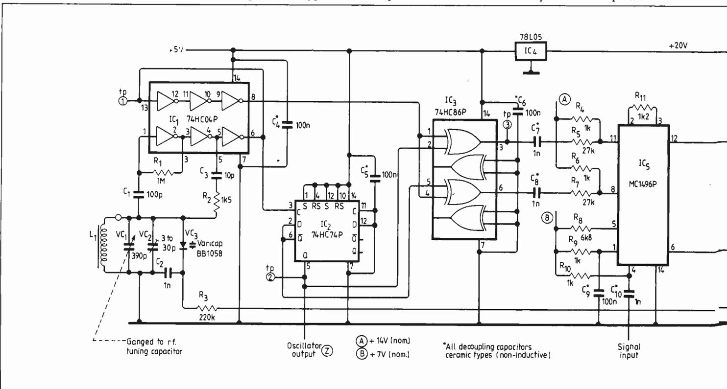
**Fig. 7. Complete phase-locked oscillator**
