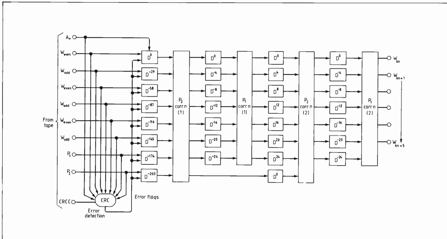
**Fig. 8. De-interleave and correction diagram for JVC format. Depending upon distribution of errors, it may be better to correct with either P1 first or P2 first: multiple re-interleave and de-interleave allows both choices. See text.**
