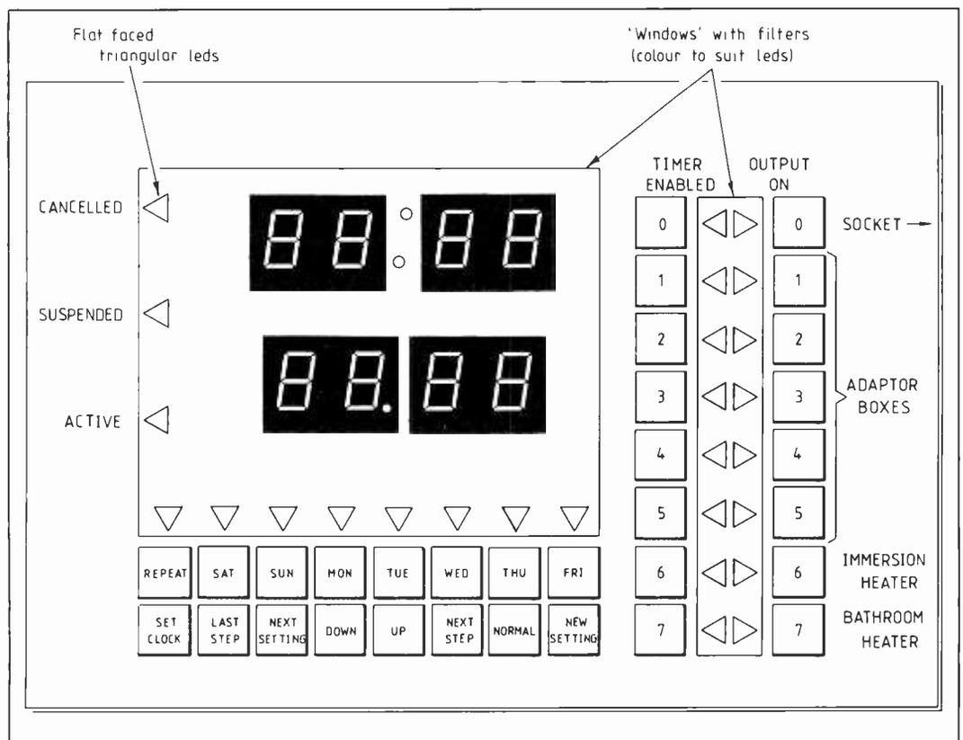
turn. The display in this mode shows on and off times, day, channel and either active or suspended. For non-repeated settings the last day flashes.
