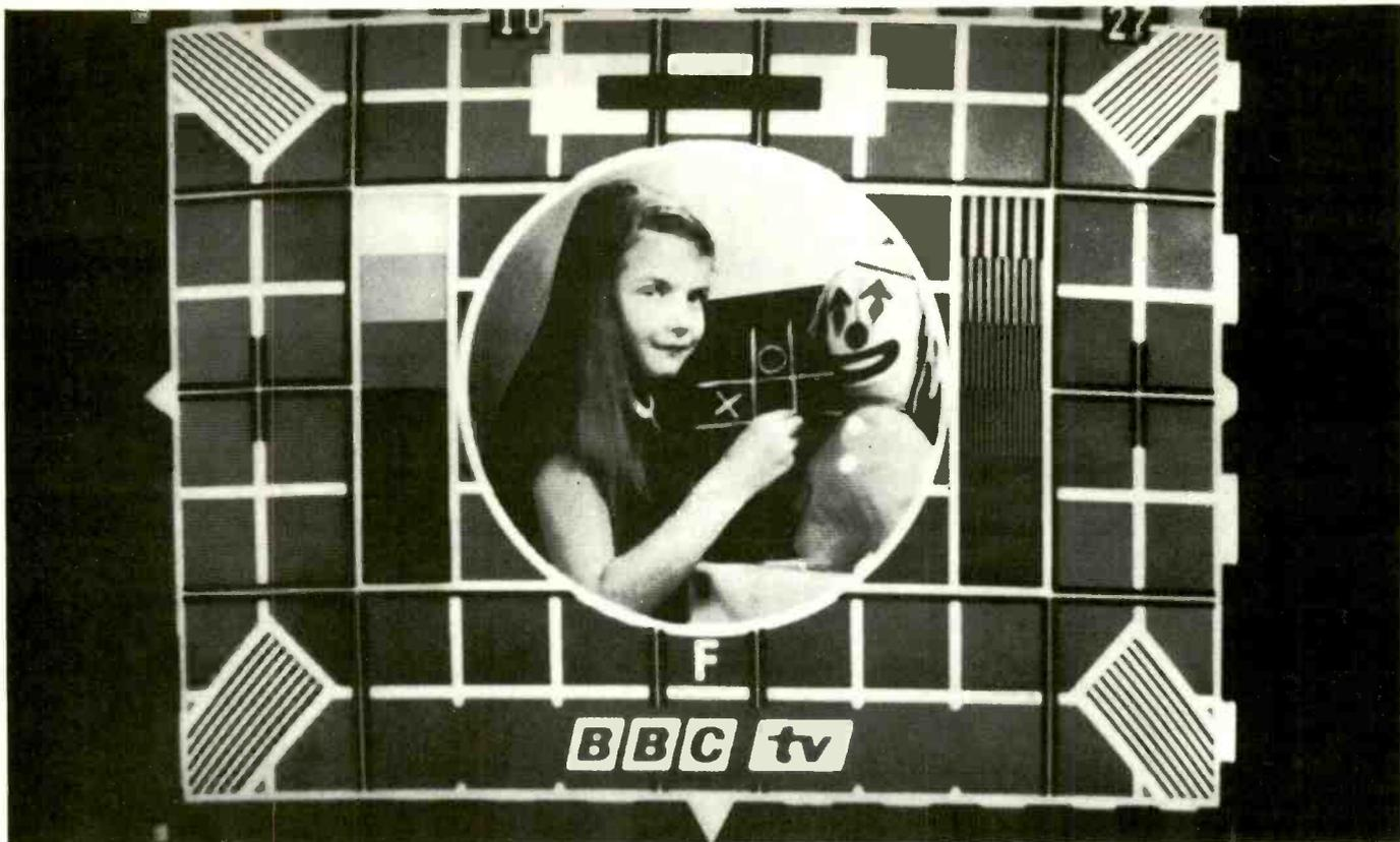
Fig.6. Split-screen picture with two apertures. Apertures 10 (left half) gives vertical aliasing visible in the diagonals, while aperture 27 virtually eliminates the aliasing.
