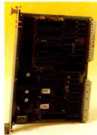
One of Kemitron's first boards which takes advantage of the double eurocard design is a processor card with Hitachi's 6MHz 64180, 768ram, dma, four serial channels, floppy and hard-disc interface, maths processor, counter/timer and r.t.c. with battery. Two interface cards are also available which are a 64/32 channel analogue input with eight analogue outputs and a 32-channel opto-isolated input/output board with 10-channel c.t.c.
