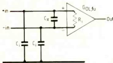
Fig.2. Active component models used with in Analyser. Hybrid-pi bipolar-transistor model (a), field-effect-transistor model (b), and operational-amplifier model (c).
