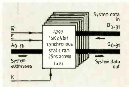
Fig.3. Internal structure of an MCM6292 synchronous static ram. Write-pulse logic required for standard static ram is on chip so fewer external control components are needed.
