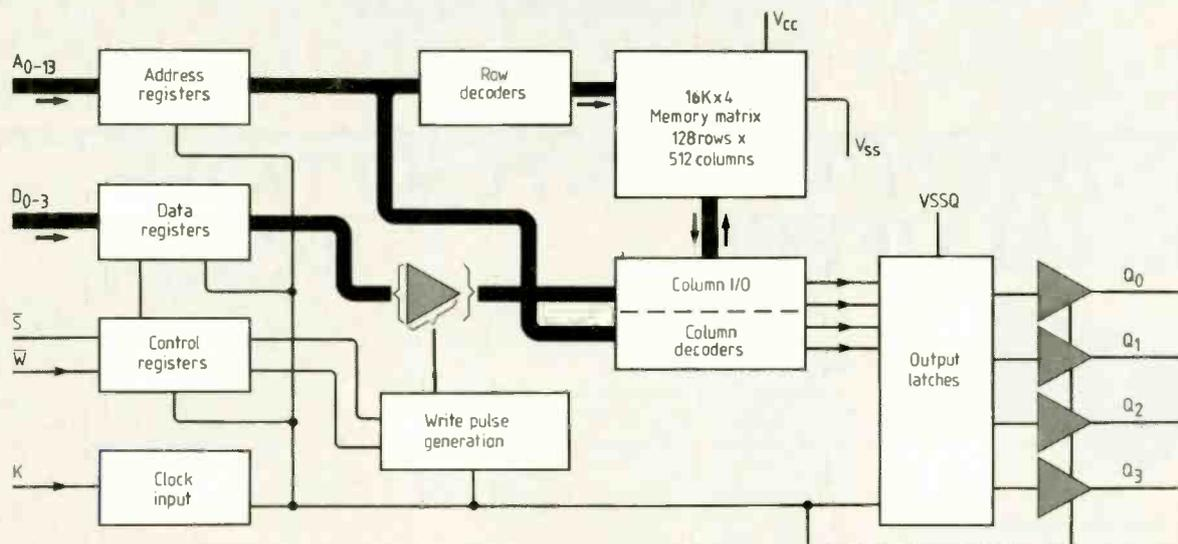
nal logic to interface them to the microprocessor, as Fig.2 shows. Internal elements of the synchronous static ram are illustrated in Fig.3.
