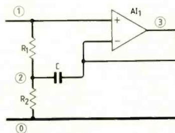
1. Literal analysis of this circuit immediately shows those components affecting performance. e.g.  $Z_{in} = (R_1 + R_2) + j\omega R_1 R_2 C$ .
