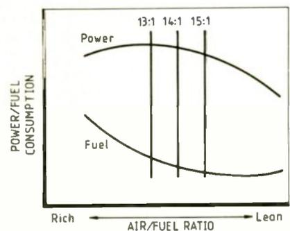
Fig.1. For minimum emission of carbon monoxide and unburnt hydrocarbons, an engine must work at the stoichiometric air-to-fuel ratio of 14:1. This means striking a compromise between maximum power and minimum fuel consumption.
