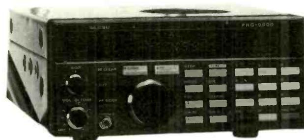
• All Band Capability. LW, MW, SW, VHF/Low Air-band, 137-Satellite, HF/High, Military, UHF/Low, UHF/High, TV, UHF-CB, Cellular. (All Broadcast, Air, Marine, Amateur, Business Radio, Military, TV, Cellular, up to 950MHz). This unit is now suitable for use in any country as all bands/channel steps are now available.
