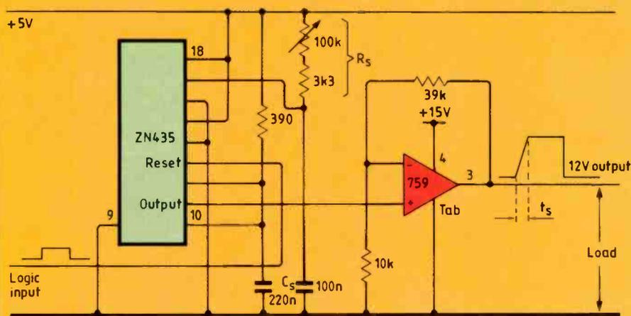
cuit provides control of the switch-on ramp using a d-to-a converter.
