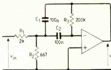
2. Literal analysis of an active bandpass filter circuit gives a voltage transfer function which can be adjusted to the required value by altering components and evaluating the result.
