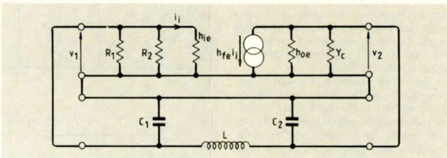
Fig.4. The first step replaces the transistor with its h-parameter equivalent as before. The feedback path via the L-C circuit forms another four terminal network.
