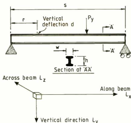
**Fig. 1. Deflection of an elastic beam by vertical loading.**
