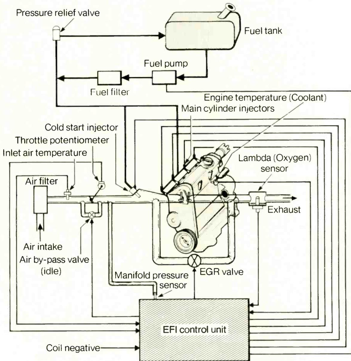
done by modifying either the ignition timing or the intake of air, but it is most effectively done by modifying both together. A fast response is then achieved by modifying the timing (as air intake has a relatively slow response time) and dynamic range is obtained by controlling an air by-pass valve on the throttle. Timing varies idle speed only within very tight constraints and to the detriment of emissions.
