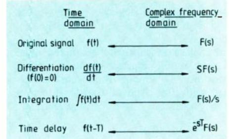
Fig.2. A few important results demonstrating the equivalence of time-domain and frequency-domain signal processing.
