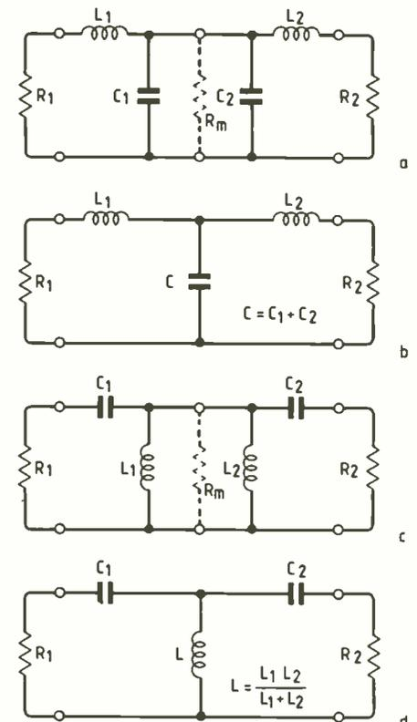
Fig.6. When two L-sections combine in various ways, all the interesting T and  $\pi$  circuits can be derived. In (a) the two Ls form a T network, as shown in (b). (c) and (d) show the high-pass version of the same T-network.
