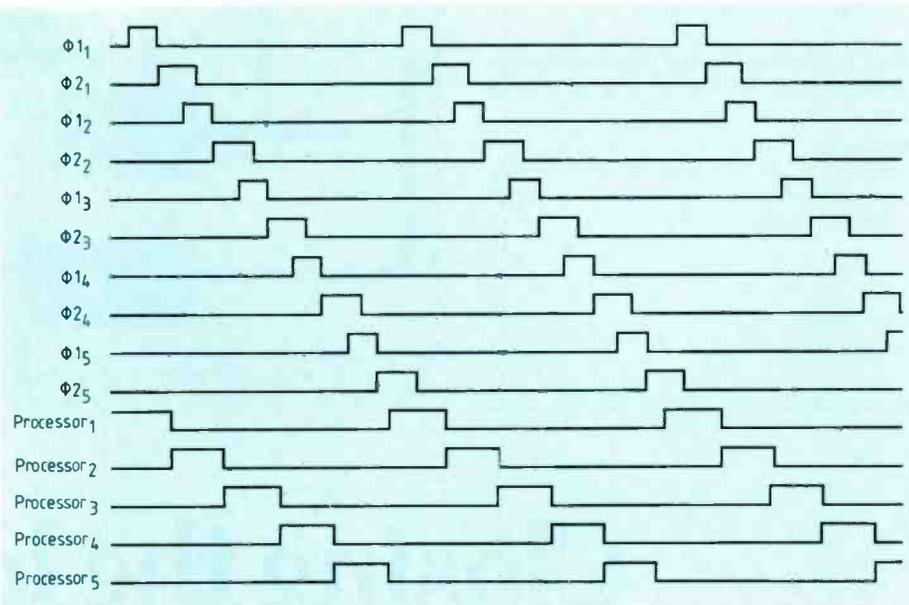
Asynchronous buses readily accommodate different types of processor running at different speeds whereas with a synchronous bus all of the processors must run at the speed of the slowest processor, reducing overall performance.
