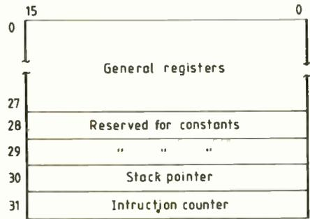
Fig.7. Allocation of the demonstration processor's 32 registers.
