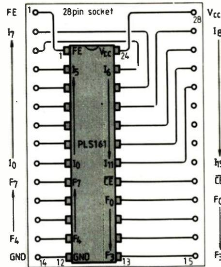
Device types other than the PLS100/101 can be programmed by making modifications. With minor software modifications, using a piggy-back socket like the one shown here allows 24-pin PLS161 p.l.as and PLS162/3 address decoders to be programmed.
