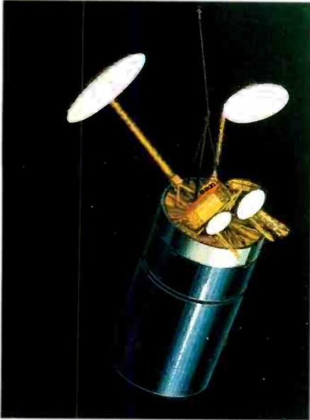
Above: artist's impression of the completed Intelsat VI, which is 11.8m high on-orbit. The satellite's complex channelization plan (right) employs six-fold frequency re-use.
