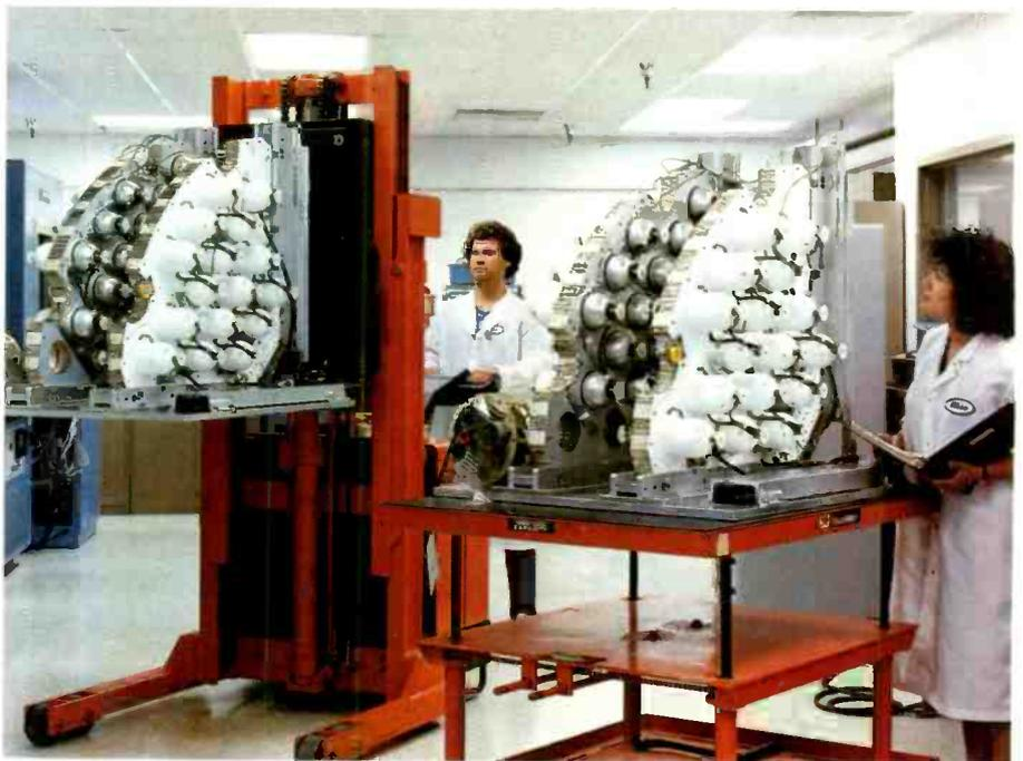
Sections of the C band feed array for Intelsat VI.
