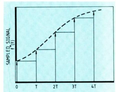
Fig.7. Modelling the sampled signal as a train of weighted pulses. The effect of the a-to-d converter is to take a sample in zero time and to hold this snapshot constant until the next sampling instant occurs one period later.
