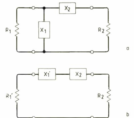
Fig.4. The transformation of the L circuit shown here employs the series-to-parallel conversion, which simplifies calculations considerably.
