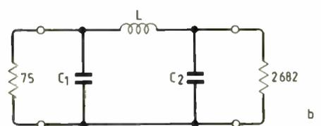
Fig.9. This shows a typical application. In (a) a non-resonant aerial and its terminal equivalent circuit is converted to the parallel form by the transformation. A  $\pi$  network then matches it to 75 $\Omega$ .
