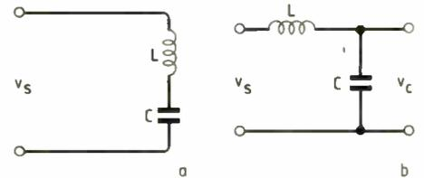
Fig.1. A series L-C circuit can be thought of as a reactive potential divider, as well as a resonant circuit.
