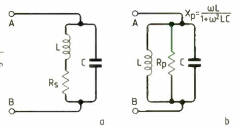
Fig.2. The parallel resonant circuit has some interesting properties, not least the fact that smaller and smaller  $R_s$  gives rise to a larger and larger  $R_p$ .
