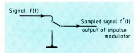
Fig.5. Periodic processing of a continuous time signal can be represented by this simple switching circuit. Asterisk notation denotes a periodic sampled signal occurring every T seconds.
