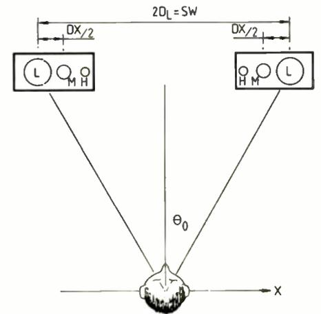
Fig. 2. Geometric arrangement of proposed method of improving image sharpness.  $\theta_0 = 30 \text{ degrees}$ ,  $SW = 230 \text{ cm}$ .
