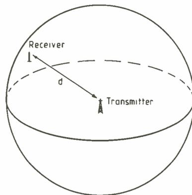
Fig.1. A receiver is located d metres from a transmitter. All the power radiated by the transmitter passes through a sphere of radius d. Power density at the receiver is therefore equal to the radiated power divided by the sphere's surface area.
