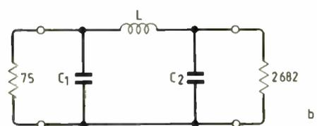
Fig.9. This shows a typical application. In (a) a non-resonant aerial and its terminal equivalent circuit is converted to the parallel form by the transformation. A  $\pi$  network then matches it to 75 $\Omega$ .
