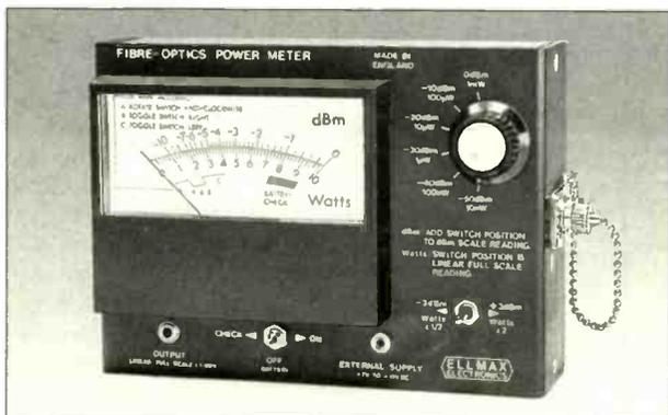
The Ellmax Fibre-Optics Power Meter is an accurate, sensitive, low-cost instrument, incorporating a pointer scale giving readings in both **dBm** and **μW**. It measures power levels from 1mW (0dBm) down to below 1nW (-60dBm) at its calibrated wavelength of 820nm, and contains a large area detector in a connector housing. Connector options include **SMA** and **STRATOS**. Battery life is typically **500 hours**.
