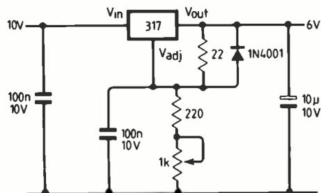
Fig. 4. Regulator i.cs provide some of the voltages needed to program the p.l.d.
