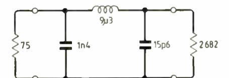
Fig.10 The final network for the aerial with values.
