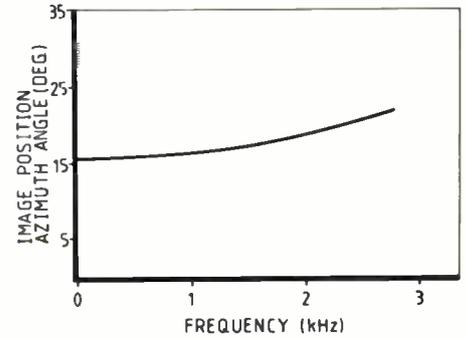
Fig. 1. Image position variations with frequency ( $R/L = 0.3$ ,  $D = 14 \text{ cm}$ ). Ref. 12.
