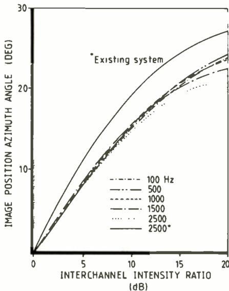
Fig. 5. Image displacements with interchannel intensity ratio in proposed system (60dB/decade filter).
