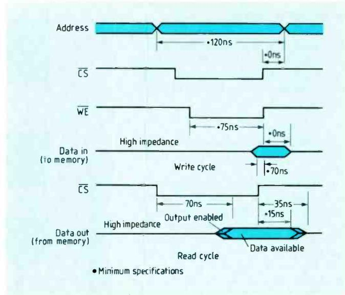
Fig.3. Memory timing specifications for 2114 static RAMs, top right.
