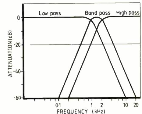
Fig. 4. Filter response characteristics.
