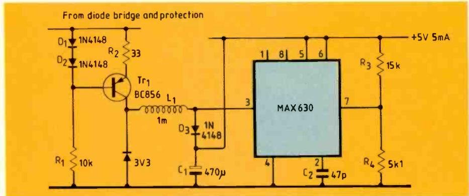
A Maxim MAX230 i.c. with its oscillator running at about 40kHz (set by  $C_2$ ) provides d.c.-to-d.c. conversion. Supply voltage determines whether the oscillator is on or off.
