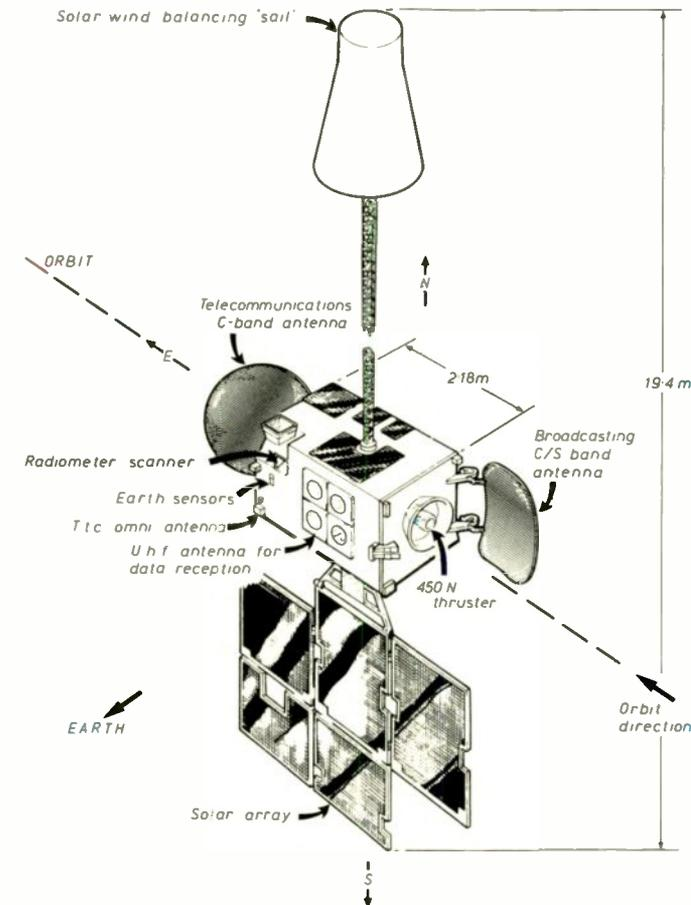
**India's second multi-purpose satellite has an asymmetrical structure with a solar array on one side and a balancing solar-wind 'sail' on the other. Diagram shows the orientation of the spacecraft in its geosynchronous orbit, with its antennas facing the Earth (somewhere off the picture to the bottom left). Overall height is 19.4m.**
