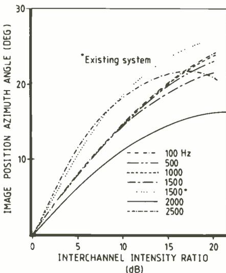
Fig. 6. Image displacement with interchannel intensity ratio in proposed system (-20dB/decade filter).
