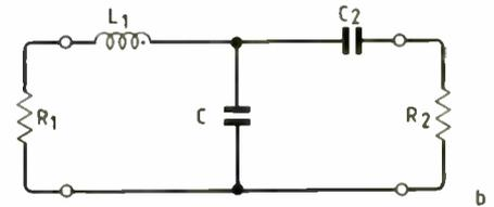
Fig.7. By making a kind of 'hybrid' with the Ls, as in (a), asymmetrical T-networks, such as the lossy L shown in (b) can be obtained.
