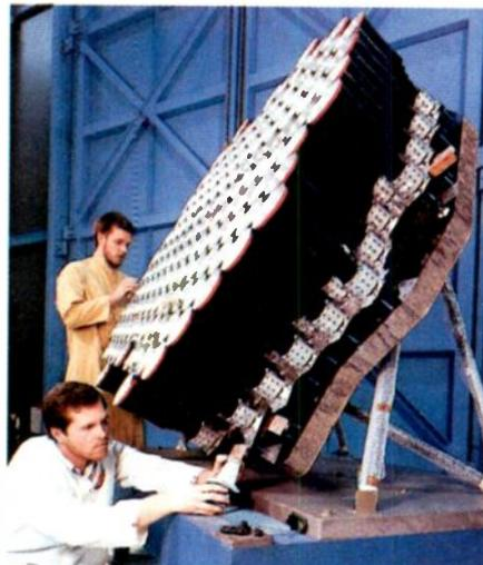
A section of Intelsat VI's antenna feeds. These determine the complex-shaped coverage areas of the satellite's footprint.
