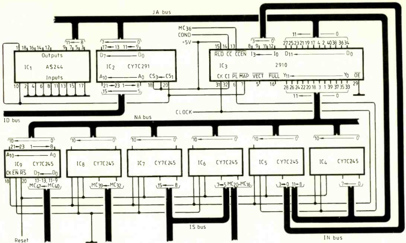
Fig.3. This controller, based on the 2910, is optimized to work with the a.l.u. of Fig.5 to produce a simple 16bit c.p.u.
