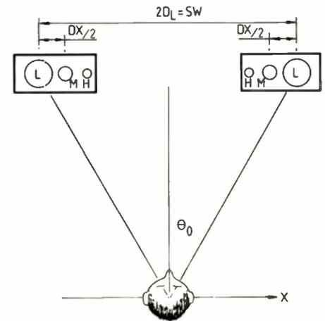
Fig. 2. Geometric arrangement of proposed method of improving image sharpness.  $\theta_0 = 30$  degrees,  $SW = 230 \text{ cm}$ .
