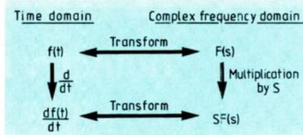
Fig.1. To evaluate the Laplace transform of  $df(t)/dt$ , trace the top right-hand path giving  $F(s)$  followed by the operation of multiplication by s. Alternatively follow the left hand path to obtain  $df(t)/dt$  and then perform the transformation – both routes are equivalent.
