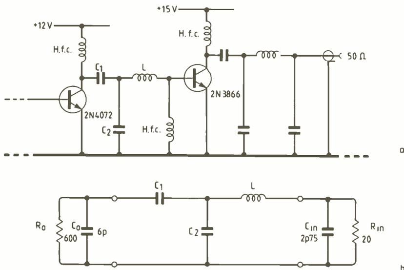
Fig.11. The circuit in (a) shows a driver stage and p.a. with the equivalent output and input impedances of the devices running at the power level assumed, shown in (b). The problem is to calculate suitable values for  $C_1$ ,  $C_2$  and  $L$  for maximum drive to the p.a.
