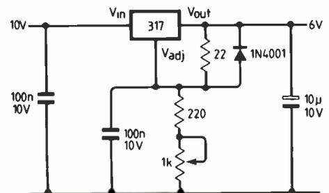
Fig. 4. Regulator i.cs provide some of the voltages needed to program the p.l.d.
