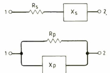
Fig.3. The impedance seen between 1 and 2 in both these circuits is the same, so that transformations can be made between them as desired.
