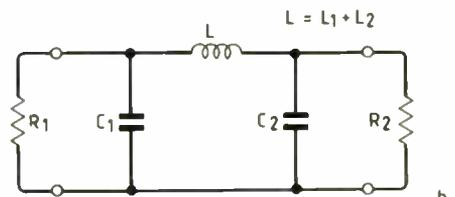
Fig.8. By turning round the L-networks, the  $\pi$  circuits result, as seen here in (a) which forms the low-pass  $\pi$  type matching network.
