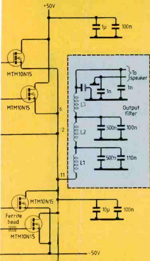
Requirements for a class-D power amplifier are much tighter than those for conventional amplifiers. Output devices must be capable of passing high currents and have an extremely low on resistance. This design, providing 200W continuous power into a 4Ω load, is one of about 50 designs illustrating the merits of Tmos power fets in Motorola's Tmos power-fet design ideas book.
