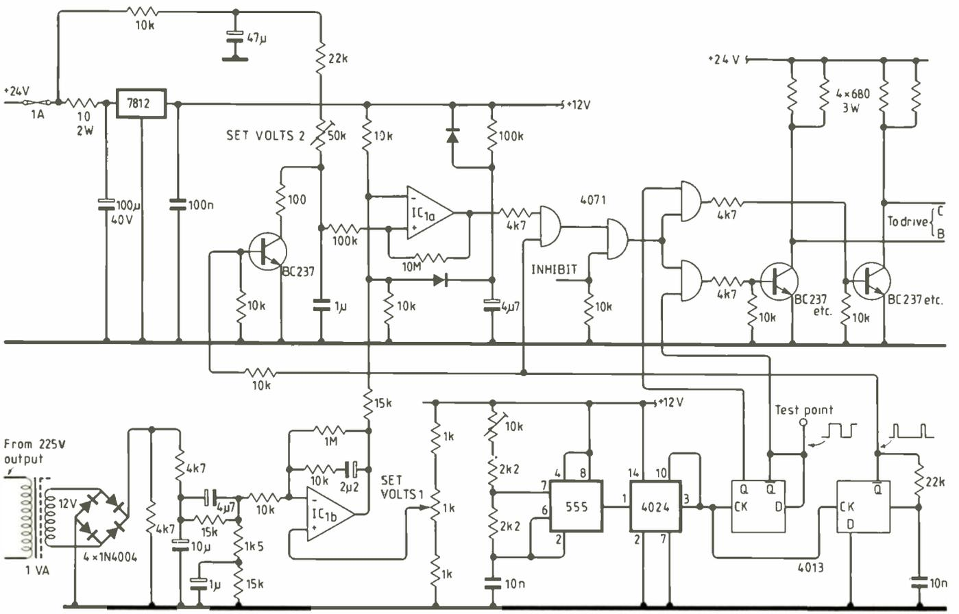
Fig.4 The inverter is controlled by varying the power transistor conduction periods by means of the waveforms at B and C.
