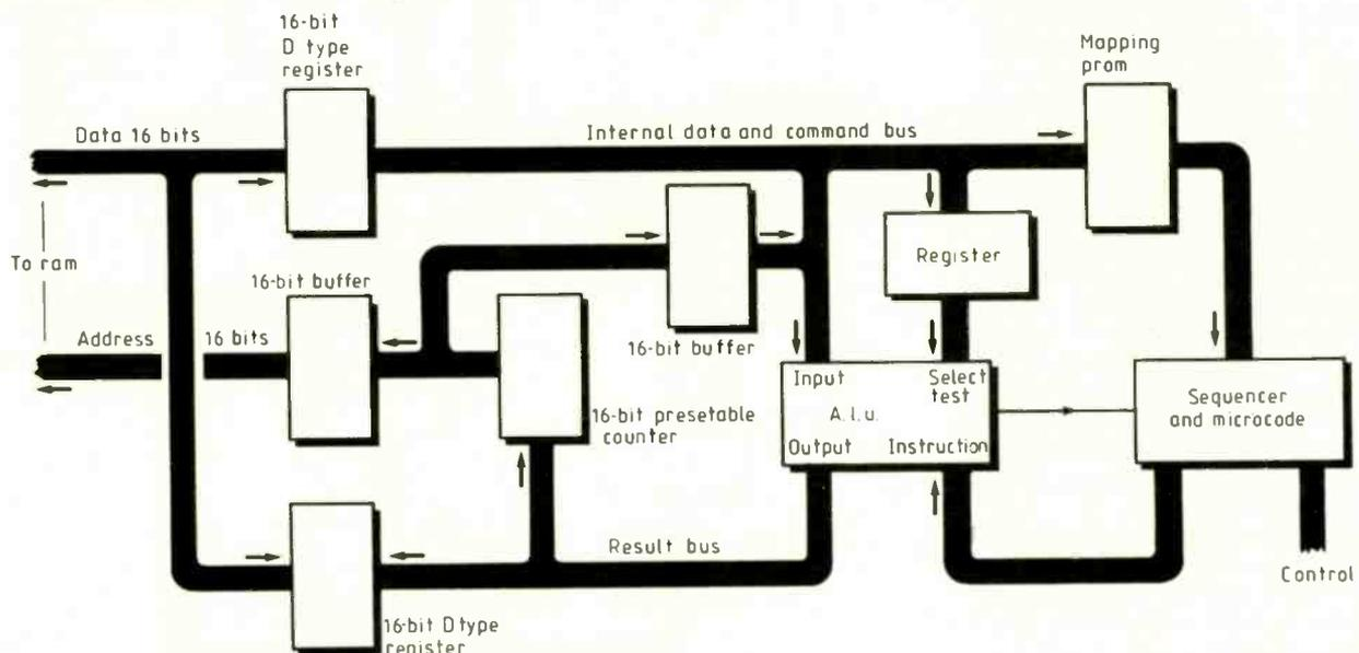
Fig.5. Demonstration 16bit c.p.u. design using an AMD a.i.u.
