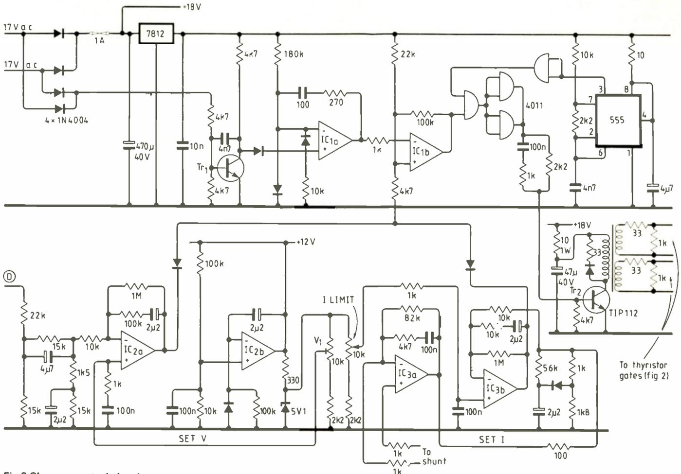
Fig.3 Charger control circuit.
