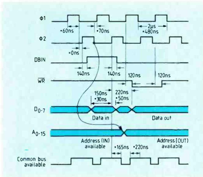
Fig.2. Timing characteristics relevant to connection of an 8080A microprocessor to a common synchronous bus.
