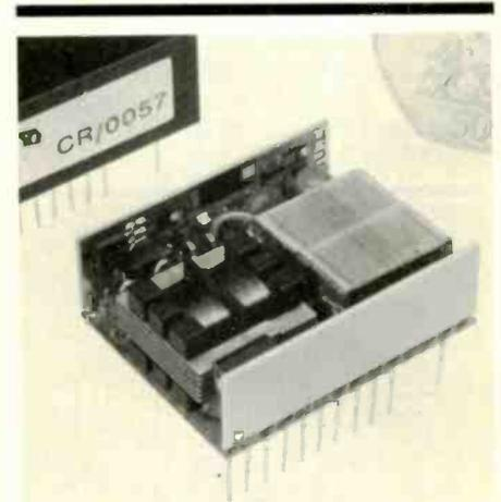
The data-communications line interface shown in the photograph is BAPT recognized and so reduces modem design approval time.
