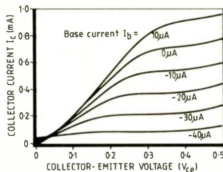
Unusual characteristics of the cadmium mercury telluride transistor by Mullard and RSRE.
