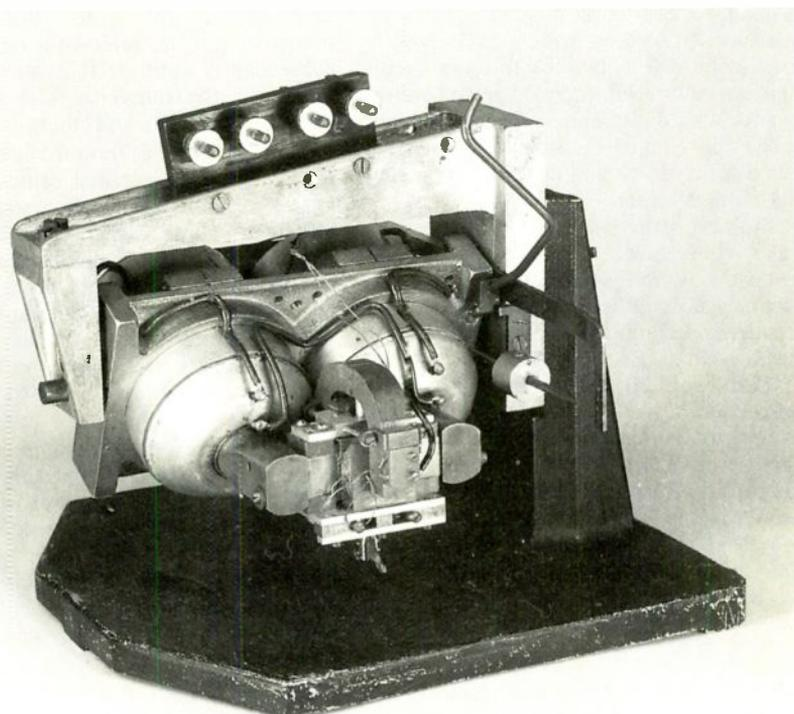
Moving-coil recording head, 1930/31 (Thorn EMI Central Research Laboratories).
