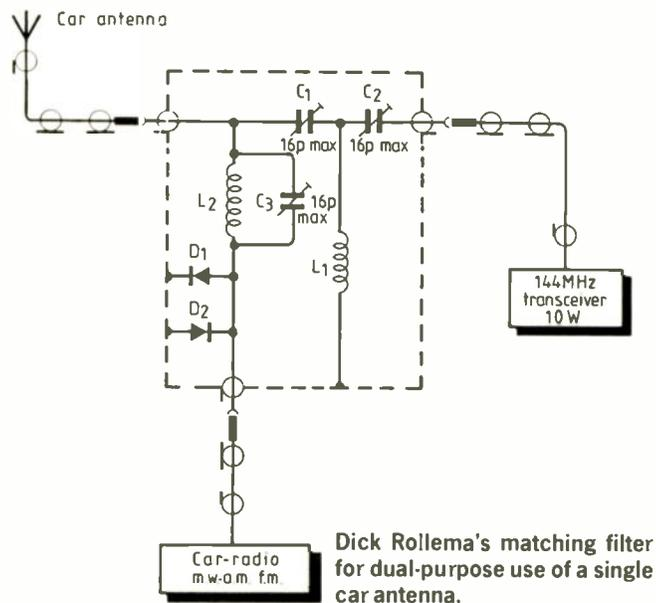
Dick Rollema's matching filter for dual-purpose use of a single car antenna.
