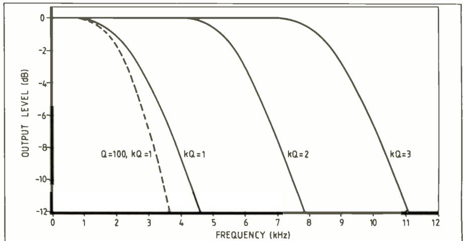
Substituting gives a loss of 10.8 dB, relative to that at  $f_0$ , at  $\pm 6$ kHz. For three i.f.t.s, the response will be -32.5 dB at  $\pm 6$ kHz, which agrees well with the chart.
