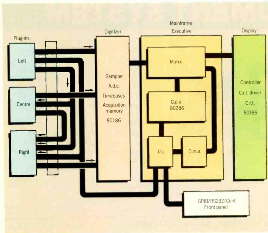
power of its central processor and the extent to which that power is harnessed, so a digitizing oscilloscope will only be as good as the hardware on which it is based.
