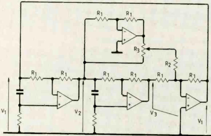
Fig.12. Wide-range frequency control, one variable resistor.
