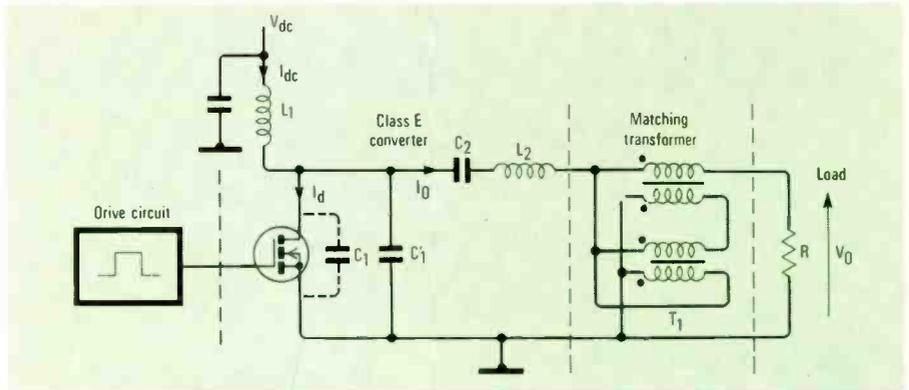
Fig.5. Basic class E amplifier circuitry.
