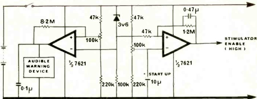
Fig.3. Possible design of battery-discharge manager. During discharge, with the stimulator operating, the battery current is typically 250 mA. At the end of discharge, with the stimulator disabled and the audible warning operating, the remanant battery current is 130 µA.
