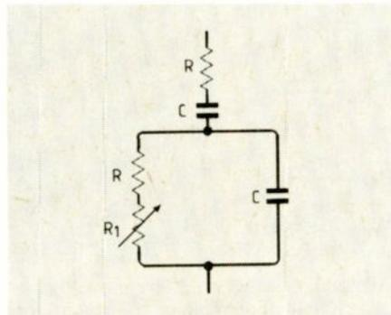
Fig.1. The variable resistor gives a large shift in frequency when  $R$  is small and vice versa.
