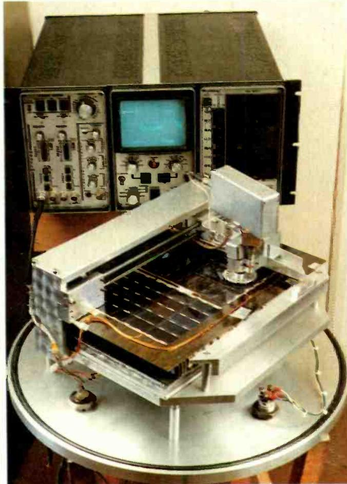
Fig.2. ERA Technology's laboratory equipment for investigating discharges in solar arrays. The portion of an array is charged up by electron bombardment in a vacuum. Circular table is the base of the vacuum chamber.
