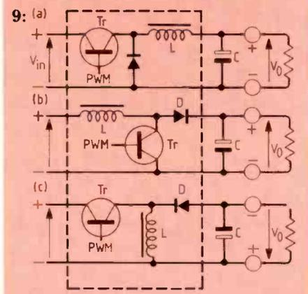
9: (a) Step-down circuit (buck), (b) step-up circuit (boost), (c) inverting buck-boost circuit.
