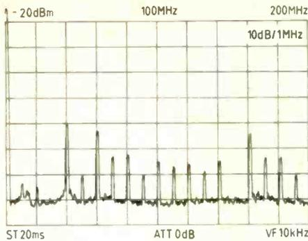
**Plot 7.** At higher frequencies, the p.c.b. tracks radiate.
