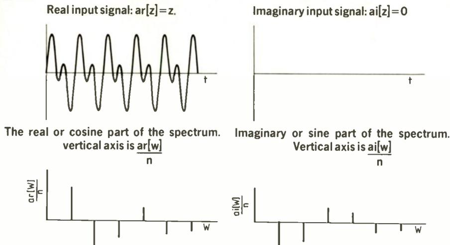
Squaring and adding the real and imaginary parts of the spectrum gives the power spectrum.
