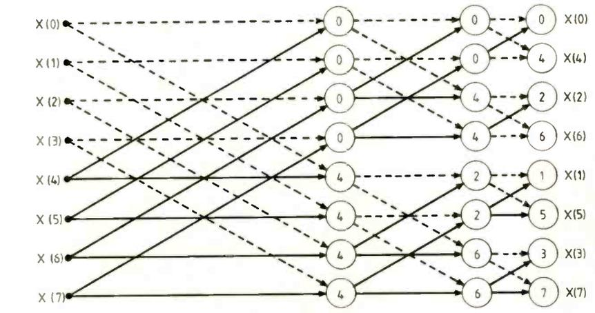
processed output in binary form, it will be apparent that the scrambling is not random, but a mirror image of the input - where the results are placed in bit-reversed order<sup>7</sup>.
