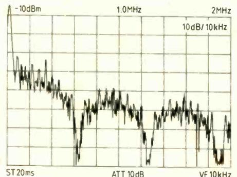
Plot 5. With a 'random' input at the microphone, the serial data-stream spectrum shows rapidly changing data.
