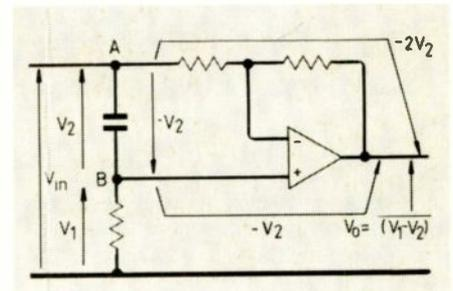
Fig.4. Op-amp version of Fig.3 circuit.
