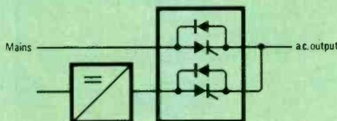
Fig.2. This static switch arrangement shows the output voltage of the inverter being fed to the load via a thyristor switch. Any deviation from the design specifications causes switch B to turn on.
