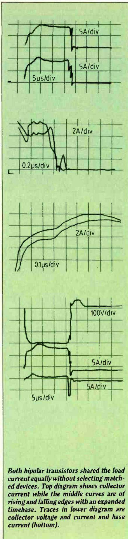
Both bipolar transistors shared the load current equally without selecting matched devices. Top diagram shows collector current while the middle curves are of rising and falling edges with an expanded timebase. Traces in lower diagram are collector voltage and current and base current (bottom).
