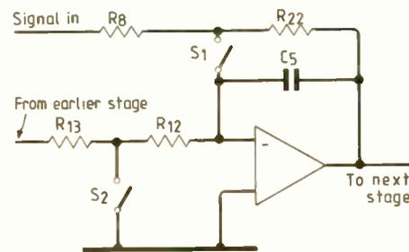
Fig. 6. Op-amp time shared between phase-sensitive detector and integrator schematic.
