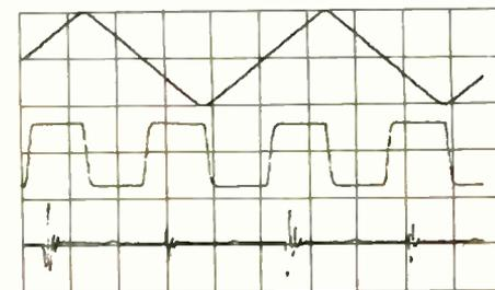
Fig. 7. Upper trace: sensor excitation ( $Tr_1$ ,  $Tr_2$  emitters, 10V/div.) Middle trace: phase-sensitive detector reference (IC<sub>1</sub>, Pin6, 20V/div.) Lower trace: typical sensor output (500 mV/div.) (Horizontal scale 0.1ms/div.)
