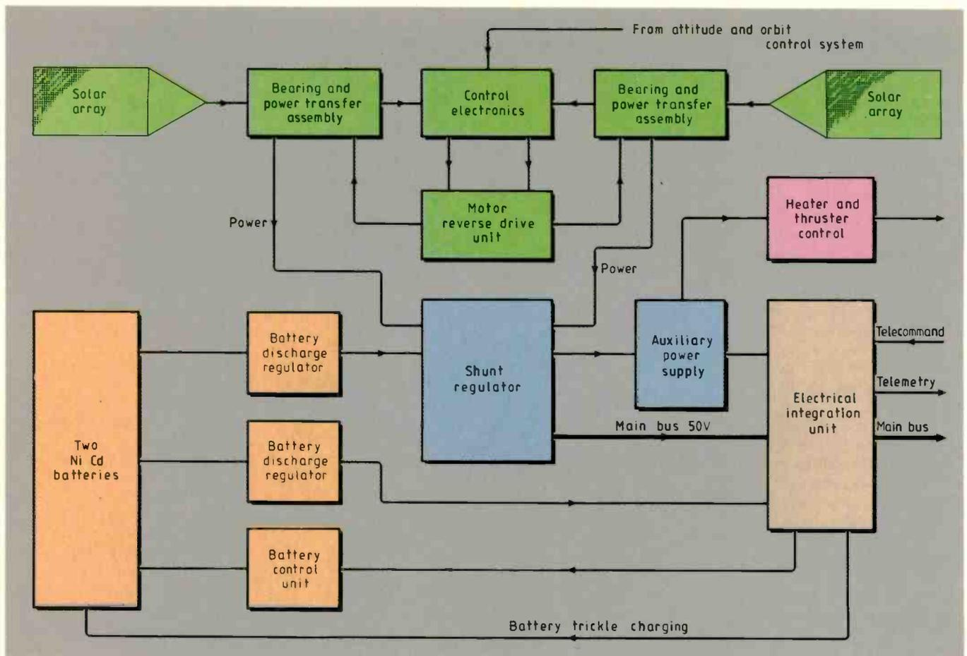
Fig.1. Solar power generator system in the ECS-5 communications satellite.
