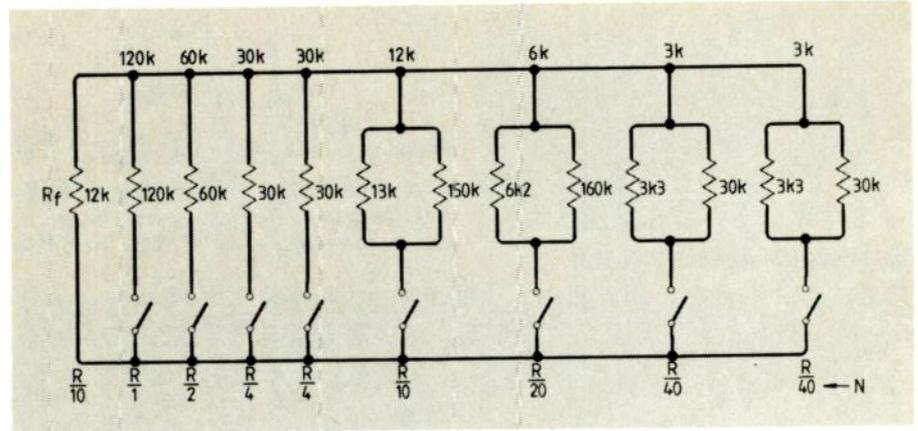
Fig.9. 1,2,4,4 switching combination for frequency control.
