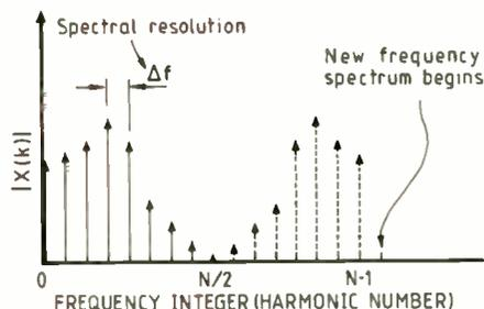
Fig. 13b. Discrete Fourier transform. The spectral resolution  $\Delta f$  equals  $1/N \cdot T$  hertz, where  $N$  is the number of samples and  $T$  the time increment between samples. For example, if the time between samples is 6.5ms and we decide to process 16 points, then the spectral resolution will be 10Hz. Therefore a digitized 50Hz sinewave would ideally be observed as a single ordinate at the sixth sample point.
