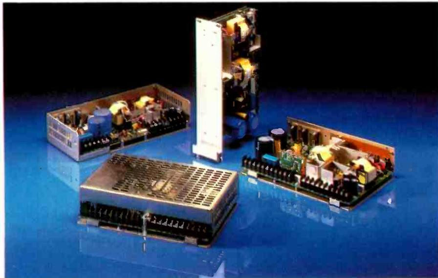
such a system is more complex in terms of component count. It has other disadvantages too such as more noise, both on the input and on the output and is more difficult and critical to design. However, it is very much smaller and lighter than a linear. It is also very much more efficient, and because of these savings it is of lower cost above a few hundred watts.
