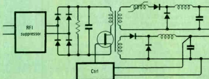
Fig.3. Keeping the input d.c. capacitor charged can be achieved in an alternative u.p.s. by using a d.c. converter to step up the voltage and using this output to keep the capacitor charged.
