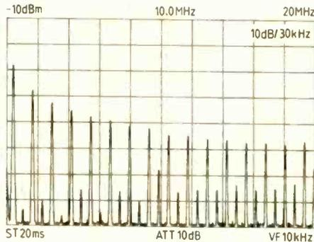
Plot 2. At the 625kHz oscillator, the spectrum shows far fewer even-order harmonics than at the 10MHz oscillator, as you would expect.
