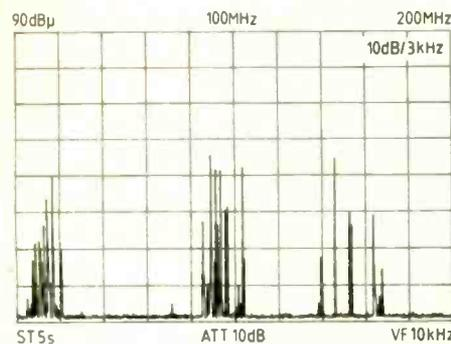
**Plot 10.** In open air, well away from radiating circuits, a vertically-mounted biconical antenna connected to the spectrum analyser picks up radio broadcasts.
