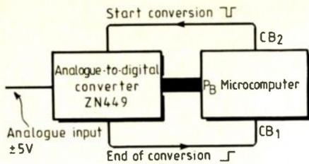
Fig.8. Interfacing an analogue-to-digital converter to the computer via the 6522 versatile interface adapter.
