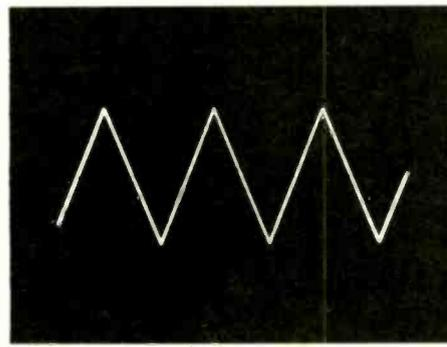
Oscilloscope display, 2V pk-pk, 10Hz.
