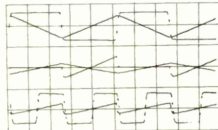
Fig. 5. Upper trace: triangle wave and square wave at frequency  $f$ . Middle trace: triangle and fet drain wave-form. Lower trace: sawtooth and comparator output at  $2f$ . (All traces vertical scale 20V/div. and horizontal scale 0.1ms/div.)
