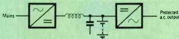
Fig.1. The conventional means of secure power – a u.p.s. – uses battery as an energy store. A sinusoidal output is maintained irrespective of whether it is taken from the mains or the battery.
