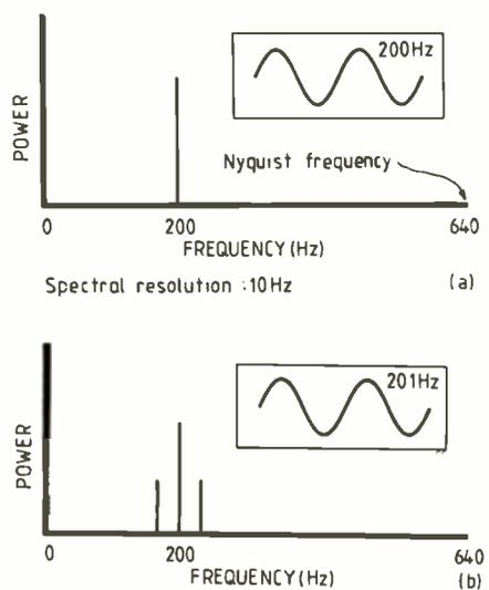
Fig.21. Results of processing synthetic data through FFT program to demonstrate the effects of spectral spreading due to signal truncation. At (a), no signal truncation results in the displayed spectrum agreeing with the anticipated result. At (b), effects of spectral spreading (leakage); 128 samples captured in 100ms.
