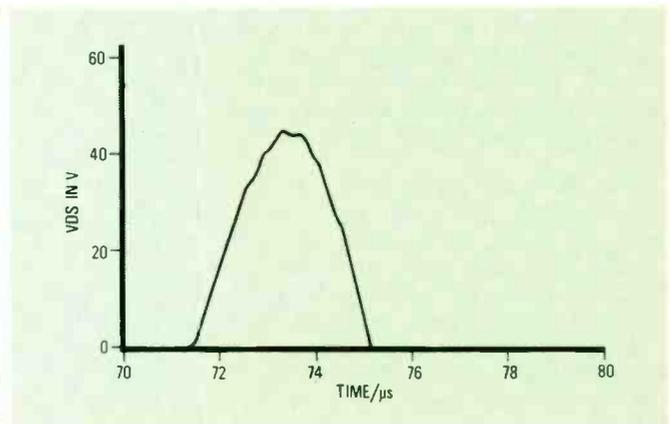
Fig.3. Theoretical waveform using Spice of drain source voltage across a mosfet feeding two-element tank circuit.
