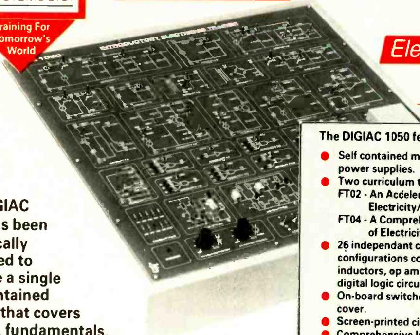
The DIGIAC 1050 has been specifically designed to provide a single self-contained trainer that covers a.c./d.c. fundamentals, semiconductor circuits and digital electronics.
