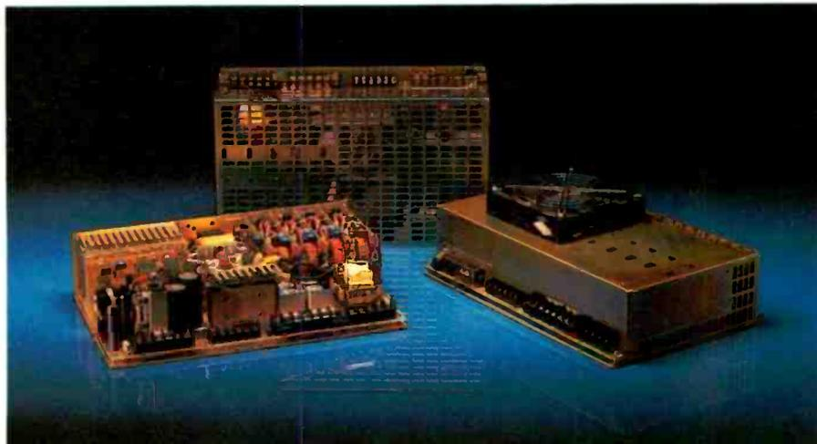
*Modular output cards give the 500watt Powerflex system a flexibility hitherto unknown, say Advance. New versions with d.c. input for telecom use are just released.*
