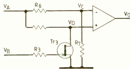
Fig. 4. Frequency-doubled reference circuit schematic
