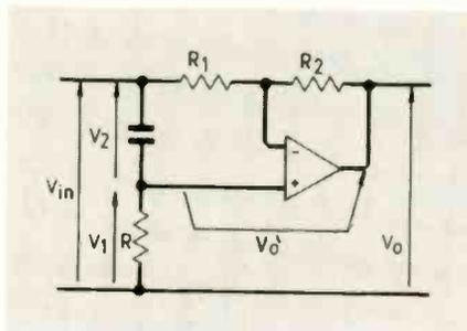
Fig.13. Frequency variation by gain variation, suitable only for fine control.
