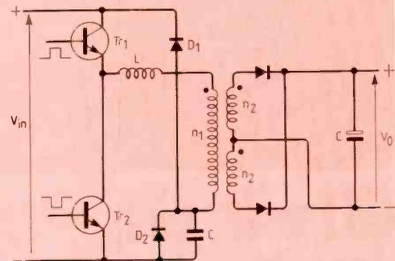
$Tr_1$  turning on again. Resonant converters can be designed using variable frequency or p.w.m. mode of control to provide a stable output voltage.
