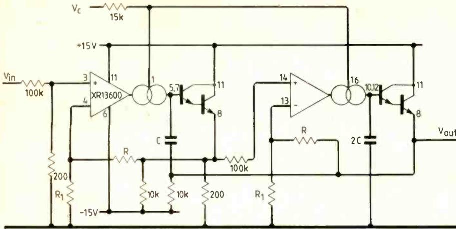
Fig.4. Butterworth low-pass of the second order using a double transconductance op-amp.
