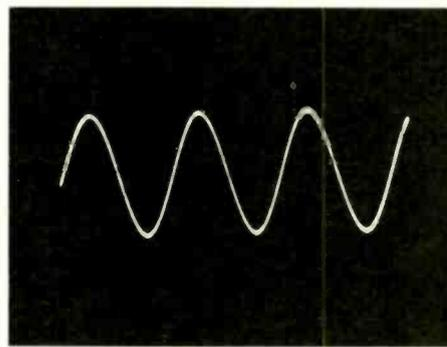
Oscilloscope display, 2V pk-pk, 10Hz.
