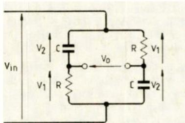
Fig.3. Circuit arrangement to give phase shift without amplitude change.
