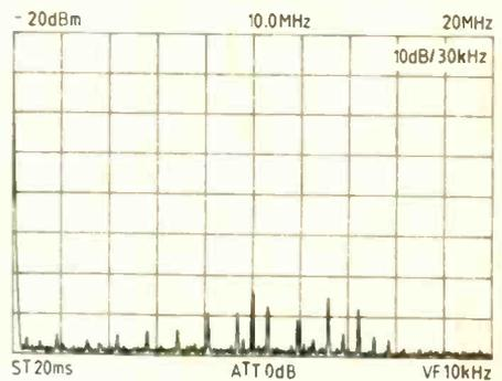
Plot 6. A simple dipole placed near the circuit shows that there is little radiation at low frequencies.
