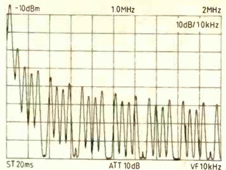
Plot 4. In the spectrum of the sampled serial data stream with the microphone switched off, regularity is caused by the constant direct voltage at the data converter's input.
