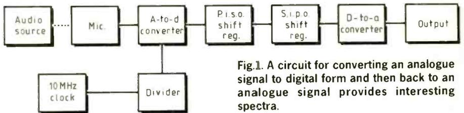
Fig.1. A circuit for converting an analogue signal to digital form and then back to an analogue signal provides interesting spectra.
