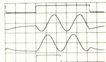
Fig. 8. Upper trace: clock output (IC<sub>4</sub>, Pin 9, 20V/div.) Second trace: phase-sensitive detector (sin)/harmonic oscillator output (IC<sub>3</sub>, Pin 7, 5V/div.) Third trace: phase-sensitive detector (cos)/quadrature output (IC<sub>3</sub>, Pin 1, 5V/div.) Lower trace: flip-flop output (IC<sub>4</sub>, Pin 5, 20V/div.) (Horizontal scale 10ms/div.)
