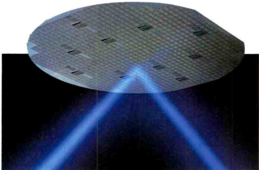
Latest Smartpower chip from Siliconix is an 80%-efficient switched-mode power converter that can be used to implement most single-ended converter topologies (type 9115).
