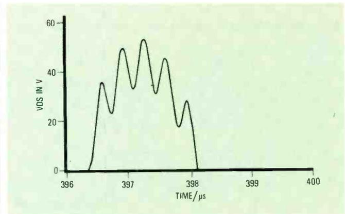
Fig.4. Theoretical waveform predicted across drain to source of mosfet when a modified tank circuit used.
