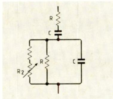
Fig.2. In this arrangement,  $R_1$  gives a small frequency shift when  $R$  is small.
