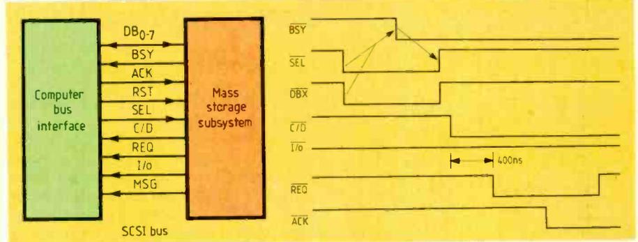
controllers. When this combination is detected by the controller, it asserts *BSY*, upon which the host releases *SEL* and the selection data bit.
