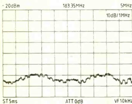
**Plot 9.** With audio input, the 183MHz spectral peak from Plot 7 reveals the effects of data.
