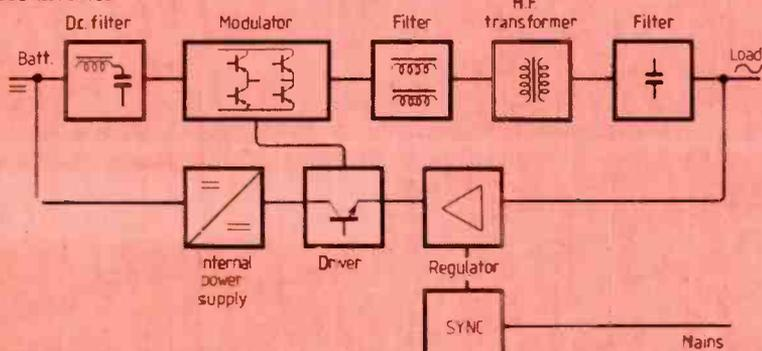
Switched-mode inverters are used for the operation of equipment, sensitive to public mains fluctuations and equipment that in the event of breakdown in public mains may effect personal safety, lead to damage of material or result in financial loss. Together
