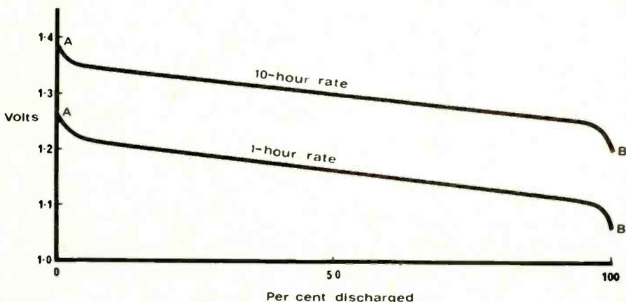
Fig.1. Form of the discharge curve for a nickel-cadmium cell.
