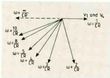
Fig.14. Phasor diagram for  $V_1$  and  $V_4$  ( $-V_3$ ) in Fig.12, showing that as  $\omega$  exceeds  $1/CR$ , phase angle nears  $180$  degrees.
