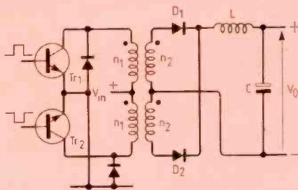
The transistors alternately turn on and the voltage across the secondary will be  $V_{in}$  multiplied by the turns ratio of the transformer. Frequency of the secondary waveform will be twice the switching frequency which means simple filtering on the output can be designed for. Each device must be rated for twice the supply voltage as this is the voltage seen by one transistor when the other is conducting.
