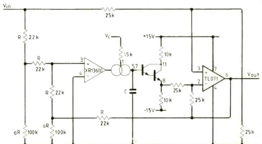
Fig.3. Inverting all-pass filter of the first order using a transconductance op-amp.
