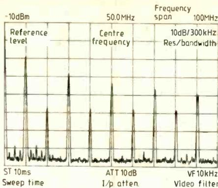
Plot 1. Spectrum of the 10MHz crystal oscillator reveals many harmonics.
