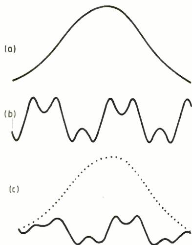
Fig. 14. The Hanning function. At (a), the Hanning data window.  $W[i]=0.5(1 - \cos(2\pi i/N))$ , where  $i$  is the sample point number and  $N$  the total number of samples. At (b), truncated data to be transformed; and at (c), the effect of multiplying by the Hanning data window.
