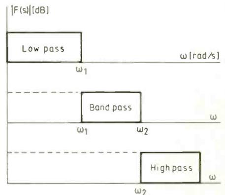
Fig.1. Modelling various filter types by use of low-pass filter.
