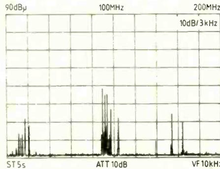
**Plot 12.** Again in open air with the circuit switched off, but now with the antenna mounted horizontally, the spectrum analyser shows broadcast radiation.
