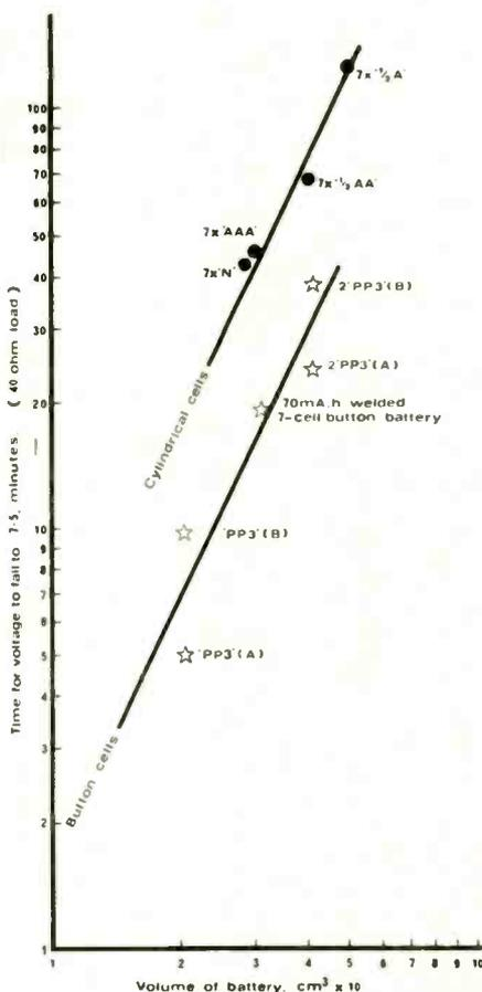
Fig.2. Time to end-of-discharge for various sizes of cell and two different forms of construction. 'PP3' (A) and 'PP3' (B) are by different manufacturers.
