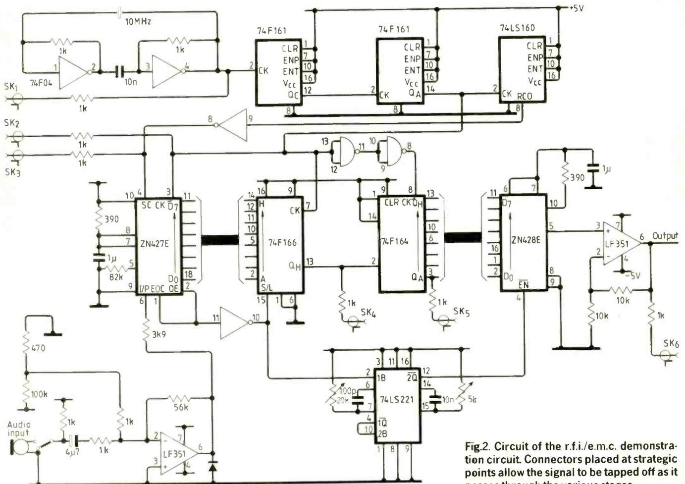
Fig.2. Circuit of the r.f.i./e.m.c. demonstration circuit. Connectors placed at strategic points allow the signal to be tapped off as it passes through the various stages.
