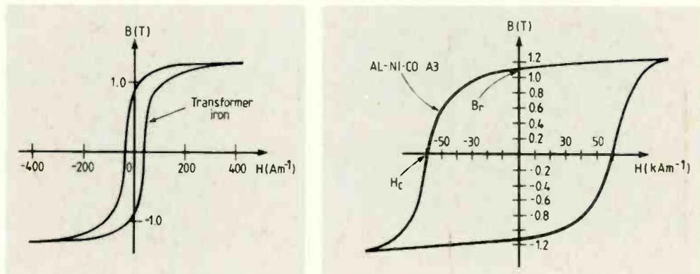
Fig. 10. This illustrates the narrow hysteresis curve characteristic of a "soft" magnetic material. Notice the small magnetizing force required for a rapid rise in flux density. Fig. 11 (right). A "hard" material has a wide hysteresis loop with a large coercivity,  $H_c$ .
