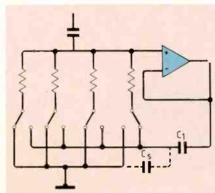
Fig.18. Two-way switches and bootstrap circuit avoids effects of strays.
