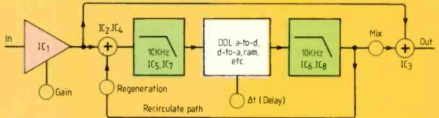
by a four pole low-pass filter  $IC_{5,7}$ .
