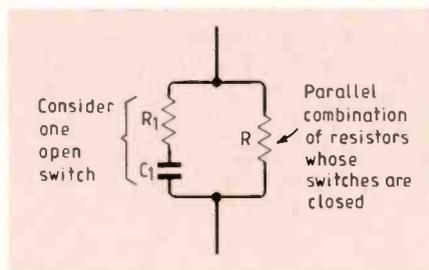
Fig.16. Equivalent circuit of "open" analogue switches.
