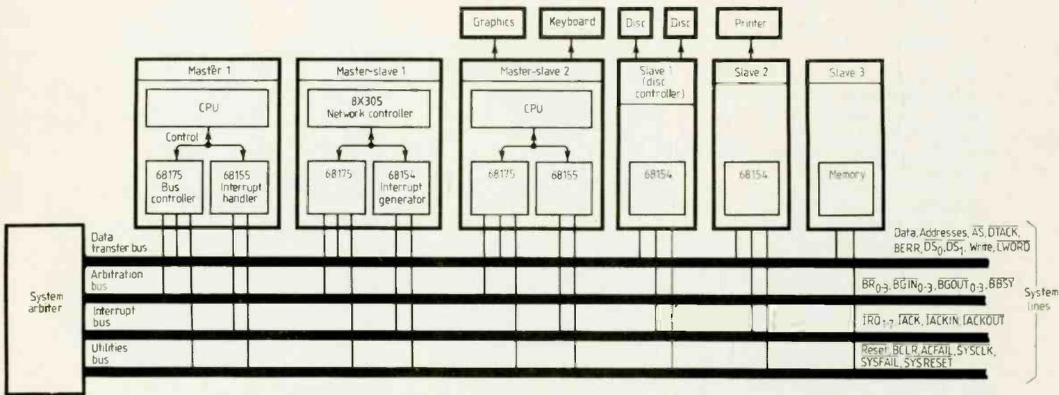
Fig. 10. The 68175, 68154, 68155 and VMEbus (above).
