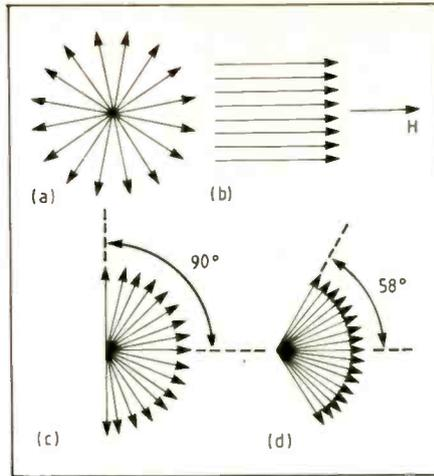
Fig.15. Whether or not the crystals of the material possess a preferred direction affects the shape of the demagnetization curve noticeably. The vector diagrams show a simplified picture of the likely effect on the remanence.
