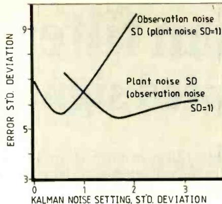
Fig.3. Variation of error, showing that proper choice of plant and observation noise setting can reduce estimate error.
