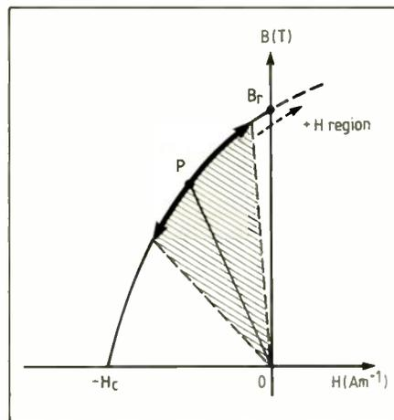
Fig.14. Very rarely do magnets possess a single operating point such as that on Fig.12. Different parts of the material operate on different sections of the demagnetization curve as shown here.
