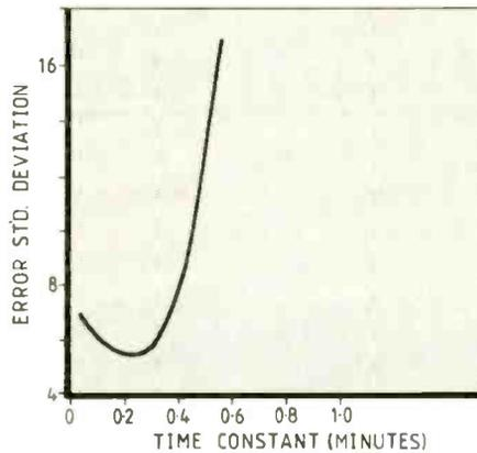
Fig.5. Plot of estimate error against time-constant of first-order filter, showing that its best performance is poorer than that of Fig.4.
