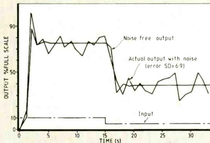
Fig.2. Model representing ideal and noisy behaviour of airflow, providing an input to the Kalman filter.
