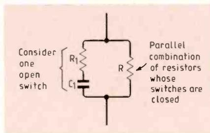
Fig.16. Equivalent circuit of "open" analogue switches.
