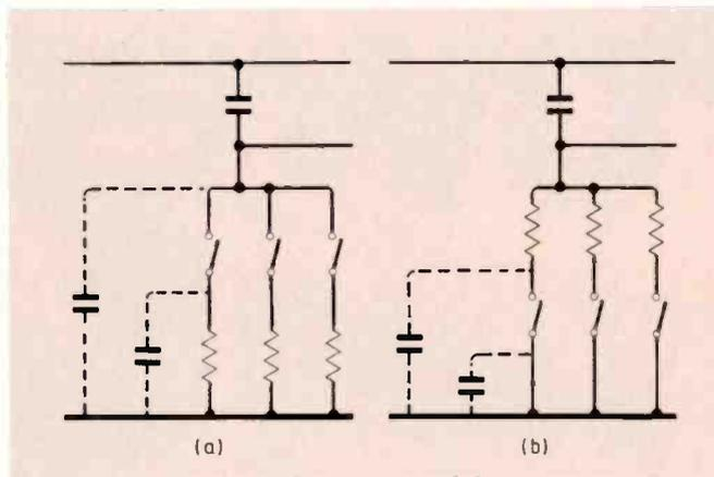
Fig.15. Switching capacitance effects for either switching method.
