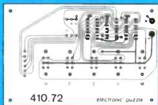
A number of ready-to-use PCB layouts are provided on film for immediate transfer onto copperclad boards, one of the manual's most popular items.
