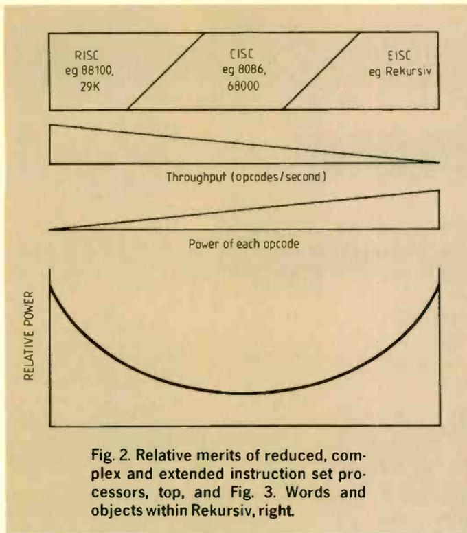
Fig. 2. Relative merits of reduced, complex and extended instruction set processors, top, and Fig. 3. Words and objects within Rekursiv, right.
