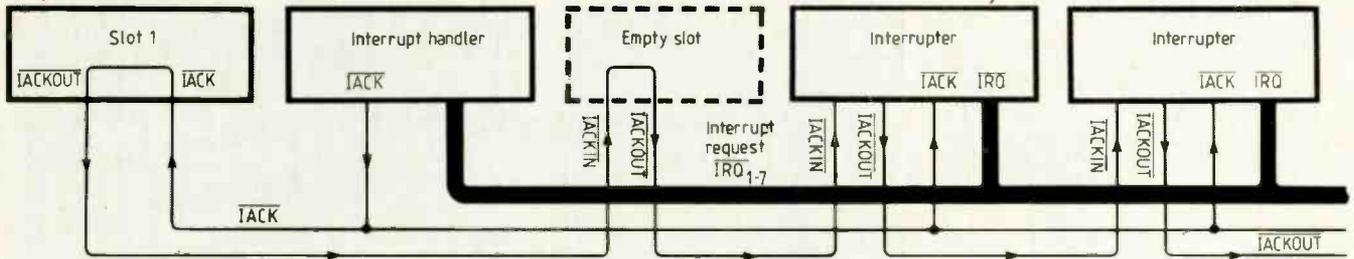
Fig. 8. The interrupt bus (above).
