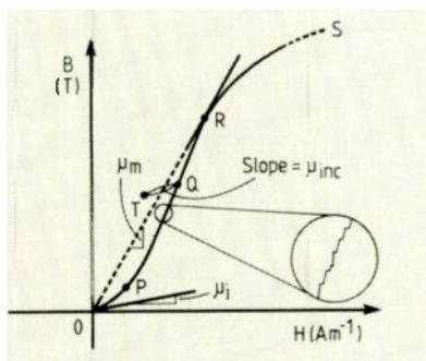
Fig.1. The relation between  $B$  and  $H$  in ferromagnetic materials is very non-linear. The various slopes from the origin give the permeabilities under different conditions. One of them, the incremental permeability, arises from the shallow slope  $Q-T$  as  $H$  oscillates along this path.
