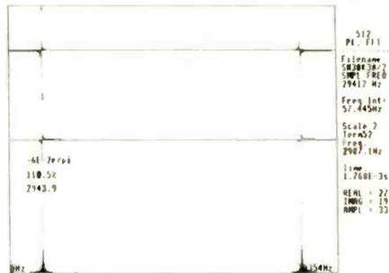
Fig. 9. 512-point FFT gives  $FREQ = 2943.9\text{Hz}$  (Freq. interval  $= 57.445\text{Hz}$ ) and phase  $= 0.068$  radians.
