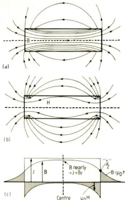
Fig.13. The continuous flux lines shown in (a), concentrate towards the remanent value in the centre of a bar, while the  $H$  field strength drops off towards zero at the same position. The field lines proceed in different directions to the flux lines. In general they go in opposite directions inside the material. The graph shows qualitatively how the field strength and the flux density varies from point to point in the material and nearby space.
