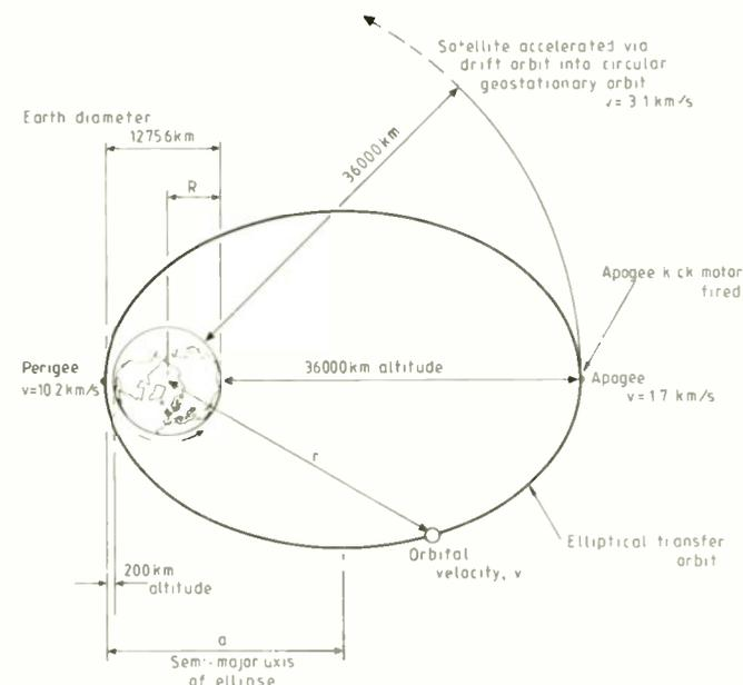
Fig.1. Principle of elliptical transfer orbit, as used by Harold Rosen to put Syncom into a geostationary orbit and now standard practice. The orbit shown here is an ideal one in the equatorial plane. For simplicity the drift orbit phase is not included.
