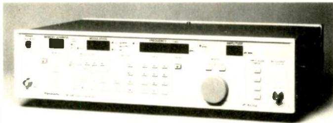
The Panasonic VP-8175A and VP-8174A (GP-IB) are broadcast frequency, AM/FM signal generators with built-in FM stereo modulator, and have comprehensive external control facilities and flexible memory modes. Separate LED displays are provided for frequency, amplitude, modulation and memory information. Output range is from  $-19$  to  $99\text{dB}\mu$  (1dB step)
