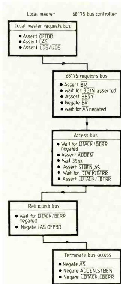
**Fig. 13. Protocol flowchart for Fig. 12.**
