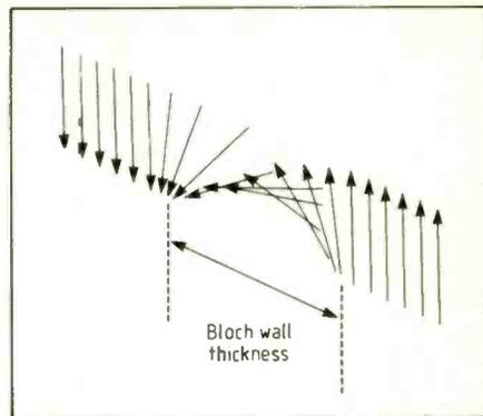
Fig.6. The Bloch Walls mark a region where the direction of magnetization has to change by 180°.
