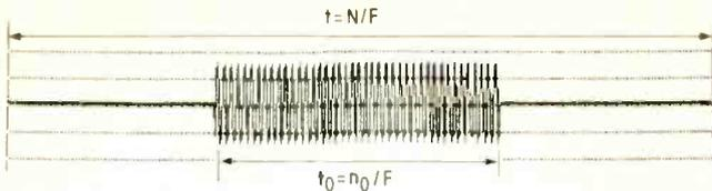
Fig. 5. Cosine function switched on for a period  $t_0 = n_0(1/f)$  less than  $T$ .
