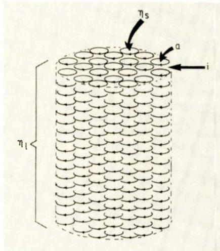
**Fig.3. Magnets in an external field experience a torque or turning moment trying to align them a long the direction of the field lines. Hence the function of the magnetic compass. You can see the two ways of looking at this in (a) and (b). The relation between the elementary loop moments and the total moment should become clear from (c).**
