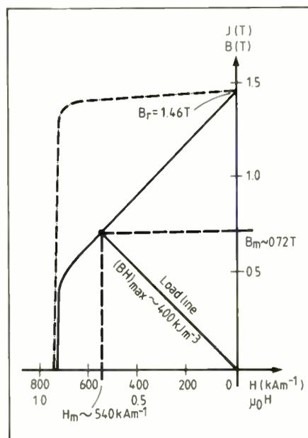
Fig. 20. This curve applies to the largest energy product achieved in a sample of permanent magnet material. The picture also illustrates that the optimum operating point yields a load line slope of 45° in these materials.
