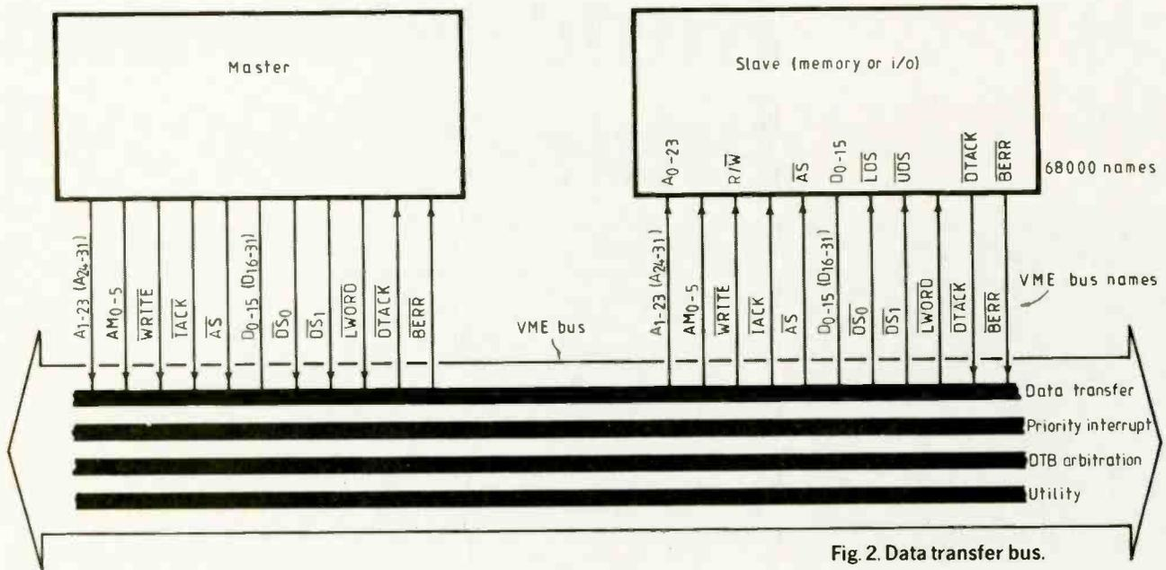
Fig. 2. Data transfer bus.
