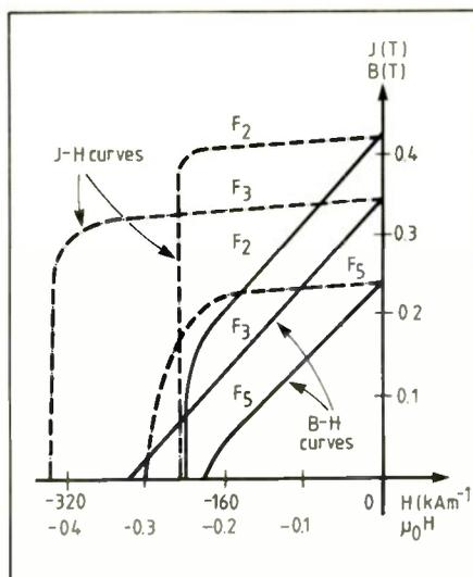
Fig. 19. The B-H and J-H curves for various grades of ferrite material all show the characteristics mentioned in Fig. 19.
