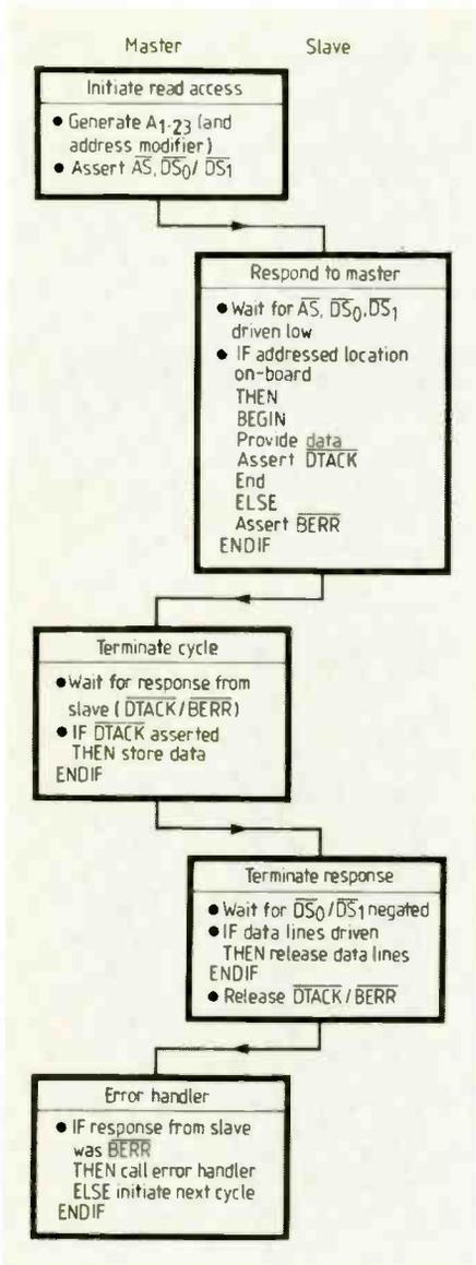
Fig. 3. Protocol flowchart for a VMEbus access.
