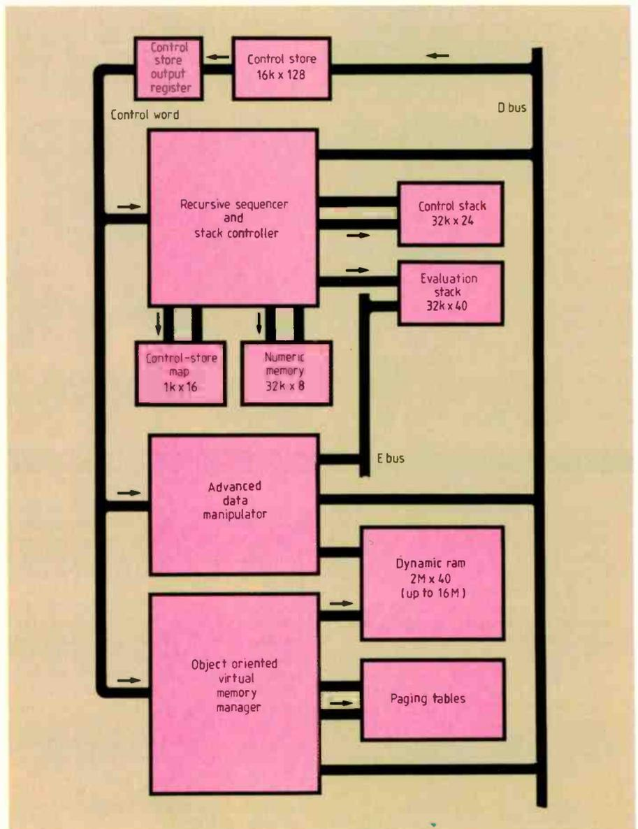
Fig. 4. Structure of one of the first products to incorporate the Rekursiv chip set – a single-board computer.
