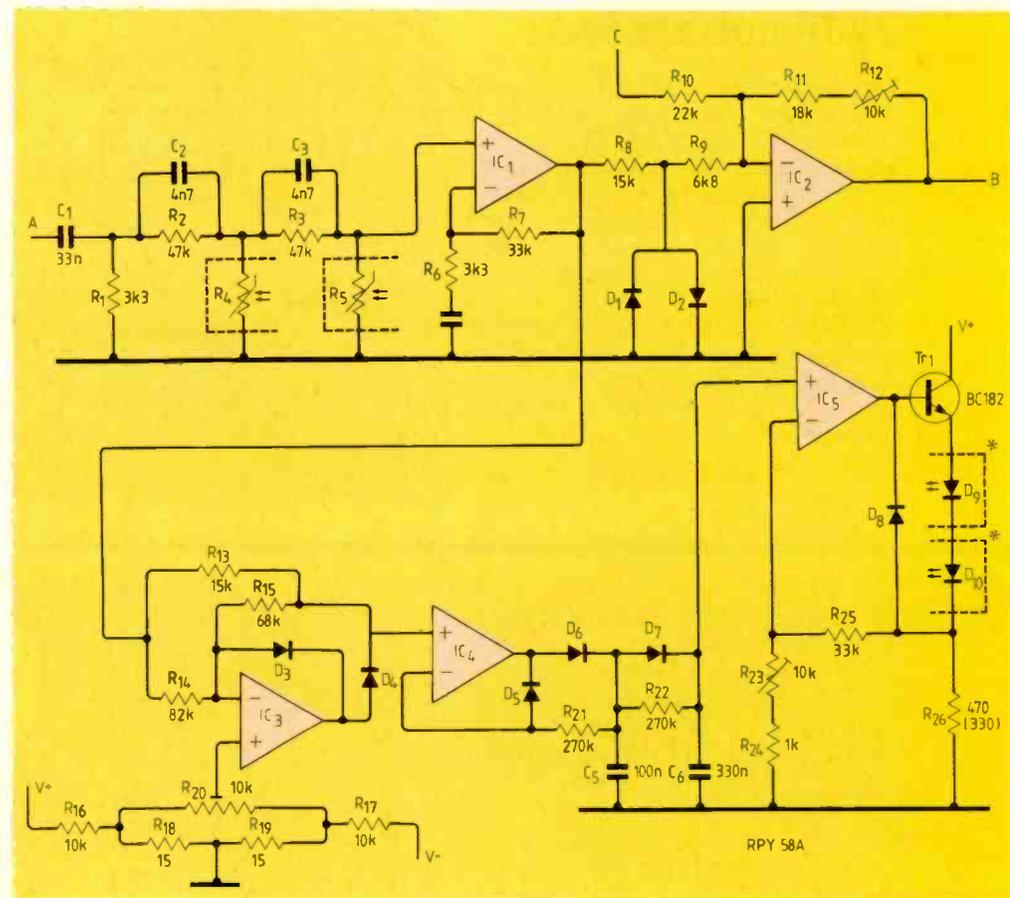
path, while IC<sub>4</sub> drives the control-loop time constant.
