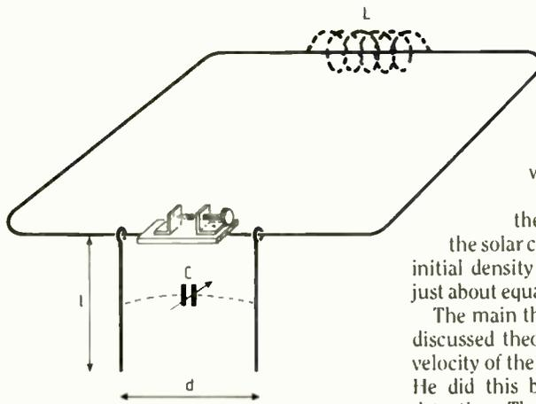
**Fig.3.** Hertz reports on his experiments with "tuning". "The easiest way of adjusting the capacity of the secondary circuit was by hanging over its two ends two parallel bits of wire and altering the length of these and their distance apart". "Exactly similar results followed when the poles of the secondary circuit were connected with the plates of a Kohlrausch condenser".
