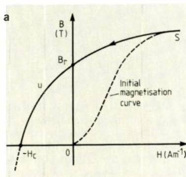
Fig.2. Looking at (a), moving back from saturation near  $S$ , a negative value of  $H$  eventually reduces the flux density to zero. The path from  $B_r$  to  $-H_c$  carries the title *demagnetization curve*. The full curve in (b), obtained by going right through a complete magnetization cycle, shows the familiar *hysteresis curve* of a ferromagnetic material.
