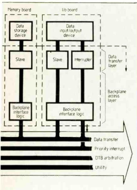
supported by three major manufacturers; Motorola, Mostek and Signetics. Today it is supported by a wide range of manufacturers and is in the process of becoming an international standard (IEEE-1014 and IEC-821). Although primarily intended for 68000-based microcomputers, the VMEbus is suitable for other advanced 16 or 32bit microprocessors.
