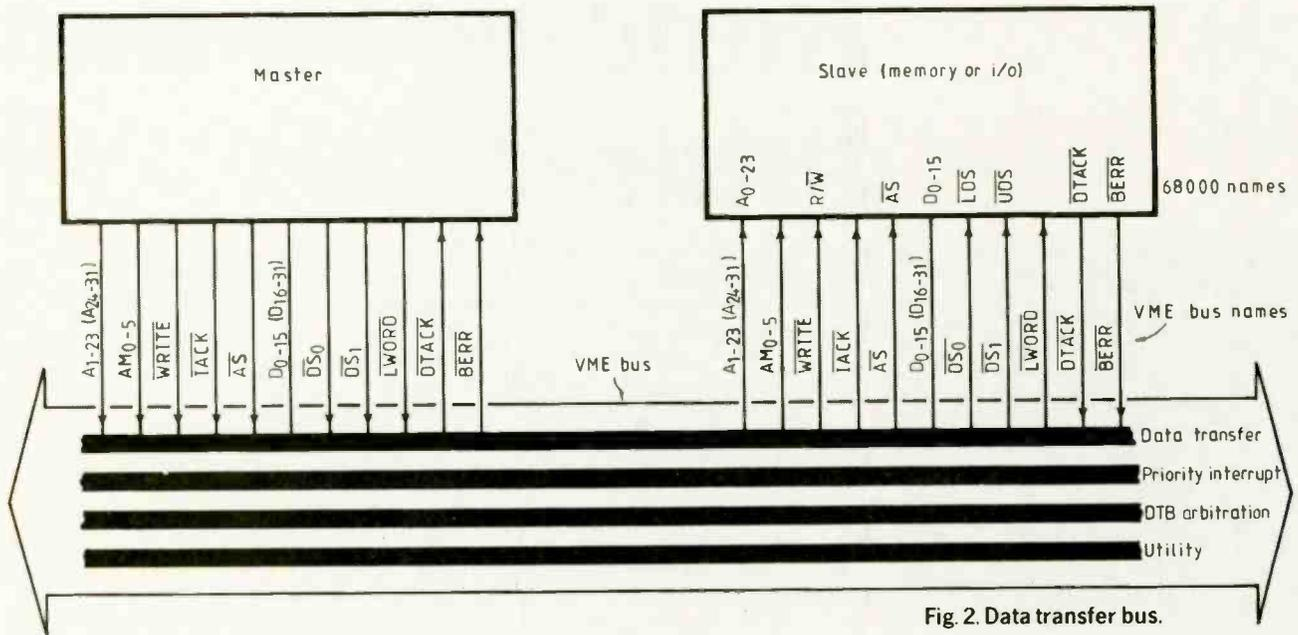
Fig. 2. Data transfer bus.
