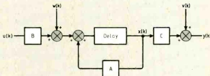
Fig.1. System diagram of a Kalman state estimator.
