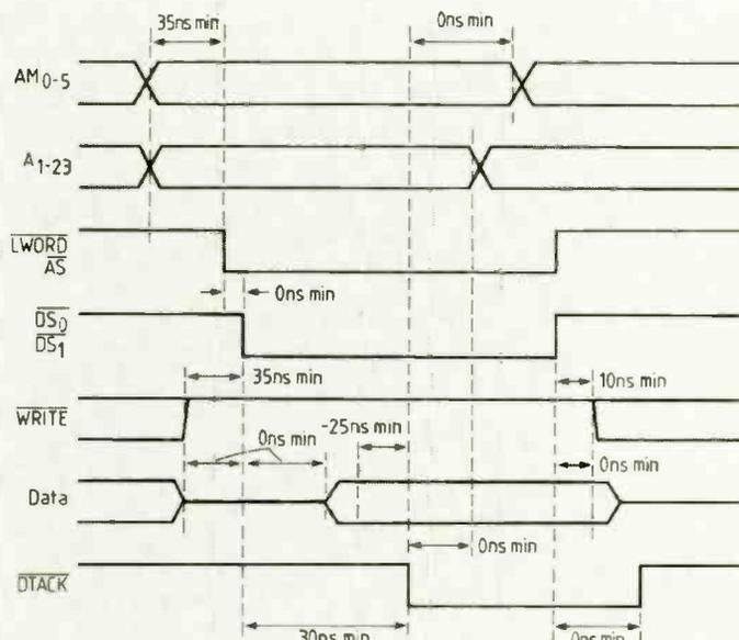
Fig. 4. Timing of a VMEbus read cycle.
