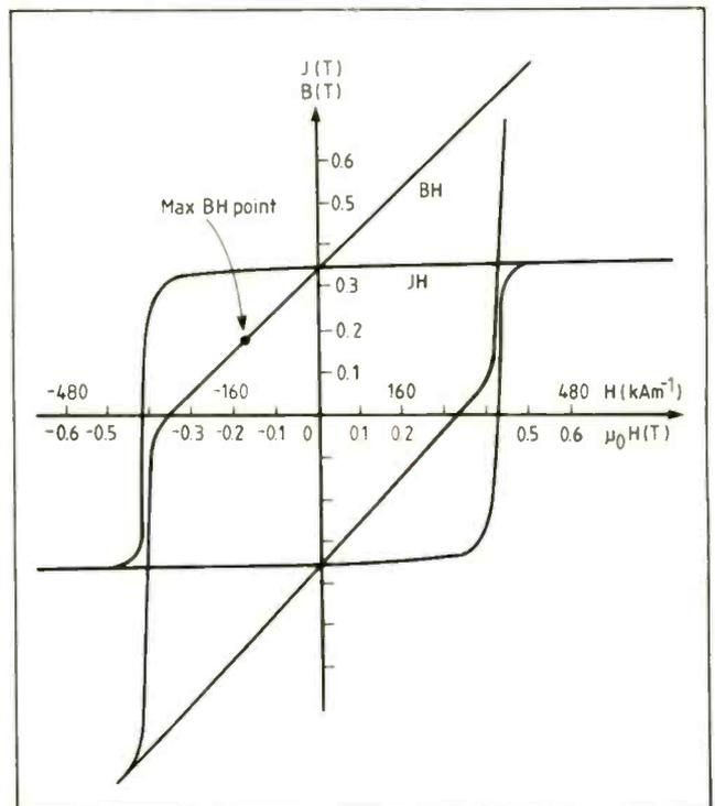
Fig.18 (right). The enormous coercivity, but considerably lower remanence of the ferrite materials produce an interesting effect. The axes can now be plotted to the same scale, as I have done here. The B-H curve now has a maximum slope of minus unity, whereas the J-H curve has a large horizontal section. B can reverse, even while J is still near the saturation value.
