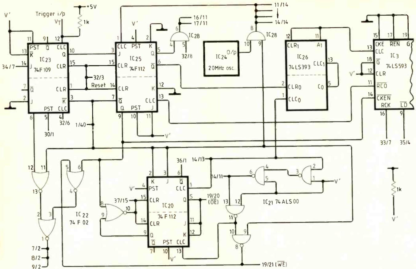
Fig.3. Oscillator and trigger circuitry.
