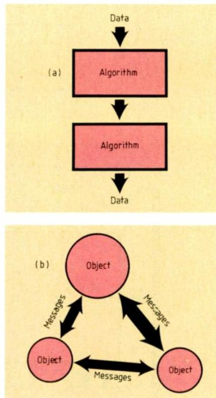
Fig. 1. (a) shows a conventional programming paradigm and (b) object-oriented programming.
