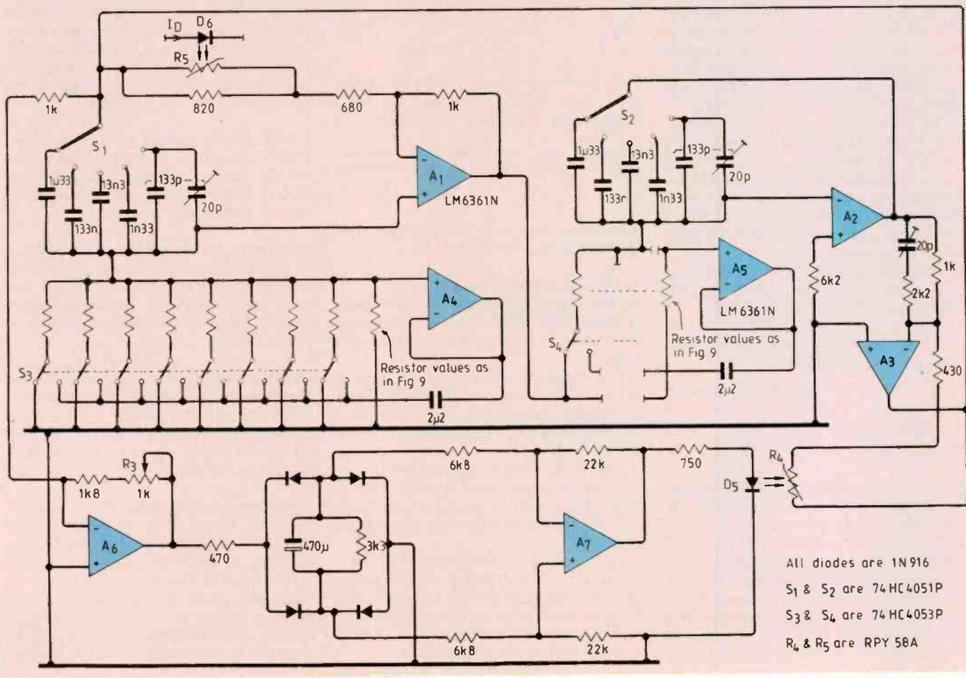
A resistor of 430 ohms was included in series with  $R_4$  to force it to stabilize at a lower value, which reduces the effect of stray capacitance within  $R_4$ . If this resistor is increased to a higher value, the capacitance effects are reduced even further, but only at the expense of reduced amplitude control.
