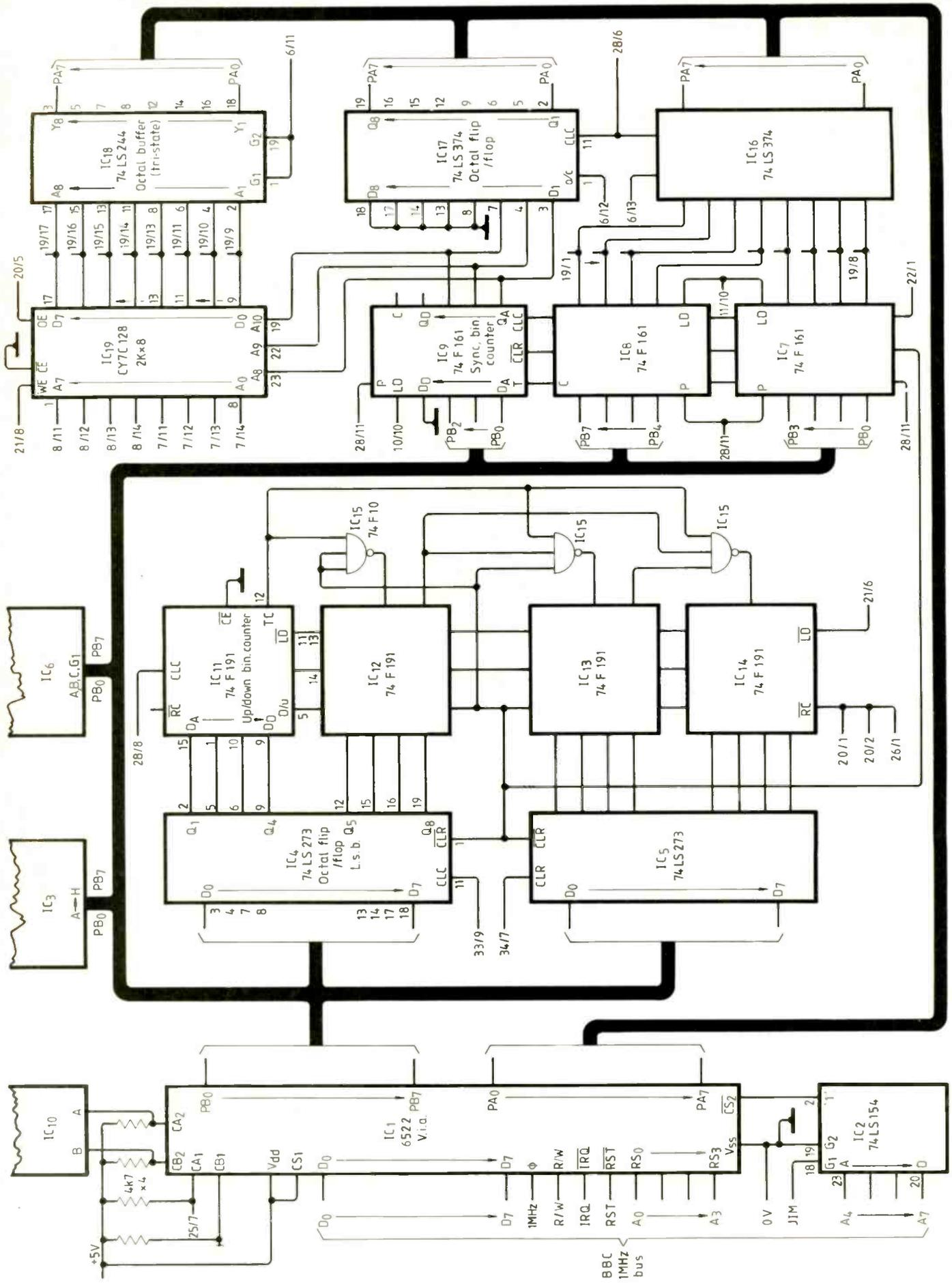
**Fig.2. Bus system. The transient analyser connects directly to the 1MHz bus port of a BBC microcomputer.**
