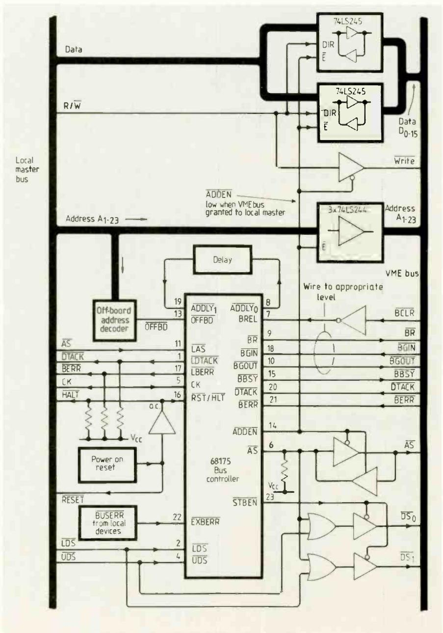
Fig. 11. The 68175 and its interface to the VMEbus and a local bus master.
