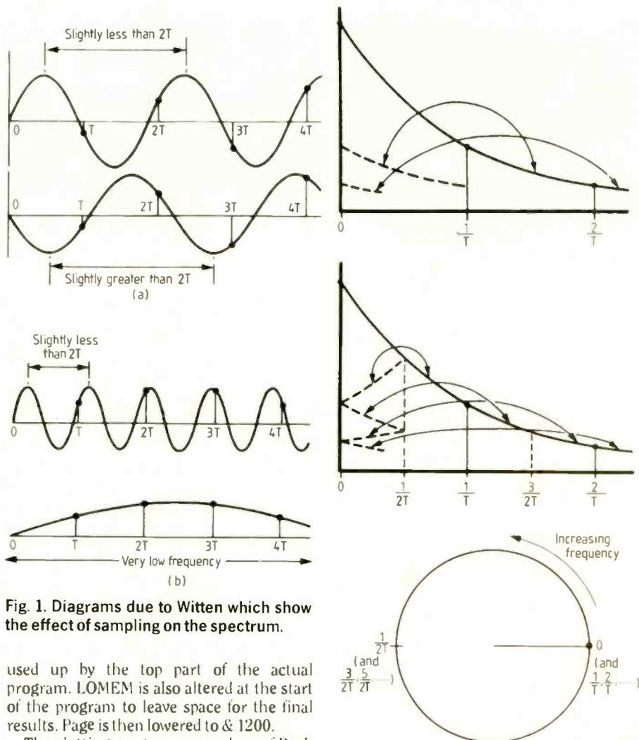
Fig. 1. Diagrams due to Witten which show the effect of sampling on the spectrum.
