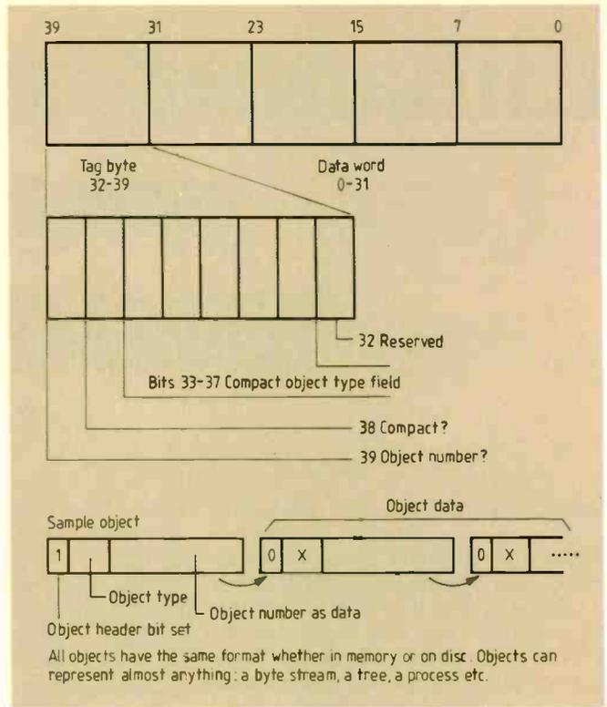
All objects have the same format whether in memory or on disc. Objects can represent almost anything: a byte stream, a tree, a process etc.
