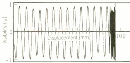
**Variation of visibility of embedded differential interferometer as a function of displacement of the centre of graphite composite bar. Rapid cycling of the visibility indicates onset of bar failure.**
