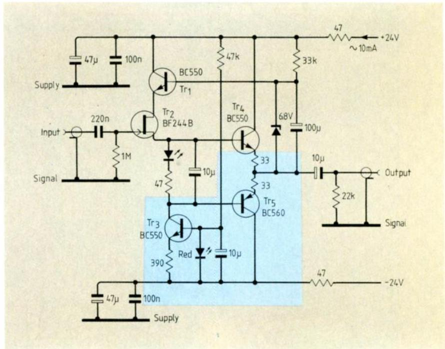
complementary output stage,  $\text{Tr}_{4,5}$ . Two LEDs form 1.6V references. In low-cost applications, current source  $\text{Tr}_3$  can be replaced by the simpler inset circuit.
