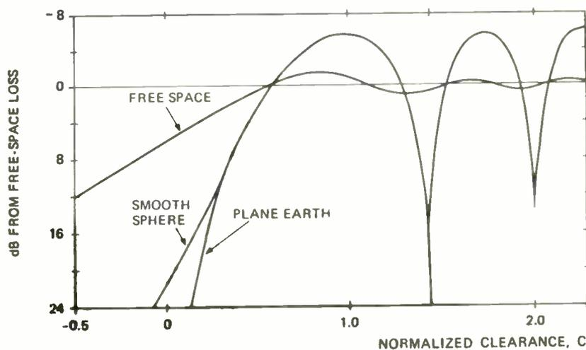
Fig.5. Loss versus normalized clearance.
