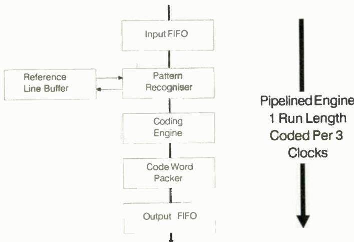
**2D Encoding:** This method transmits the difference between the current scan line and the previous scan line on a line by line basis. It assumes an imaginary first line comprising of all white pixels and compares the first scan line to this. The difference between the two lines is transmitted. Although efficient, any errors made in the document will corrupt the entire page from the point at which the error was made.
