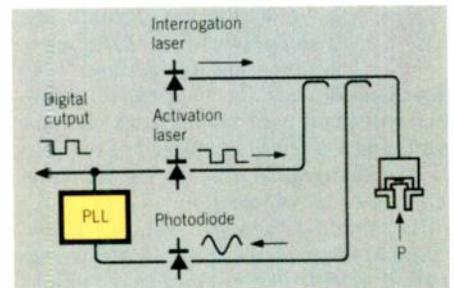
**In the latest version of the resonant silicon pressure sensor, fibre optics excites the resonator and provides the frequency output for measurement. There is no on-chip circuitry and the allowable operating temperature determined by the fibre optics is estimated to be in excess of 350°C.**
