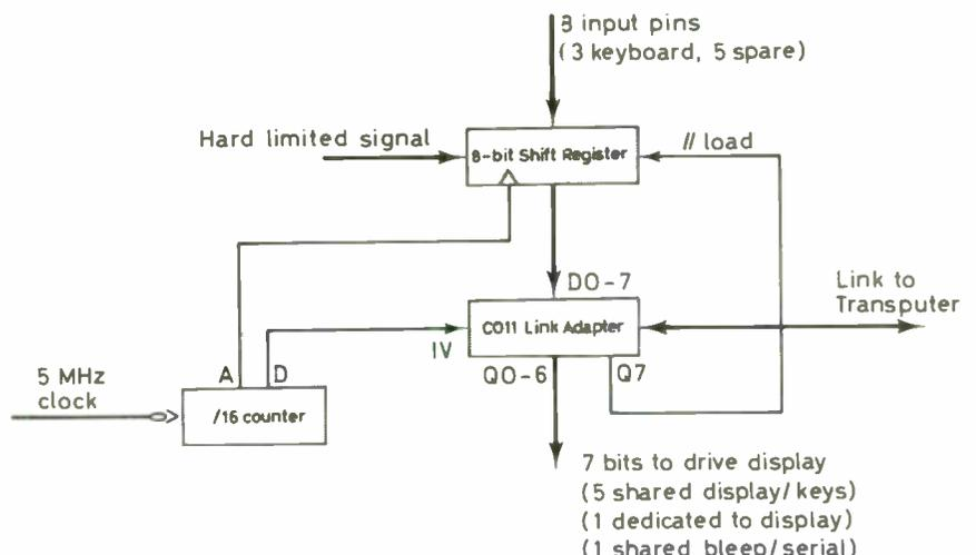
Fig. 6. Interface for 2.5MHz hard-limited samples with keyboard and screen interface.
