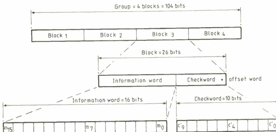
Fig.3. Basic data structure of RDS is a 26-bit sequence known as a block.
