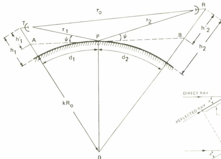
Fig.10. Geometry of a path to determine the point of reflection and angle between direct and reflected rays.
