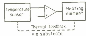
Regardless of how much heat is lost from the unit, its temperature is kept constant by means of the negative-feedback loop. All that varies as the ambient gas pressure varies is the total amount of power consumed by the heating element. Measurements of the current consumed by the device are then simply translated into pressure readings.
