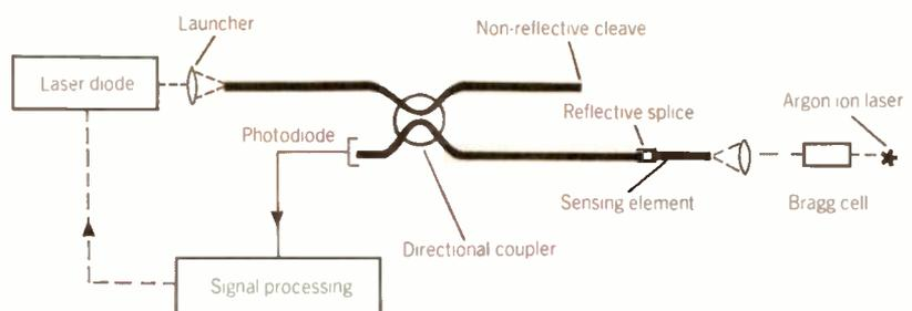
**The heat pulse measurement system is formed by fusion splicing a miniature fibre Fabry-Perot interferometer to one of the output ports of a single-mode directional coupler. A simple low-bandwidth servo controls the laser diode's injection current hence its absolute frequency such that the operating point of the interferometer is stable and not effected by low frequency environmental noise whilst remaining very sensitive to high frequency transients.**
