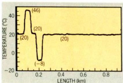
*The temperature distribution obtained from processing the curves shows the fibre loss has been eliminated and the temperature information is clearly visible. The temperature trace is flat in all regions where the fibre was held at uniform temperature.*
