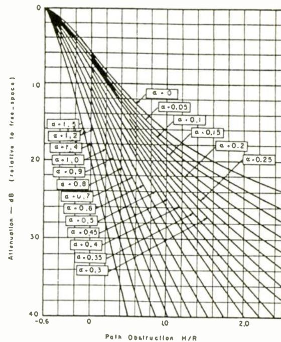
Fig.6. Diffraction over rounded obstacles.
