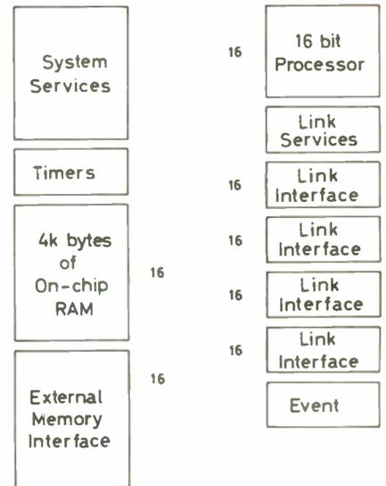
Fig. 4. Because the transputer has internal memory, accessing is very fast since the problems of driving i/o pins and printed circuit tracks do not arise.
