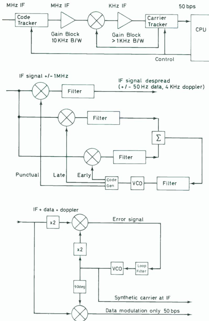
Fig. 3. Traditional GPS receivers require one of these hardware tracking channels per satellite (a). Sections (b) and (c) are a traditional code tracking loop and a hardware carrier tracking loop respectively.
