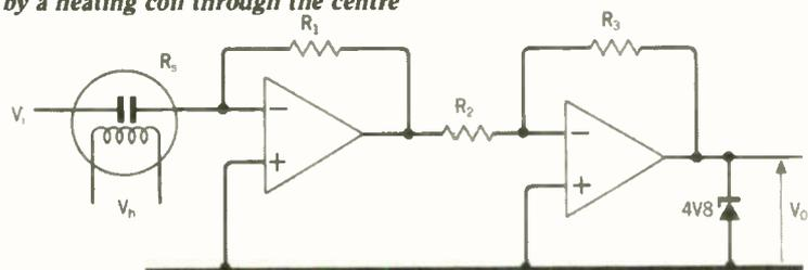
*In the improved circuit arrangement used at Warwick the gas sensors act as a current source in a virtual earth circuit feeding an inverting amplifier with fixed gain  $R_1/R_2$  to give an output voltage  $V_o$ .*
