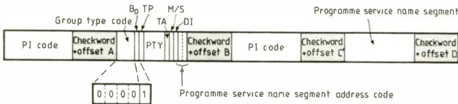
Fig.5. Type 0B group. PI is the single most important code carried by RDS and is repeated frequently.
