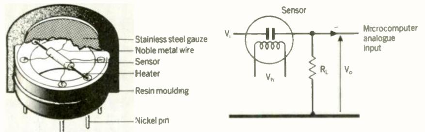
*The Taguchi gas sensor consists of a ceramic tube on which an interdigital electrode structure lies, covered by a sintered tin-dioxide layer. Film conductance changes with the chemisorption of atmospheric vapours, while its temperature is maintained by a heating coil through the centre*
