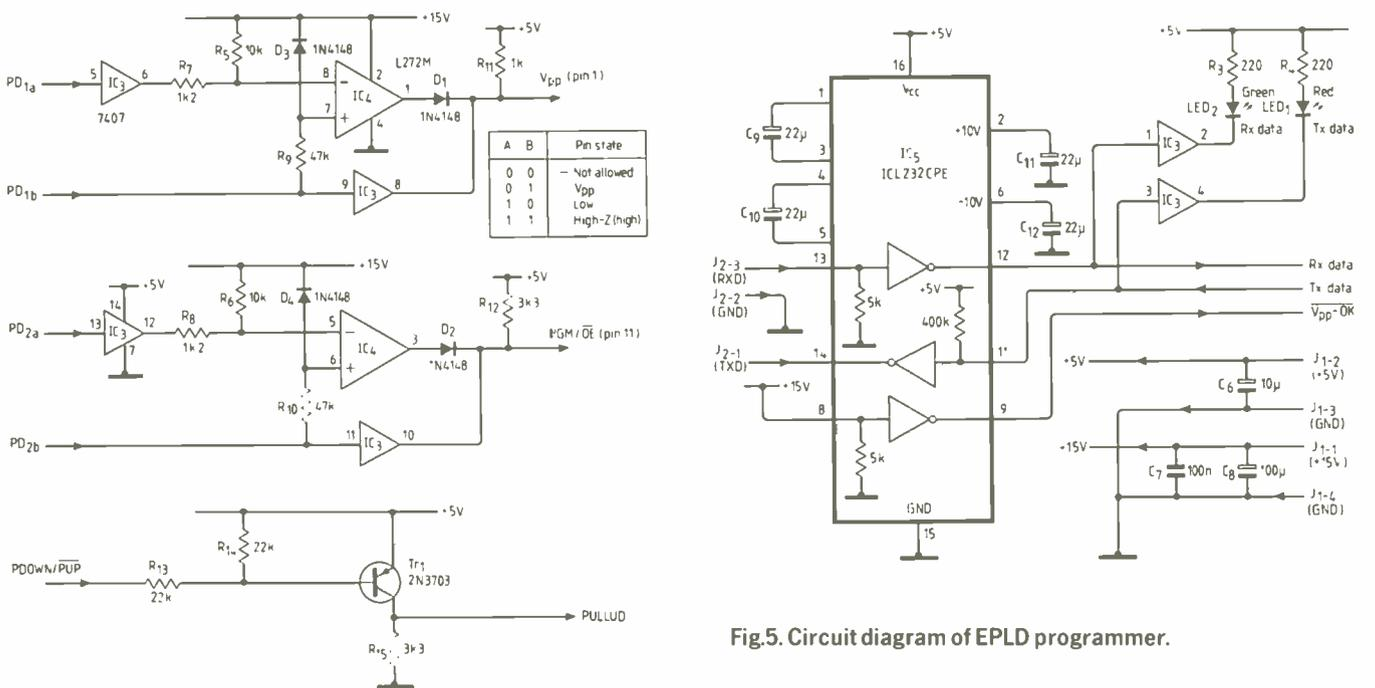
Fig.5. Circuit diagram of EPLD programmer.
