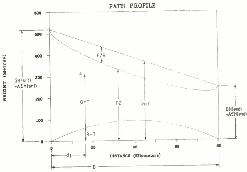
Fig.1. Parameters needed for path profiles.
