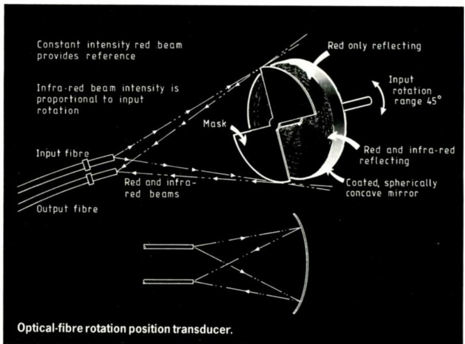
Optical-fibre rotation position transducer.
