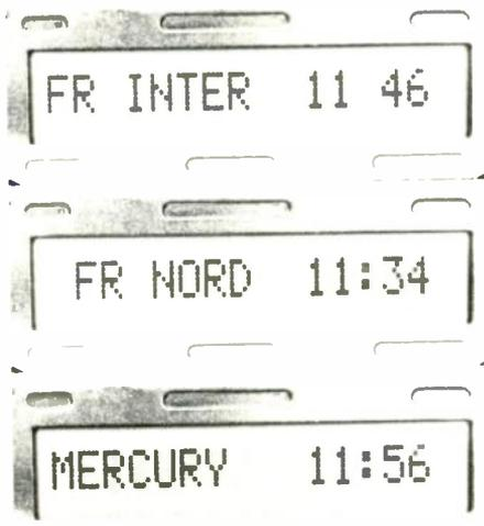
RDS is now being implemented by broadcasters all over Europe. These PS displays were received from the France-Inter and Fréquence-Nord services of Radio France, and from Radio Mercury, the ILR station for Reigate and Crawley.
