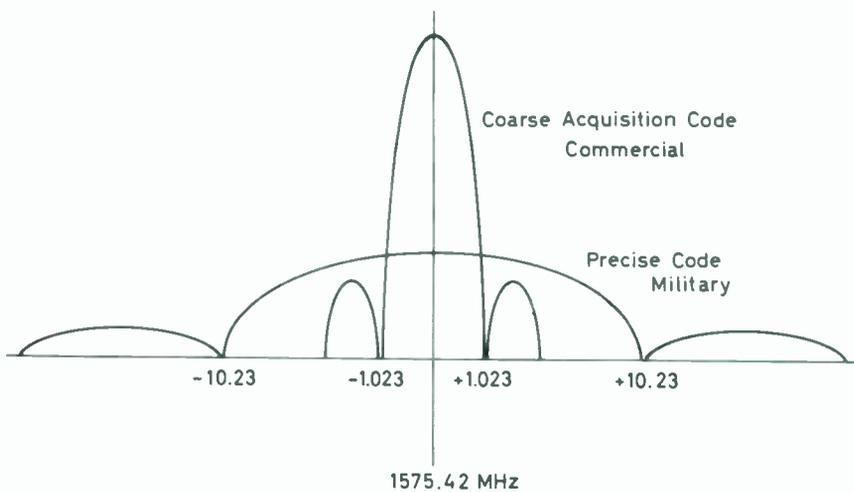
Fig. 2. In this GPS signal spectrum, the central peak is of interest; data contained in the wider curve is for military use and its code is secret.
