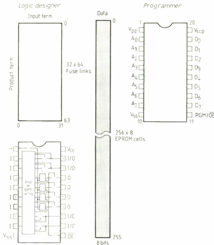
Fig.1. A PLD as seen from two different perspectives.
