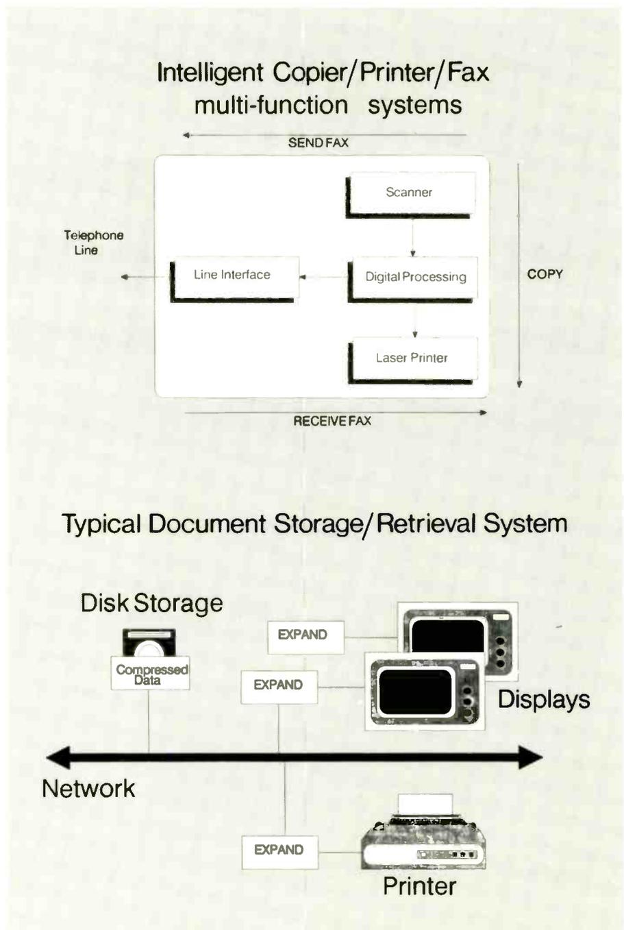
retrieval systems or multi-function copier/fax/electronic document processing systems. The ability to access a document stored on disk in compressed form, reproducing it on a display unit (in expanded form) in normal human reaction times, requires a very high throughput from the expansion processor. Such a facility would allow document browsing without the need for large, expensive buffer memory and make the resulting system more useful.
