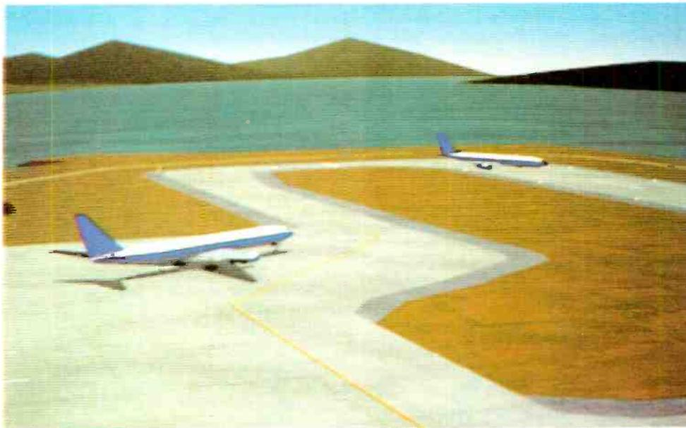
The flight deck exactly duplicates that of the aircraft type being simulated and is fitted with all controls and instruments. Forces fed back to the controls from the control surfaces are simulated and the pilot receives sounds relevant to that part of the flight envelope. The visual system reproduces the outside view and the whole thing is mounted on a system of jacks to provide motion cues to the pilot. All these processes are controlled by computer.
