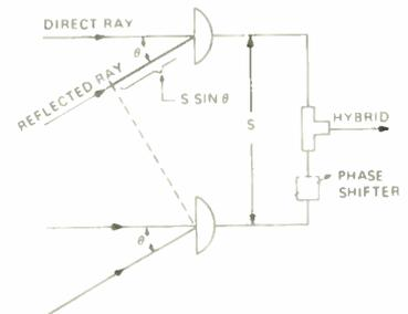
Fig.11. Reception of direct and reflected rays.
