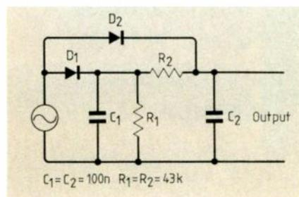
opposes the discharge of the main detector,  $\text{D}_2, \text{R}_2, \text{C}_2$ , allowing time constants to be shortened. Component values shown are for detectors working at 1kHz, having an output ripple equal to one per cent of the input signal amplitude. Discharge times of simple and improved detectors were 39 and 13ms respectively (measured as a time-constant).
