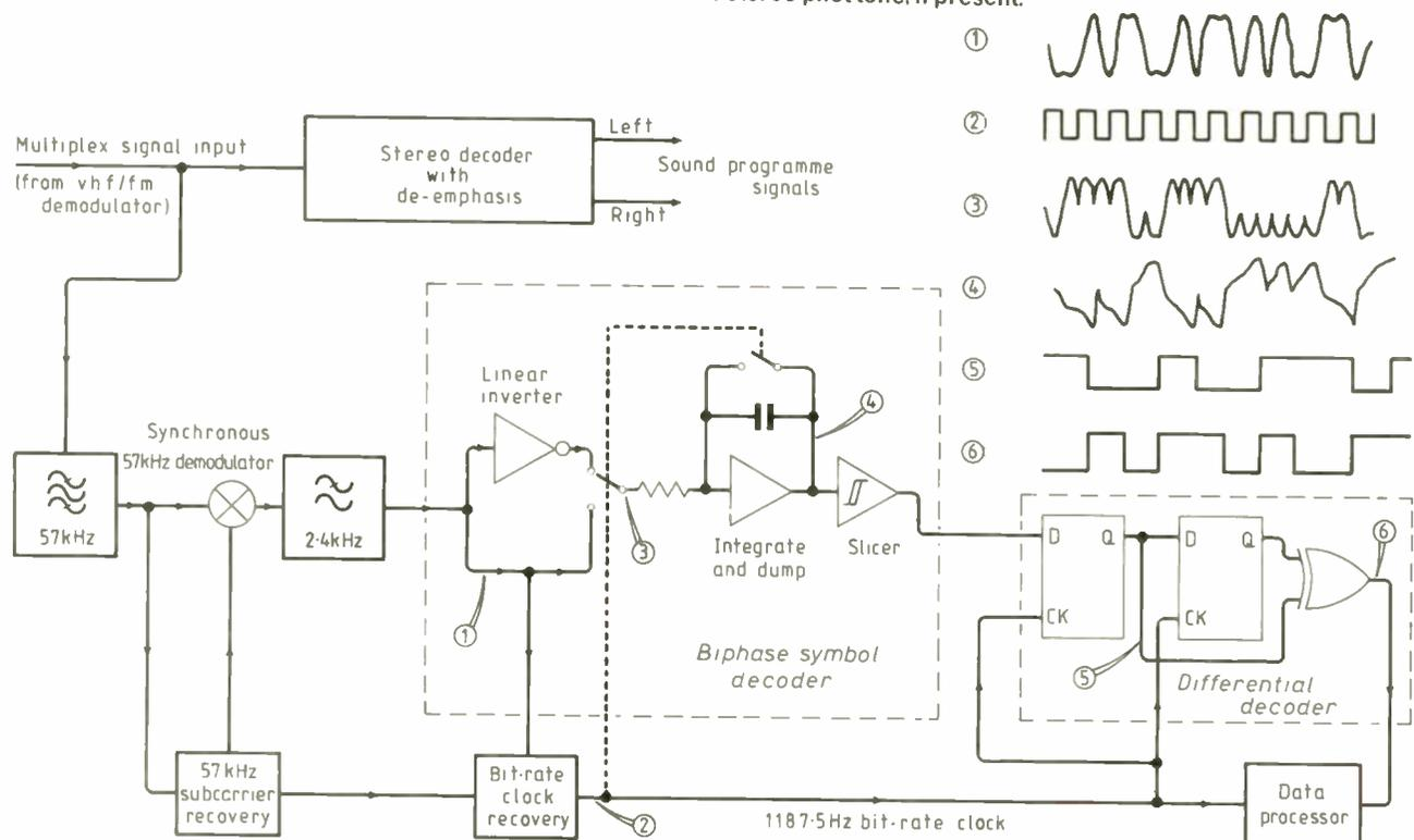
Fig. 2. Typical receiver decoding system for RDS. The rather complex modulation scheme was chosen to minimize the risk of interference to the audio programme.
