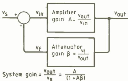
**Fig. 2. Negative feedback reduces distortion by  $1+A$ , and it has many other advantages, but it is not a cure-all. It does not reduce distortion produced in the subtraction process, and it can decrease stability.**
