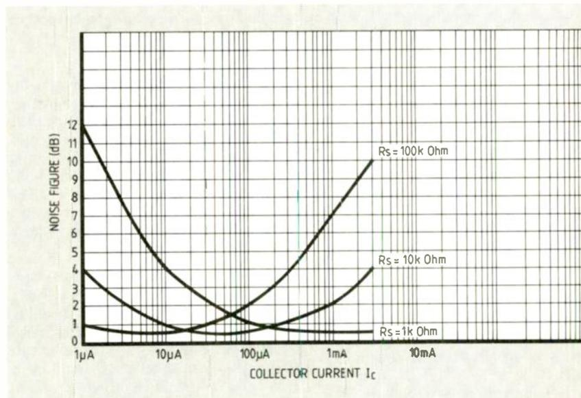
Fig.8. Noise figure and optimum source resistance  $R_s$  as a function of collector current  $I_c$  for an LM394 transistor.
