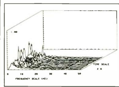
One of the most interesting finds in Doug Russell's brain-interface work (above, centre) is the tiny 40Hz ripple on this brain-wave graph that you can see disappearing towards the back of this three-dimensional plot.
