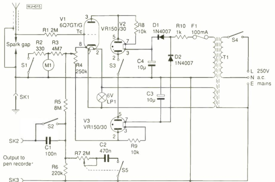
Fig.3. Circuit of the electrometer. It can accurately log atmospheric potentials in the range  $\pm 350V$  (by courtesy of the editor of *Practical Wireless*).
