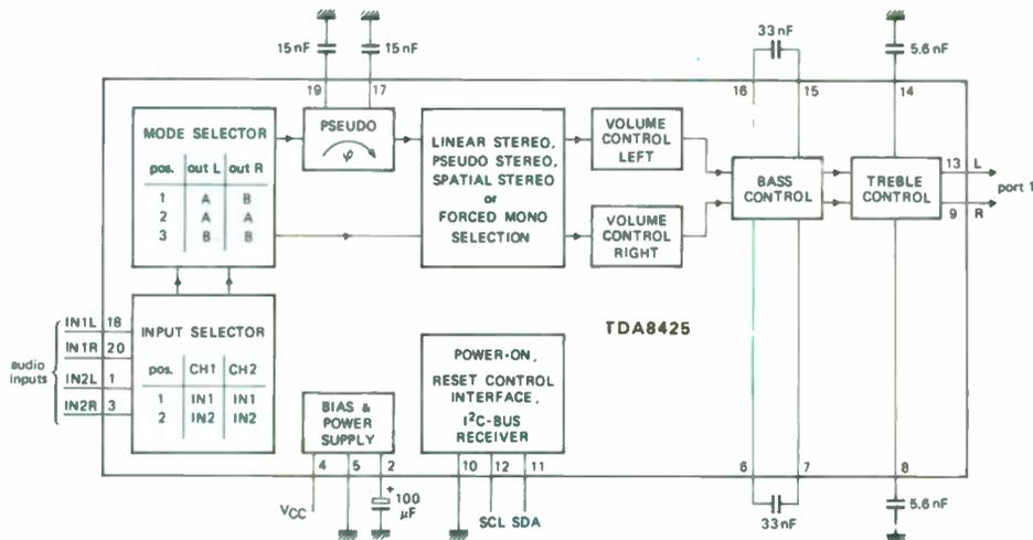
Fig.8. Hi-fi stereo sound processor for television receivers. Input selection, mode, volume, bass and treble are all controlled via the two-wire I<sup>2</sup>C-bus.
