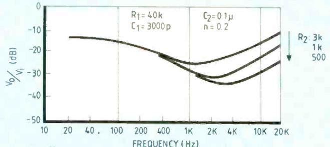
c.  $V_o/V_i$  - f curves for different values of  $R_2$
