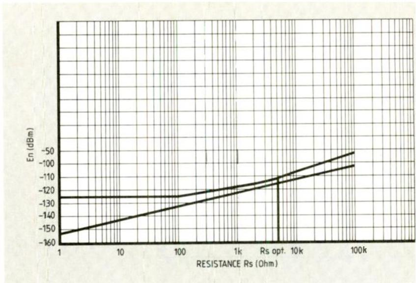
Fig.7. Optimum source resistance of an NE5534 op-amp (typical example without flicker noise in the audio band).
