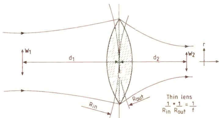
Fig.2: Re-imaging with a quasi-optical lens. Note that the radii of curvature  $R$  of the incoming and outgoing beams are not necessarily equal to the distances of the beam-waists from the lens.
