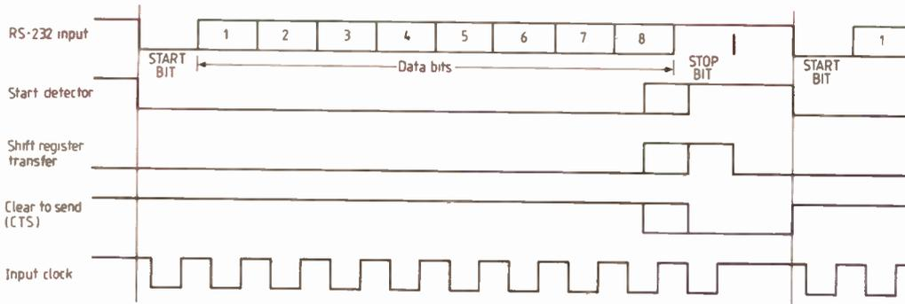
**Fig.2. Timing diagram.** Data is converted to parallel form within the circuit to allow for variations in timing between the input data and the FX439's clock.
