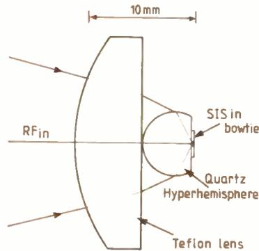
**Fig.4: Bowtie antenna on quartz hyperhemisphere. (From M.J. Wengler, D.P. Woody, R.E. Miller and T.G. Phillips, "A low noise receiver for millimetre and submillimetre wavelengths", in *Int'l J.IR and mm Waves*, vol. 6, No. 8 Aug. 1985 pp 697-706)**
