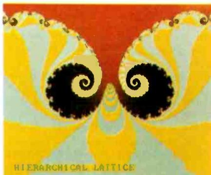
A Video Graphics Array 256-colour display. The large number allows subtle gradations in a display, though the limited resolution of 320 horizontally by 200 vertically loses fine detail.
