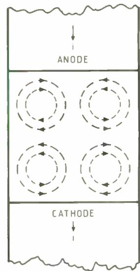
Fig.3. Circulation in liquid metal cell.
