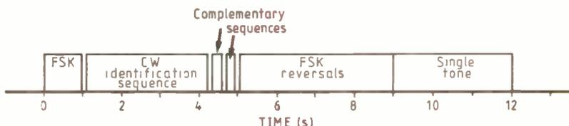
**Format of the 12-second beacon signals from the real-time-channel-evaluation (RTCE) system to be based on an HF network. This is due to become operational progressively from next July on frequencies near 5.5, 8, 11, 15 and 20MHz and will be suitable for automatic or manual use.**
