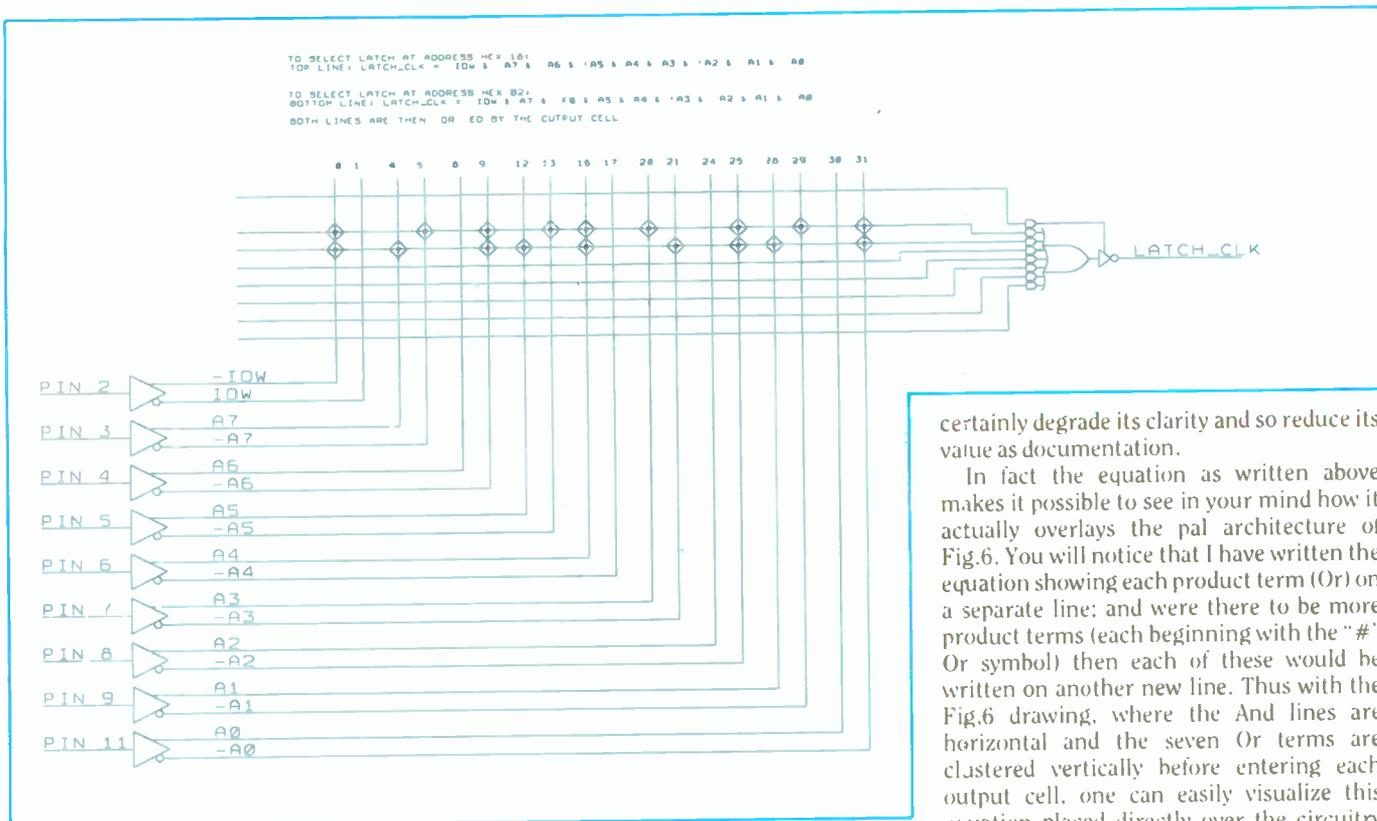
Fig.7. How your equations overlay the pal fuses.
