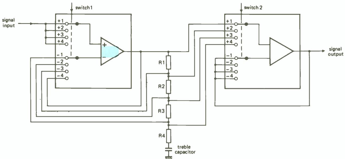
**Fig.5.** Adding a single capacitor allows the high-frequency response to be controlled. High-frequency amplification/attenuation is determined by the resistor values only, and the frequency range by the breakpoints established by the resistor and capacitor values.
