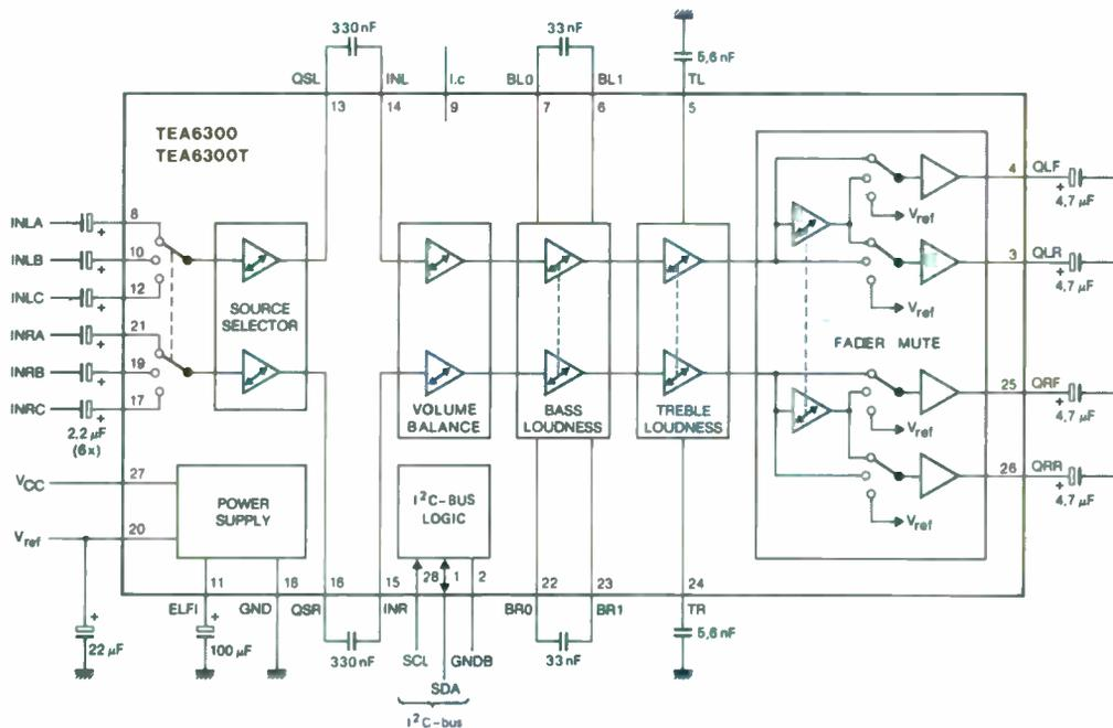
Fig.7. Car radio preamplifier based on the TEA6300. The volume/balance control consists entirely of linear op-amp stages.
