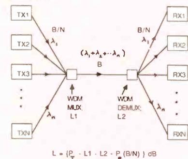
**Fig.4. Use of wavelength division multiplexing to provide high transmission capacity.**
