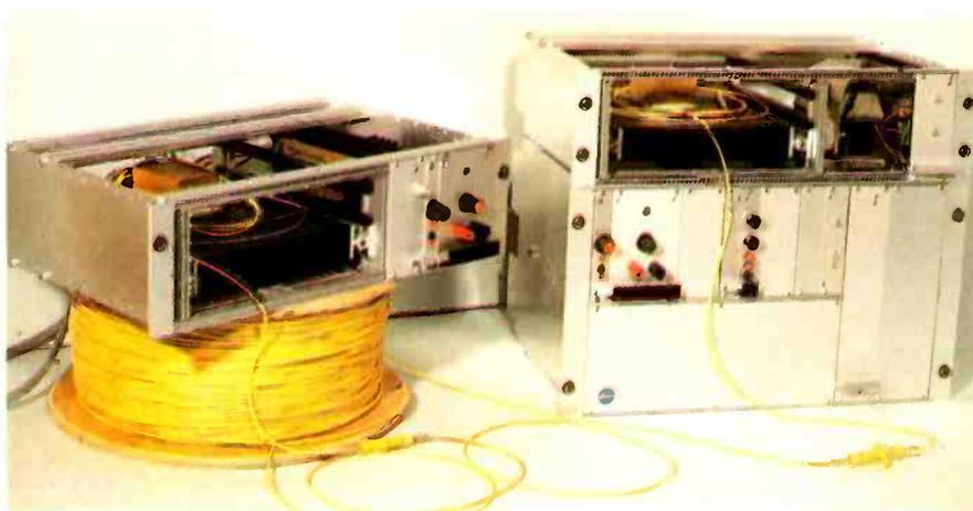
maturing rapidly. This technology is beginning to move into the phase of addressing performance and stability outside the laboratory environment. An example of this is shown in Fig.9 which shows a 140Mbit/s frequency-shift-keying system mounted in 19in racks for transportability.
