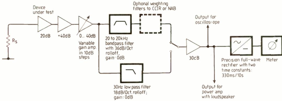
Fig.3. Block diagram of a noise measurement circuit for white noise and flicker noise.
