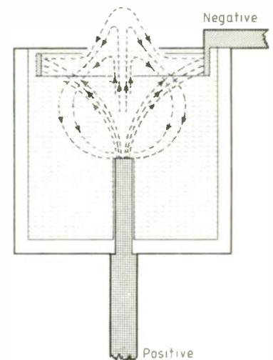
Fig.4. Above, cross-section through mercury fountain and (lower) photograph of it.
