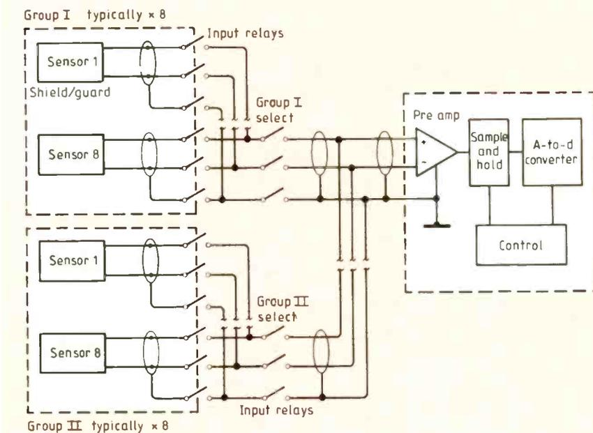
**Fig. 6. Typical multiplexer system.**
