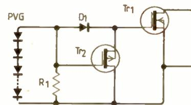
Fig. 5. Gate discharge circuit greatly reduces the release time of the PVR.
