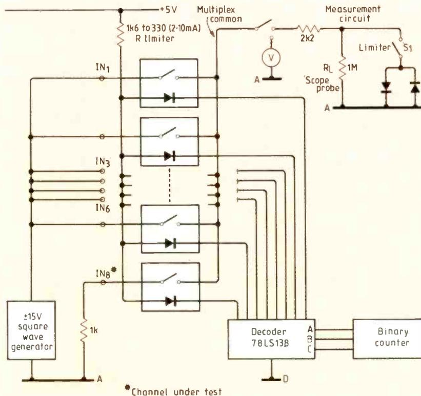
**Fig. 7. Eight-channel multiplexer test circuit using photovoltaic relays.**
