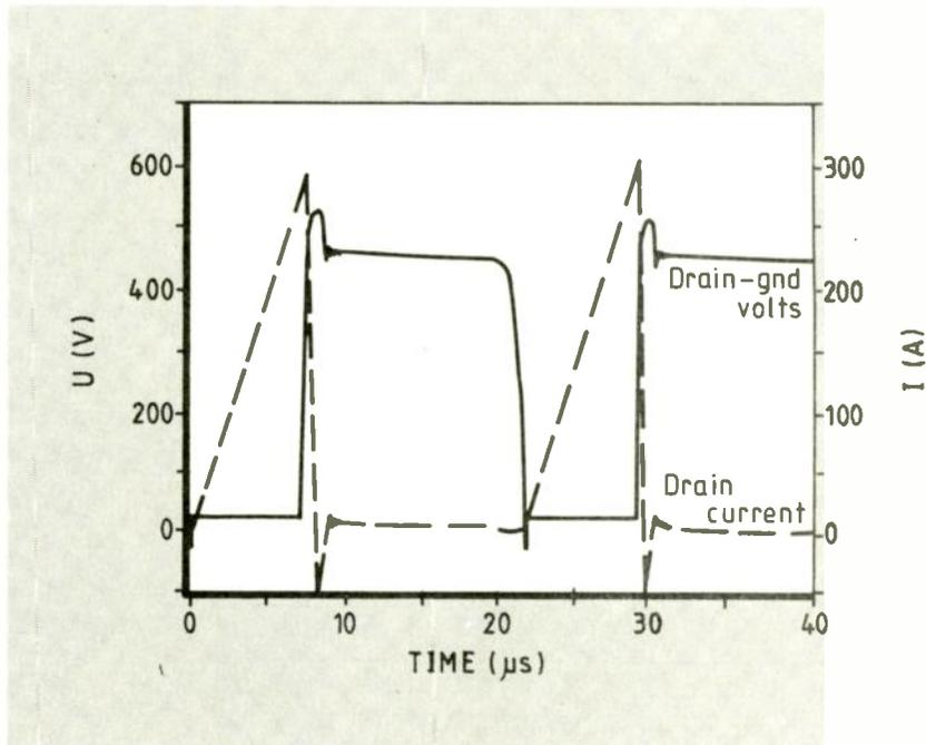
Fig.3. Transistor switching performance in full-load operation at 300V supply voltage.
