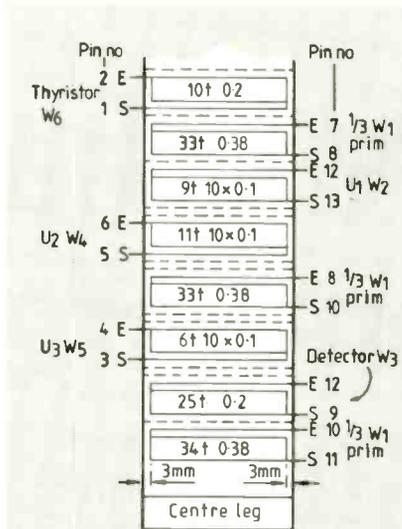
Fig. 2. Winding details of the transformer.
