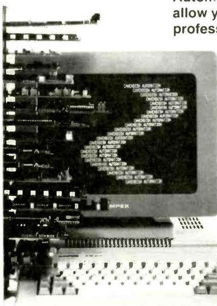
Off-the-shelf hardware includes numerous DACs, ADCs, bus-drivers and decoders, and many other forms of analogue and digital I/O cards, together with power supplies, backplanes, card cages and equipment cases.
