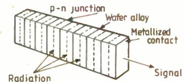
Fig. 3. Photovoltaic generator is a stack of series-connected photodiodes, edge-illuminated.
