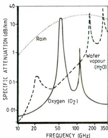
**Fig.1. Attenuation of millimetre-waves by atmospheric gases and rain. Oxygen ( $O_2$ ) has a particularly sharp peak at about 60GHz, cutting signal intensity by 95% for each kilometre. The effect of the various attenuations is cumulative.**
