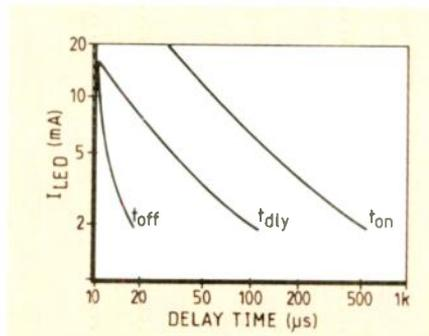
Fig.8. Typical switching delay for the multiplexer of Fig. 2.
