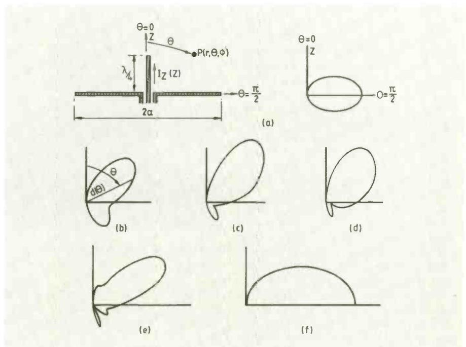
Fig.5. Vertical radiation patterns showing effect of the extent of the ground plane, as analysed by Melvin Weiner. Diagrams show elevation directive gain pattern of a thin quarter-wave element mounted on a ground plane of radius  $a$ : (a)  $2\pi a = \infty$  (i.e. wire radials in free space); (b)  $2\pi a/\lambda = 3$ ; (c)  $2\pi a/\lambda = 4$ ; (d)  $2\pi a/\lambda = 5$ ; (e)  $2\pi a/\lambda = \sqrt{42}$ ; (f) infinite ground plane (i.e. monopole over a perfect earth such as sea water).
