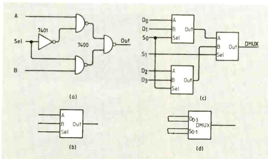
**Fig.2. The hierarchical method of information capture. Four levels of the hierarchy are shown, starting with the circuit at (a) and ending at (d) with a composite symbol incorporating several (a) circuits. The final diagram using symbols as at (d) is uncluttered with unnecessary detail.**
