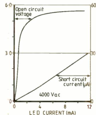
Fig. 4. Output characteristics of a 12-cell PVG.
