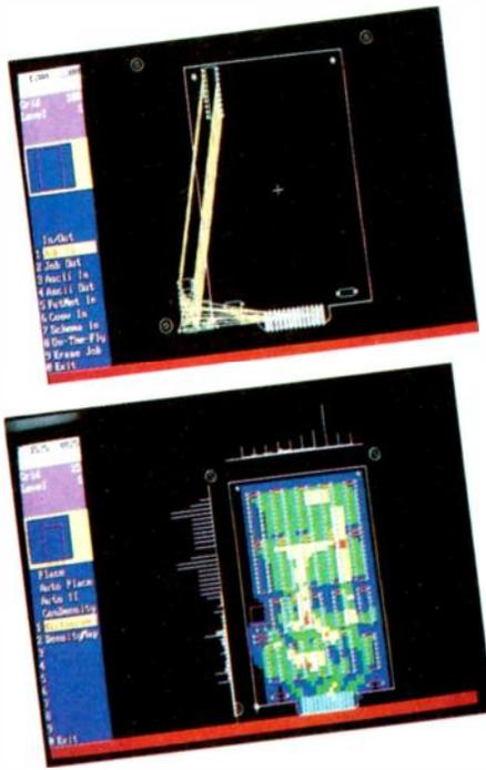
**Fig.1. Placement routine. Partial manual placement is shown at (a), while (b) shows full placement with connection density map and histogram.**
