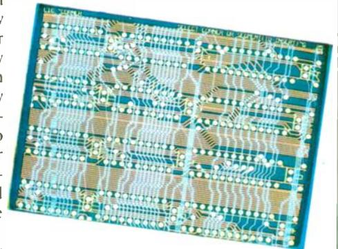
**Fig. 7. Two layers of a board layout using X and Y biasing.**
