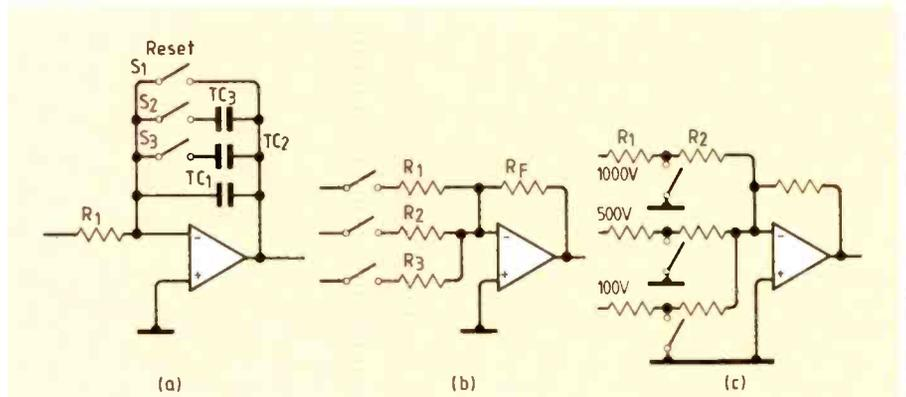
Fig. 12. Applications of photovoltaic relays: (a) integrator time constant and reset selector; (b) input selector; (c) high voltage selector.
