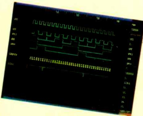
Fig.5. EE Designer III; waveforms for the circuit of Figure 3 calculated by the digital simulator. Initial conditions were set at random by the simulator. The row of figures is defined by assigning node voltages to bits in a word, in this case those giving the value of the count.
