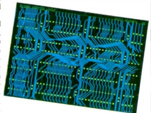
**Fig. 8. Gridless routing produces a higher track density.**
