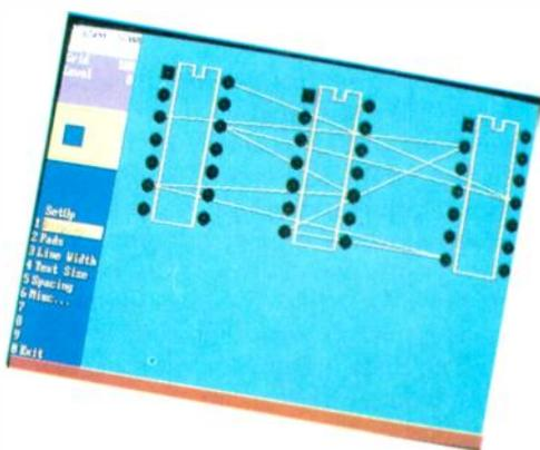
the next phase of the design is the conversion of the connections into tracks. When performed manually the operation of a cad system is closely analogous to the use of tape in a conventional layout. The great advantage which cad offers is the speed and accuracy of manual track placement. Editing is also considerably simpler, with modifications being quickly and easily made to 0.001 in resolution.
