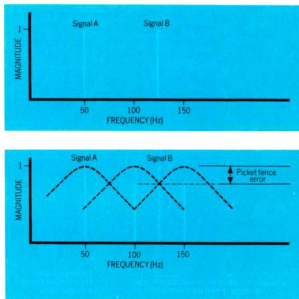
**Fig. 5. The picket fence effect. Signals falling between the lines, such as the 125Hz signal (above), could not be seen if each line was infinitely narrow. In practice, the lines have bandwidth, as below, and show the signal in each of the adjacent lines at reduced amplitude.**
