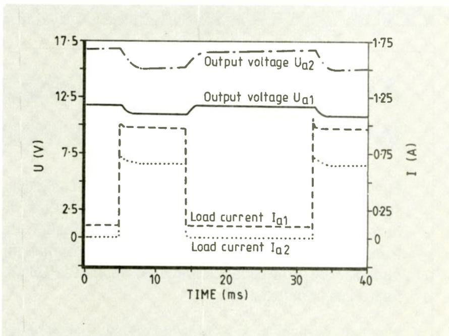
Fig.4. Dynamic performance of the converter with abrupt load changes.
