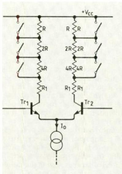
**Fig.2. On-chip resistor trimming of long-tail pair loads.**
