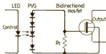
Fig. 2. Photovoltaic relay consists of led plus photovoltaic generator plus bidirectional mosfet.
