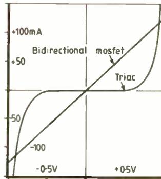
Fig. 1. Output characteristics of a typical bidirectional power mosfet.
