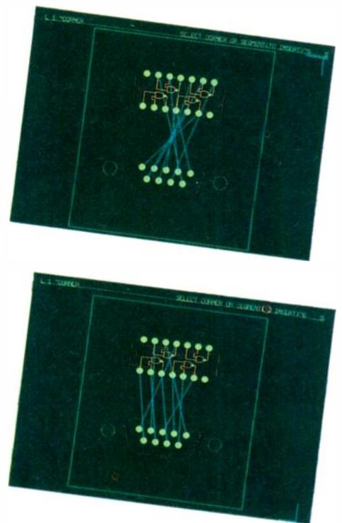
**Fig.5.** Optimising the layout by pin and gate swapping. The effect of swapping is shown below.
