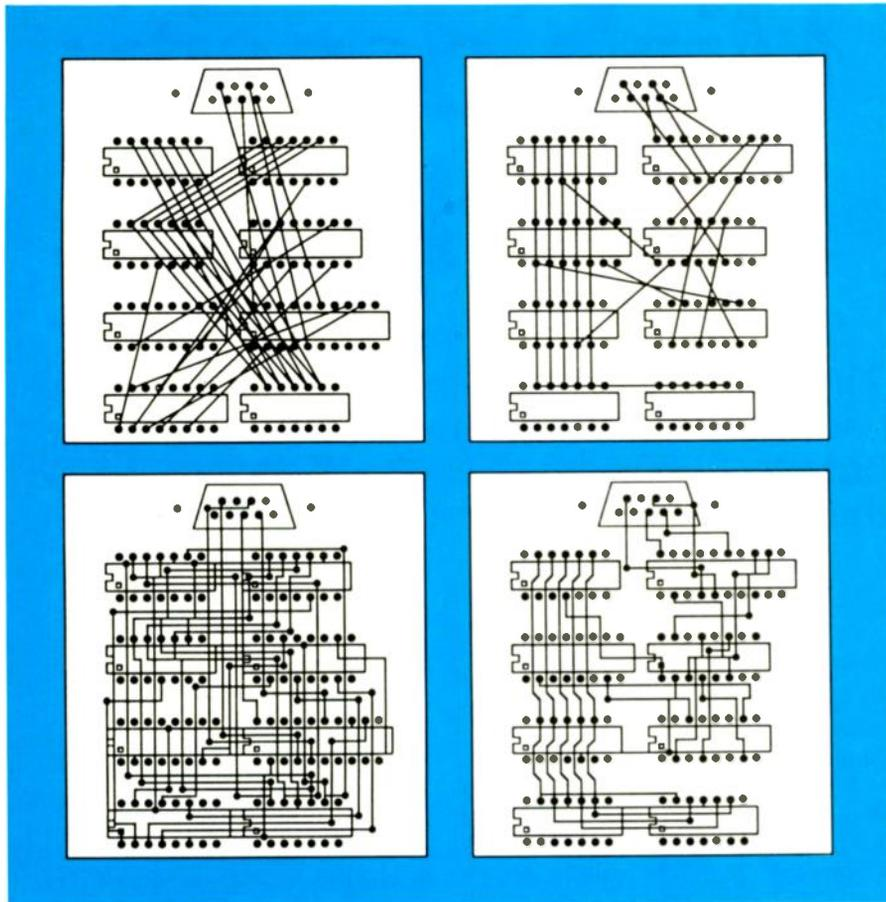
**Fig.3.** Component placement can be either random, as seen on the left, or according to the Manhattan algorithm, shown on the right. The improvement is obvious.
