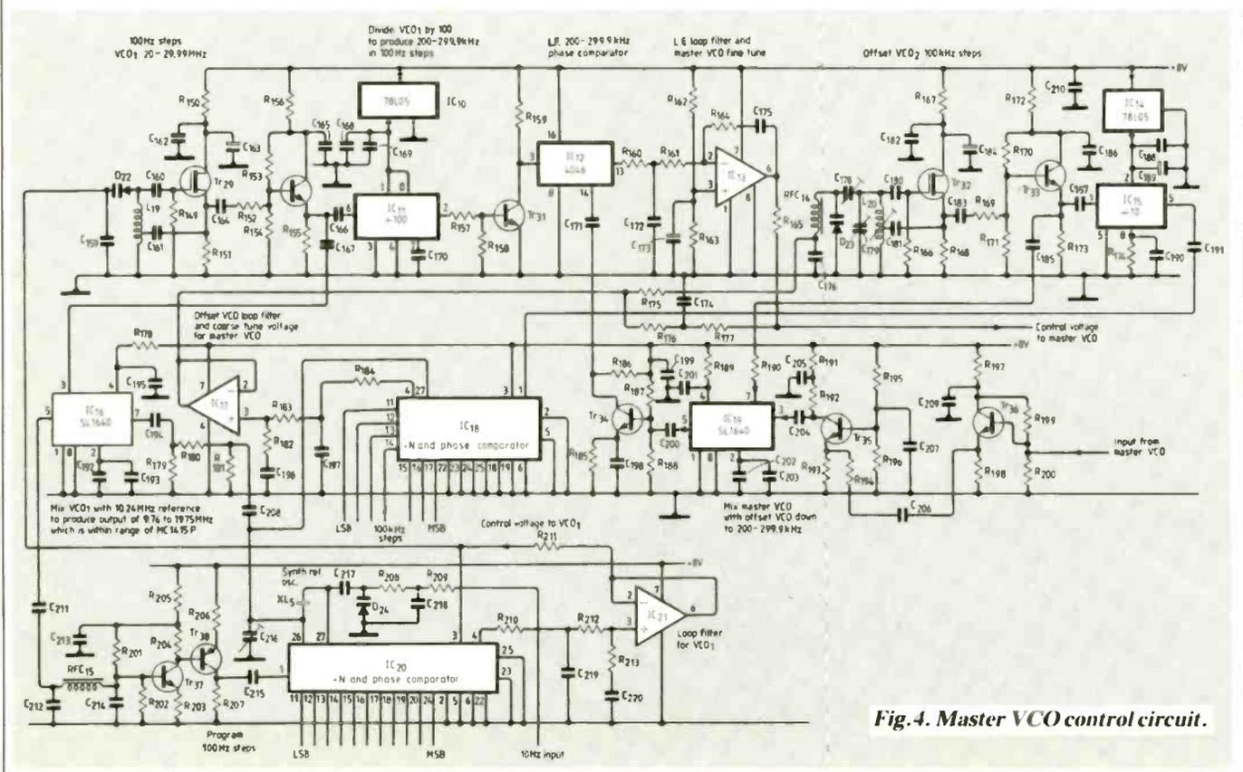
Fig.4. Master VCO control circuit.
