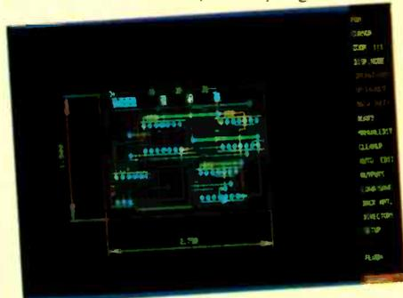
Fig.4. EE Designer III: layout for a two-sided printed circuit board. It can be displayed with trace widths to scale, as here, or with uniform thin lines. Components, except the connectors, and the traces were all placed automatically by the programme.
