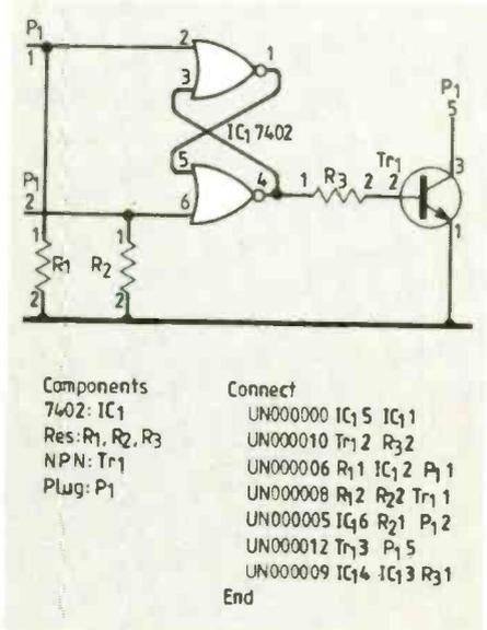
**Fig.3. A simple schematic diagram and its associated netlist.**
