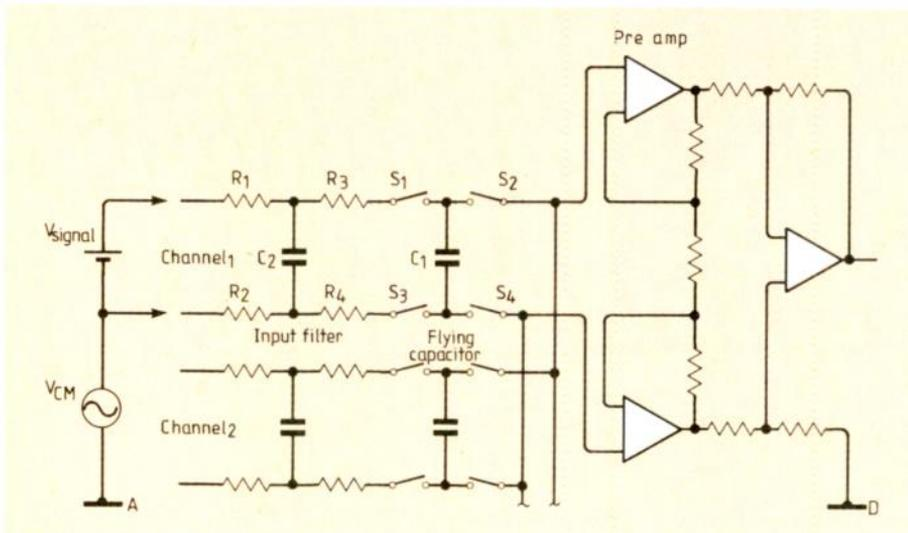
Fig.11. Flying capacitor multiplexer: this offers excellent common mode rejection and isolation of the common mode source from the measurement system.
