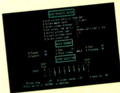
**Fig.3. User defaults screen used to select displayed layers and other screen defaults.**
