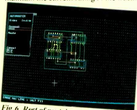
Fig. 6. Rest of routing completed manually.
