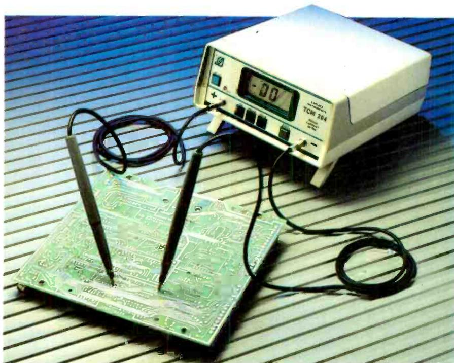
simple as it is novel, the measurement of DC potentials in the microvolt range has required some ingenuity on the part of the designer, David Mawdsley. The instrument requires twin contact electrode probes. An inner spring-loaded point measures potential while an outer fixed point provides the current injection. Successful measurement also re-
