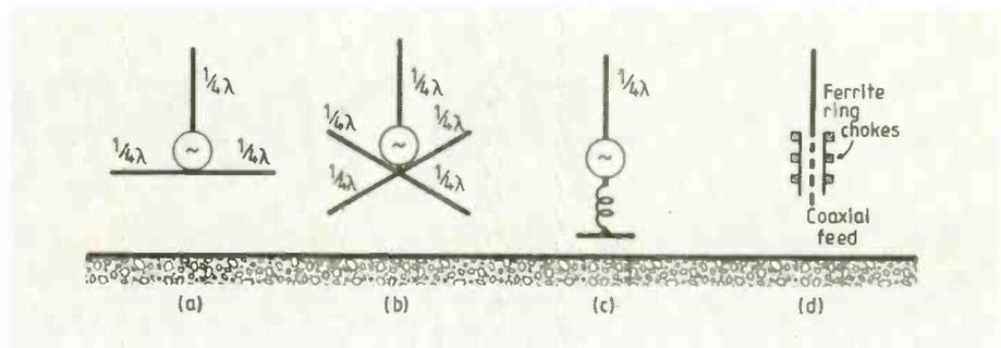
Fig.4. Elevated monopole ("ground plane") antennas: (a) original configuration as developed by Dr George Brown; (b) conventional four-rod antenna; (c) antenna with short loaded "counterpoise" as developed by Les Moxon; (d) zero-extent ground-plane antenna.
