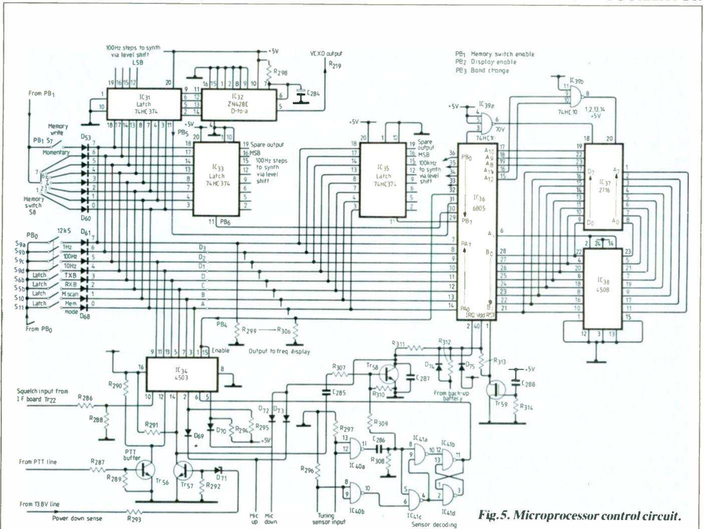
**Fig.5. Microprocessor control circuit.**
