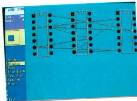
Fig.2. Length minimisation - before (a) and after (b).
