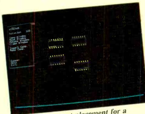
Fig. 3. Component placement for a simple board.
