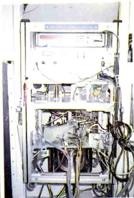
**Fig.4.** A 230-270GHz dual-polarization cryogenically-cooled Schottky-diode receiver mounted in the receiver cabin of The James Clerk Maxwell Telescope. The signal beam enters the receiver through the aperture above the middle plate.
