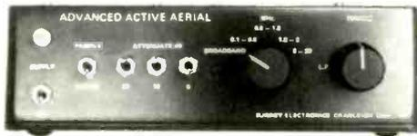
The aerial consists of an outdoor head unit with a control and power unit and offers exceptional intermodulation performances: SOIP +90dBm, TOIP +55dBm. For the first time this permits full use of an active system around the lf and mf broadcast bands where products found are only those radiated from transmitter sites.
