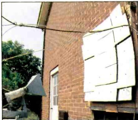
*View of the flat plate antenna. Outer plates can be set back in increments of half a wavelength, to reduce the physical depth of the reflector.*
