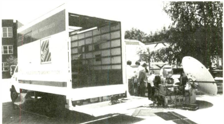
**BBC Radio's new transportable satellite dish makes it possible to relay events in stereo from sites far from the UK's main telecommunications trunks, where stereo links are not easily obtainable. Signals are downlinked to Broadcasting House.**
