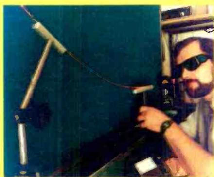
not marvellous compared to the performance of optical fibres at shorter wavelengths, but it should permit a whole new degree of freedom for surgeons using CO<sub>2</sub> lasers. What's more, ERA Technology and Cogent are already predicting considerably improved performance when the waveguide is manufactured using precision machine-drawn fibres. They are at present looking for suitable partners to develop the technology further.
