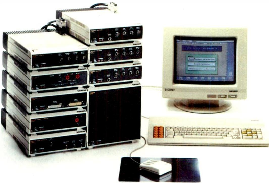
**F**our generations of devices in the development of electronic instrumentation have existed over the last thirty years. The "classical" form of instrument, with its pointer and rotary knobs, was soon followed by the second generation: instruments with digital displays, albeit still operated by knobs or push-buttons.
