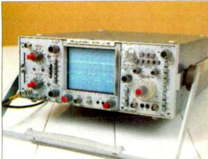
Telequipment D755 Dual Beam 50MHz
