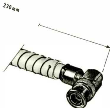
Experimental normal-mode helix antenna for portable VHF/FM receivers (BBC Research).
