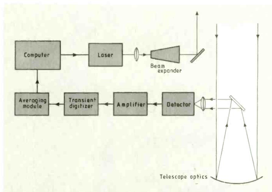
**Typical lidar block diagram. Aircraft mounted versions extend the scope of upper atmosphere research. NASA plans a satellite mounted Doppler lidar for wind speed measurement.**
