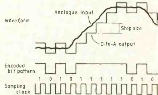
*The TMS3477 uses a CVSD (continuously variable slope detection) conversion technique for digitising speech.*
