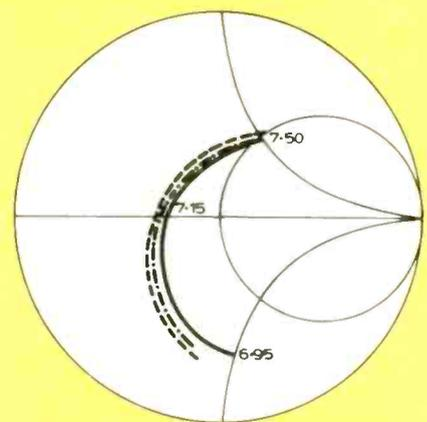
Fig.2. Input impedance of the Yagi-Uda array, by Lawson (solid line), Mininec (dots and dashes) and Pozar (broken line).
