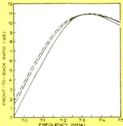
**Fig.3. Front-to-back ratio of the Yagi-Uda array: Lawson (solid line), Mininec (broken line) and Pozar (dots and dashes).**
