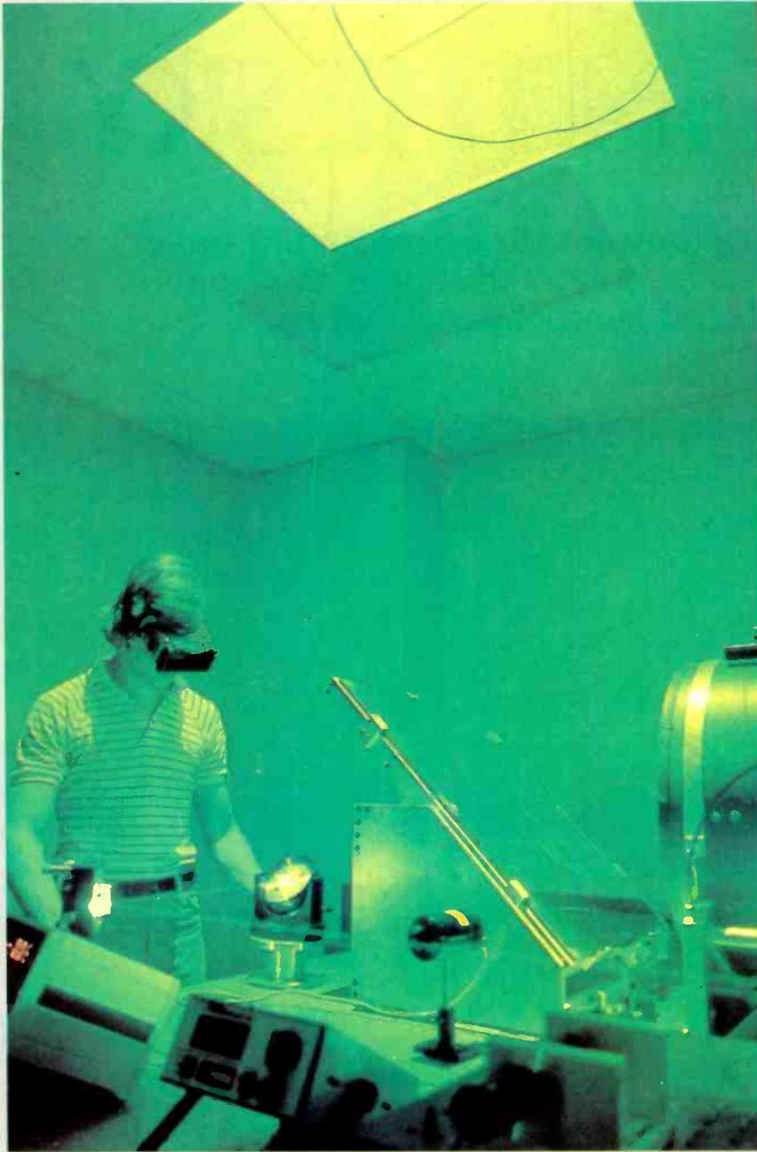
*The powerful lasers used in lidar can blind instantly at many miles. Extraordinary precautions have to be taken to ensure that nothing gets into the beam.*
