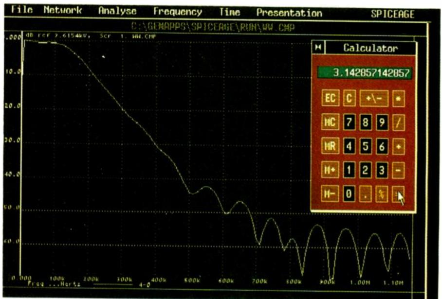
Fig. 5. Fourier transform of the transient response.
