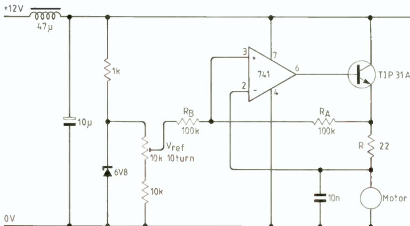
op-amp's input, the same voltage is dropped across  $R_A$ . Current through the resistor flows through  $R_B$  which has the same value as  $R_A$ , so the voltage at the bottom of  $R_B$  must be the same as the voltage applied to the motor. Since this voltage can be controlled by the
