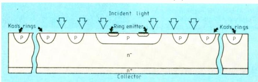
Fig.1 (above): cross-section of annular 3kV bipolar photo-transistor.
