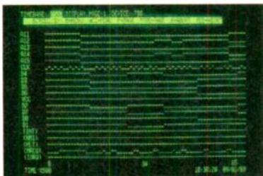
A Z80 logic trace showing part of the test sequence
