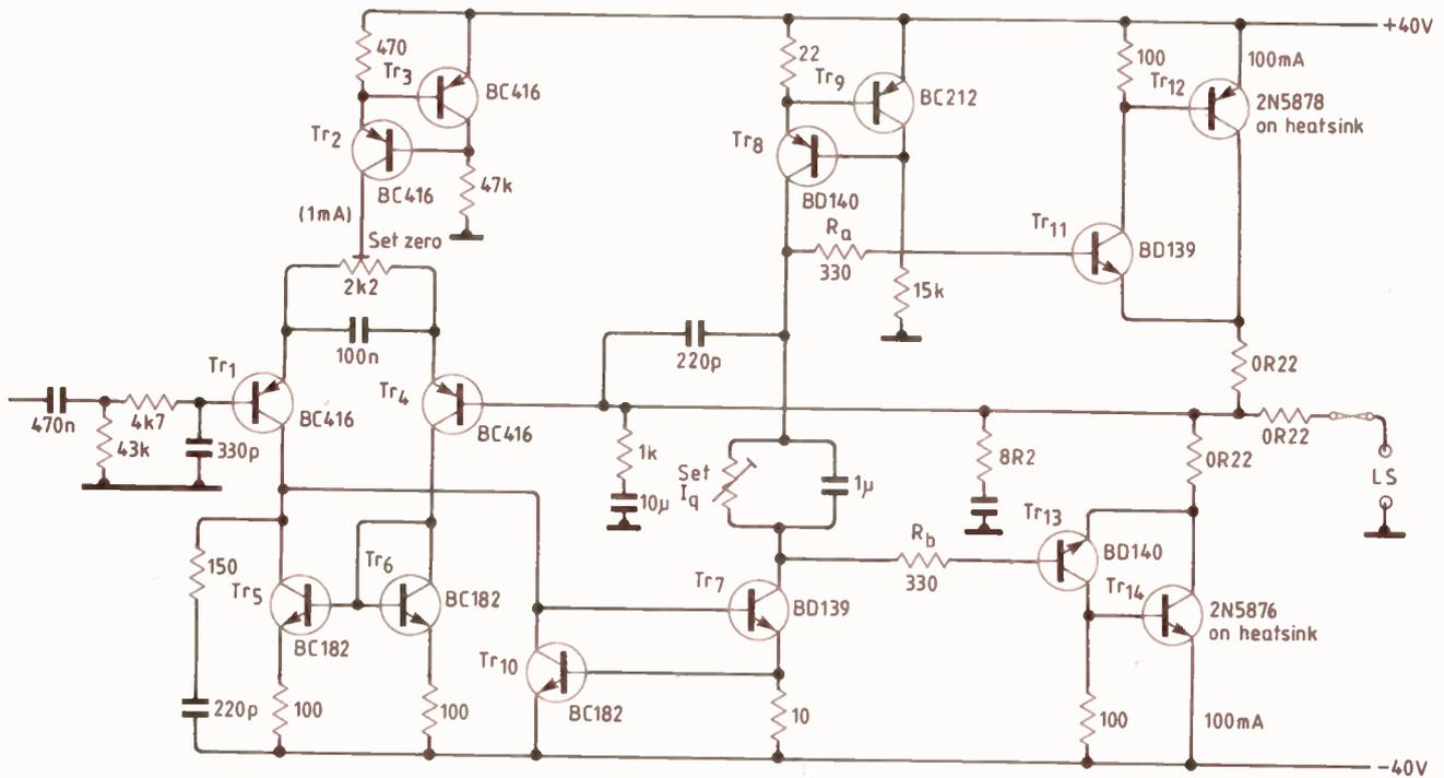
Some temperature compensation for the output transistor forward bias can be obtained from a suitable degree of thermal contact between the output devices and  $Tr_7$ .
