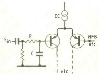
Fig. 16. Input RC filter restricts rate of input voltage change to that of rest of circuitry.
