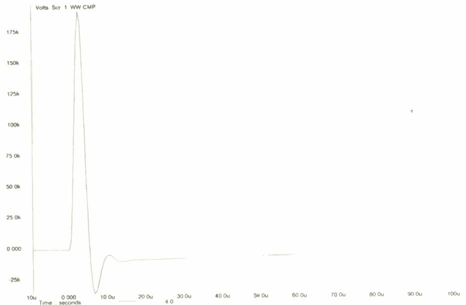
Fig. 4. The transient response of the circuit to a 1V impulse. Note the peak in excess of 175kV – try seeing that on an oscilloscope!
