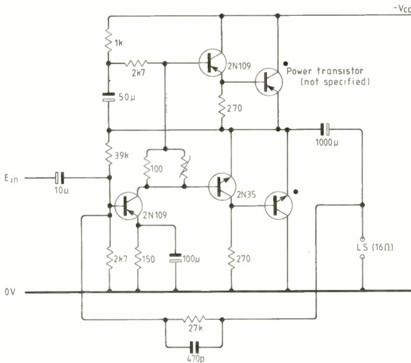
**Fig. 1. Original quasi-complementary transistor power amplifier by H.C. Lin, from 1956.**
