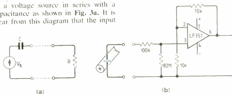
**Fig. 3. Sensor model (a) and a possible preamplifier design (b).**
