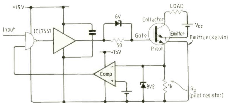
**Fig. 2. Using a pilot resistor for overcurrent protection.**
