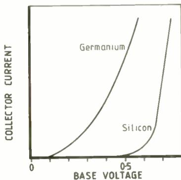
**Fig. 2. Comparison of silicon and germanium base-voltage/collector-current curves at 25°C.**
