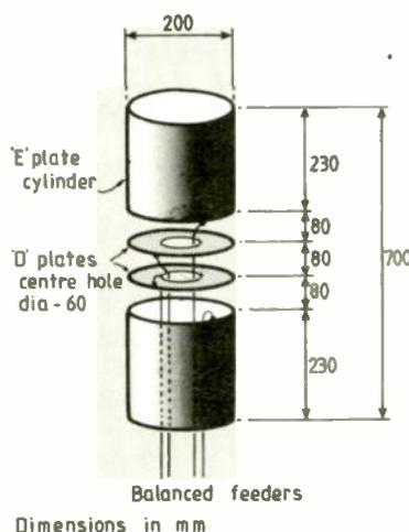
forming seven annular support members from polystyrene packing material. The 50% power split and phasing were arranged as in Fig.2. Perched on an easterly-facing window ledge, this unit yielded a number of successful contacts with British, Irish and European stations on 7MHz, at 100W.
