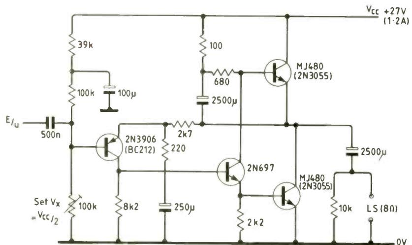
**Fig. 6. Author's 1969 10W class A amplifier. Since the operation is not push-pull, there is no crossover distortion.**
