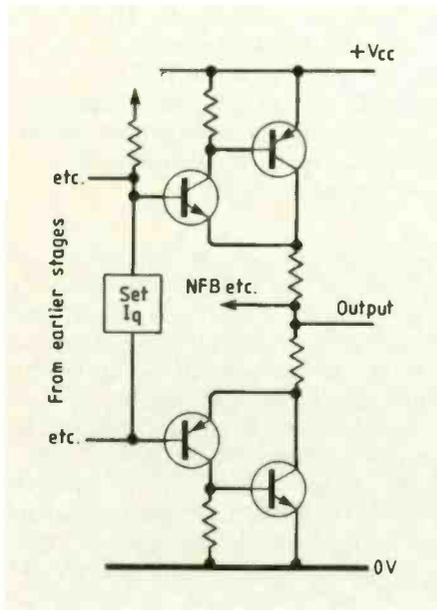
**Fig. 9. Symmetrical compound emitter-follower. Bias is less temperature-dependent.**
