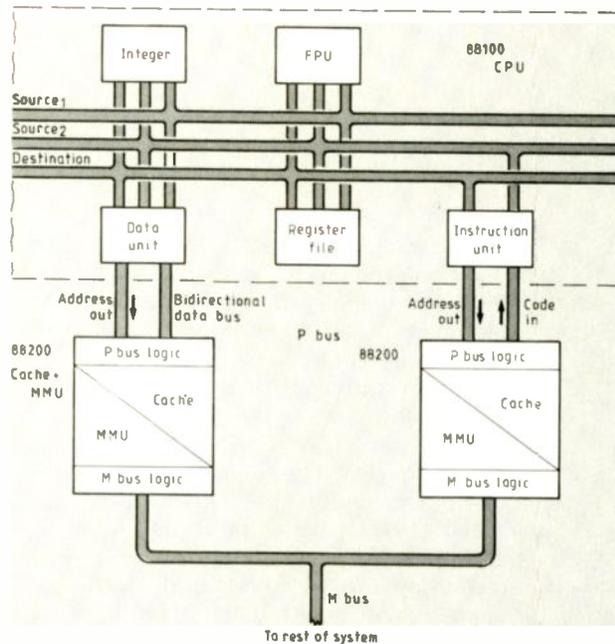
**In Motorola's M88000 risc family, the 88100 CPU talks to the rest of the world through the P-Bus Harvard architecture.**
