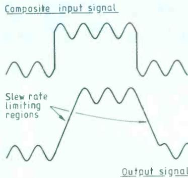
Fig. 15. Effect of slew-rate limiting.
