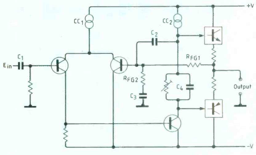
Fig. 17. Preferred position for HF loop compensation capacitor.
