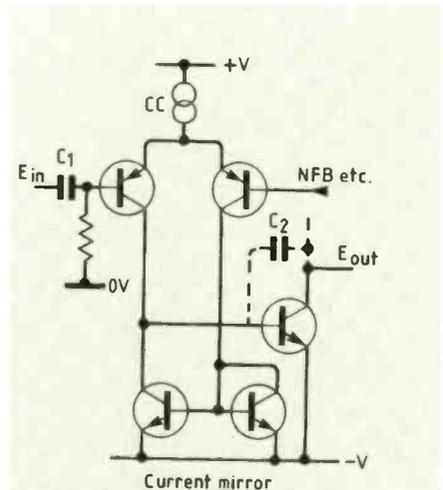
**Fig. 13. Current mirror presents high dynamic-impedance load.**
