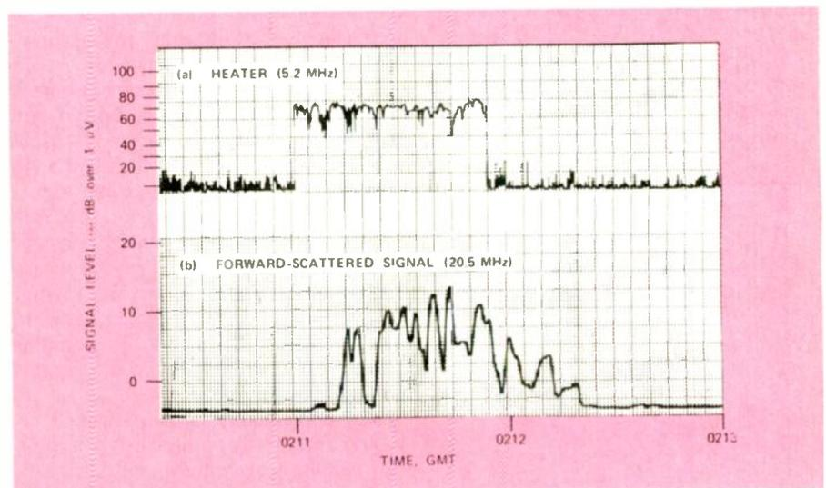
An example from the American experiments in the early 1970s showing F-region scatter reception of signals on 20.5MHz over an Arkansas/California path at a time when this was above the MUF. Signal enhancement appears about 20 seconds after the "heater" on 5.2MHz is turned on, with the signal again fading into noise some 20 seconds after the high-power transmitter is turned off. (Scattering characteristics of artificial radio aurora, by Victor Frank, WB6KAP, Ham Radio, November 1974).
