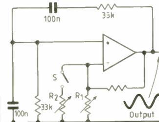
In the circuit shown, it would be easy to adjust resistors  $R_1$  and  $R_2$  so that with  $S$  closed, oscillations doubled in amplitude every second and with  $S$  open, halved in amplitude every second. If, at some time, the instantaneous amplitude were 1V and  $S$  were to be opened, the amplitude would decay to 1mV after 10s. If the switch were then closed, the amplitude would rise to 1V after a further 10s. If, however,  $S$  had been open for 24 hours instead of 10s, one would
