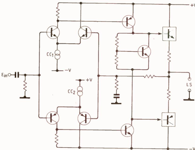
Bongiorno<sup>16,17</sup> and Borbely<sup>18</sup>, have offered fully symmetrical amplifier circuits of the form shown in Fig. 19, so that the maximum practicable rate of change of signal voltage at the gain-stage output is not limited by the final driver-stage constant-current source load.
