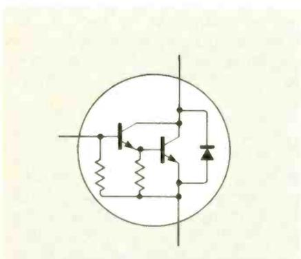
**Fig. 10. Internal structure of n-p-n Darlington transistor.**
