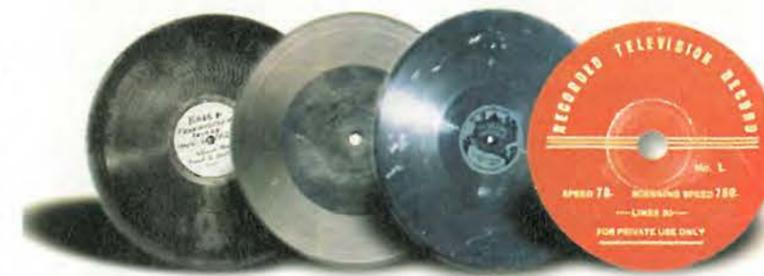
Fig. 1. Resembling contemporary audio discs, these are the different types of discs that contain the world's earliest-known recordings of television.
