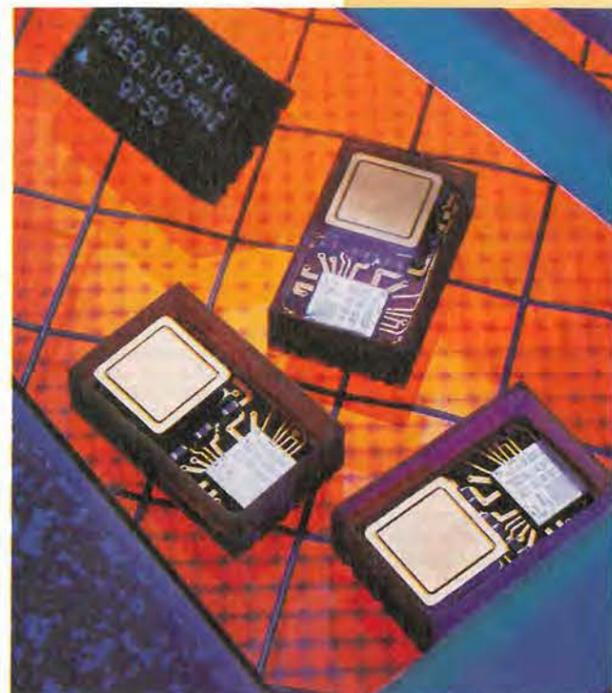
isolation voltage, high current transfer, high-speed switching and the option of multiple packages. The range is contained in TO-5, TO-18 and 8-pin and 16-pin dips in a variety of mounting choices, operating temperature being -65°C to 125°C. Faraday screening in the multiple units avoids common-mode interference and assists with radiation performance.
