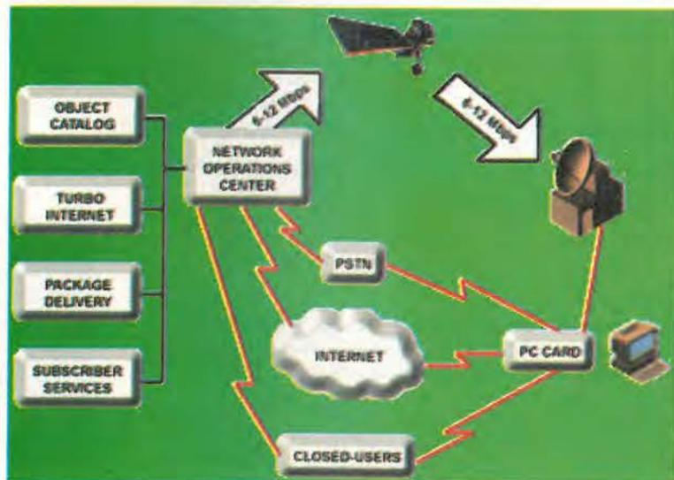
Fig. 3 With DirecPC, since Internet data is transmitted via satellite, downloading speed has a theoretical rate of 400kbit/s. Uploading still relies on a 14.4kbit/s modem connected to your telephone.
