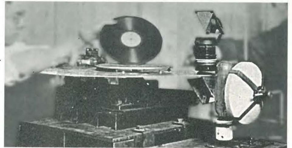
Fig. 8. The experimental 'Phonovisor' replay device used a large diameter Nipkow disc underneath the record platter. A light source at the right shines up through the disc via a mirror. This arrangement could also have been used for recording.
