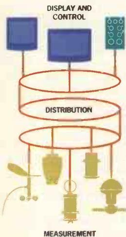
Above: The four main elements of this on-board information system for navigation at sea are measurement, distribution, display and control. Unlike traditional alternatives, this system keeps the four key elements entirely separate. The benefits: flexible information displays instead of fixed-role instruments, plus choice in the way you put together your boat information system.
