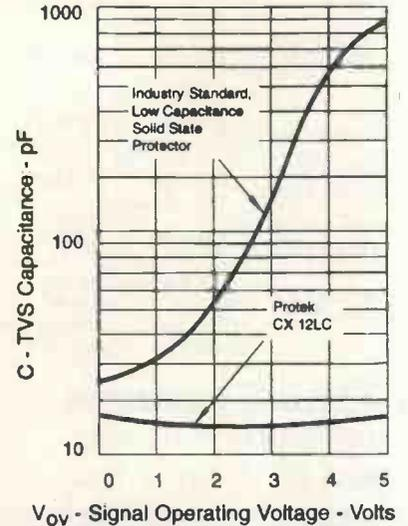
Capacitance in protection devices can be a source of significant signal attenuation.
