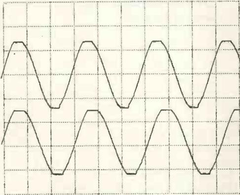
Fig. 8a) Two sine-wave outputs, a semitone apart.
