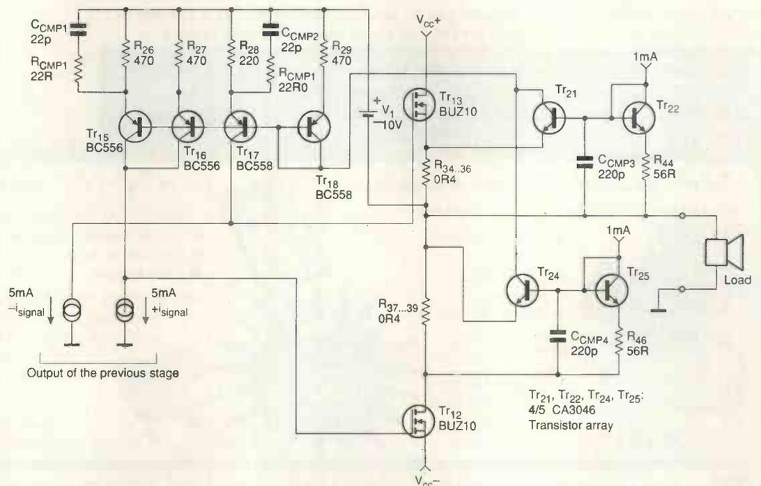
**Fig. 1. Simplified output stage of a power amplifier incorporating a non-linear common-mode loop. The circuit may look asymmetrical, but the source follower and common-source stages behave similarly when current driven.**
