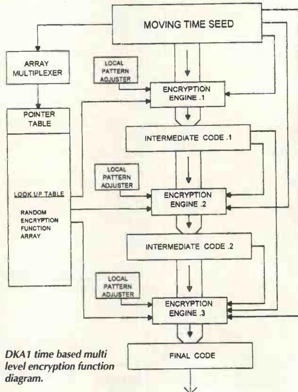
DKA1 time based multi level encryption function diagram.
