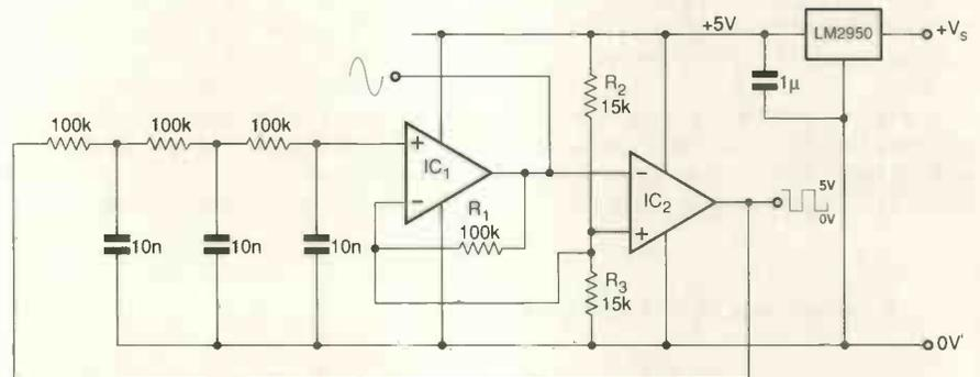
Fig. 3. With modern rail-to-rail-swing op-amps, this amplitude-stabilised RC oscillator achieves a sine-wave output of around 3.2V pk-pk from a 5V supply. Square-wave output is in antiphase relative to the sine wave.
