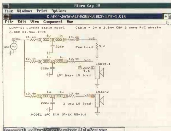
**Fig. 1. Working in MicroCAP IV, the sine source on the left is like a test power amp with infinite current and 1 $\mu\Omega$  output source impedance, so it can drive into three different loads down three cable models without its output voltage being significantly modulated.**
