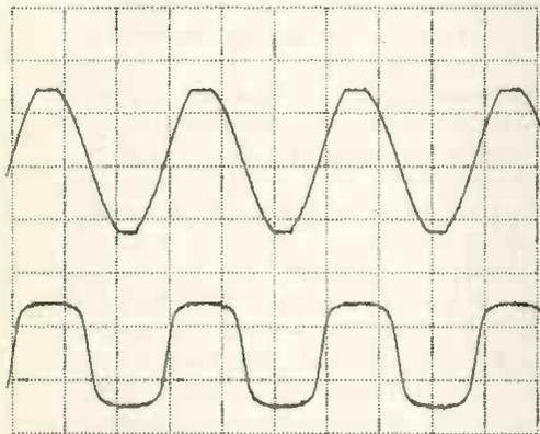
b) Comparing the 'square-wave', lower trace, with the input sine-wave.
