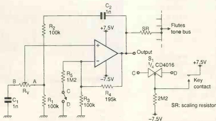
Fig. 4a) A keyed sine-wave generator. Using cmos switches for keying results in cheapness and compactness.
