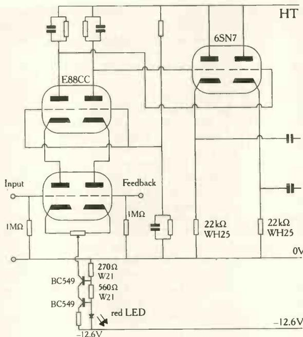
Fig. 1. Cascode differential pair with direct coupled cathode followers. Sometimes referred to as the Hedge circuit, this design differs because of the inclusion of cathode followers.
