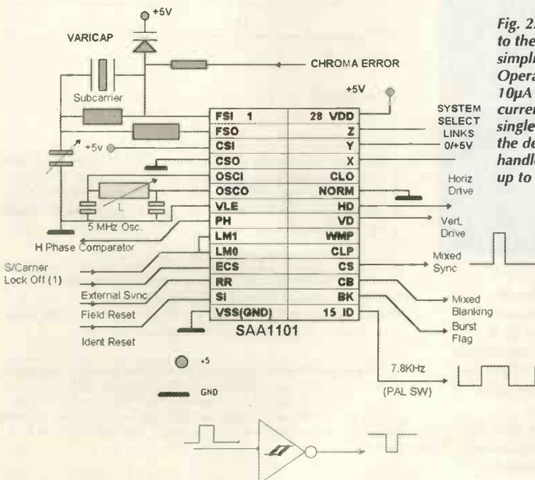
Fig. 2. Connections to the SAA1101 simplified. Operating with just 10µA quiescent current from a single 5V supply, the device can handle input clocks up to 24MHz.
