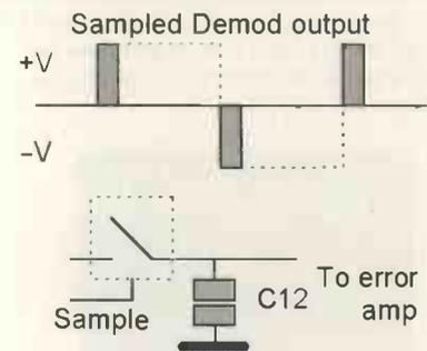
Fig. 5. PAL switch recovery basics.
