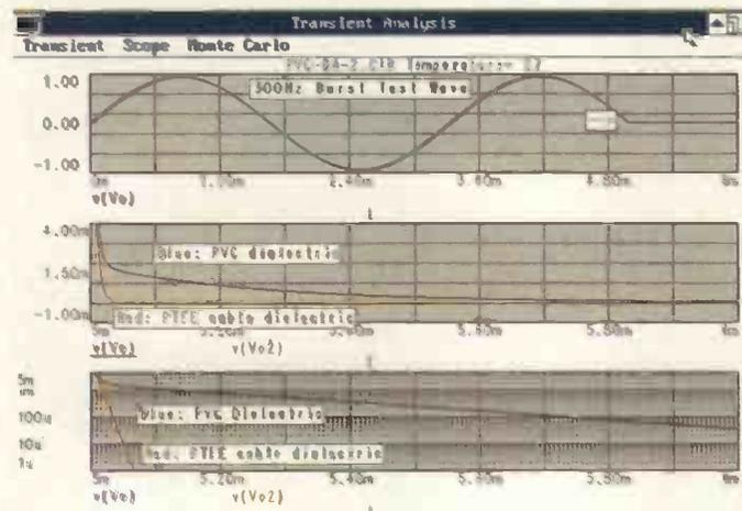
**Fig. 8.** Effects of dielectric absorption are clear immediately after the burst sinewave signal ceases (upper panel, arrowed). In the centre panel, voltage across the capacitance of an ideal cable falls to 0V within 20µs and at a uniform exponential rate. However, the discharge of voltage across a PVC dielectric has a dual slope and it takes at least 1ms, or 50 times longer, to come close to 0V. The lowermost panel employs a log scale to show how it has only decayed to 33µV in this time.
