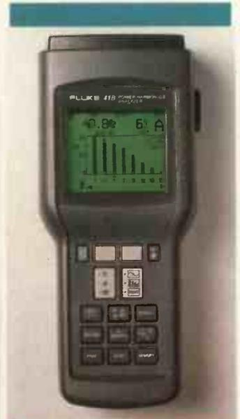
**Three-phase harmonic analysis.** Fluke's *41B Power Harmonics Analyser* is a handheld instrument measuring true rms voltage and current, frequency and power factor and displaying three-phase power. Display is as a waveform, as a bar-graph showing the level of harmonics present or as a numeric value, data being downloaded if required. PIDA. Tel. (and fax), 0756 799737.
