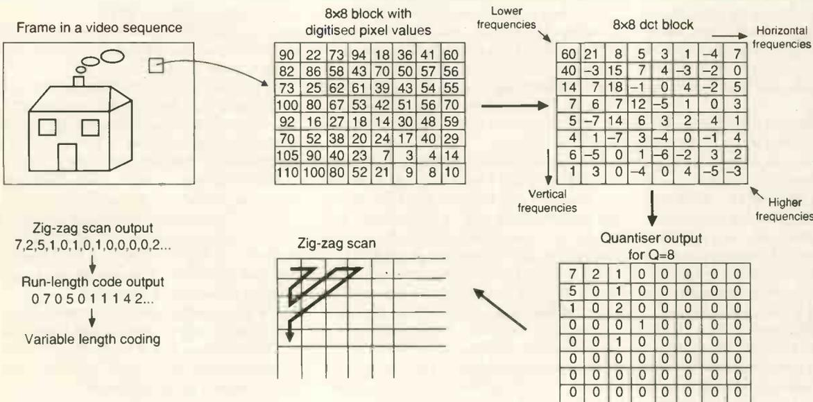
**Fig. 1. DCT-based video coding scheme. The discrete cosine transform (DCT) is at the heart of the coding schemes used in MPEG, JPEG and H.261. This figure shows how an 8 by 8 block of data is extracted from a field of video data. Note the presence of significant low frequencies in the 8-by-8 block of transform coefficients, with most of the higher frequencies going to zero after quantisation.**
