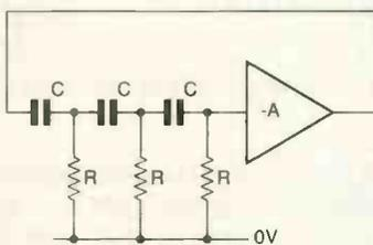
Fig. 2. The common CR-network based cascade oscillator relies on phase advance.
