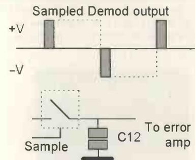
Fig. 5. PAL switch recovery basics.
