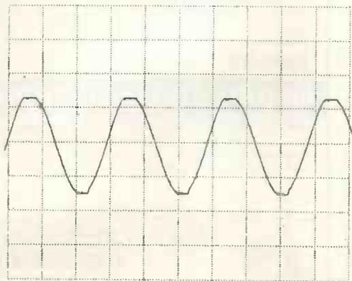
Fig. 2. Output of an oscillator based on Fig. 1 shows little distortion.
