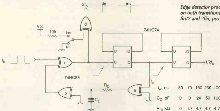
Edge detector producing output pulses on both transitions of the input at  $f_{in}/2$  and  $2f_{in}$ , positive or negative.
