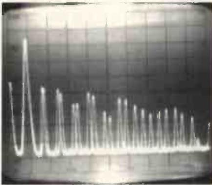
b) As a consequence, amplitude and harmonic content of the circuit's sine-wave output is virtually the same for both semitones. (10dB/div vertical, 2kHz/div horizontal, span 0-20kHz.)
