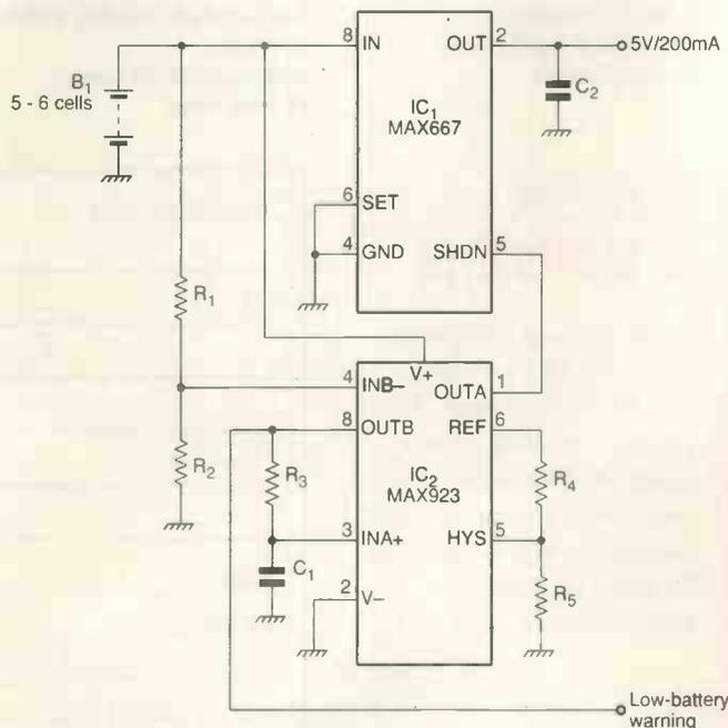
On detecting low battery voltage, this very frugal circuit issues a warning signal and shuts a power line down after a precise time interval, rather than after the usual, somewhat indefinite time taken for the battery voltage to decrease even further.
