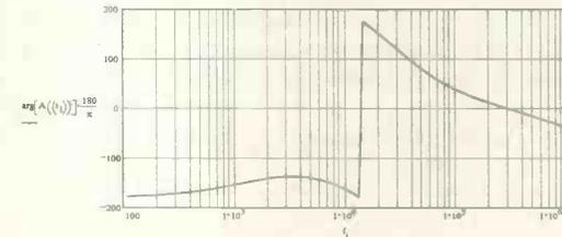
Transfer function (output phase to reference phase)
