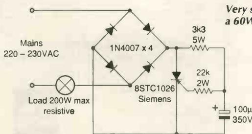
Very simple circuit to flash a 60W lamp at about 1Hz.
