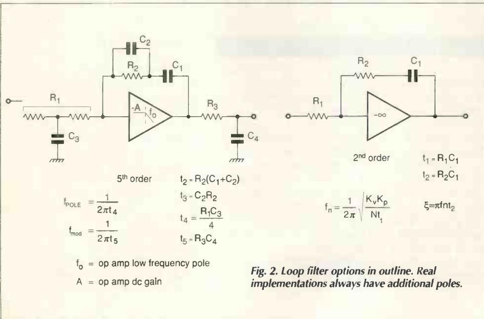
Fig. 2. Loop filter options in outline. Real implementations always have additional poles.
