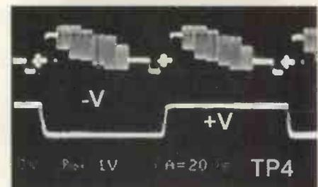
Fig. 6. Recovered PAL switch signal.
