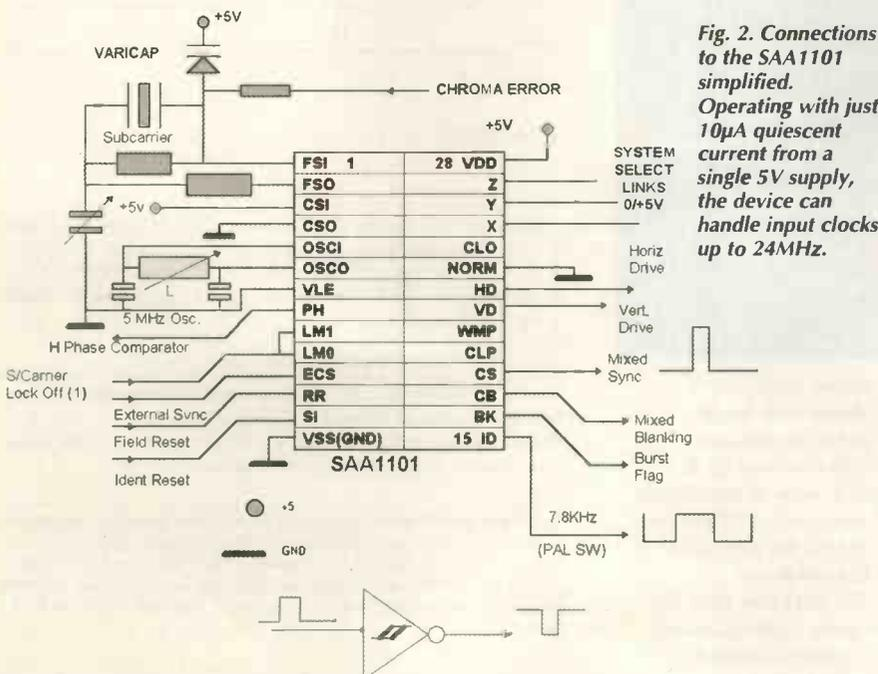
Fig. 2. Connections to the SAA1101 simplified. Operating with just 10µA quiescent current from a single 5V supply, the device can handle input clocks up to 24MHz.
