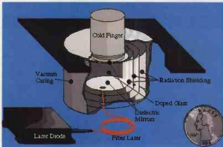
frequencies that are much higher than the possible frequencies at which the glass could vibrate. So when the glass is pumped with laser light at the right
