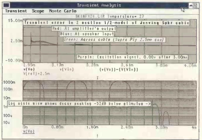
Fig. 13. Running the Fig. 12 model, showing how the decay error in the Jenving cable construction is much reduced, becoming comparable to the error tail of the power amplifier. This and Fig. 11 corroborate with Audio Precision dsp measurements taken on real cables<sup>4</sup>.
