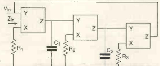
Using current conveyors instead of op-amps in this fdnc increases its bandwidth and improves stability with reactive loads.
