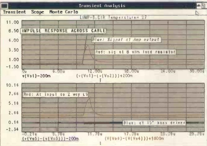
Fig. 4. Simulation permits differential measurements across lengths of cable that would be difficult or impossible in realspace. Here, the shark fins indicate the leading-edge energy in the pulse that appears across the cable – not the speaker.
