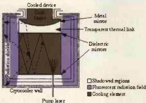
Input laser light is shown as the solid lines and fluorescence as the dashed ones. Violet-coloured areas indicate the regions where the fluorescent radiation is most intense. White areas are in the shadow of the dielectric mirrors. These shadowed regions are not completely free of fluorescent radiation, however, due to the band pass of the dielectric mirrors. Hence, a metal mirror and baffles are required to fully eliminate fluorescent-radiation heat loading of the object to be cooled.
