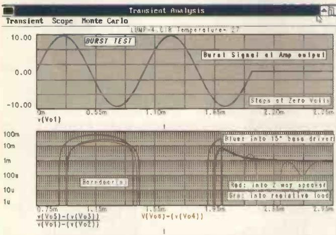
Fig. 5. The test condition is as Fig. 4, but the signal is a sine wave burst, stopping at 2ms where it is at 0V. Due to phase shift in the cables, the signal at the speaker end at this instant has not reached 0V.
