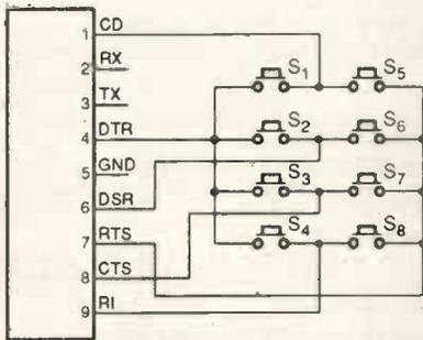
This circuit reads eight buttons through the pc's serial port.
