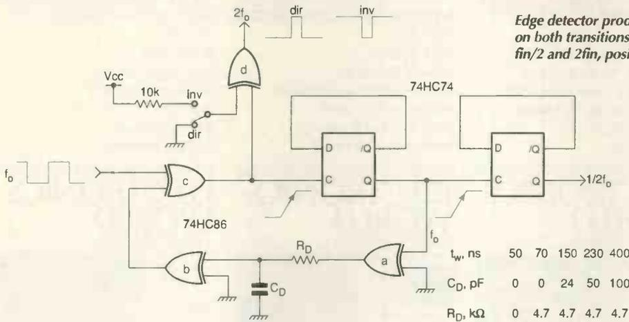
Edge detector producing output pulses on both transitions of the input at  $f_{in}/2$  and  $2f_{in}$ , positive or negative.
