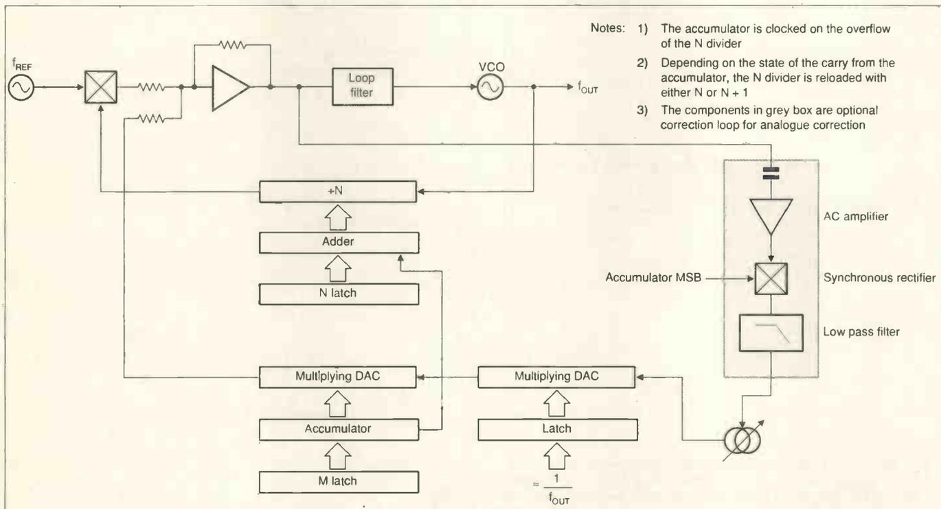
Fig. 3. Basic fractional-n synthesiser with additional d-to-a converter for scaling the correction by  $1/f_{\text{out}}$ .
