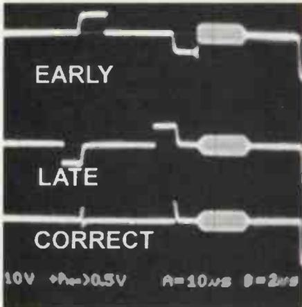
Fig. 7. Horizontal phasing – cancellation of sync on locking input by sync out from the sync generator, using the A-B display on an oscilloscope.
