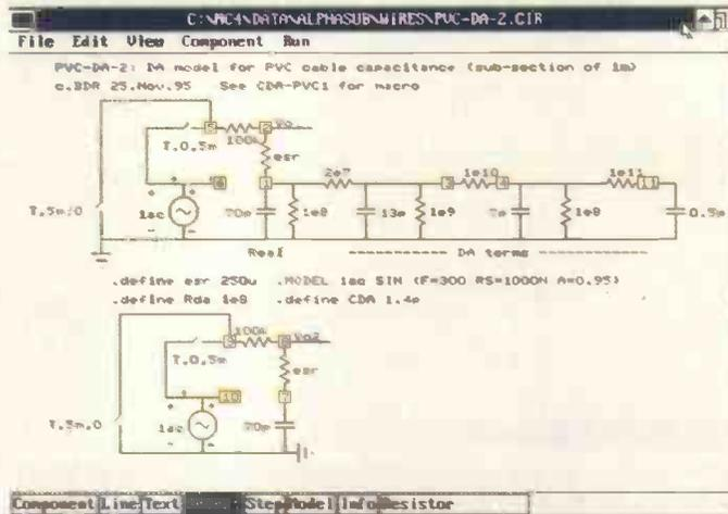
**Fig. 7.** The RC networks on the right are modeling dielectric absorption in a 0.3mm length of the PVC. On the left, a sine source is connected via a time switch. The point following the switch is shorted after this time. As a result source impedance is zero. In the lower circuit, the stimulus and main capacitor are identical. Only the components simulating dielectric absorption are omitted.
