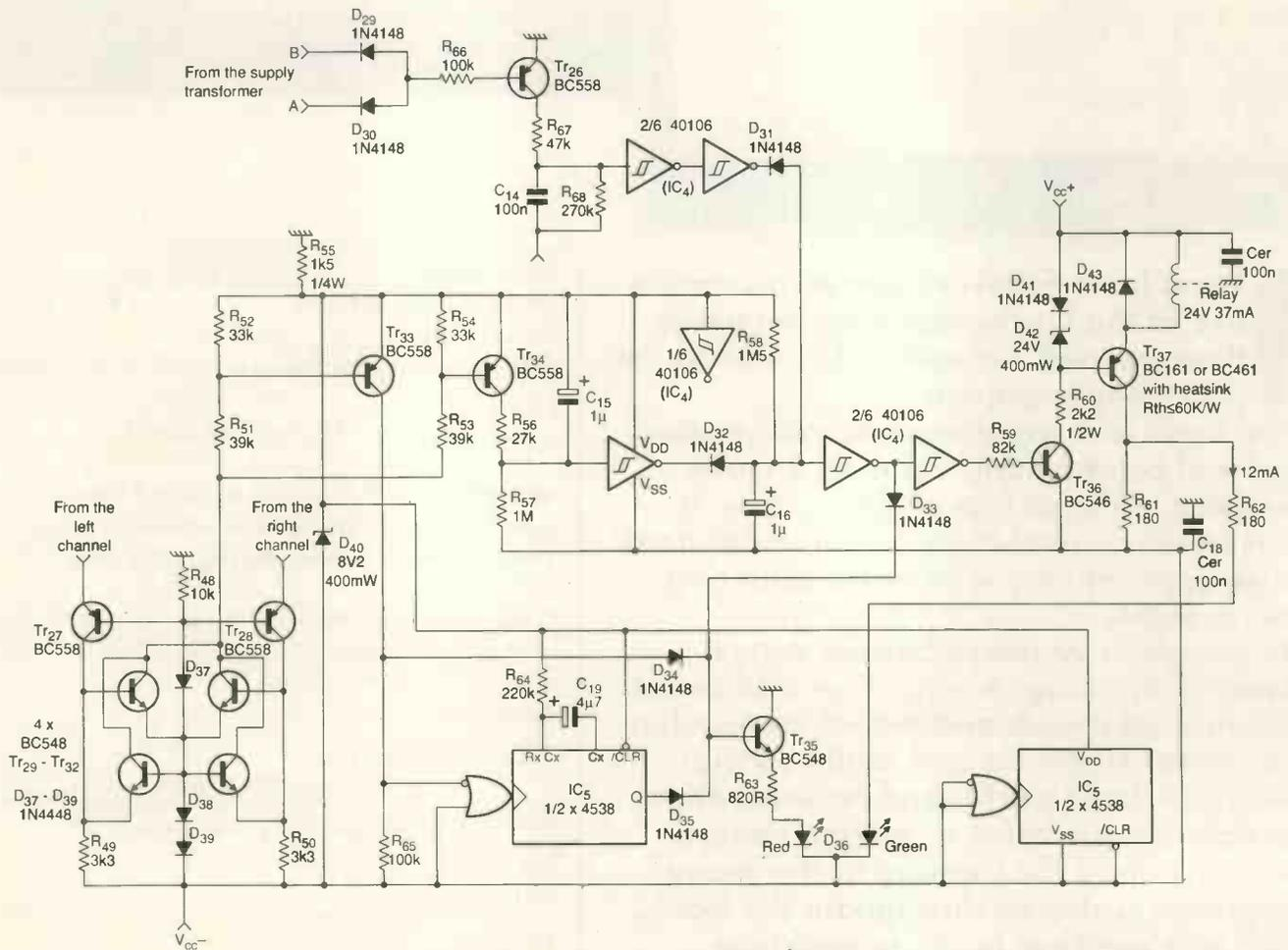
**Fig. 4. Power supply and protection circuit, common to both channels of a stereo amplifier. The relay is a double pole type which switches both channels on or off.**
