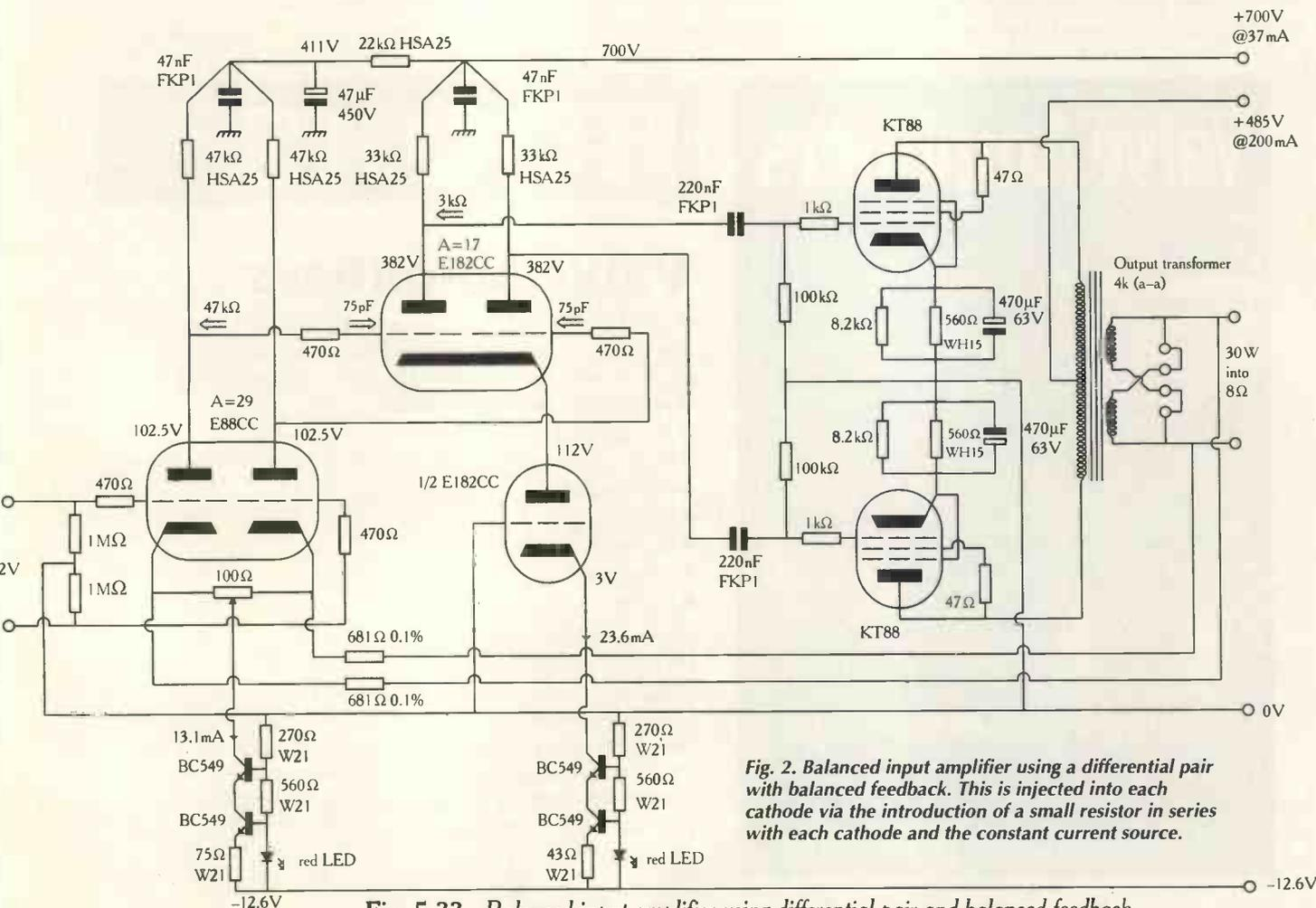
Fig. 5.33 Balanced input amplifier using differential pair and balanced feedback
