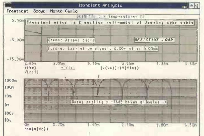
**Fig. 15.** Model of Jenving's Supra Ply cable correctly predicts an approximately 20dB lower peak perturbation (-54dB arrowed, lower, where the decay angle changes). The upper plot shows that after 3.0ms, amplifier output error is of the same order or likely dominant.
