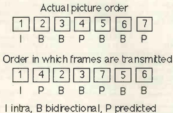
*Fig. 3. Transmission of MPEG 1 frames. MPEG-1 is particularly suitable for video CD, and is optimised for operation at around 1.5Mbits/s. It uses three type of frame, Intra, Prediction and Bidirectional. In order to facilitate the MPEG-1 decoder, these are not transmitted in the same order as they are encoded. Frames 1 and 4 are needed to decode 2 and 3, and frames 4 and 7 are needed to decode 5 and 6.*
