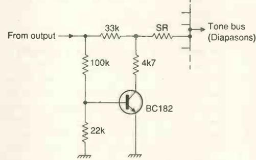
Fig. 6a) Circuit for adding second - and other - harmonics to the sine-wave.
