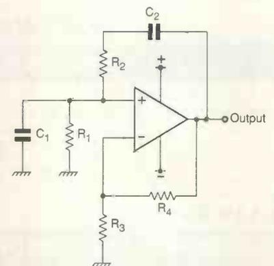
Fig. 1. One of the simplest audio oscillators or tone generators is based on the Wien bridge.
