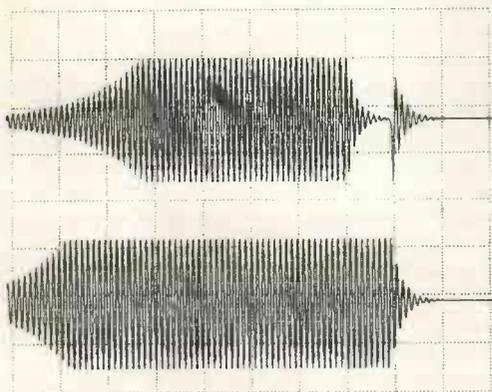
c) Delaying the removal of the semitone pitch change control signal to avoid chirp on end transient of the square-wave output when sounding the upper tone causes a hiccup in the ending transient of the upper tone sine-wave output, audible as a slight key click.
