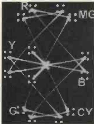
Fig. 8. Vector scope trace – subcarrier from sync generator is reference, and signal is locking input.
