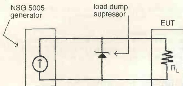
Fig. 3. Centralised load dump suppressor in the test harness to the EUT helps simulate the type of environment that the EUT might meet in an automobile.
