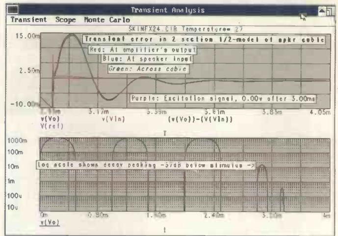
Fig. 11. Signal residue after the sinewave burst has stopped. The purple plot shows how signal across a speaker fed hypothetically without any cable immediately falls to 0V. The speaker at the end of the cable sections is not so favoured, blue. Initial error is about 1/70th of the historic peak input signal.
