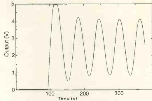
Fig. 4. Start-up characteristic of a 60s period RC cascade oscillator demonstrates extremely fast stabilisation.
