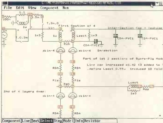
Fig. 12. In the Jenving cable, simple patented techniques prevent diodicity between strands, so each mesh section is simplified. The Skin-4 macro is the Blue (Jenving) plot in Fig. 6. One extra PVC capacitor covers increased capacitance, while  $L_{sect}$  is cut by tenfold.
