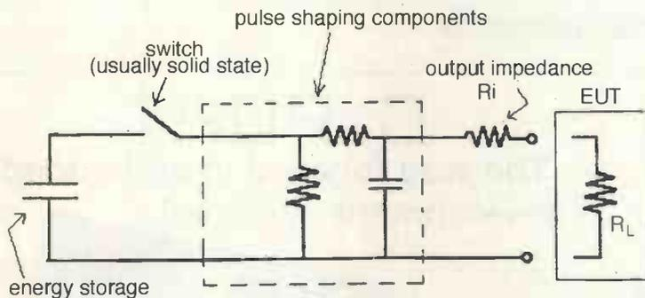
Fig. 1. Simplified block diagram of a transient generator. Both transient and burst generators typically have requirements for generating very fast rise times and short pulse widths.
