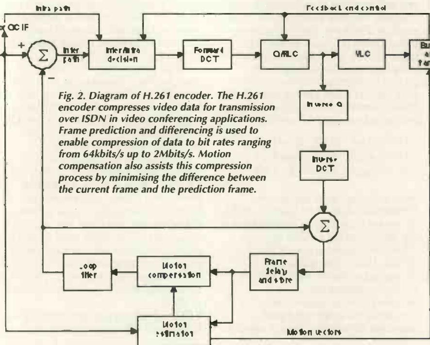
Fig. 2. Diagram of H.261 encoder. The H.261 encoder compresses video data for transmission over ISDN in video conferencing applications. Frame prediction and differencing is used to enable compression of data to bit rates ranging from 64kbits/s up to 2Mbits/s. Motion compensation also assists this compression process by minimising the difference between the current frame and the prediction frame.
