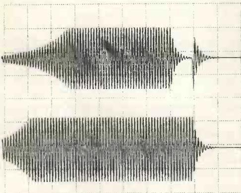
c) Delaying the removal of the semitone pitch change control signal to avoid chirp on end transient of the square-wave output when sounding the upper tone causes a hiccup in the ending transient of the upper tone sine-wave output, audible as a slight key click.
