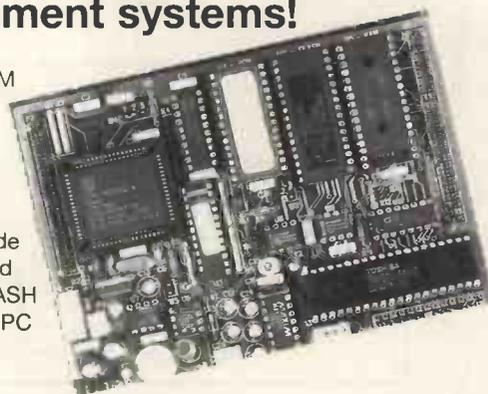
C-PORT based systems can accept in-field software upgrades from floppy - no EPROM changing.
