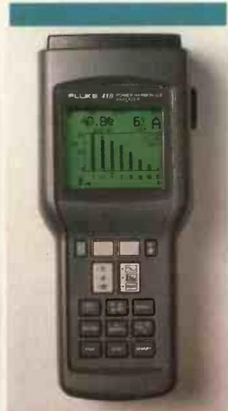
**Three-phase harmonic analysis.** Fluke's *41B Power Harmonics Analyser* is a handheld instrument measuring true rms voltage and current, frequency and power factor and displaying three-phase power. Display is as a waveform, as a bar-graph showing the level of harmonics present or as a numeric value, data being downloaded if required. PIDA. Tel. (and fax), 0756 799737.
