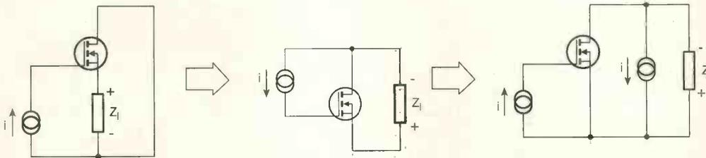
Fig. 2. By redrawing the circuit and applying a Blakesley transformation, the source follower on the left is shown to be equivalent to the common source stage with the extra current source on the right. As long as the current gain factor of the mosfet is much larger than unity, the influence of the extra current source is negligible.
