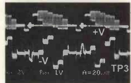
Fig. 4. Chroma, demodulated using U axis carrier.
