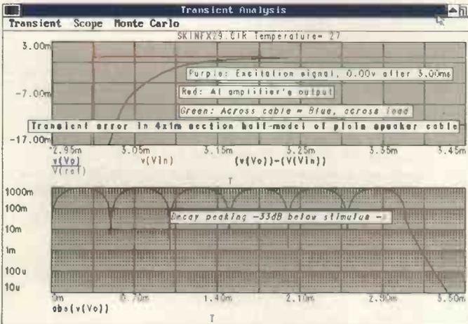
Fig. 14. Here, the plain 2.5mm cross-sectional cable model (Fig. 10) is driven into a pure 5.6Ω. Peak signal across the cable, green, is surprisingly large. It is about as large as with the speaker load (Fig. 11), but more quickly damped.
