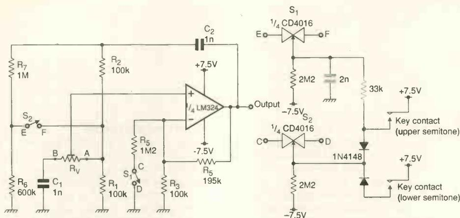
Fig. 7. Circuit Fig. 6 modified to sound either of two adjacent semitones, according to which key is pressed. Addition of both  $R_6$  and  $R_7$  keeps the loop gain the same when  $S_2$  is closed, leaving the amount of clipping at the rails the same for either semitone (see Fig. 8a).
