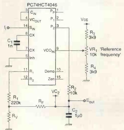
Frequency comparator provides hysteresis adjustable by resistor values.
