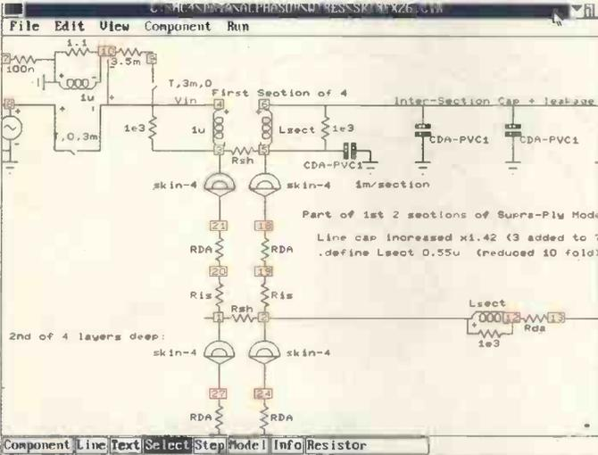
**Fig. 12.** In the Jenving cable, simple patented techniques prevent diodicity between strands, so each mesh section is simplified. The Skin-4 macro is the Blue (Jenving) plot in Fig. 6. One extra PVC capacitor covers increased capacitance, while L<sub>sect</sub> is cut by tenfold.
