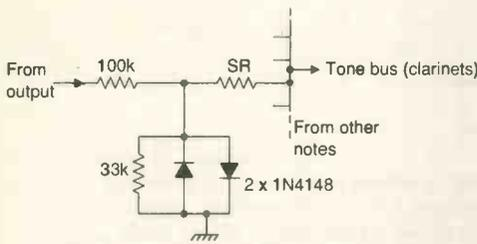
Fig. 5a) Simple clipper circuit provides an approximation to a square-wave for simulating, say, a clarinet.
