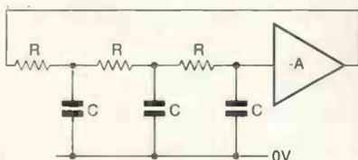
Fig. 1. In principle, the RC phase-retard cascade oscillator is similar to its CR phase-advancing counterpart.
