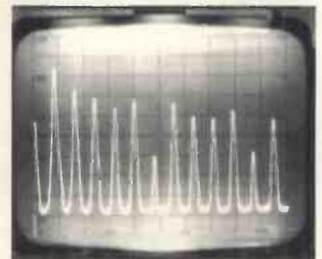
c) Showing the fundamental at about 1.7kHz, the second harmonic about 10dB down - about right for an open diapason - and many other harmonics. (10dB/division vertical, 2kHz/division horizontal, span 0-20kHz.)
