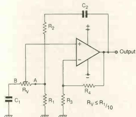
Fig. 3. Adding trimmer potentiometer R<sub>V</sub> permits tuning of the oscillator without changing the attenuation via the Wien network – provided the resistance of the pot track does not exceed a tenth of the reactance of C<sub>1</sub>. R<sub>1</sub>=R<sub>2</sub>=100k.
