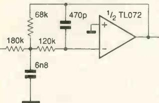
I also wrote to one of the American op-amp manufacturers, and have since heard that the explanation is thought to be the variation of input bias current with common-mode input level. I have also heard from one or two interested readers who have detected audible distortion in S&K circuit.
