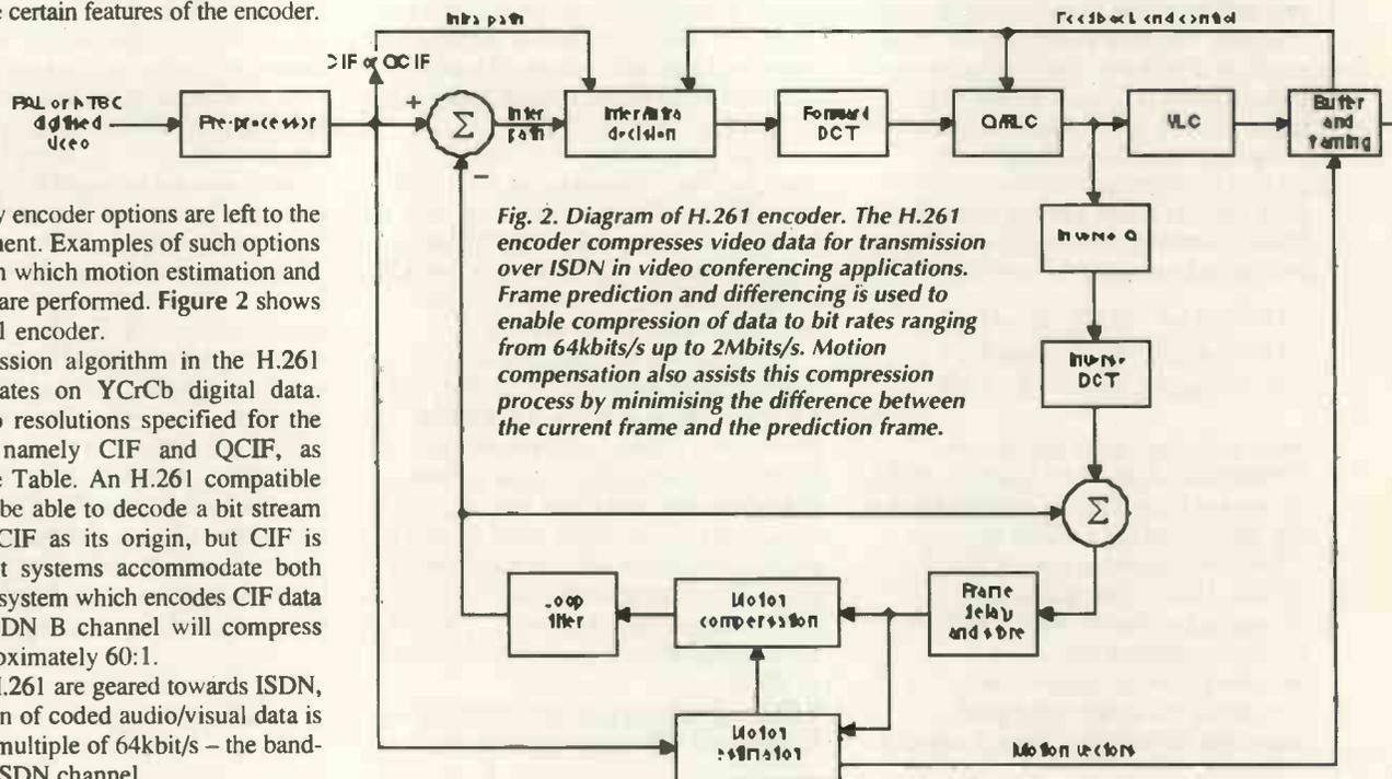
Fig. 2. Diagram of H.261 encoder. The H.261 encoder compresses video data for transmission over ISDN in video conferencing applications. Frame prediction and differencing is used to enable compression of data to bit rates ranging from 64kbits/s up to 2Mbits/s. Motion compensation also assists this compression process by minimising the difference between the current frame and the prediction frame.
