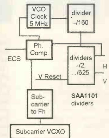
Fig. 1. Dividers within the SAA1101 allow not only separate and composite sync pulses to be generated, but also allow pulses to be generated for different tv standards.
