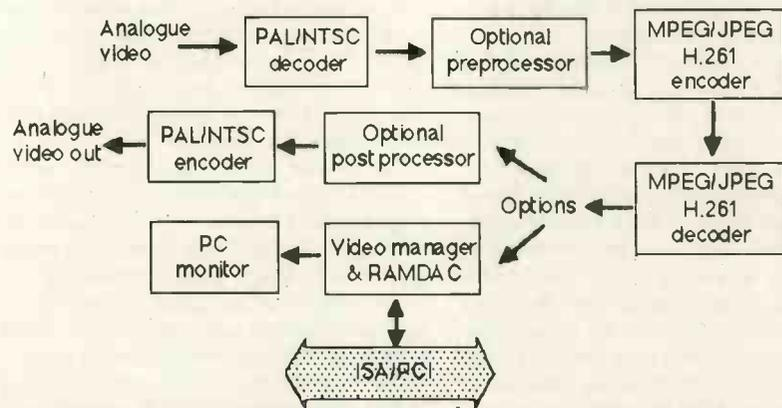
*Possible hardware requirements. A typical hardware video coding system will need to digitise analog video, and process that digital video using a JPEG, MPEG or H.261 encoder. The compressed video is then stored or transmitted. In PC based systems the decoded video will be merged with the other PC graphics for display on the monitor. In a stand-alone system, however, the output may be a PAL signal for display on a composite monitor.*
