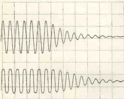
c) Due to the limiting action of the diodes, the ending transient of the square-wave output is extended compared to that of the sine-wave.
