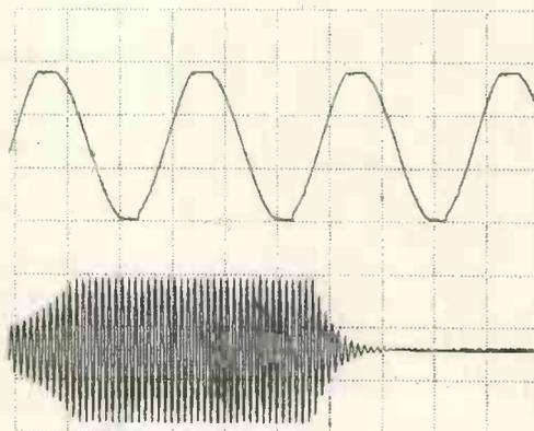
b) Output waveform is basically sinusoidal, suitable for use directly for stops of the flute family, upper trace. Begin and end transients are smooth and free from any incidental dc shift, lower trace.
