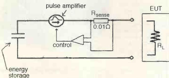
Fig. 2. Simplified schematic of the NSG 5005 operating in current mode. An in-line sense resistor develops a feedback voltage to control the pulse amplifier.
