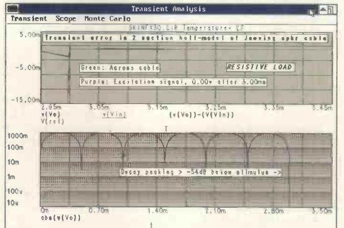
Fig. 15. Model of Jenving's Supra Ply cable correctly predicts an approximately 20dB lower peak perturbation (-54dB arrowed, lower, where the decay angle changes). The upper plot shows that after 3.00ms, amplifier output error is of the same order or likely dominant.
