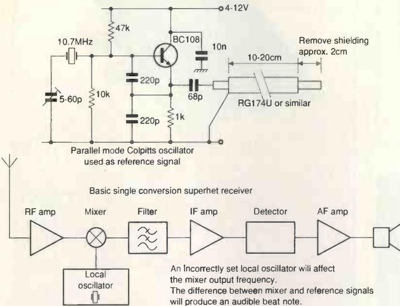
Beat oscillator helps to retune crystal-based receivers to different channels.
