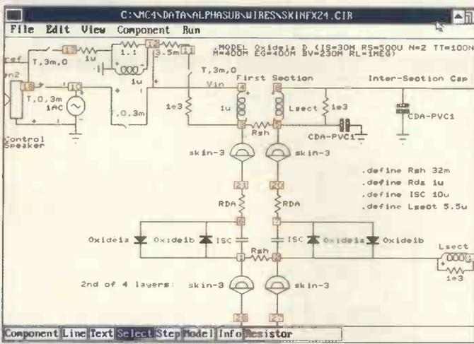
Fig. 10. Realistic speaker cable modelling begins with the mesh of R,L, PVC cap macros, oxide diodes and skin effect macros seen here. The Y axis is concentric depth, so the lowest layer, not visible here, represents the innermost strand. At the top left, a second speaker macro is arranged as a control. It receives the same test signal but free of cable.
