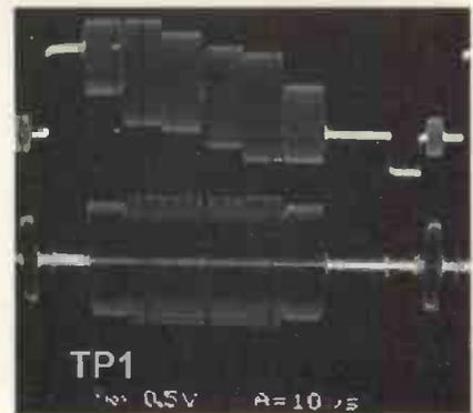
Fig. 3. Limited chroma. In this design, chroma in the active line is not so important, but a constant-amplitude burst is useful.
