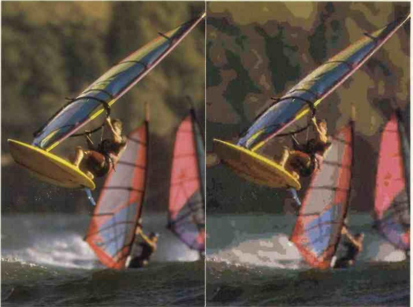
*File size of the JPEG original on the left is 1215Kbyte while that of the version on the right, compressed with loss, is only 61Kbyte.*
