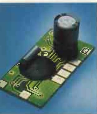
Plugging a radio-code receiver into your PC's COM port and running the dos and windows software supplied gives you access to the atomic-clock referenced 60kHz time signal transmitted from Rugby. This signal is accurate to a second in a million years and corrected automatically for summer/winter time.
