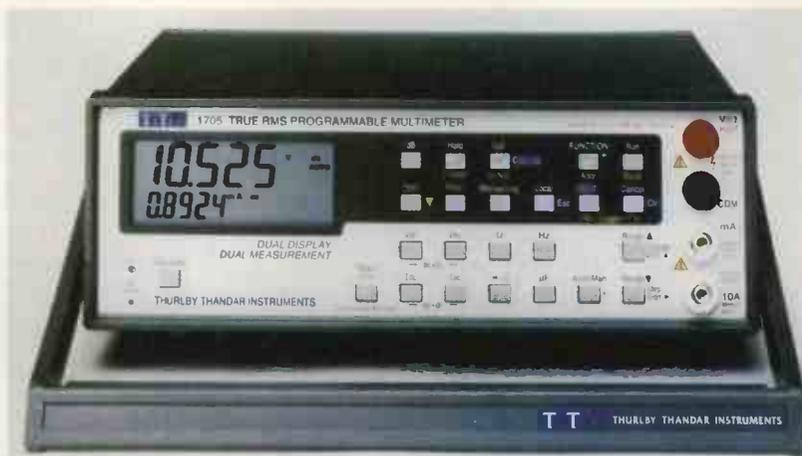
This high-performance bench multimeter could be yours in exchange for a good idea. Featuring a dual display, the 4.5-digit 1705 multimeter resolves down to 10µV, 10mΩ and 0.1µA and has a basic dc accuracy of 0.04%. Frequency measured is 10Hz to 120kHz with an accuracy of 0.01% and resolution to 0.01Hz. Capacitor and true rms measurements are also featured.
