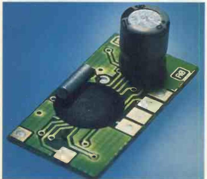
Typical MSF receiver module with a footprint of only 7 by 24mm.
