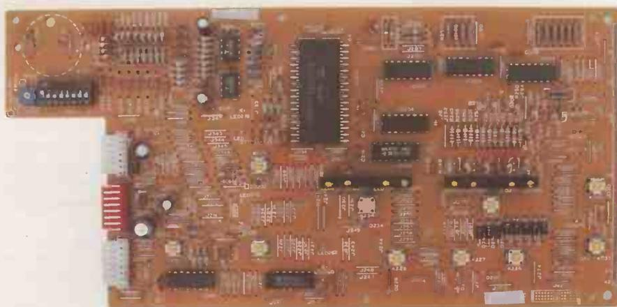
Fig. 2. Microprocessor-based dc controller of Japanese manufacture illustrates that it may wise to consider single-sided designs even for fairly complex
