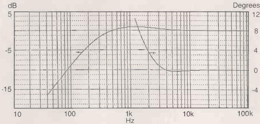
Fig. 5. Bode plot for the circuit of Fig. 4, where all Cs are 1nF and all Rs=100kΩ. Gain peaks at +0.9dB at 1.2kHz, but is still in excess of unity at the zero phase-shift frequency of 3.9kHz.
