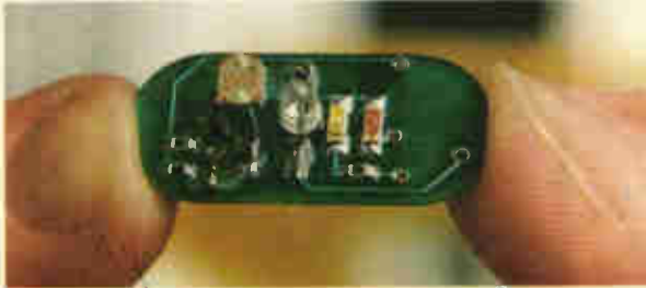
Active eyes... Shown is the circuit board from the cats' eyes alternative.
