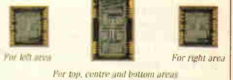
Fig. 4. The typical optical metering configuration of the Canon EOS-1N. Above the eyepiece and taking light from the pentaprism is the silicon photocell (SPC) exposure meter. In the base of the mirror box are the TTL flash metering SPC and the Multi-Basis (base stored image sensor) for autofocus - both taking light reflected by the sub-mirror.
