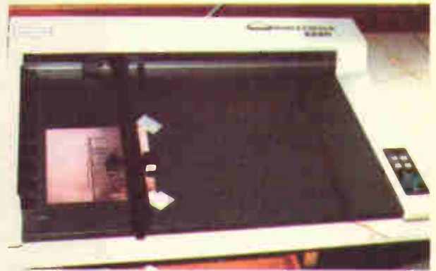
Plotting with a 0.3mm pen directly on to 0.35mm copper board. Note that the board is clamped on the left-hand side and held flat on the right using masking tape – not the usual magnetic strip.
