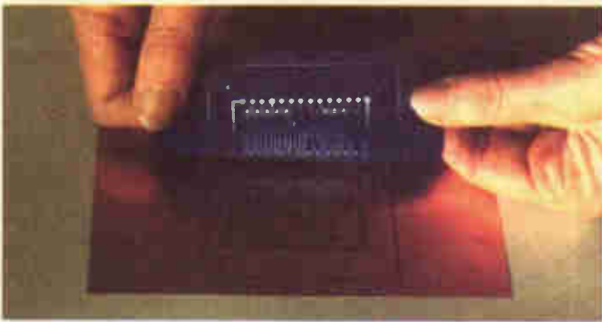
After being passed through a pouch laminator, the PnP sandwich is peeled off by hand.
