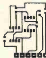
Fig. 2. Actual size of a surface-mount board showing that plotters are capable of fine detail.
