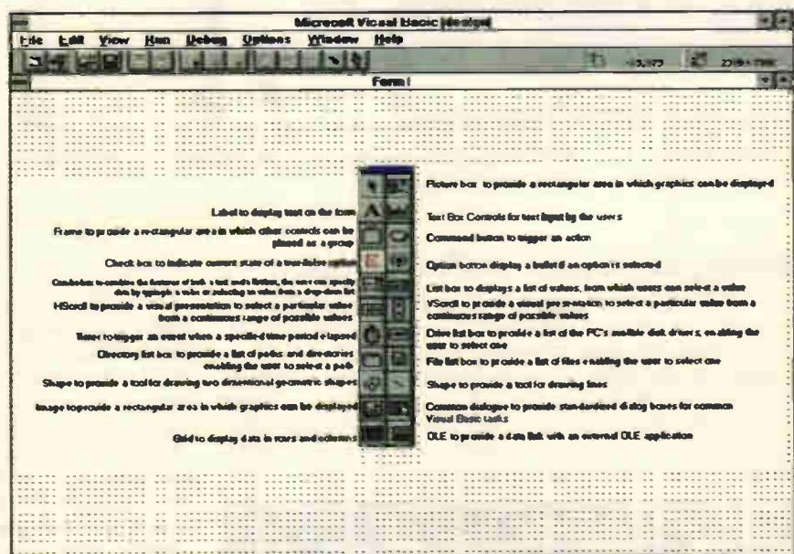
Fig. 1. Part of the task of writing a Visual Basic program involves selecting tools from the tool box and placing them on a 'Form'.
