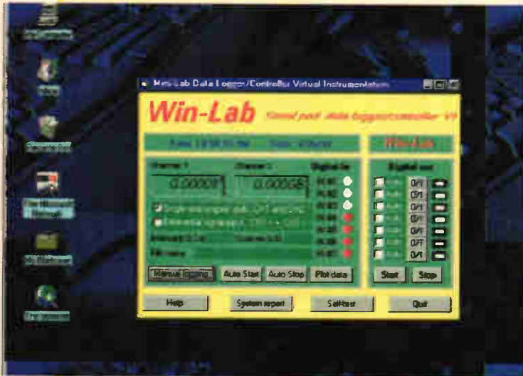
Fig. 3. Shot of virtual instrumentation display produced using software developed by the author for controlling the interface.
