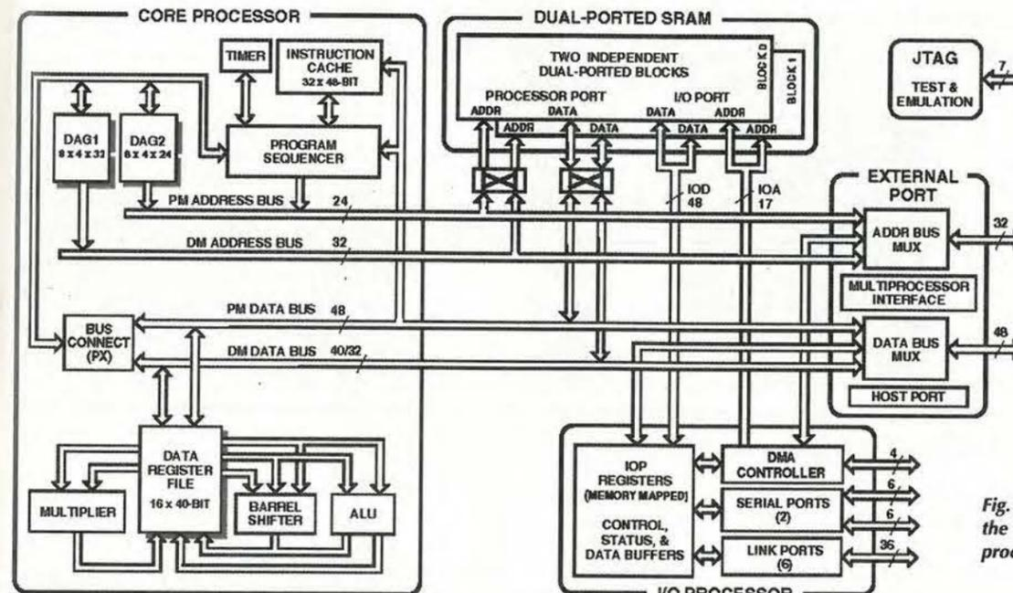
Fig. 4. Block diagram of the 'Sharc' 240 pin signal processor.
