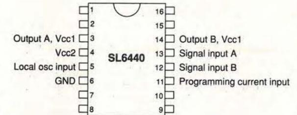
Fig. 6. Around since 1980, the SL6440 still has its uses. A drawback though is that it needs quite a few external components.
