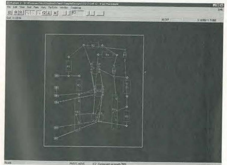
Fig. 2. Rat's nest produced from the test circuit.
