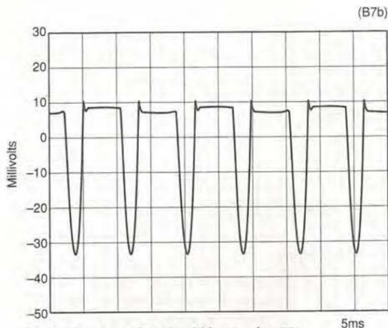
Fig. 2. Charging pulses should be equal at TP2.
