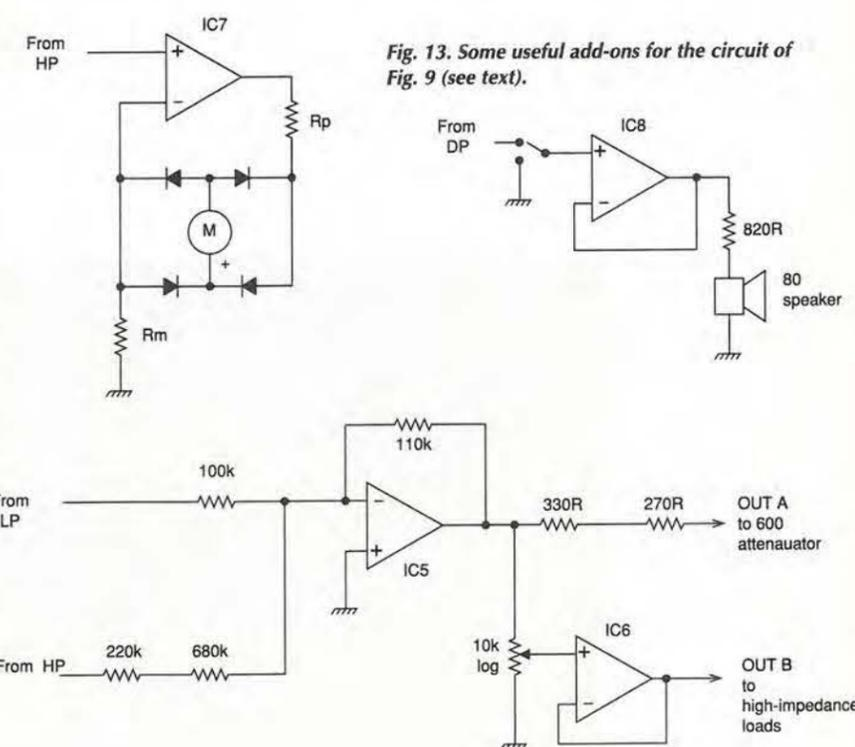
Fig. 13. Some useful add-ons for the circuit of Fig. 9 (see text).
