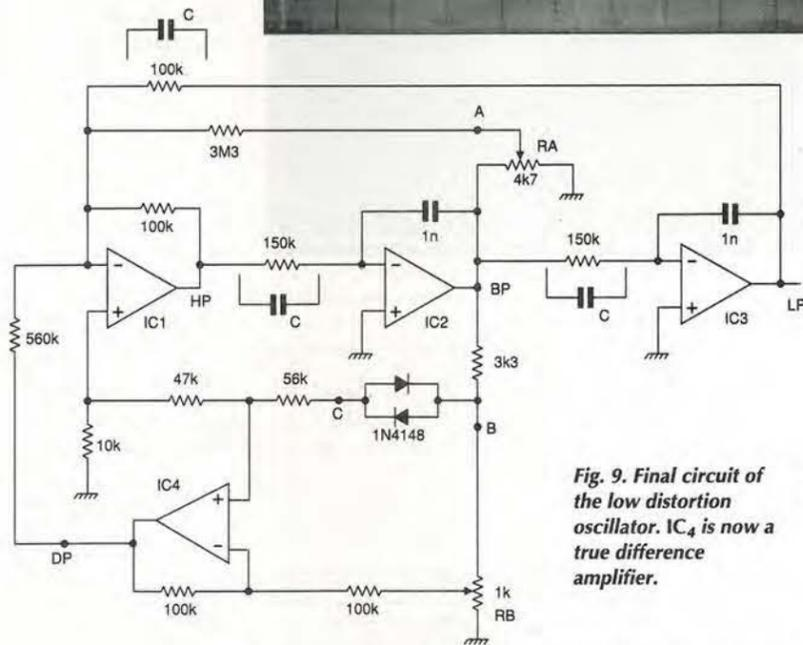
Fig. 9. Final circuit of the low distortion oscillator.  $IC_4$  is now a true difference amplifier.
