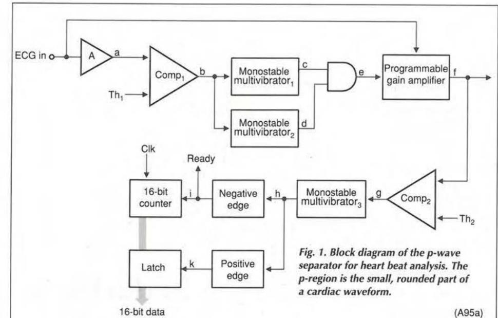
Fig. 1. Block diagram of the p-wave separator for heart beat analysis. The p-region is the small, rounded part of a cardiac waveform.
