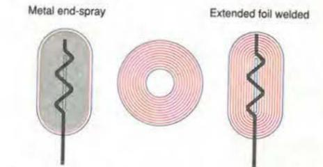
Fig. 4. Winding on a larger diameter mandrel allows the roll to be flattened to form the capacitor element. Both metallised and extended-foil electrode capacitors can take advantage of sprayed-metal end connections. Foil electrodes that extend beyond the dielectric roll allow resistance welded, directly attached lead wires. In the centre is the wound capacitor before compression.
