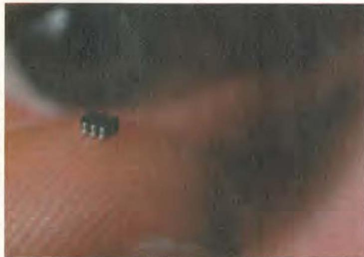
A quarter of a century after its introduction, the company has redesigned the LM300 family of op-amps using a relatively advanced 0.8µm BiCMOS manufacturing process. For designers of modern equipment, the most important outcome is that supply voltage now ranges from 2.7 to 5.5V. Other
