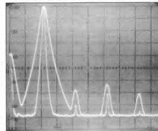
Fig. 2. Upper trace, output of the circuit of Fig. 1. Span 0-5kHz, 100Hz resolution (IF) bandwidth, video (post detection) filter off. Lower trace, as above, but with component values in brackets, resolution bandwidth 30Hz.
