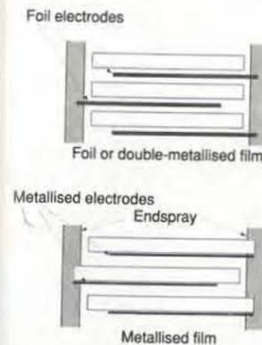
Fig. 1. Having no discrete electrodes, the metallised film capacitor maximises capacitance and voltage for a given size, but has limited current handling. Use of foil electrodes maximises current handling but reduces capacitance. Double metallised film electrodes, described in a German Patent, offer intermediate capacitance and current handling.
