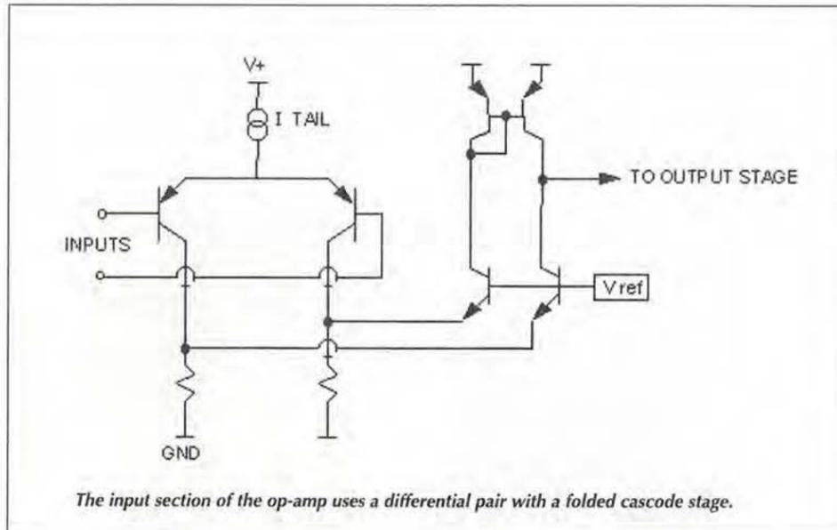
The input section of the op-amp uses a differential pair with a folded cascode stage.
