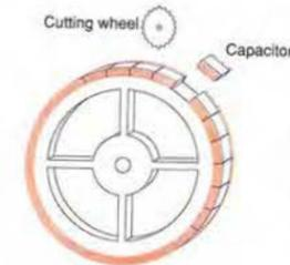
Fig. 3. Stacked film production technology. Large rings of metallised film, of width equal to the final capacitor body length, are wound on 'core' wheels. These rings are metal end sprayed, then sliced to make individual capacitors.
