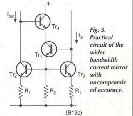
Fig. 3. Practical circuit of the wider bandwidth current mirror with uncompromised accuracy.
