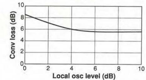
Fig. 10. Typical diode-mixer conversion loss versus local-oscillator level.
