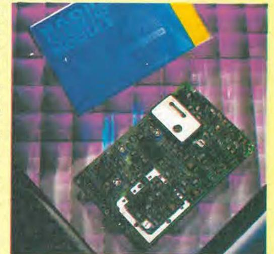
The main feature of this telemetry receiver is that it provides programmable operating frequency with the performance of a fixed-frequency crystal alternative. It includes an fsk data extractor and has either modem or controller options. Operating frequency is 450 to 470MHz, programmable either by replacing the PIC microcontroller or by downloading serial data from a pc.
