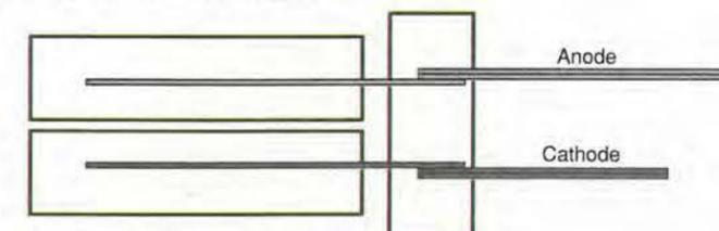
Fig. 5. Sectional view of typical small radial capacitor showing centre foil tab connections, minimising self inductance, which is typically much less than 20nH.
