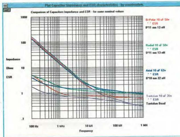
Fig. 7. As measured, plots of impedance and esr for bi-polar radial, polar radial, polar axial and bead tantalum 10µF capacitors. Shows the Panasonic bi-polar performs best of aluminium variants, but all types have near 45° phase by 10kHz and deteriorating performance from as low as 1kHz.
