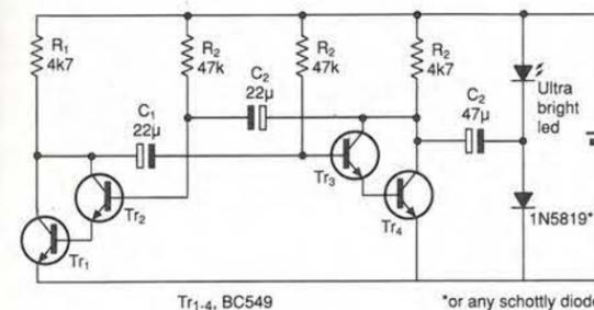
Comprising a multivibrator followed by a voltage doubler, this led flasher should run for up to a year on one alkaline AA cell.
