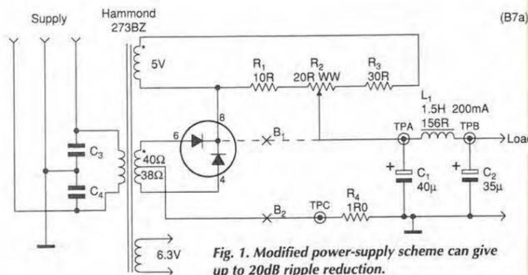
Fig. 1. Modified power-supply scheme can give up to 20dB ripple reduction.
