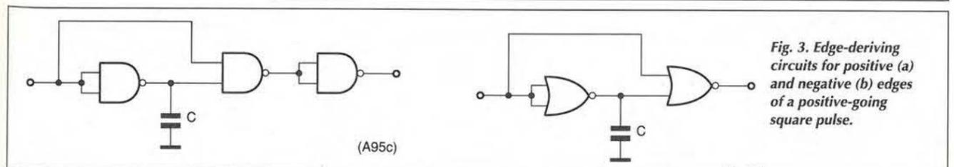
Fig. 3. Edge-deriving circuits for positive (a) and negative (b) edges of a positive-going square pulse.
