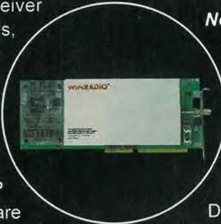
WiNRADiO™ provides a complete communications system on a full-length ISA PC Card, with software for Windows 3, NT or 95.
