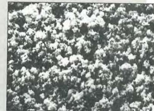
Fig. 14. Large magnification electron microscope view of the surface of a very high 'gain', low-voltage anode foil. Etching and forming methods are optimised for low voltage capacitor use.
