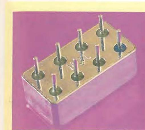
SBL-1 diode mixer from Mini-Circuits. Although not an active device, this mixer produces good results in a wide range of receiver applications.
