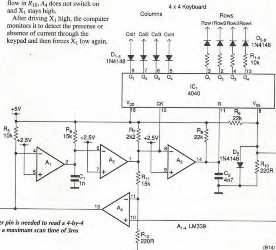
Only a single input/output microcomputer pin is needed to read a 4-by-4 keypad (or up to 6-by-6, if required) with a maximum scan time of 3ms (42ms for 6-by-6).
