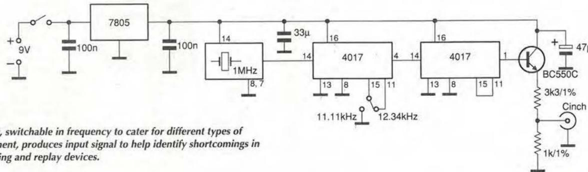
Simple circuit, switchable in frequency to cater for different types of digital equipment, produces input signal to help identify shortcomings in digital recording and replay devices.
