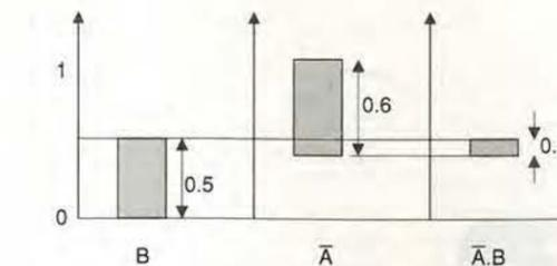
Fig. 9. An operation using the complement function.
