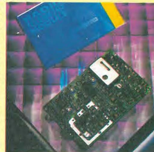
The main feature of this telemetry receiver is that it provides programmable operating frequency with the performance of a fixed-frequency crystal alternative. It includes an fsk data extractor and has either modem or controller options. Operating frequency is 450 to 470MHz, programmable either by replacing the PIC microcontroller or by downloading serial data from a pc.
