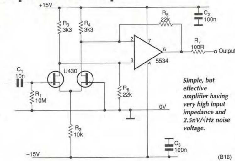
Simple, but effective amplifier having very high input impedance and 2.5nV/√Hz noise voltage.
