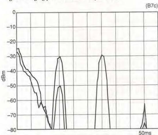
Fig. 3. 20dB improvement in power supply ripple after adjustment of R<sub>2</sub>.
