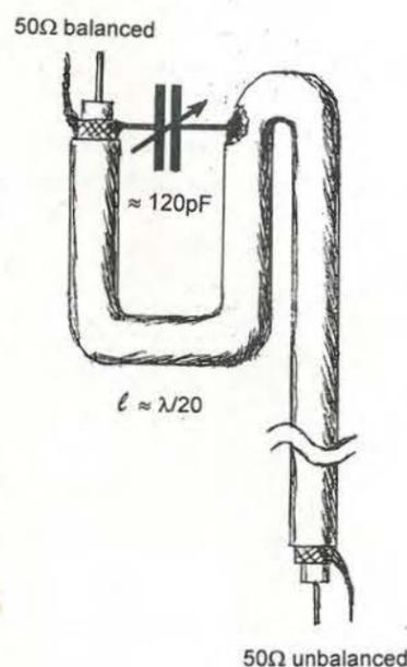
Fig. 7. Variable balancing unit. The capacitor is part of a tuned circuit where a length of the coaxial cable, typically around  $\lambda/20$  corresponding to a length of 0.55m in the citizens' band, represents the inductance. There is little improvement with respect to a standard balun and its best use could be as a variable splitter. The capacitance, measured at 120pF, could be substituted by a silvered mica capacitor once its exact value is known.
