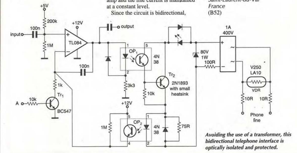
Avoiding the use of a transformer, this bidirectional telephone interface is optically isolated and protected.
