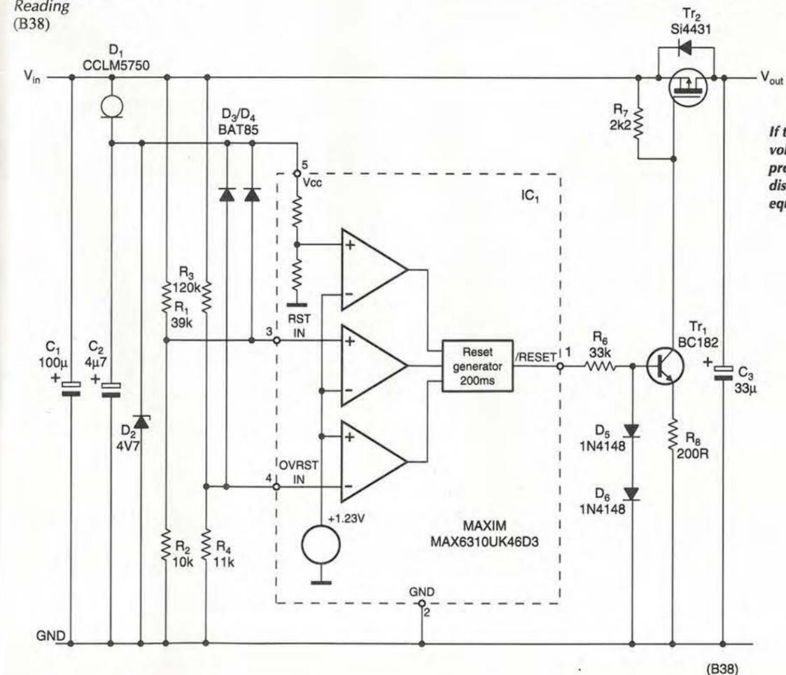
If the power supply voltage is under or over preset limits, it is disconnected from the equipment within 20µs.
