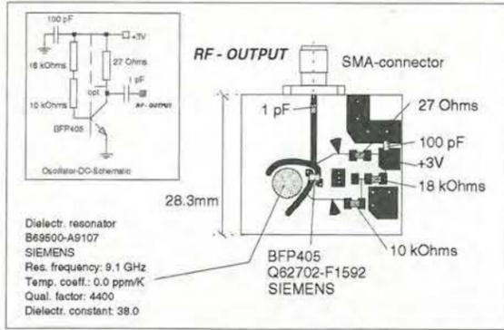
Fig. 4. Usable at frequencies to 12GHz, this Siemens laboratory prototype was built on 0.38mm thick PTFE board.
