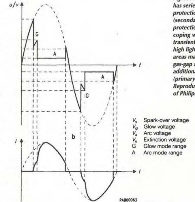
Fig. 10. Showing a) the voltage across and b) the current through a gas-filled surge arrester versus time, and c) the V/I characteristic of the arrester. Reproduced courtesy of Siemens.
