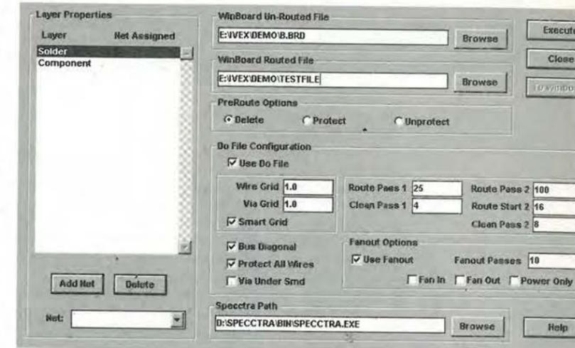
To reach this stage, the interactively-sorted rat's nest should be saved as a file in WinBoard, and this file loaded in the 'placed file' box in the interface menu. A file for the completed board must also be placed in the 'routed file' box in order that the Spectra results can be transferred to it after auto-routing has finished.
