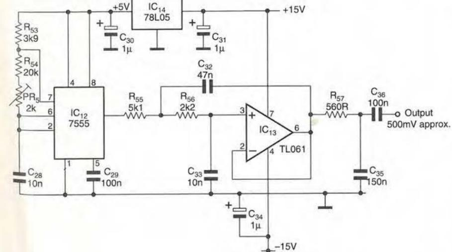
Fig. 6. 3150Hz reference oscillator. A divided-down crystal reference is often used here, but this circuit was found to give adequate stability, as you will see from Table 2. The circuitry conditioning the 555 output turns the rectangular wave into a sinusoidal one.
