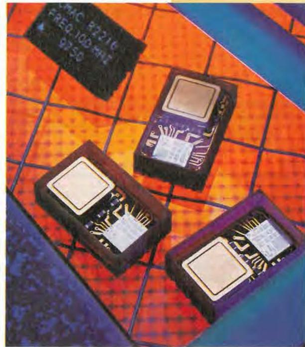
isolation voltage, high current transfer, high-speed switching and the option of multiple packages. The range is contained in TO-5, TO-18 and 8-pin and 16-pin dips in a variety of mounting choices, operating temperature being -65°C to 125°C. Faraday screening in the multiple units avoids common-mode interference and assists with radiation performance.
