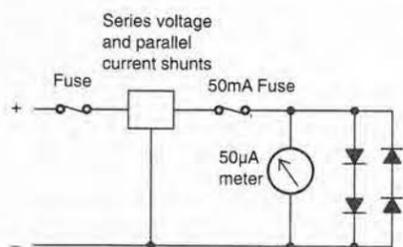
Fig. 6. A 50µA meter can be protected by a 50mA fuse, with the aid of some diodes.
