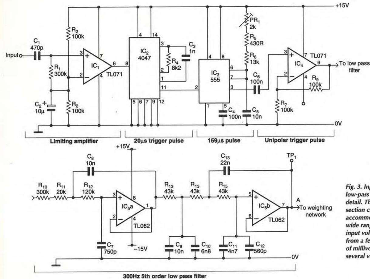
Fig. 3. Input and low-pass filter detail. This section can accommodate a wide range of input voltages from a few tens of millivolts to several volts.
