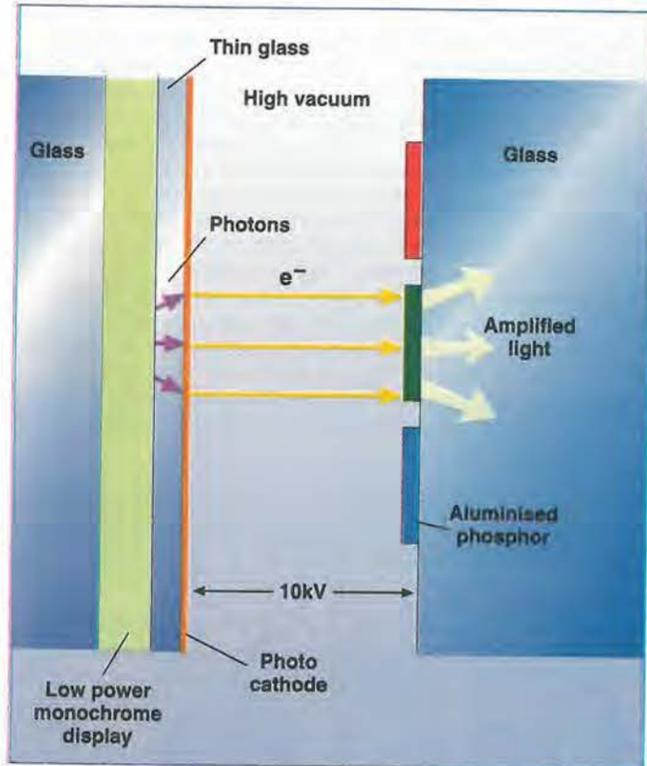
In a night-sight image intensifier, light impinging on the cathode causes localised electron emission. In this new technology, the photocathode is activated by a low power electroluminescent, or similar, display. Note the similarities between the photocathode display and a conventional cathode-ray tube.
