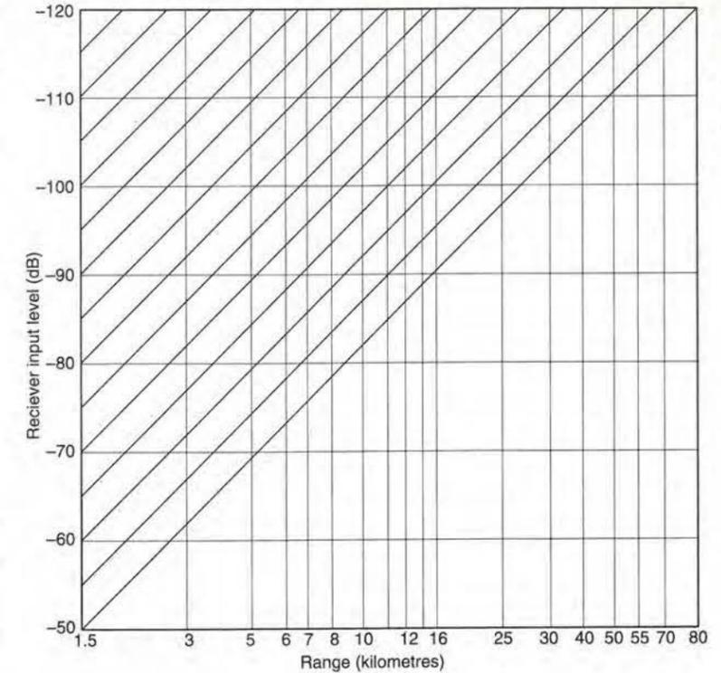
This chart is for finding the required receiver sensitivity at any distance from the transmitter.
