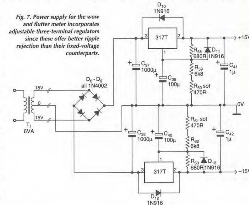
**Fig. 7. Power supply for the wow and flutter meter incorporates adjustable three-terminal regulators since these offer better ripple rejection than their fixed-voltage counterparts.**
