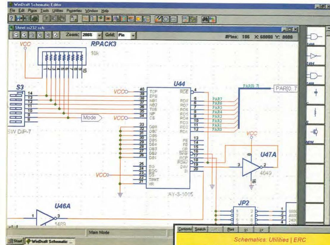
Fig. 1. View of WinDraft schematic drawing. Note the symbol palette on the right, which can be turned off to increase screen area.
