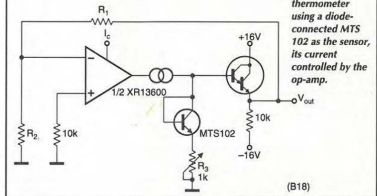
Wide-range thermometer using a diode-connected MTS 102 as the sensor, its current controlled by the op-amp.
