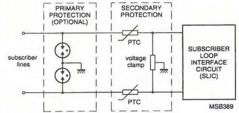
Fig. 9. A SLIC usually has series and shunt protection (secondary protection) for coping with normal transients, and in high lightning risk areas may also have gas-gap arresters for additional protection (primary protection). Reproduced courtesy of Philips.
