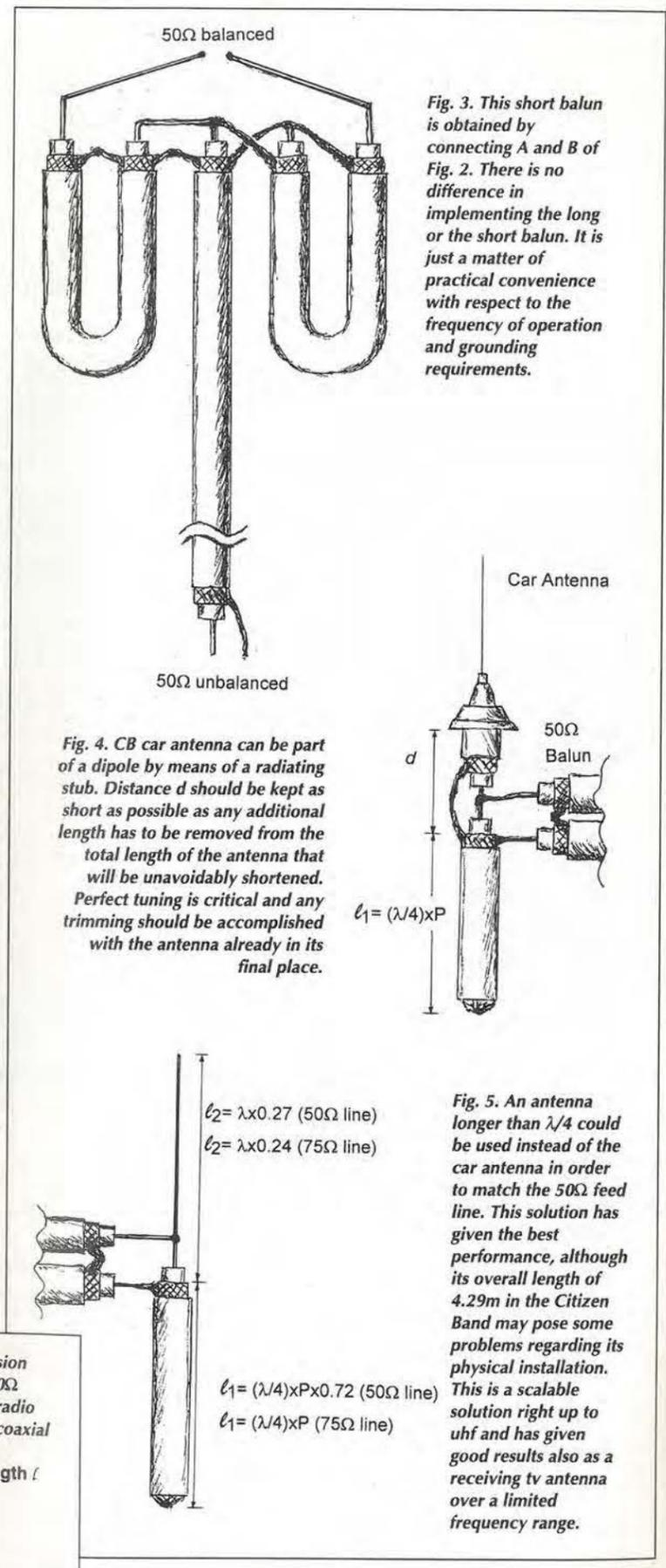
It is worth mentioning that points A and B are at the same potential so they can be connected together thus getting a more compact balun, Fig. 3. Eventually the complete antenna was wired as in Fig. 4.
