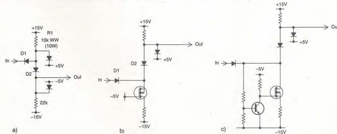
Fig. 8a). Given suitably rated diodes, this frequency-counter input-stage provides protection up to 316V dc, 612V rms continuous, 1kV rms short term. b) Substituting a mosfet constant-current generator for R<sub>1</sub> greatly reduces the maximum dissipation... c) ...which can be reduced further still if the mosfet drain current is shut down beyond some positive-going limit.
