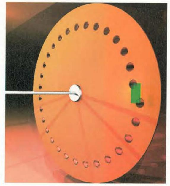
**Fig. 2. A single spiral 30-line Nipkow lens disc set up for the Baird standard. The area for imaging or display is shown in green. For a 1.5m diameter disc, this area is only about 6cm horizontal by 14cm vertical.**
