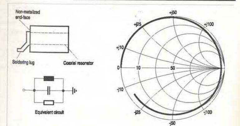
Fig. 3. Sectional view and equivalent circuit for a ceramic coaxial resonator. The Smith chart clearly shows this particular device's 2.4GHz self-resonant frequency.
