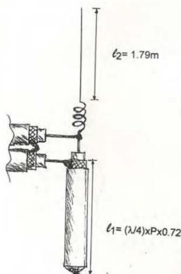
Fig. 6. A shorter antenna is feasible if a coil is added near the dipole feed point. 17 turns of insulated 2mm wire are closely wound on a 17mm form. The total length is now only 3.19m at  $f=27.185\text{MHz}$ .
