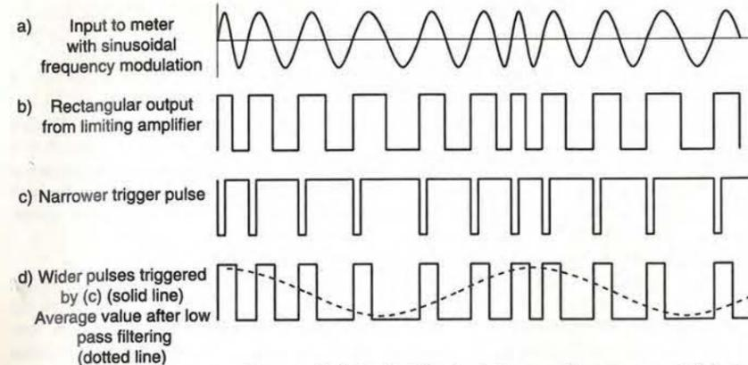
Fig. 2. Wow and flutter cause the recorded signal at the top to become frequency modulated. Demodulating allows the wow and flutter content to be separated and quantified.
