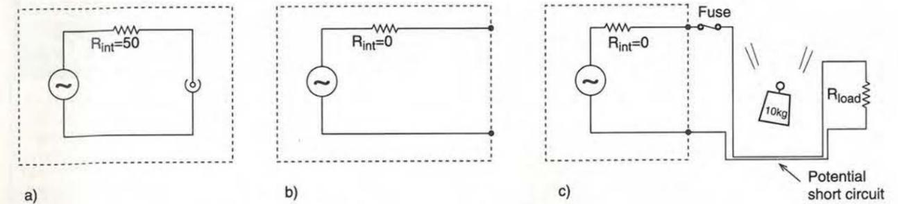
Fig. 1a). An rf signal generator typically has a source resistance (internal resistance) of 50Ω. b) An ideal constant voltage generator has an internal resistance of zero. c) Consequently, if its output is short circuited, a very large fault current will flow, unless fuse protection is provided.
