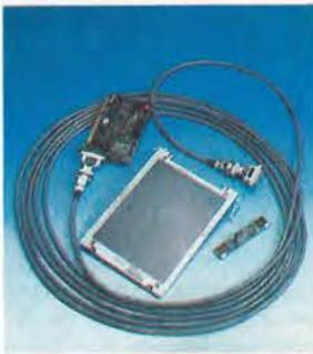
Trident Microsystems' new LVDS system, provides the cabling solution to overcome all the problems associated with driving Digital TFT over long distances.
