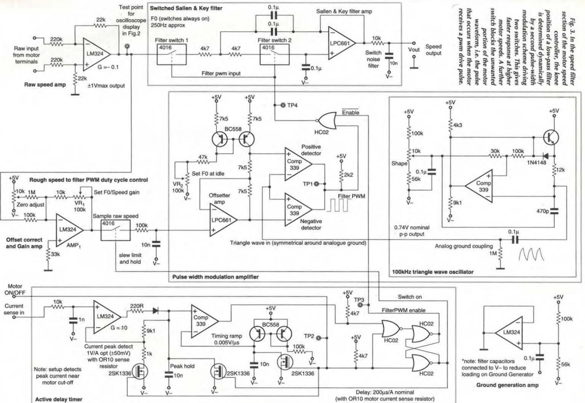
Fig. 3. In the speed filter section of the motor speed controller, the knee position of a low-pass filter is determined dynamically by a second pulse-width modulation scheme driving two switches. This gives faster response at higher motor speeds. A further switch blocks the unwanted portion of the motor waveform, i.e. the pulse that occurs when the motor receives a pwm drive pulse.
