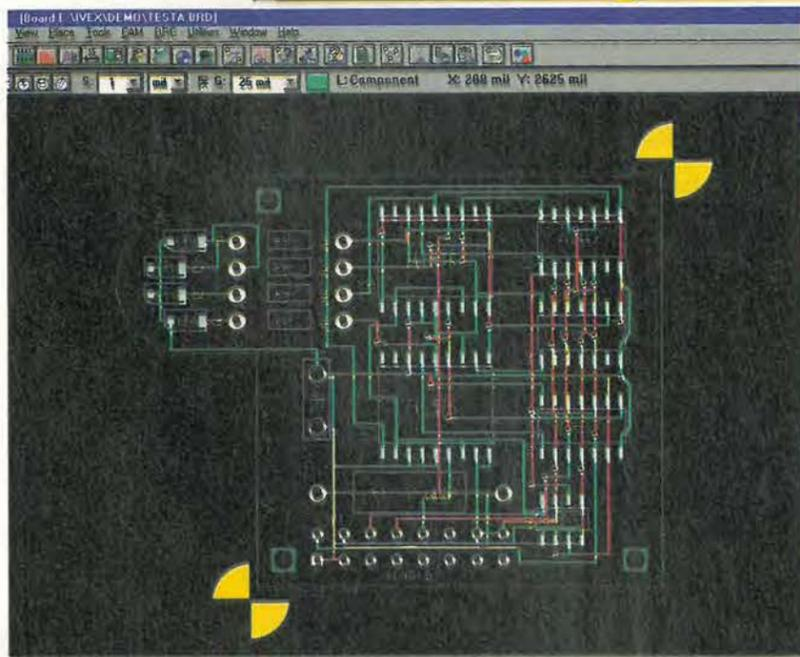
Fig. 4. The rat's nest of Fig. 3 autorouted in Spectra and returned to WinBoard format. Note the non-mitred corners. See the text for an explanation of this.
