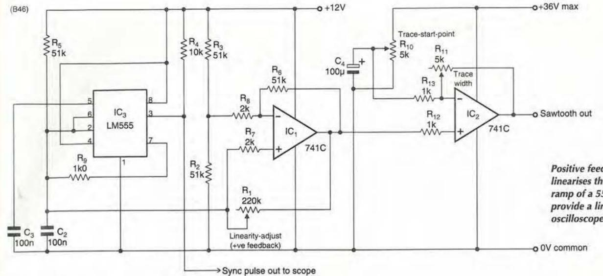
Positive feedback linearises the output ramp of a 555 to provide a linear oscilloscope trace.
