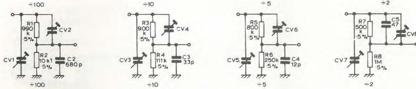
Fig. 7. Due to the high values of the resistances involved, the input attenuator of an oscilloscope is robust against overvoltages. The first stage fet is similarly protected. (Reproduced from ref. 3)
