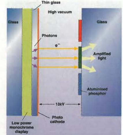
This new display technology produces crt brightness and viewing angle without the bulk. **Steve Bush** explains how on page 775.
