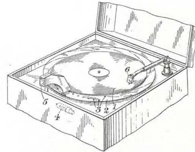
Fig. 7. Baird's patent for the 'Phonovisor'. A Nipkow disc under the record platter provides what must be the cheapest and simplest video replay device ever designed. The Phonovisor required the specially prepared Phonovision discs to be recorded synchronously with the camera disc. Looking into the viewport, the picture would be seen perfectly stable, independent of playback speed.
