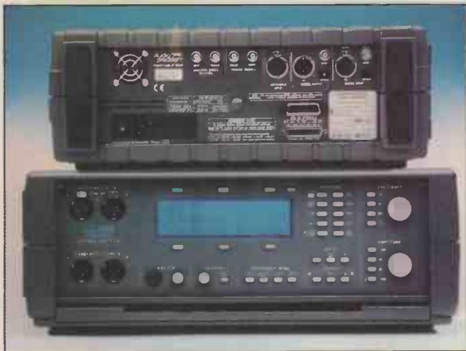
**Audio analyser interface.** As an option for the Audio Precision Portable One range of audio analysers, Thurby Thandar can now supply a GPIB interface for both versions of the instrument. The interface controls all the operation of the instruments including the recently introduced digital audio measurement in the dual-domain version for which Visual Basic sample source-code programs are supplied. The interface is also available as an upgrade.
