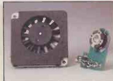
'Thinnest' fan. Sunon's GB0535ACB blower measures 35 by 35 by 4.8mm. It is claimed to be the world's thinnest, yet produces a static pressure of 0.28in of water. Its aluminium housing allows it to be attached directly to the hot component without a baffle and also acts as a heat sink itself. The fan uses only 0.5W and, at an airflow of 0.67cf/min and 0.91cf/min, there is little noise.
