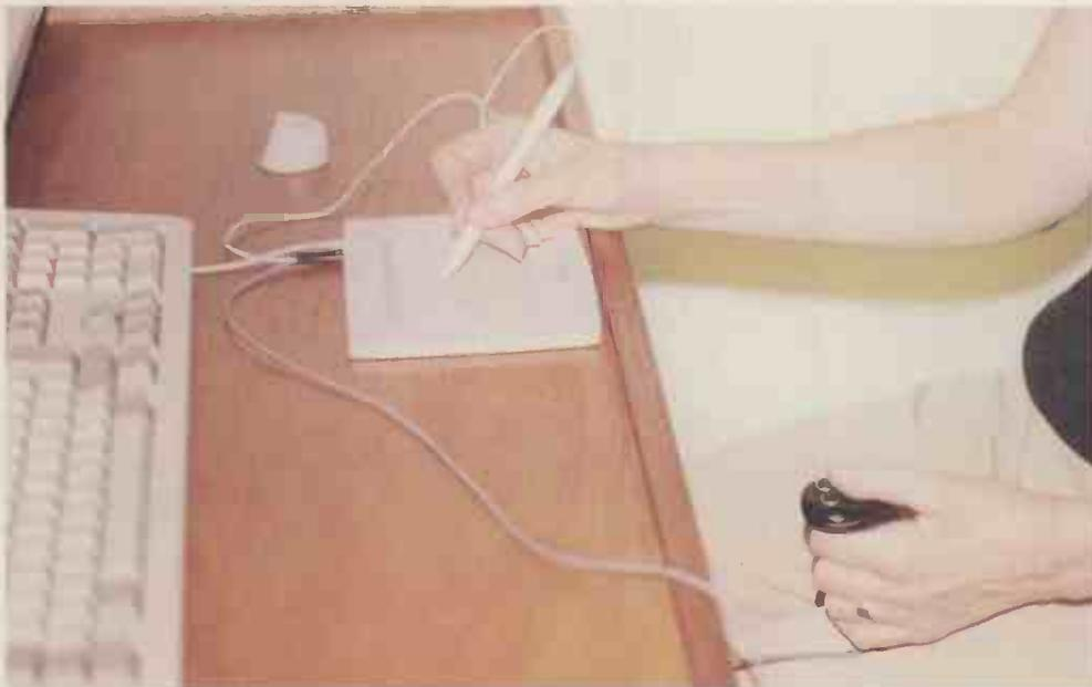
**Increased productivity.** As mentioned in last month's article, I experimented by replacing the two push buttons on a graphics tablet pen with a pistol grip designed to be used in the left hand, as shown. This made using the tablet much easier and faster.
