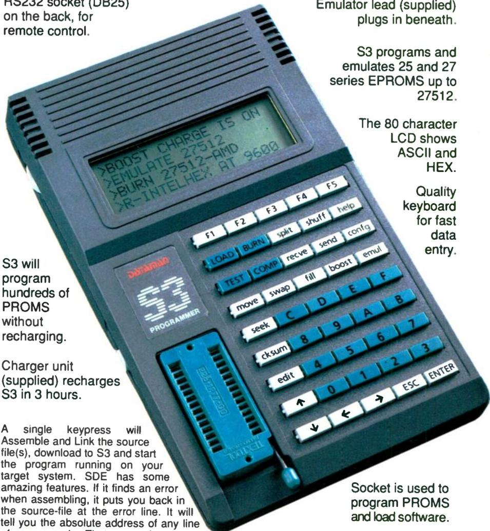
Socket is used to program PROMS and load software.
