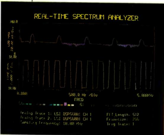
Fig. 7. Displays from spectrum analyser and oscilloscope can be combined in one frame.
