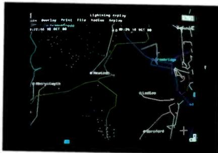
Pictures above are of lightning strikes in Wales, showing programmable overlays – in this case the 400kV overhead power lines in blue, 275kV in red and 132kV in white. Lower picture of central Wales shows Electricity Board boundaries in green.
