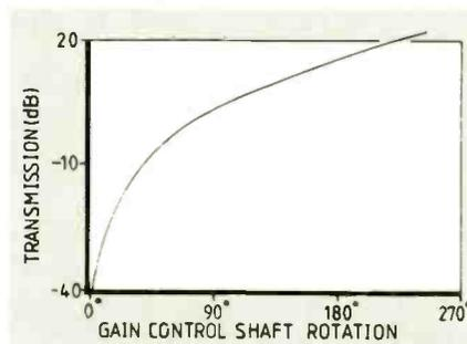
Fig. 5. Characteristic of circuit of Fig. 5, using linear potentiometers.
