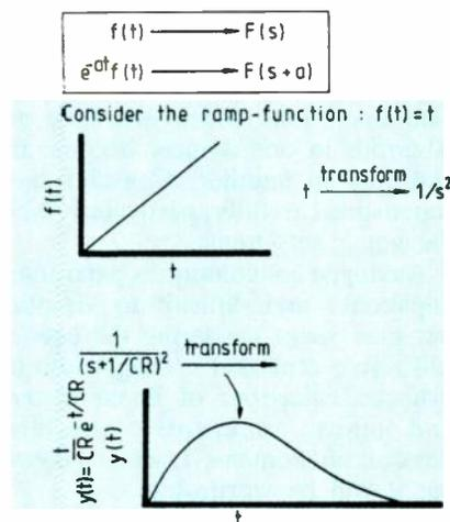
Fig. 4.4 To obtain the time-domain response, use the frequency shifting rule with a table of transform pairs.
