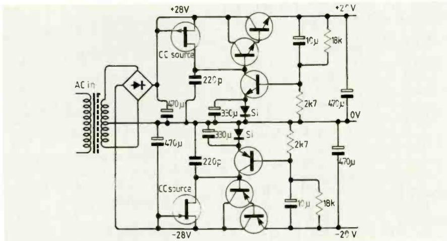
Fig 15. Discrete-component stabilised PSU for Pioneer preamplifier (similar type used by Marantz).
