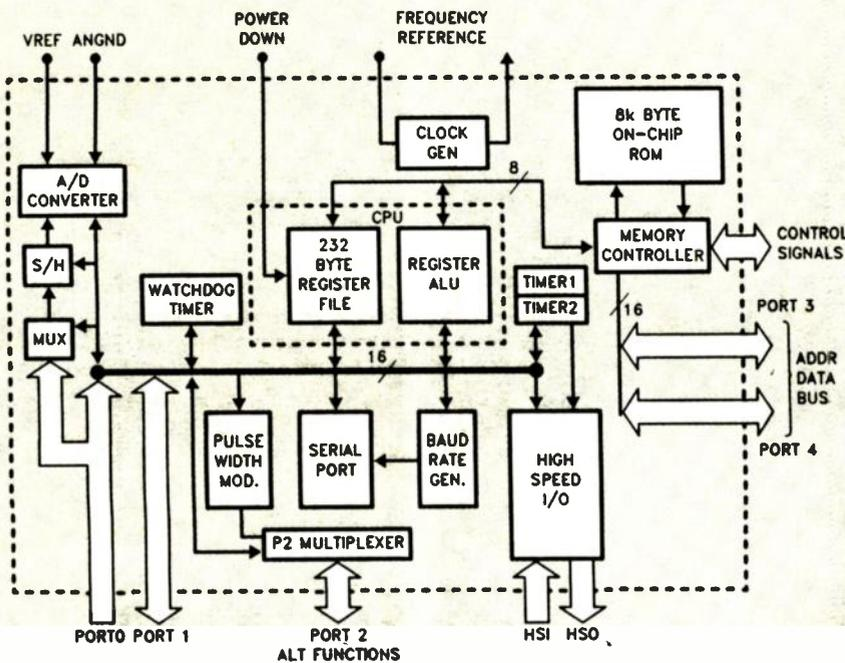
Block diagram of Intel's MCS-96 family, intended for high-speed control.
