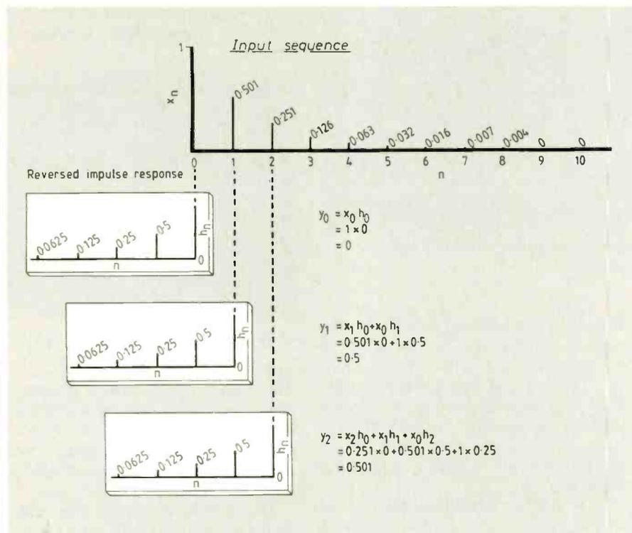
Fig. 4.9. Graphical convolution of the input signal  $x(n)$  and the impulse response  $h(n)$  is achieved by reversing the impulse response under the sample of current interest.
