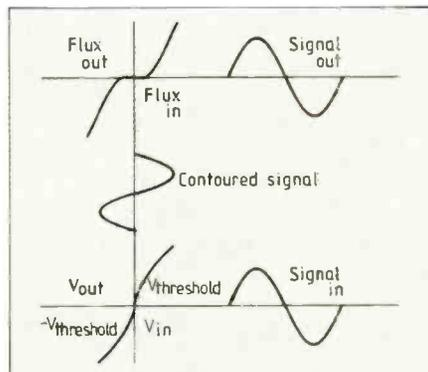
mechanisms which must be dealt with. The first is caused by the fact that the line of recording sweeps backward and forward across the head gap. This causes the rising edges of a sine wave signal to be expanded, while the falling edges are compressed. The remedy is an anti-Doppler correction – adding harmonic energy on the increasing cycles, and subtracting it on the falling edges.
