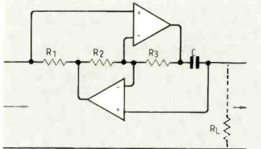
Fig. 3. Gyrator due to Riordan, after Antoniou, which forms the basis for the present design.
