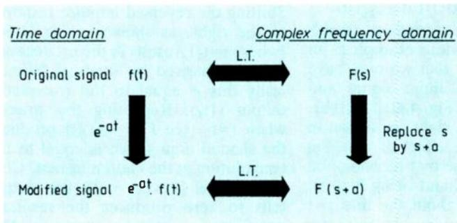
Fig. 4.3. Frequency shifting rule.
