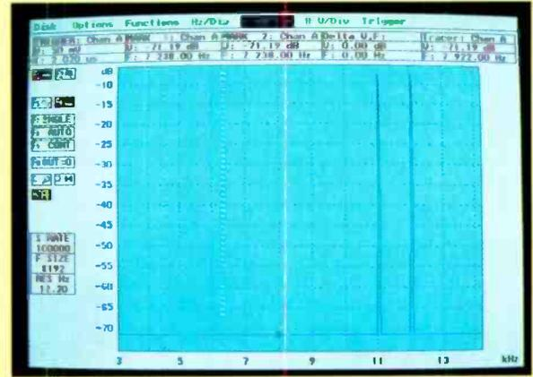
Oscilloscope display of 11kHz and 12kHz sine waves added (top left). Options menu shown pulled down. Sample rate 100kHz. Display at top right shows volts/div menu pulled down and 200mV selected, that at
