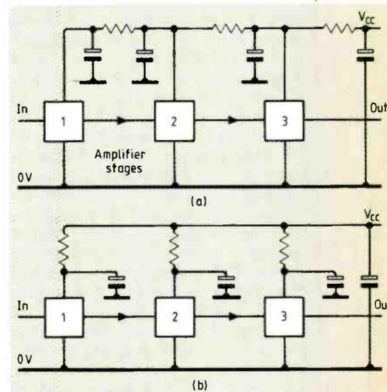
Fig. 12. Earlier methods of supply-line decoupling to avoid LF instability.
