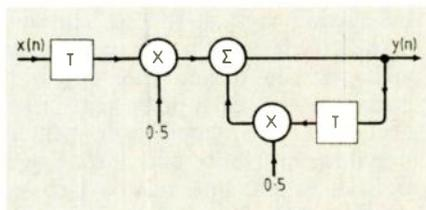
Fig. 4.8. System block diagram of the digital filter described by the recursive relationship  $y(n) = 0.5y(n-1) + 0.5x(n-1)$ .
