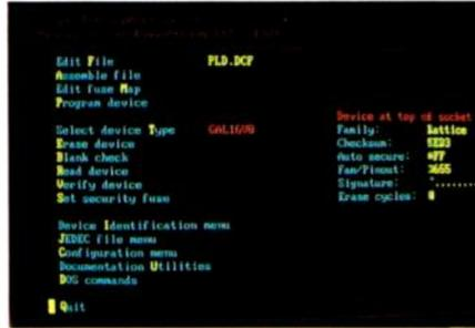
Main menu of MPE PowerLogic EPLD development system, with 16V8 device selected.
