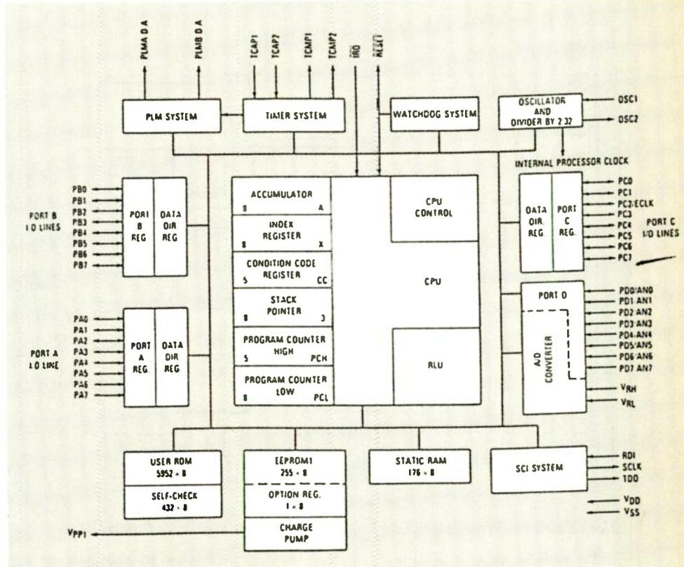
**MC68HC05B6 hc-mos device, with 256byte of eeprom, 8-channel AD/DA and two PWM outputs.**
