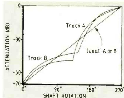
Fig. 3. Ideal logarithmic gain-control response and that given by ganged controls in a stereo system, which may not be well matched.
