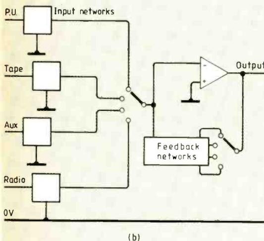
Fig 7. Contemporary practice is to separate low-level from high-level inputs to preamplifier, as at (a). Earlier method was to provide a separate input arrangement for each input (b).
