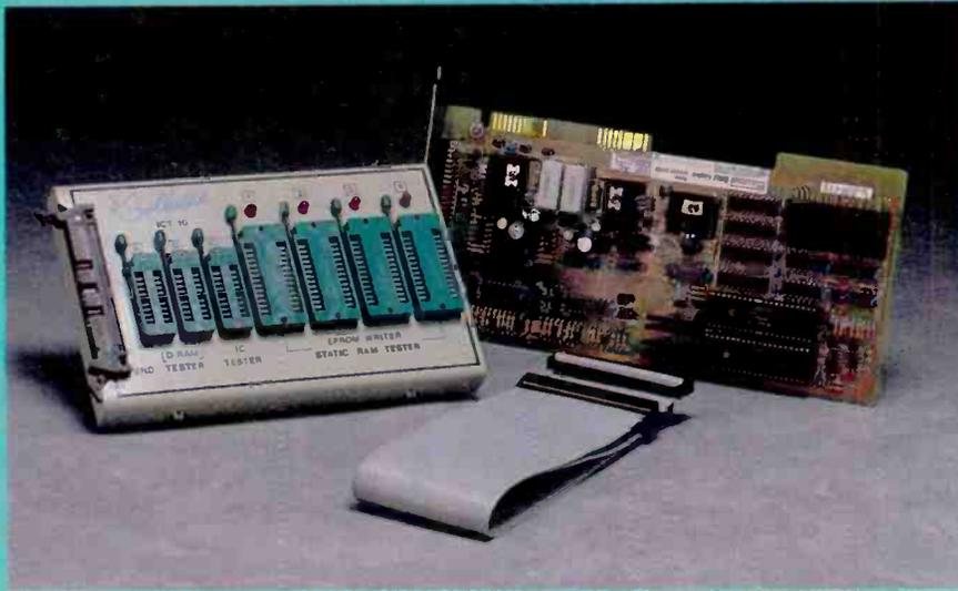
The Sollatek ICT10 IC tester and programmer card fits into the backplane of any IBM compatible XT/AT computer turning the machine into a powerful IC programming and test facility.
