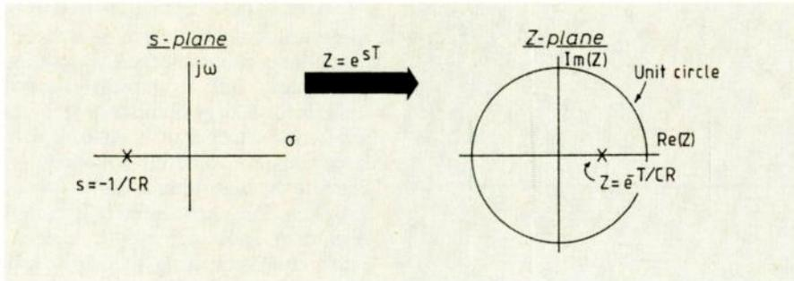
Fig. 4.7. A digital equivalent of the first-order low-pass filter can be derived from the pole position of the system impulse response.
