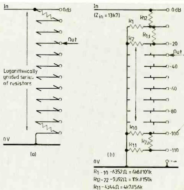
Fig. 6. Log-law switched gain control used by Quad (a), in which graded resistors are switched by c-mos elements. At (b) is alternative type by author which uses non-graded resistor values.
