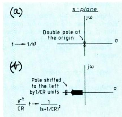
Fig. 4.5. The effect of the frequency shifting rule on the pole-zero diagrams corresponding to the signals (a)  $f(t)=t$  and (b)  $f(t)=te^{-t/CR}$ .
