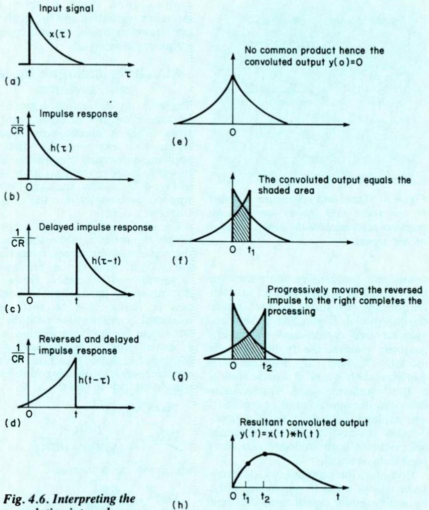
**Fig. 4.6. Interpreting the convolution integral graphically.**
