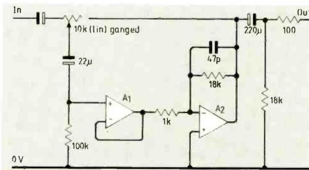
Fig. 4. Active gain control by Baxandall, which uses a combination of input attenuation and feedback.
