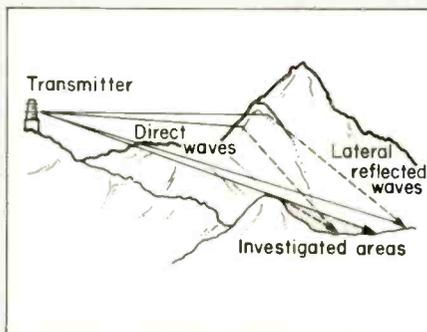
A second test sector took the form of a trench 100m to 200m a.s.l. flanked by mountains but nearly parallel to the direction of propagation, with a few places not line-of-sight.
