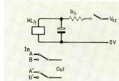
Fig. 8. Simple relay input selector, most suitable for high-level inputs which are not affected by switching transients and hum.
