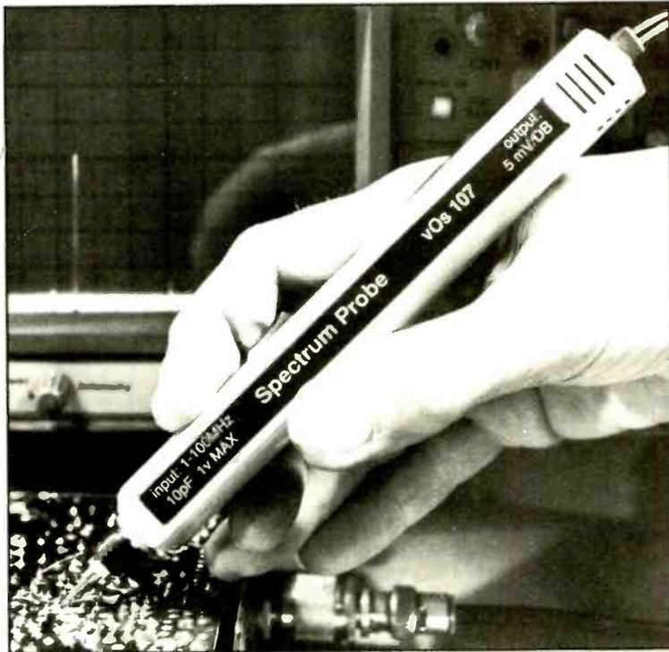
The 107 SPECTRUM PROBE converts a standard 1 MHz scope into a 100 MHz spectrum analyser.
