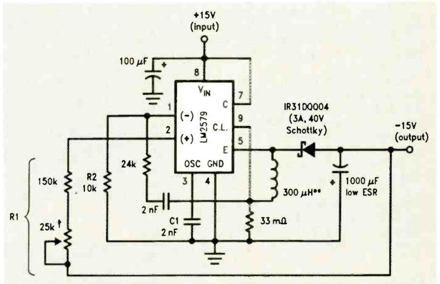
device to be used in an inverting configuration without an extra output transistor. There is an oscillator on-chip, whose frequency is controlled between <1Hz and 100kHz by one external capacitor:
