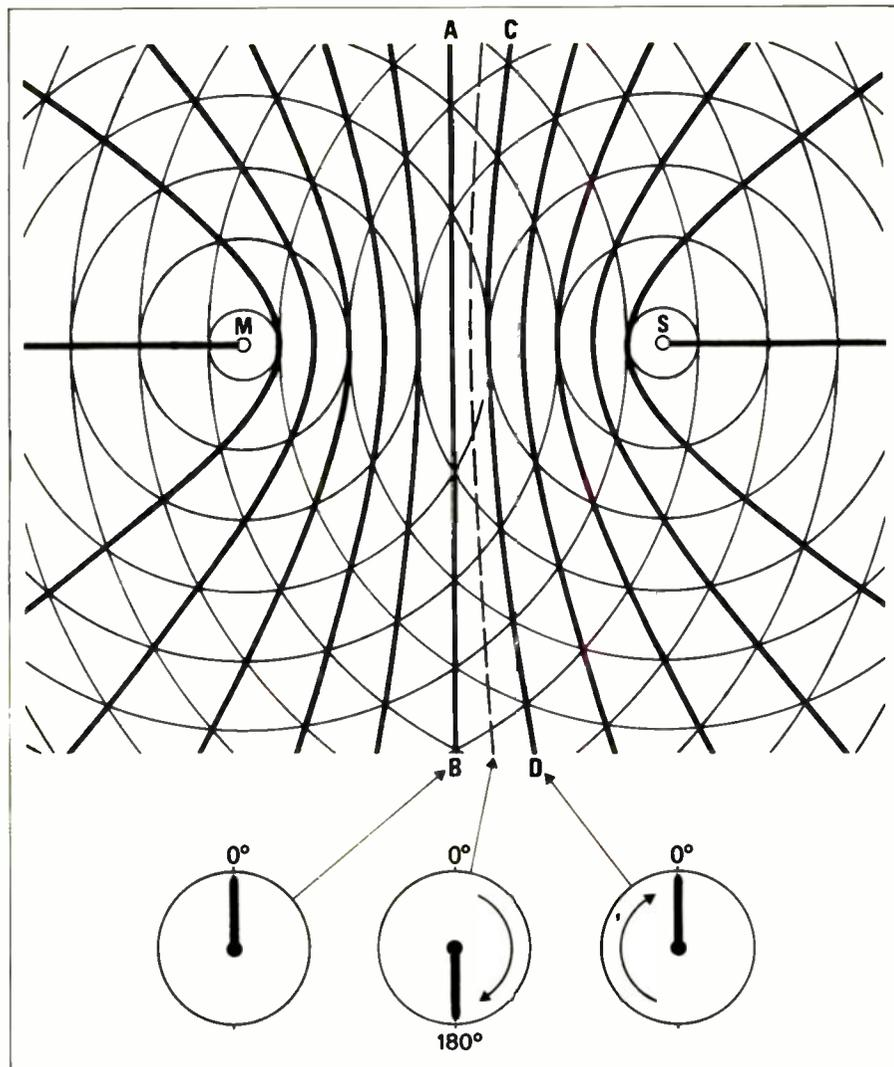
**Fig.1.1. Hyperbolic pattern generated by phase-locked c.w. signals. The concentric circles represent successive wavelengths. The space bounded by two adjacent hyperbolae on which the signals are in phase (e.g. AB, CD) is termed a lane. By convention, the Deccometer turns clockwise for movement from master to slave.**
