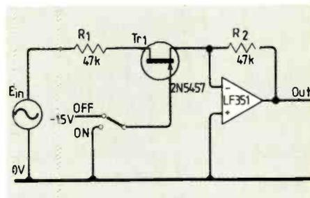
Fig. 11. Series-connected fet switch, which needs virtual-earth succeeding stage.
