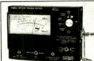
dBm and  $\mu W$  scale; battery life 500 hours.
