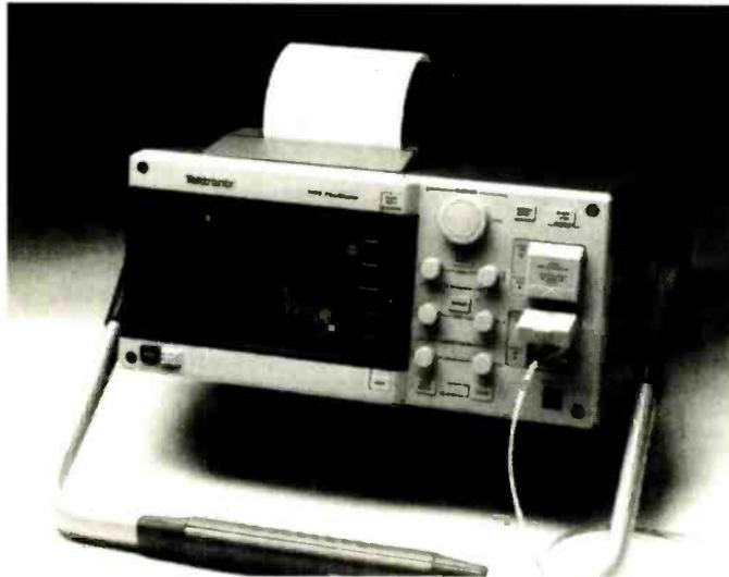
*Tek FiberMaster is the only OTDR to accommodate two dual-wavelength optical plug-ins at the same time*
