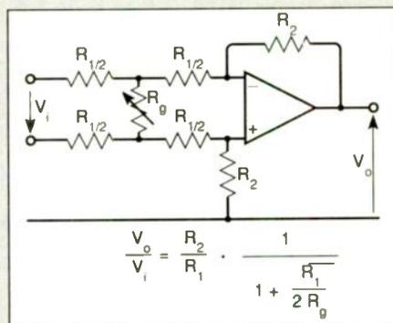
Fig. 2. One way of providing gain adjustment without losing benefits of simplicity and accuracy. Gain is from zero to  $R_2/R_1$ .
