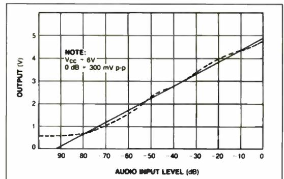
Fig. 2. The dotted line indicates the response of Fig. 1's circuit for the 100Hz to 10kHz audio range; solid line indicates an ideal response. Full scale (0dB) equals 300mV pk-pk.
