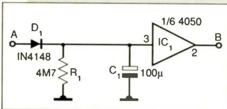
Simple timer for long time intervals, which could be made variable.
