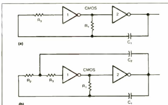
its transition region,  $C_2$  provides positive feedback, thus rapidly moving Gate 1 out of its transition region.
