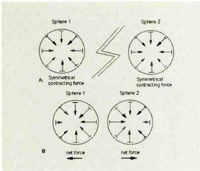
**Fig. 6. Surface forces on two positively charged spheres.**
