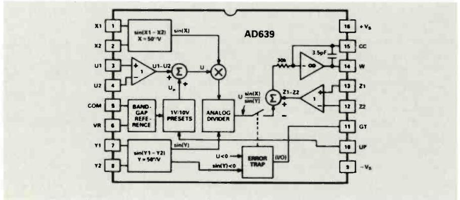
**Fig.1.** Block diagram of AD639 trig. function converter which, among its other roles in life, makes a good function generator.
