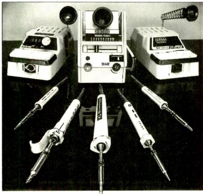
The art of accurate soldering is to maintain the bit temperature at the optimum level.
