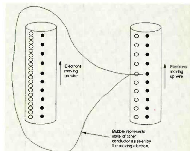
Fig. 8a. Electron and proton densities in a current-carrying conductor. A stationary electron on this conductor observes an equal density of protons and electrons in the left-hand conductor. Although the electrons in the other conductor are moving past the protons they have the same linear density as the protons.
