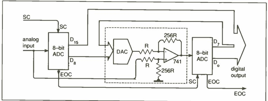
Two low-resolution A-to-D converters perform the function of one high-resolution type, the principle being capable of extension to an increase of  $n$  times.
