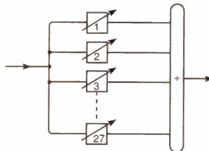
Fig. 2. Implementing a parallel structure.
