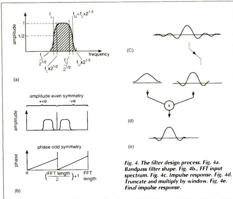
Fig. 4. The filter design process. Fig. 4a. Bandpass filter shape. Fig. 4b., FFT input spectrum. Fig. 4c. Impulse response. Fig. 4d. Truncate and multiply by window. Fig. 4e. Final impulse response.
