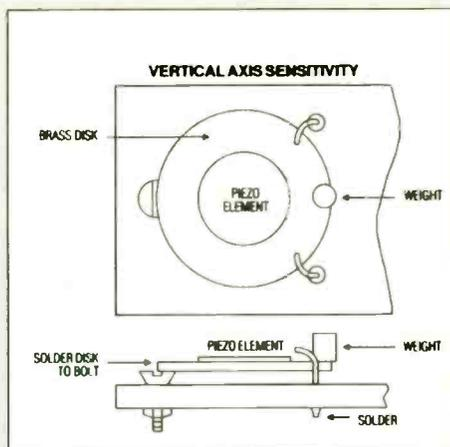
Fig. 2. Mounting of sensor for sensitivity in the vertical direction. Weight increases sensitivity.
