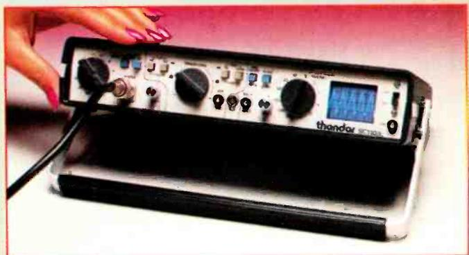
SC110A miniature portable oscilloscope
