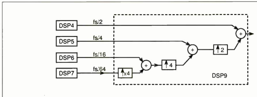
Fig. 10. DSP9 increases the sample rate of DSP4-7 up to 22.05kHz.
