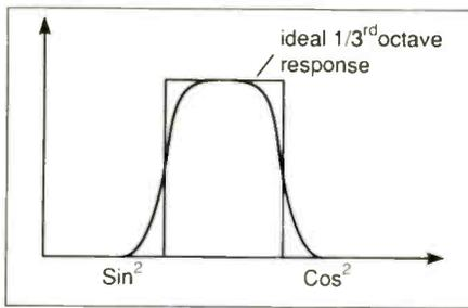
Fig. 3a. Filter's practical response with  $\sin^2$   $\cos^2$  transitions.
