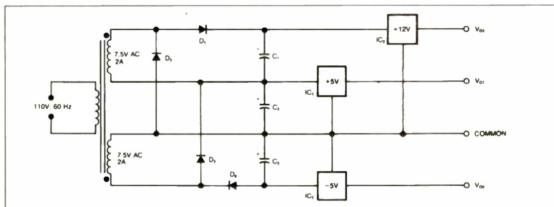
Fig. 1. Simple power supply generating three regulated voltages using a minimum of components.
