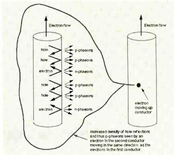
Fig. 9b. Phaeon flux from a conductor carrying a current as seen by a moving electron in another conductor.
