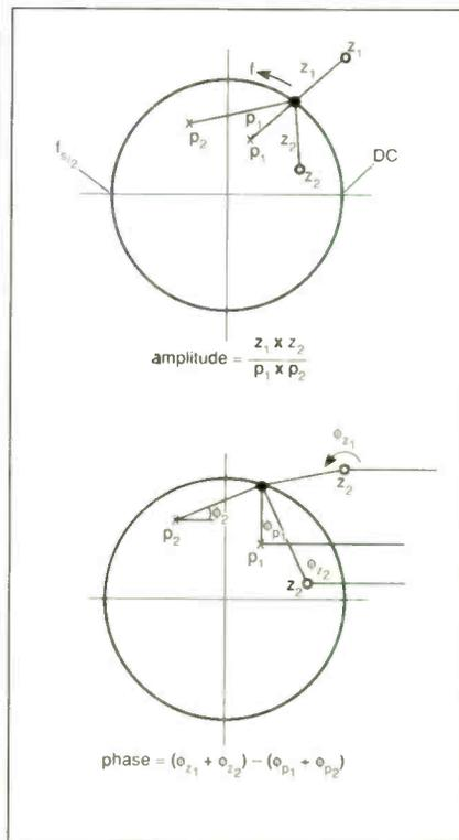
Fig. 1a. (top) Calculated amplitude and phase. Because zeros only cause decrease in amplitude, they can be placed anywhere. Poles cause an increase in amplitude and can only be placed inside the circle.
