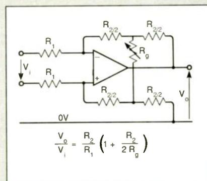
Fig. 3. Another way, giving adjustment from  $R_2/R_1$  to a high value.
