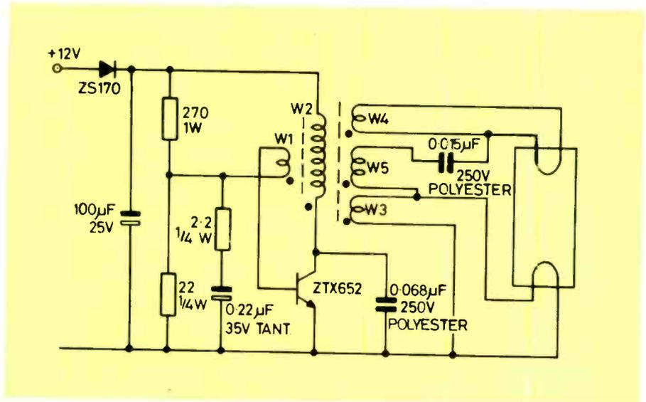
Fig. 3. Driver for an 8W fluorescent tube running at 20kHz. Only one transistor is needed since the ZTX653 supplies energy to the tube in both forward and flyback modes.
