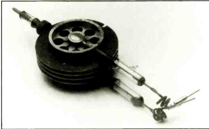
1. This is clearly a prototype 10cm cavity magnetron. What is unusual about it? (Clue: The efficiency would probably have been very low, say, 10-12%)
