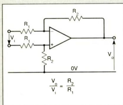
Fig. 1. Ordinary differential amp for fixed-gain operation.
