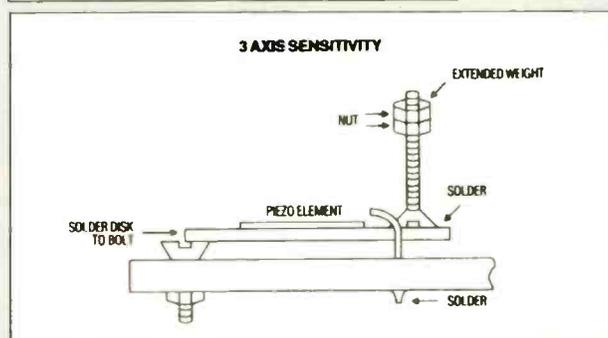
Fig. 3. Sensitivity in all directions is given by this layout, nuts on the 1/4in bolt being adjusted for sensitivity.
