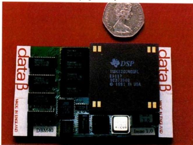
and communications transputer section. As well as a 16bit T222 processor, this section has 64Kbit of sram and 32Kbit of rom to store user code. Dean Microsystems, 0734 845155.
