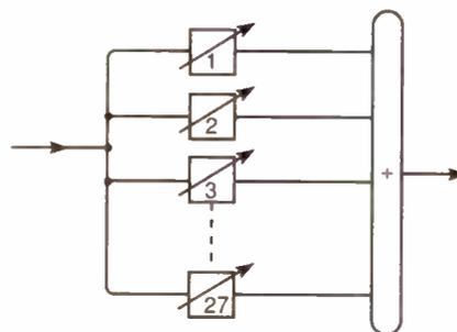
Fig. 2. Implementing a parallel structure.
