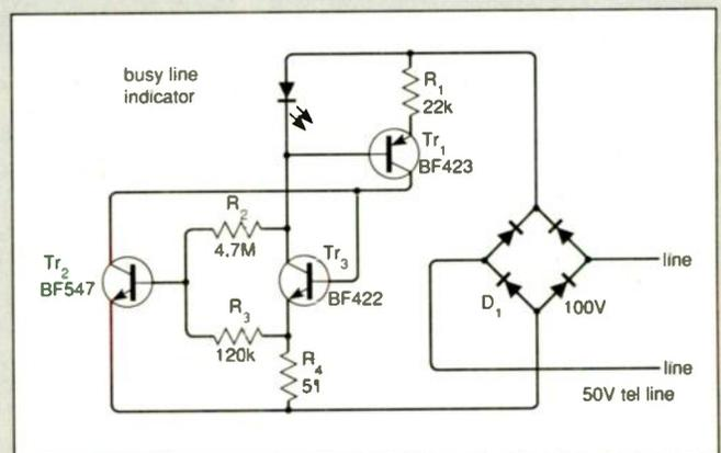
*Telephone line activity indicator uses a mere 50µA in standby mode and may be modified for use in control.*
