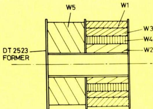
Transformer details. Core type FX3439 with 0.005" (0.125mm) spacer.
