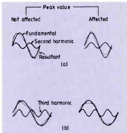
Fig. 3 In a wide band detector measuring the input signal's positive peak may affect the expected ratio of peak to RMS voltage. (a,b) Show resultant phases in second and third harmonics.
