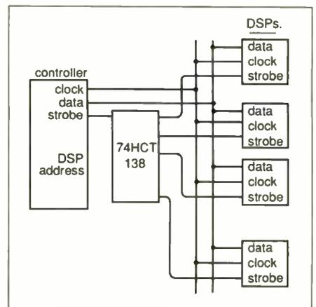
Fig. 8. Passing control data to the DSPs.
