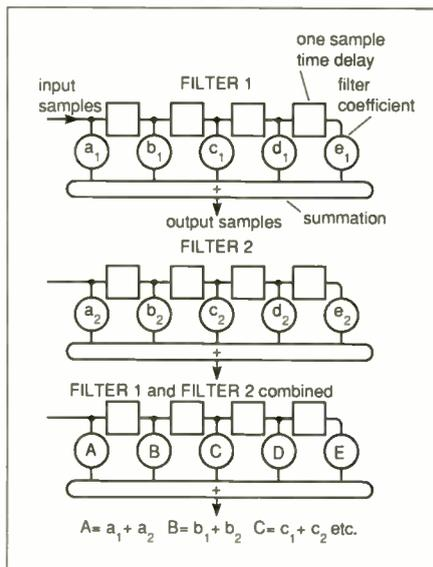
Fig. 6. Combining FIR filters into a single filter.
