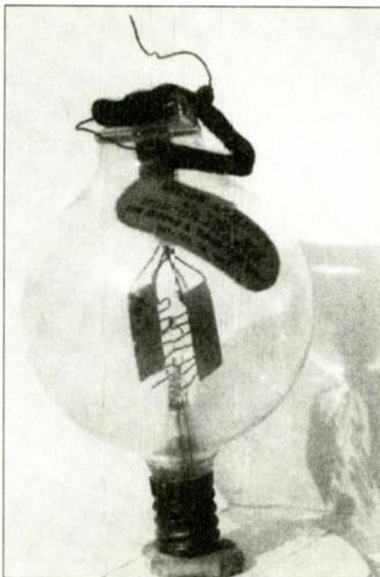
*Marconi's magnetic detector, introduced in 1902 and the predecessor to the valve.*
