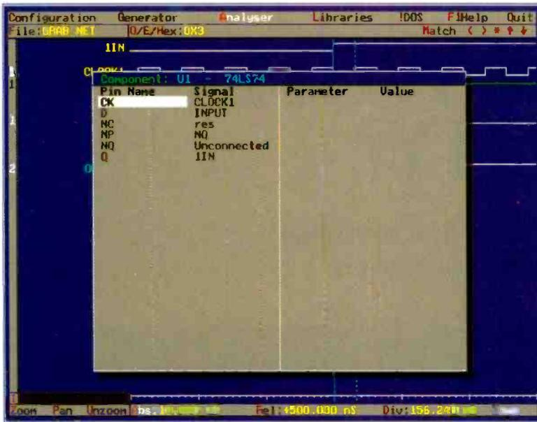
The net list can be entered by using the built in on-line netlist editor.
