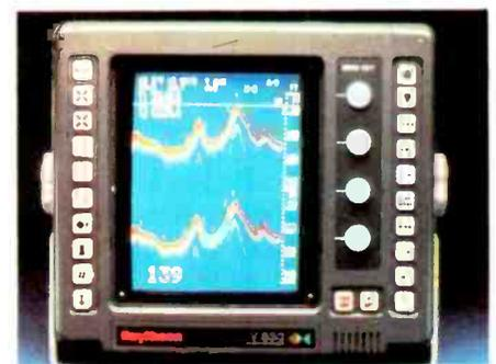
*Digital signal processing techniques have revolutionised the display of sonar imaging*
