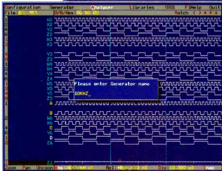
down resistors, high impedance and undefined. During simulation, it looks ahead to each change in logic state and only stores data when a change occurs.
