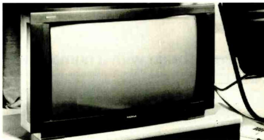
**Fig. 3. Pal-plus pictures would be displayed on 16:9 widescreen TV sets similar to this current model for standard transmissions made by Nokia Consumer Electronics. (When standard 4:3 format pictures are shown on wide-screen sets the image can be expanded to fill the full width of the screen, though of course this cuts off some lines at the top and bottom).**
