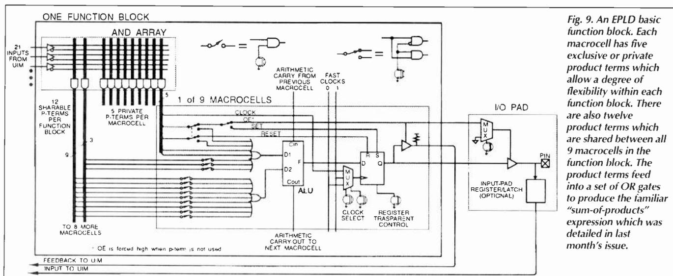
Fig. 9. An EPLD basic function block. Each macrocell has five exclusive or private product terms which allow a degree of flexibility within each function block. There are also twelve product terms which are shared between all 9 macrocells in the function block. The product terms feed into a set of OR gates to produce the familiar "sum-of-products" expression which was detailed in last month's issue.
