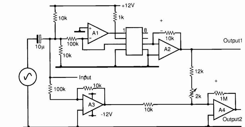
**Fig. 2.** Test circuit used for evaluating the IL300 operating in positive unipolar photovoltaic mode. Ideally, there should be zero resultant signal at output 2.
