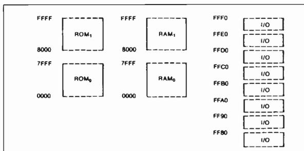
Fig. 1. 64kbyte memory system provides 64kbytes of physical ram virtually overlapped by 64kbytes of physical eprom.
