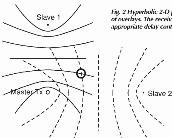
Fig. 2 Hyperbolic 2-D positioning with two sets of overlays. The receiver is positioned where the appropriate delay contours intersect.
