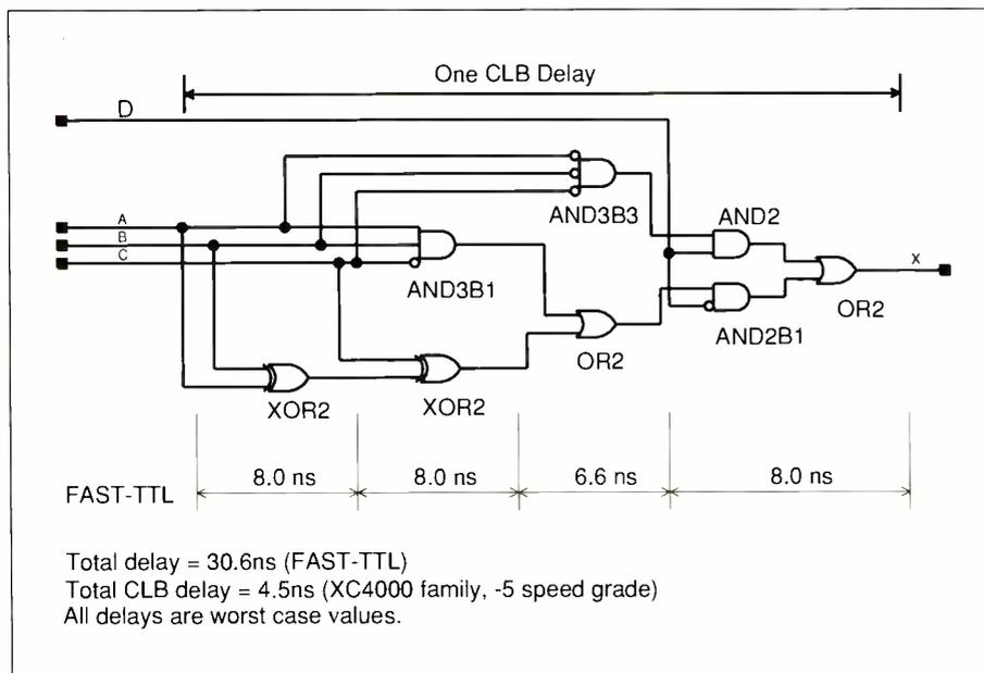
Fig. 6. Comparison of FAST-TTL and CLB delay. The worst case delay through a single CLB is between 4.5 and 7ns depending on the speed grade of the device. Compare this with the delay of the same logic when implemented in fast-TTL. The performance increase is obvious, and as all FPGAs use a cmos process they also have the advantage of drawing much less power.
