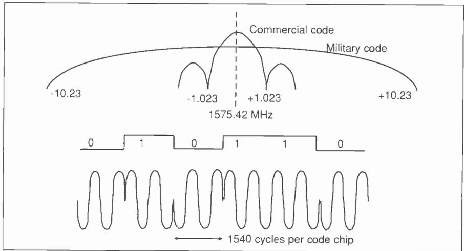
Fig. 5. GPS combines the benefits of terrestrial systems with continuous availability, satellite systems for global coverage, at the cost of many satellites and a complicated receiver to decode a complex modulation scheme. Spread spectrum allows all 24 satellites to transmit continuously on the same frequency.
