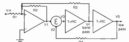
**Fig. 2.** Configuration of **ML2111** filter block, in which a resistor is simulated by a switched capacitor.
