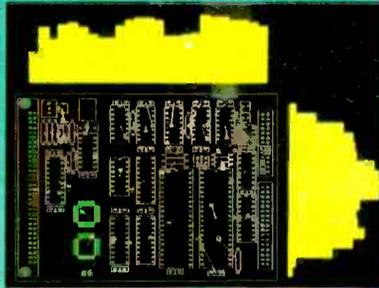
ULTIshell, the integrated user interface, makes sure all your design information is transferred correctly from ULTIcap to ULTIboard. Good manual placement tools are vital to the progress of your design, therefore ULTIboard gives you a powerful suite of REAL-TIME functions such as, FORCE VECTORS, RATS NEST RECONNECT and DENSITY HISTOGRAMS. Pin and gate swapping allows you to further optimise your layout.
