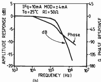
Fig. 6. (left) Bandwidth of the *IL300* optocoupler: a) in photovoltaic mode b) in photoconductive mode.
