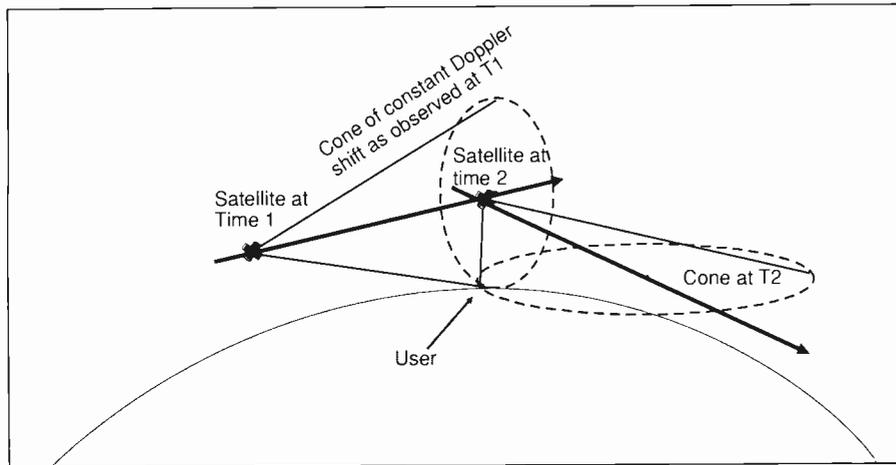
**Fig. 4.** The Transit satellite system operates by measuring the Doppler shift caused by the satellite's motion. As multiple satellites are not usually available, the same one can be used twice with a time separation, but the vessel's course and speed meanwhile must be accurately known. Fixes are infrequent, as there are one to two hours between each low-orbit satellite pass
