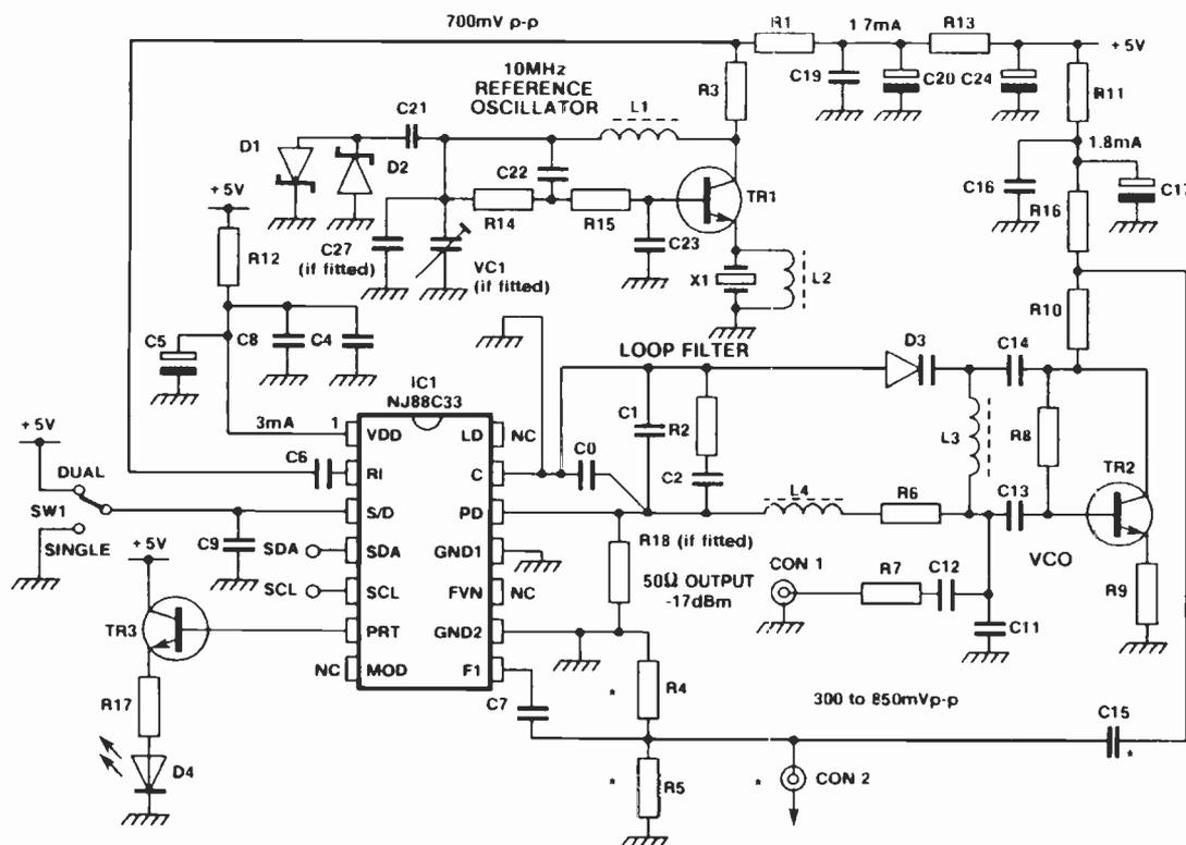
Fig. 8. The GEC-Plessey NJ88C33 evaluation board provides a reference oscillator, a 60 to 80MHz VCO and a simple loop filter to complete a minimal frequency synthesiser loop. The two units allow analysis of different loop variables as well as the selection of comparison frequencies for fast frequency-losing loops.
