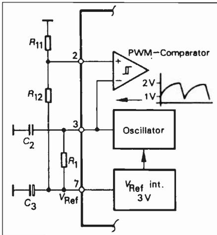
Fig.3. PWM comparator circuit; a variable pin 2 voltage allows matching to different battery capacities.
