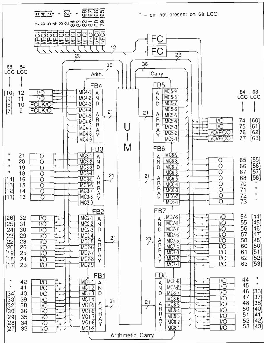
Fig. 8. A typical EPLD structure. This is the Xilinx XC7272 device.
