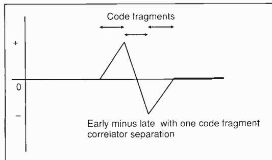
**Error signal that advances or retards tracker. Differencing the signals from two correlators that have a small time offset yields an error signal that can control a tracker to keep the receiver in lock with the transmitter.**
