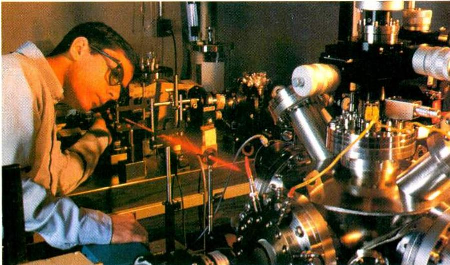
An ultra-fast laser is used to heat the sample and also to trigger the electronic camera.
