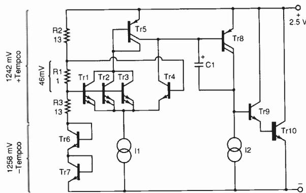
Closing the feedback loop with a bias string. The resistor values refer to multiples of 750Ω.
