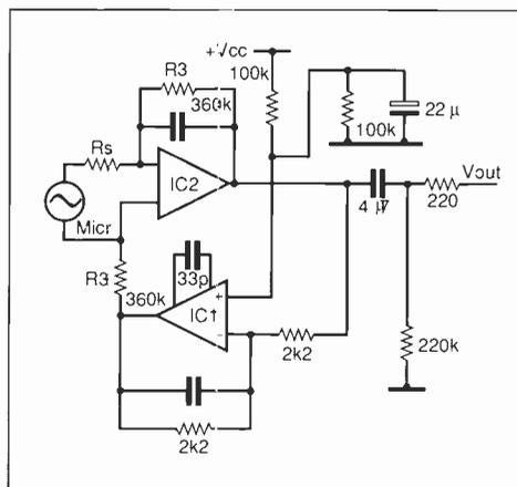
Fig. 1. Alternative mic preamp design
