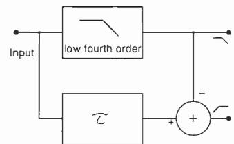
**Fig. 1.** A phase-linear network with a low-pass section and a high-pass using time delay and subtraction.
