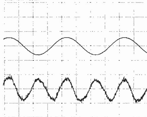
Fig. 3. 5V pk-pk 50Hz input test signal to circuit of Fig. 2 (upper trace) and outphased distortion products (lower trace).
