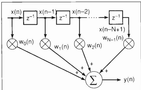
Fig. 3 Linear finite impulse response filter structure
