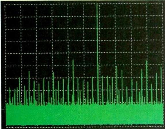
Fig. 6. STEL2173 typical output spectrum using the application circuit of Fig. 5. Particular attention must be paid to the wiring between the DDS controller chip and the outboard dac. Any variation in phase delay between the bits presented to the converter will manifest itself as increased spur levels in the output spectrum.. Frequency span 0-400MHz Reference level +0dBm Resolution bandwidth 10kHz Scale log 10dB/div Output frequency 234.567MHz Clock frequency 1GHz.
