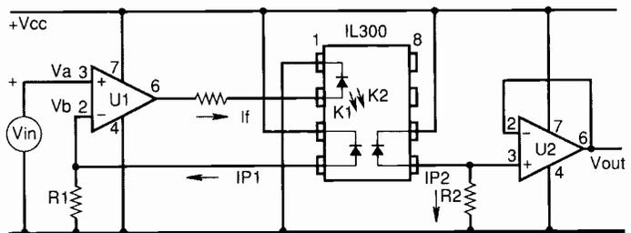
**Fig. 1.** Typical application circuit for the IL300 linear optocoupler, in positive-going unipolar photoconductive mode. Although  $K_1$  and  $K_2$  vary with temperature, their ratio  $K_3$  is virtually temperature independent. Devices are coded into bands according to the spreads of  $K_1$  and  $K_3$ .
