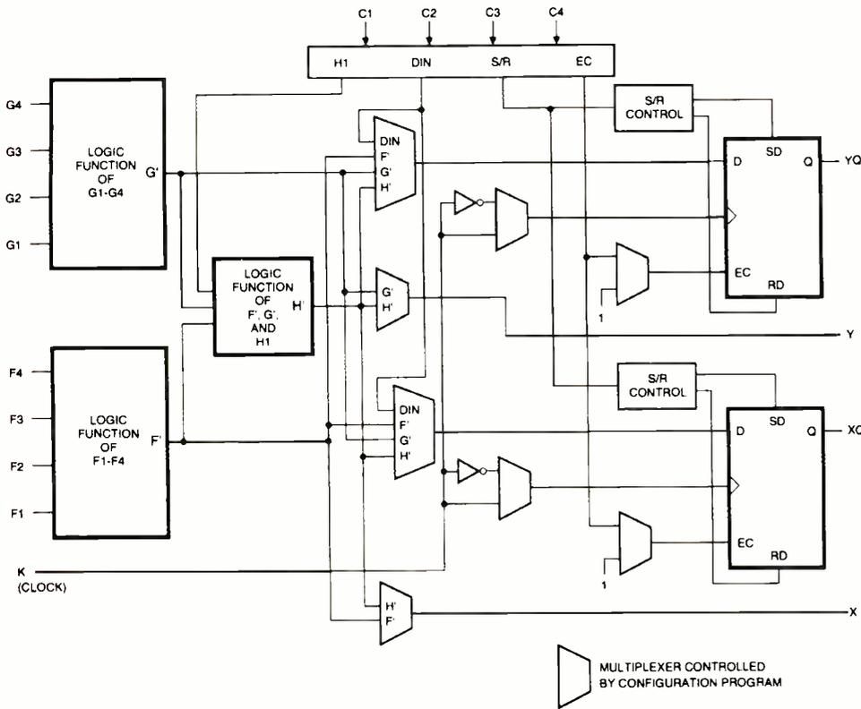
Fig. 5. Structure of an XC4000 configurable logic block. Each function generator (F and G) is a look up table that can implement any function of four variables. These may be optionally combined together via the smaller function generator (H) to provide various permutations of up to nine separate logic variables.
