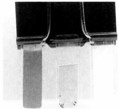
*Before, between and after (right to left) exposure to UV. The layered viologen compound left in the dark, exposed to sunlight for 2h, and irradiated with a UV lamp for 2h.*
