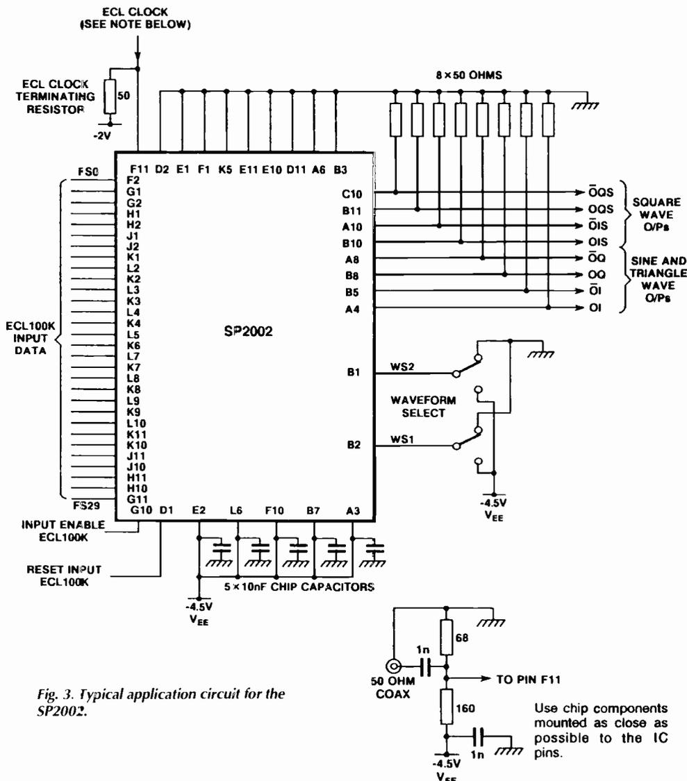
Fig. 3. Typical application circuit for the SP2002.
