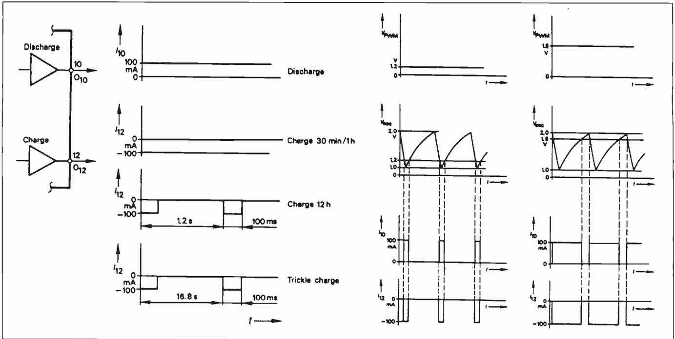
Fig.2. Timing of the discharge, charge and trickle charge operations. Pulse operation comes into action for a 12h charge and trickle charge.
