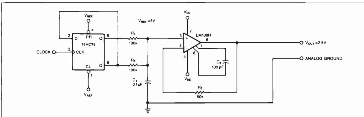
Dividing  $V_{REF}$  in half using no precision components.
