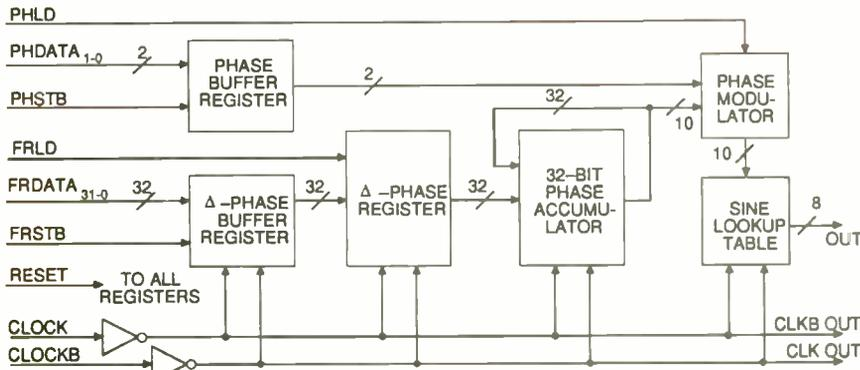
Fig. 4 The STEL2173 Numerically Controlled Oscillator from Stanford, usable for synthesis of up to 400MHz, provides 32-bit frequency resolution (i.e. 0.23Hz at 1GHz clock) and very fast frequency hopping – although the external digital to analogue converter required will add to the settling time.
