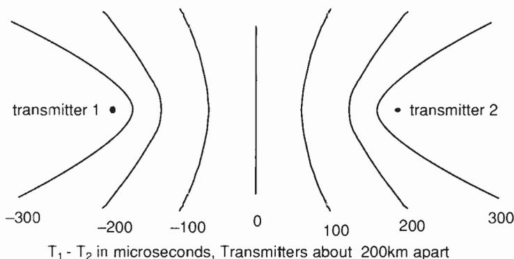
Fig. 1. Hyperbolic systems before the microprocessor used an overprinted chart to lookup the lines of position, having read the relative delay from the receiver. The drawing shows the overlay for a pair of transmitters, after subtracting the delays in transmitter start time that are inserted to ensure the signals due not overlap each other.
