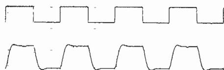
Fig. 5. Input and output 1 (Fig. 2) with a 3.5V pk-pk 20kHz square-wave input.
