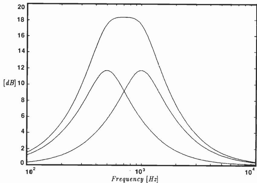
Fig.3. Interaction of two adjacent (one octave apart) sections at maximum boost. The resulting boost is 18dB. If this is undesired, more selective and more complex filter types must be used.
