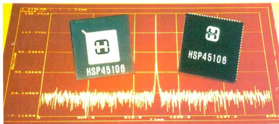
Harris has recently added to its range of NCOs for use up to about 40MHz output, with the HSP 45106. Frequency resolution is 32 bits (0.01Hz at 40MHz) and programmable phase control register allows control to better than 0.006 degrees. For applications at these frequencies, the range provides a cost-effective solution – the HSP 45102 is offered as a low-cost device at £17.90 (100-off price). 69dB of spurious-free dynamic range is claimed to be attainable.
