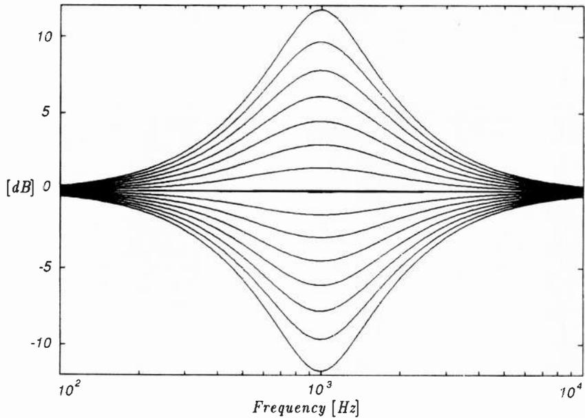
Fig.2. Frequency responses of a single 1kHz equalising section at various code values (0F, 1F, 2F, ..., 7F, 8F, 9F, A0, ..., F0). Maximum boost and cut is 12dB. Because of the  $x/(1-x)$  law, the steps are not equidistant; the lowest is around 1.5dB and the highest is around 2.2dB.
