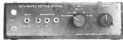
The aerial consists of an outdoor head unit with a control and power unit and offers exceptional intermodulation performances: SOIP +90dBm, TOIP +55dBm. For the first time this permits full use of an active system around the 1f and mf broadcast bands where products found are only those radiated from transmitter sites.
