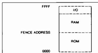
Fig. 2. Logical organisation of the memory in Fig. 1 locates memory-mapped i/o space at the top of the ram and allows the boundary to be set between the ram and eprom by manually setting a fence address.
