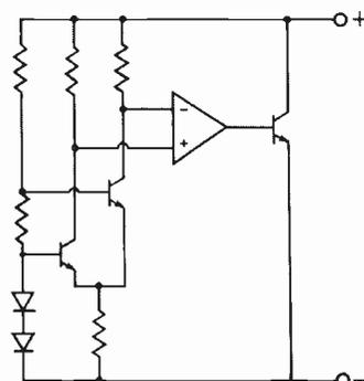
Functional circuit diagram of ZRA series bandgap voltage references.
