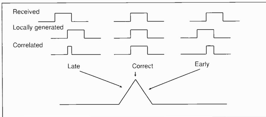
**Correlation response of a squared pulse. Recovering a spread-spectrum signal relies on the fact that it can be de-spread when multiplied by the same spreading code again. More than one chip of the code in timing error means no signal, and a single correlator does not know which way to adjust to find the peak.**
