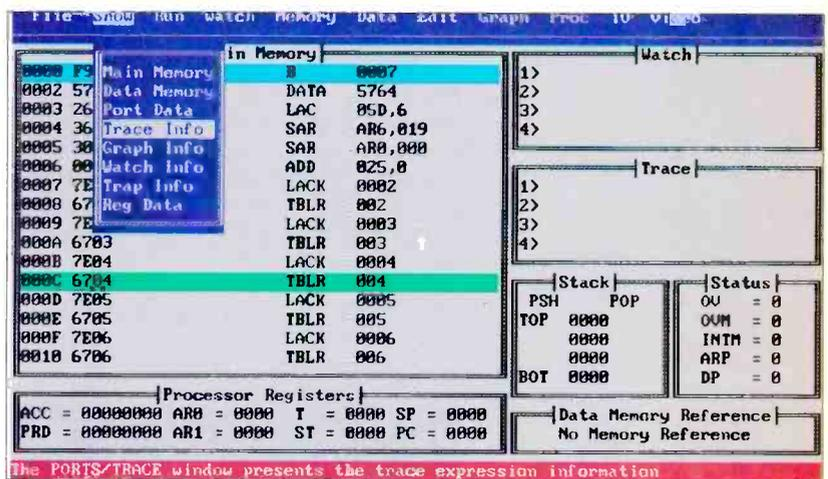
*Simulator display has a major part given over to the code being executed. The current line of execution is highlighted.*
