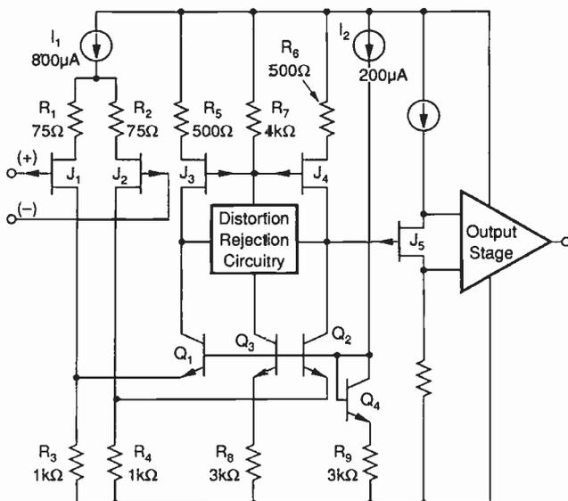
tortion by a factor of 101 to make it possible to measure it. Resistor  $R_3$ , added to what is a standard inverting op-amp, leaves the closed-loop gain alone but reduces the feedback for error correction by 101 times. Input signal and load arrangements are normal.
