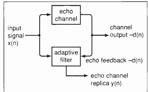
Fig. 1 Block diagram of the adaptive filter demonstration program.
