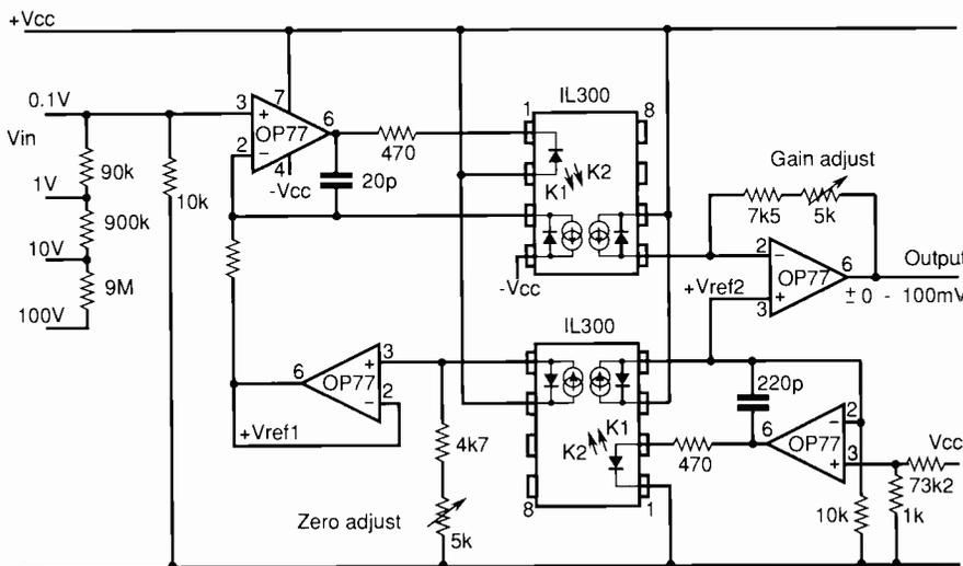
Fig. 9. Bipolar photoconductive isolation amplifier using an additional optocoupler to convey to the input amplifier the same pre-bias voltage used in the output amplifier. (
