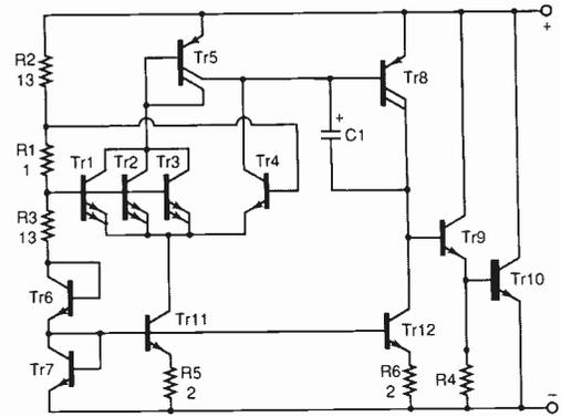
Adding the bias currents through current mirrors. The 200mA output transistor allows exceptional dynamic range for a bandgap reference.
