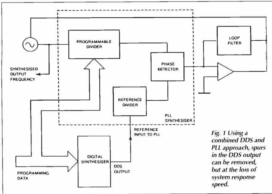
Fig. 1 Using a combined DDS and PLL approach, spurs in the DDS output can be removed, but at the loss of system response speed.
