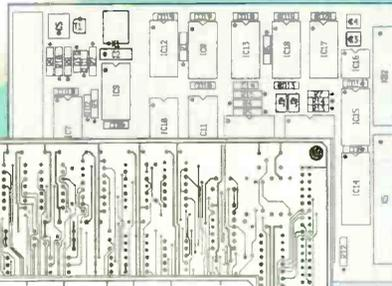
ULTIboard's backannotation automatically updates your ULTIcap schematic with any pin and gate swaps or component renumbering. Finally, your design is post processed to generate pen / photo plots, dot matrix/laser or postscript prints and custom drill files.
