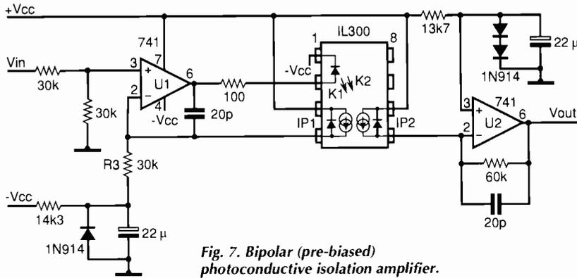
Fig. 7. Bipolar (pre-biased) photoconductive isolation amplifier.
