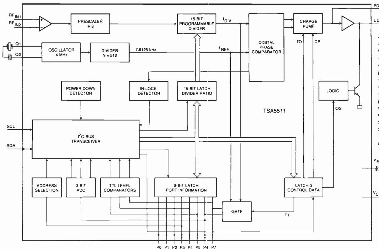
Fig. 9 At £1.45 (100-off price) the TSA 5511 phase-locked loop IC from Phillips provides a cost-effective single-chip solution for TV tuners to 1.3GHz
