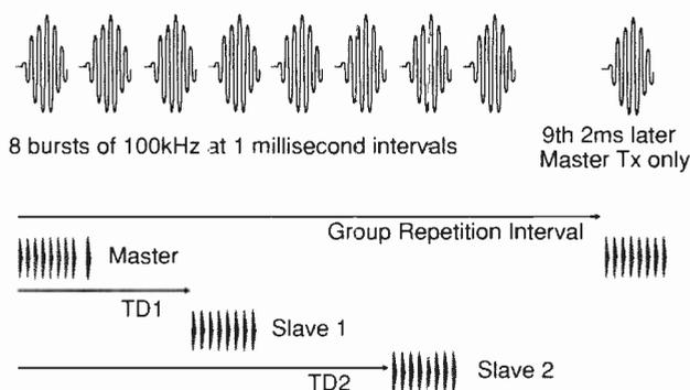
Fig. 3. The Loran-C system operates in burst mode to allow many transmitters to share the same frequency, leading to a very simple radio front end to the receiver. Master transmitters are identified by a 9th pulse, which can be blinked to indicate system problems. The actual chain in use is identified by its repetition rate.
