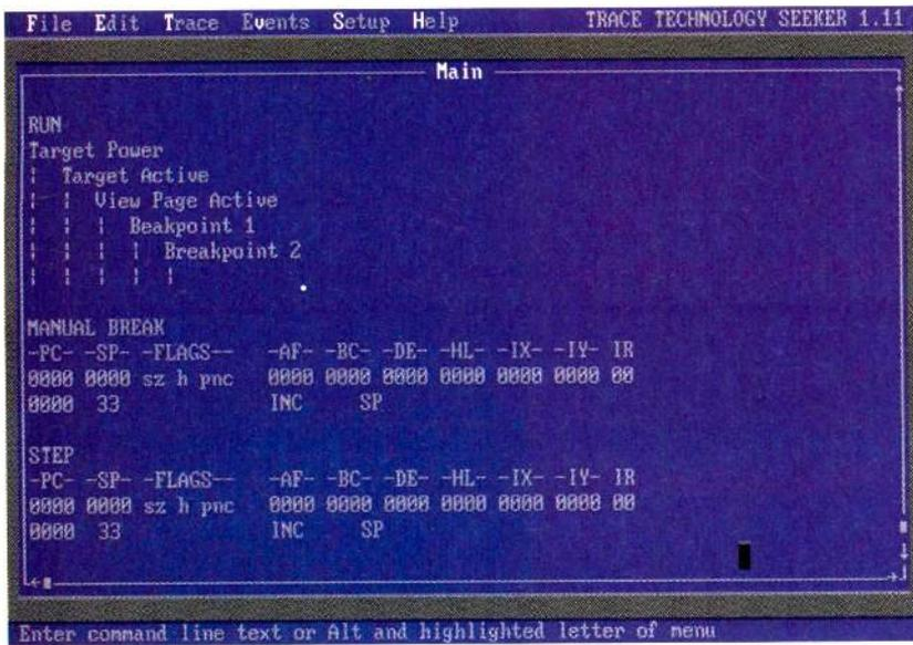
*Seeker can single-step, showing the processor status at each step.*
