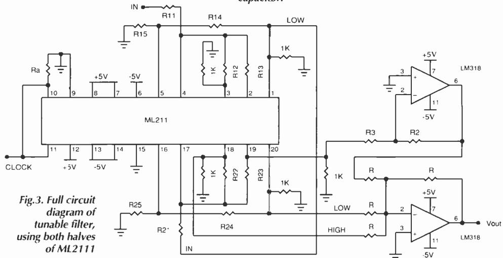
**Fig. 3.** Full circuit diagram of tunable filter, using both halves of **ML2111**
