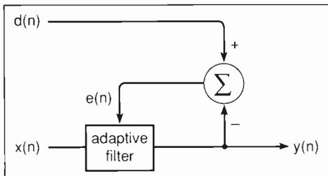
Fig. 2 Block diagram of an adaptive LMS filter
