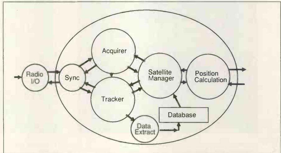
Fig. 3. Breaking down the GPS task into its sub-processes. GPS is by far the most complex process, both to design and to compute. Most of the CPU time is used in the tracker, after acquirer has finished, but the complex maths is in the satellite manager and position calculator
