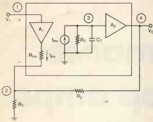
Fig. 3. Expanded non-inverting current mode circuit.
