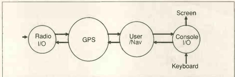
Fig. 2. All-software system overview. A parallel processor like the transputer allows simple programming, as if there were a CPU per task. Only the console I/O process is hardware dependent, and then only at the lowest level.
