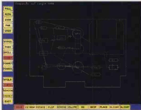
Far right This circuitry, routed with the autorouter, is the maximum circuitry possible on the free version.
