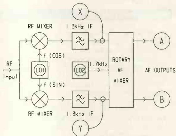
mixer is 2.7kHz. The lower row shows that an RF input frequency 1MHz-1kHz also gives an IF of 1kHz, but this time gives a rotary mixer output of 700Hz.
