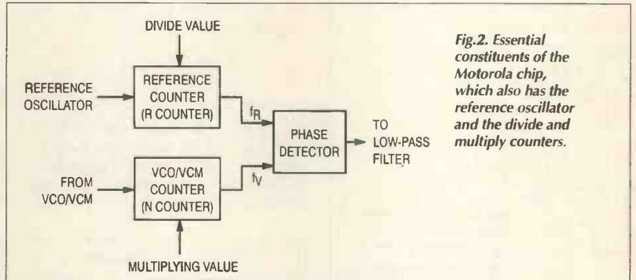
Fig. 2. Essential constituents of the Motorola chip, which also has the reference oscillator and the divide and multiply counters.
