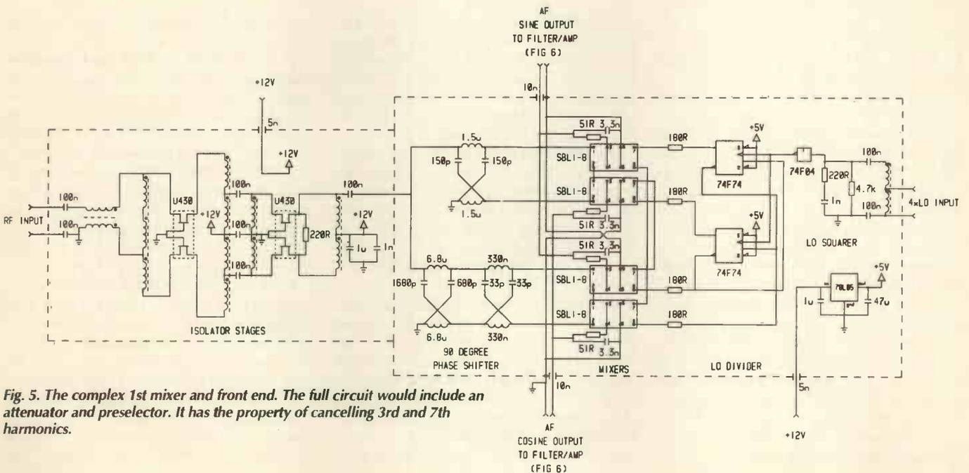
Fig. 5. The complex 1st mixer and front end. The full circuit would include an attenuator and preselector. It has the property of cancelling 3rd and 7th harmonics.
