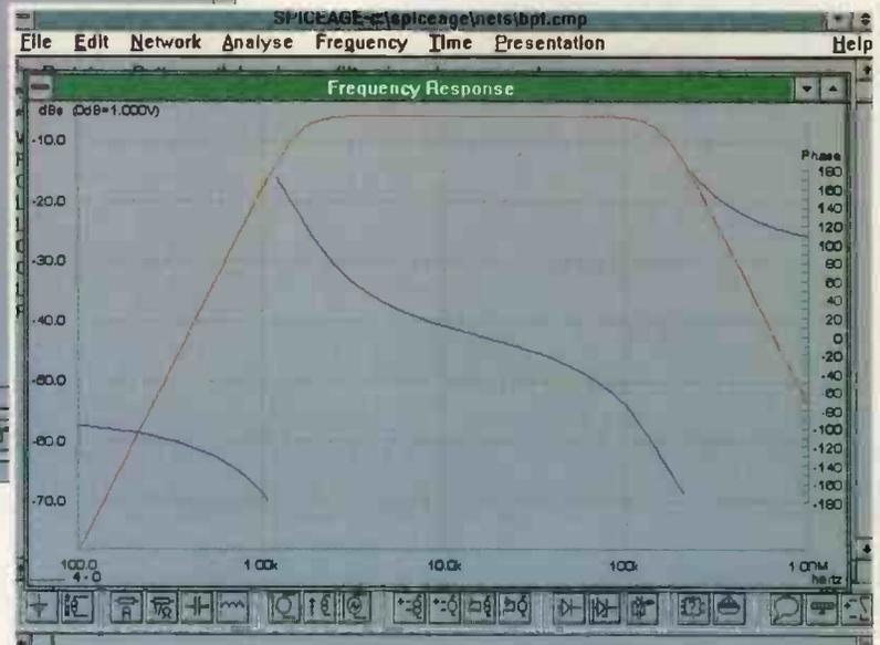
Below: Displaying a filter frequency and phase response
