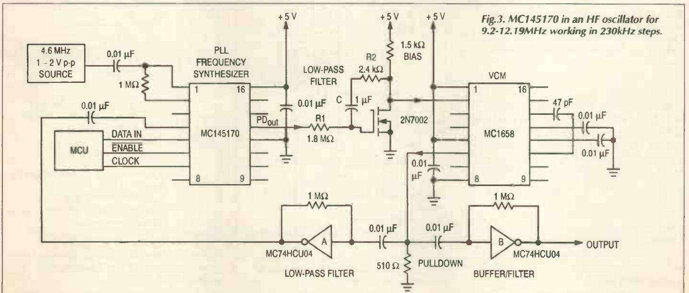
Fig. 3. MC145170 in an HF oscillator for 9.2-12.19MHz working in 230kHz steps.
