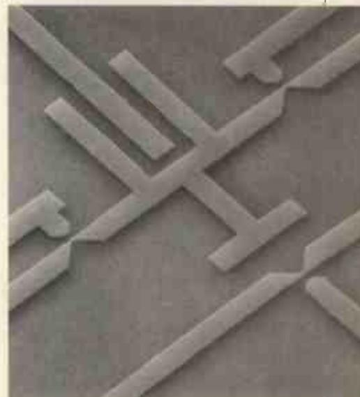
The cell already developed uses two multiple tunnel junctions to control the flow of electrons along a conductive path leading to a capacitor memory cell and a charge sensing detector. The junctions write and erase the memory cell by squeezing a conductive path with an electric field so that electrons are allowed past one at a time. Changing the field strength can turn this current on and off.
