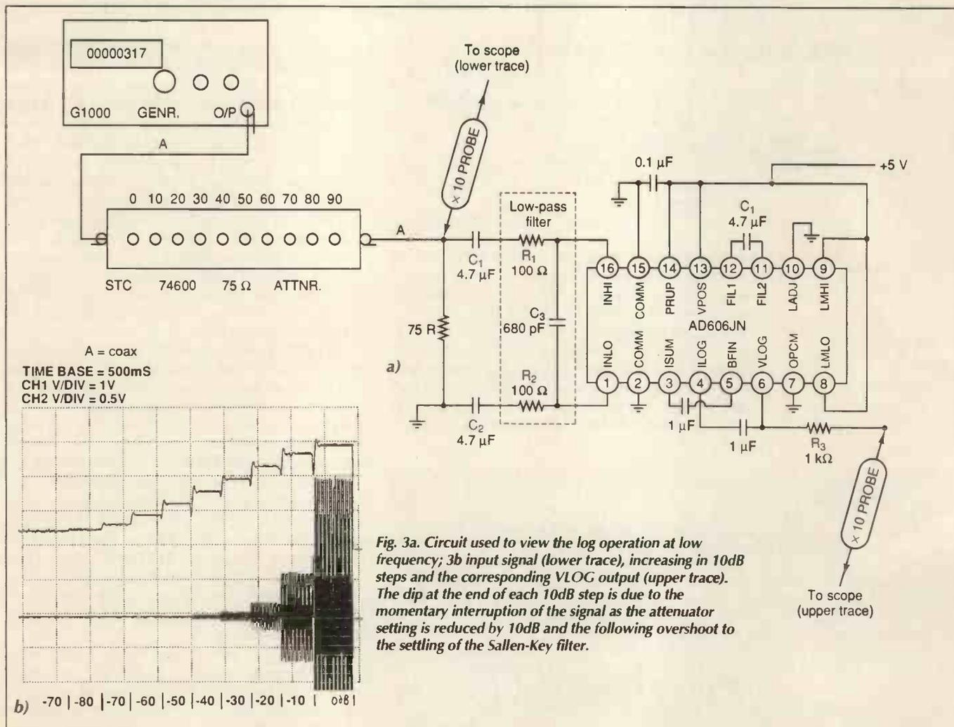
Fig. 3a. Circuit used to view the log operation at low frequency; 3b input signal (lower trace), increasing in 10dB steps and the corresponding VLOG output (upper trace). The dip at the end of each 10dB step is due to the momentary interruption of the signal as the attenuator setting is reduced by 10dB and the following overshoot to the settling of the Sallen-Key filter.
