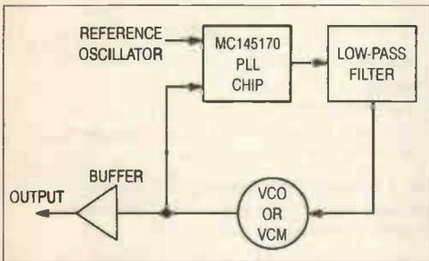
Fig. 1. Basic block diagram of a phase-locked-loop frequency synthesiser, in this case using Motorola's MC145170 PLL IC and a low-pass filter.
