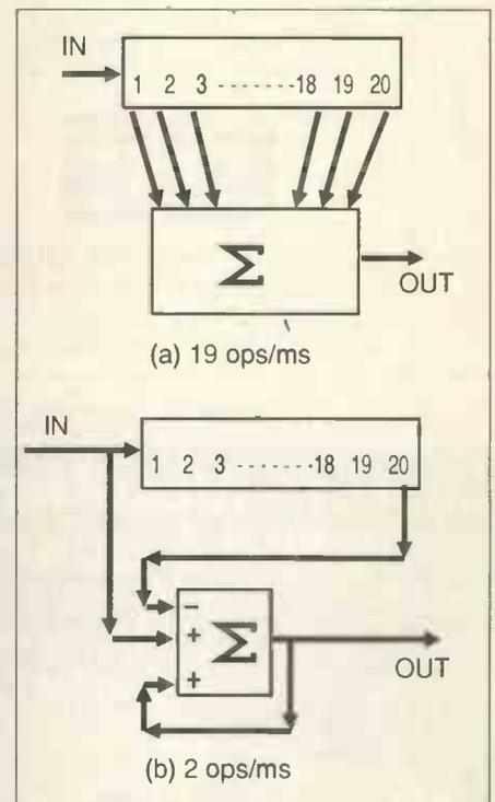
**Fig. 6a and b. Filter implementations.** This is a continuous 20ms filter that optimally drags 50baud data from the noise. In fact, at this point the GPS signal is well above the noise, as it has been filtered to a few hundred hertz bandwidth. The two implementations shown produce the same output, but one is ten times faster. Note it must be cleared at startup.
