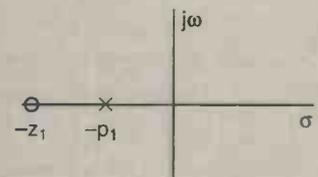
Fig. 4. Pole and zero location on the  $s$ -plane
