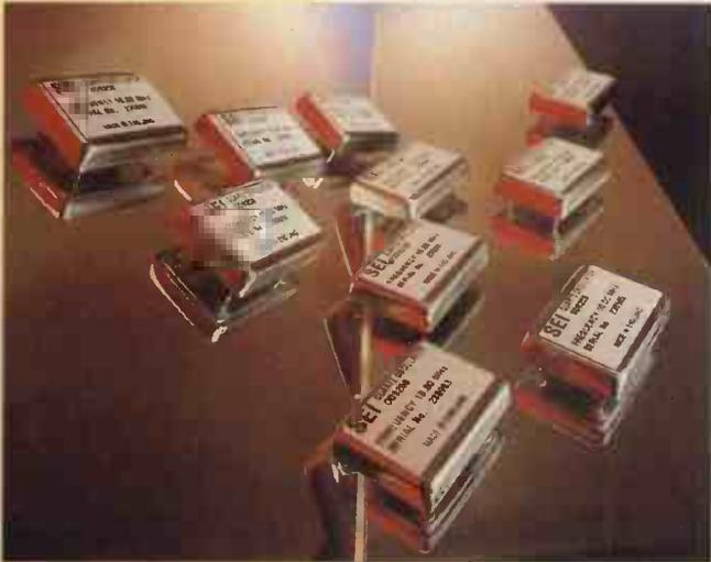
**Compensated oscillators.** As an alternative to oven-controlled crystal oscillators, SEI offers the OD9208 series of digitally compensated devices that cost less than half the price of oven types and use a hundredth of the power. Short-term stability is better than  $2 \times 10^{-9}$  and in the long term better than 0.5ppm in a year. Frequencies range from 4MHz to 25MHz with a tolerance of better than  $\pm 0.3$ ppm. External adjustment can handle  $\pm 5$ ppm. SEI Ltd, 0706 367501.
