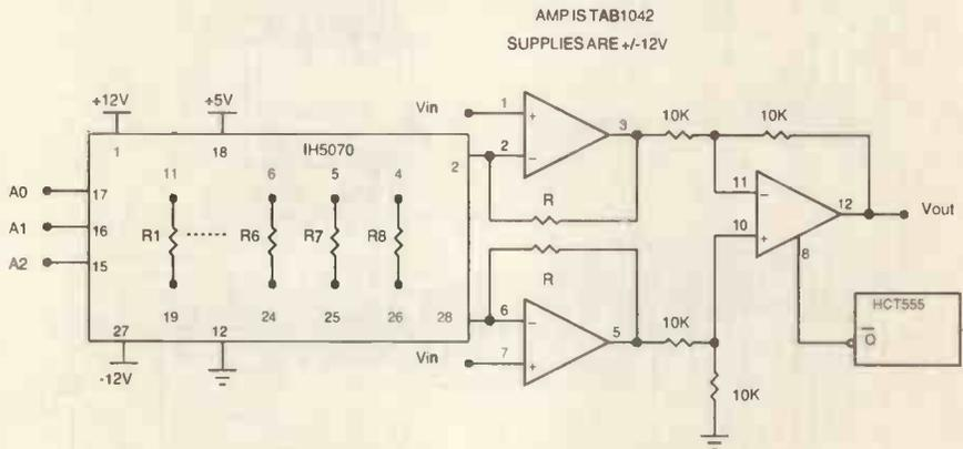
Three op-amp instrumentation amplifier, programmed in time range and gain, which is set by selecting one of the IH5070 resistors by the A<sub>0</sub>-A<sub>2</sub> digital input.
