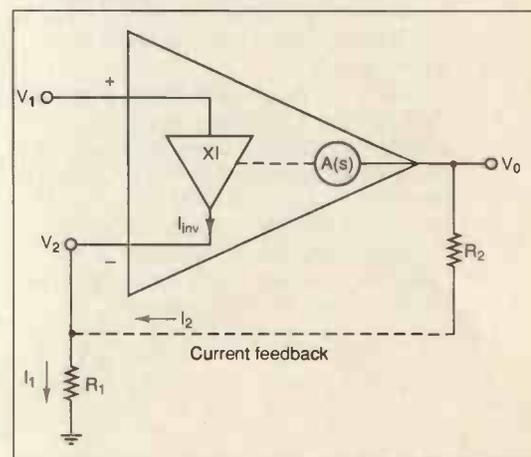
Fig. 2. Non-inverting current mode op amp. Pole locations – hence performance – can be held constant.
