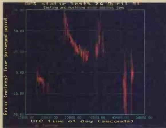
Performance with SA. A week later, with SA turned on, and in the day time, the position wanders by up to 90 metres, but two receivers behave identically, so the error can be removed by differential means.
