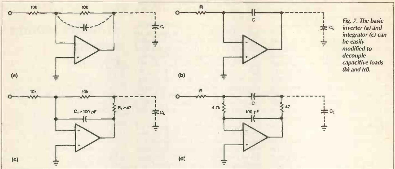
Fig. 7. The basic inverter (a) and integrator (c) can be easily modified to decouple capacitive loads (b) and (d).
