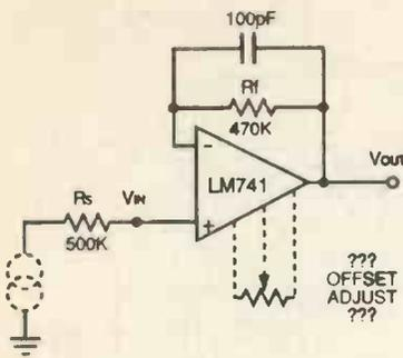
Fig. 1. If you run an op amp at such high impedances that  $I_b \times R$  is more than 20mV, you'll be generating big errors, and a  $V_{offset}$  trim pot can't help you cancel them out. Please don't even try!
