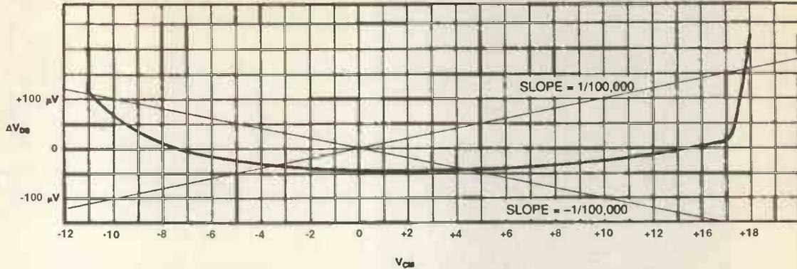
Fig. 2. The CMRR of an op amp can't be represented by a single number. It makes more sense to look at the CMRR curve,  $\Delta V_{OS}$  versus  $\Delta V_{CM}$ , and note its nonlinearities, compared to a straight line with a constant slope of 1 part in 100,000.
