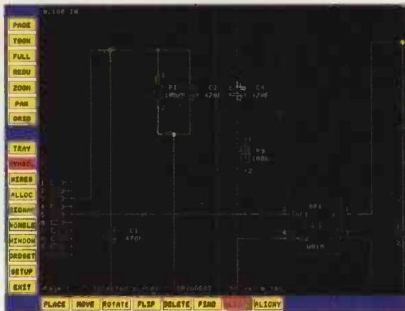
*ALIGN will ensure that components are exactly placed, ready for connecting up.*
