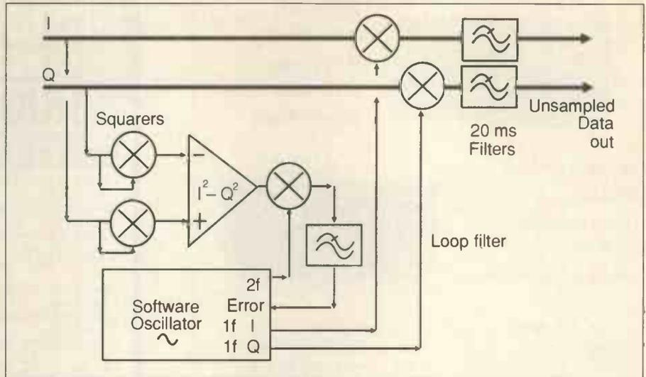
**Fig. 5. Carrier Tracker 2f loop.** The carrier tracker only runs during downloading, and again mimics earlier hardware designs... with the advantage that a software oscillator can output several frequencies and phases, and take phase steps on command.
