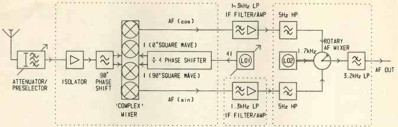
Fig. 4. Receiver block diagram.
