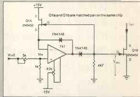
Current at the output of this simple circuit is proportional to the square of the input voltage, for inputs greater than zero. Absolute-value circuit makes it a true squarer.
