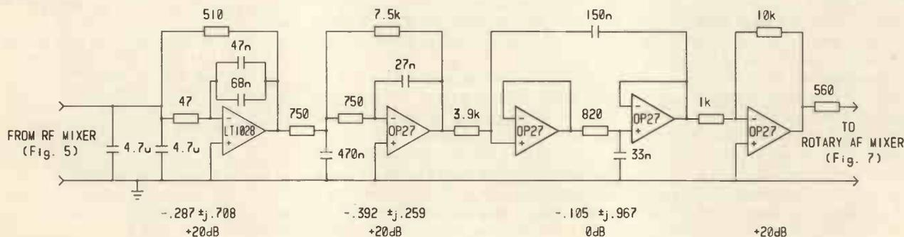
Fig. 6. 1.3kHz low pass IF filter/amplifier stages
