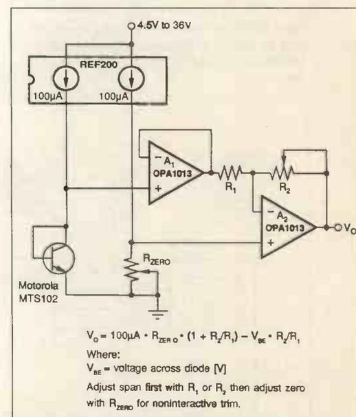
Fig. 4. Combination of Figs. 2 and 3 gives independent control of span and zero and non-inverting output, but uses a single-ended positive supply.
