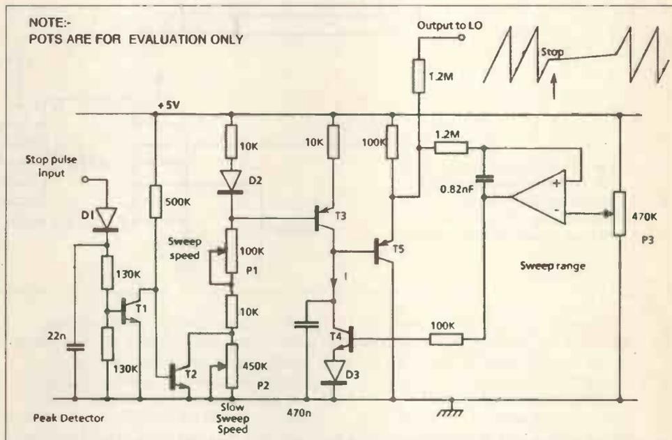
Fig. 2. Ramp generator. Ramp rate set by  $P_1$ , rate in slow section by  $P_2$ . Pulses from stop circuit detected and used to switch capacitor charging current to low level, slowing the ramp.
