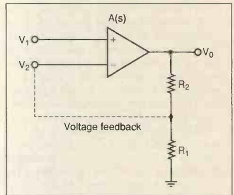
Fig. 1. Standard non-inverting voltage mode op amp, with the location of the closed loop poles being a function of  $G$ .
