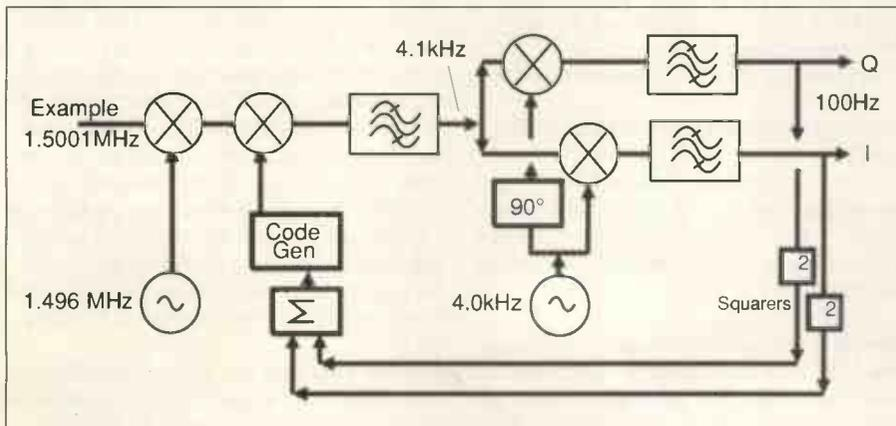
Fig. 4. Downconvert and code track software. Shown as a signal flow diagram, as if it were hardware, the DSP software is very easily understood. This section runs both when downloading and when positioning, the prime output being signal for downloading, and code-phase when positioning.
