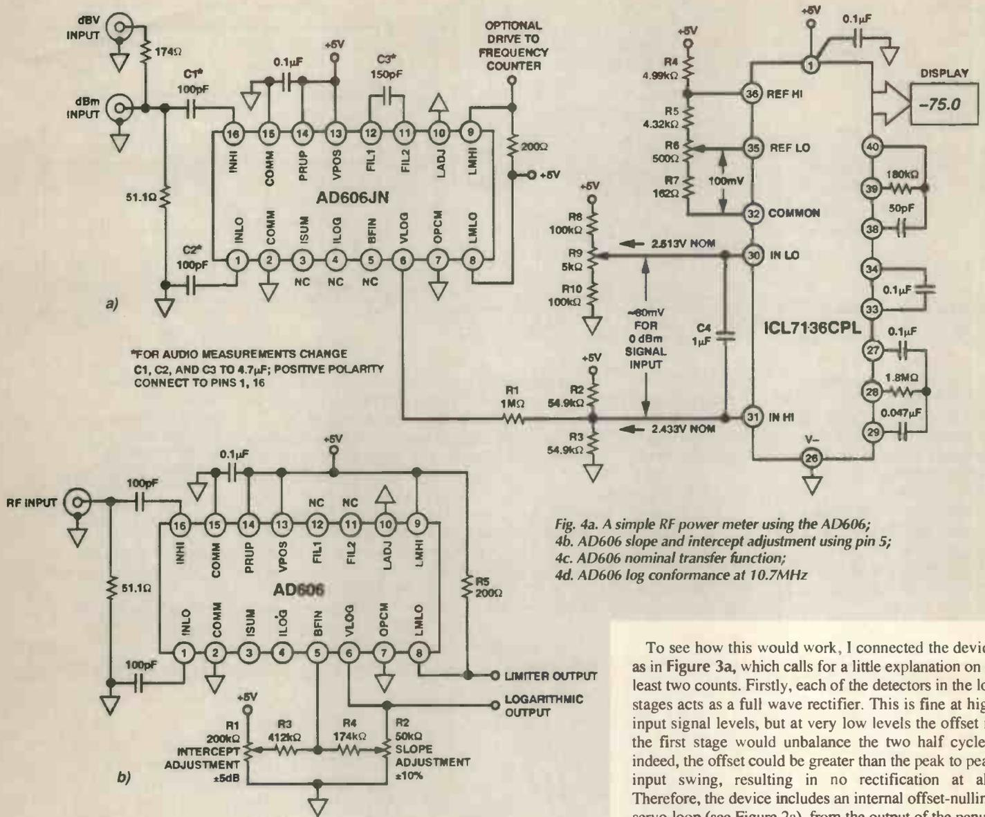
Fig. 4a. A simple RF power meter using the AD606; 4b. AD606 slope and intercept adjustment using pin 5; 4c. AD606 nominal transfer function; 4d. AD606 log conformance at 10.7MHz
