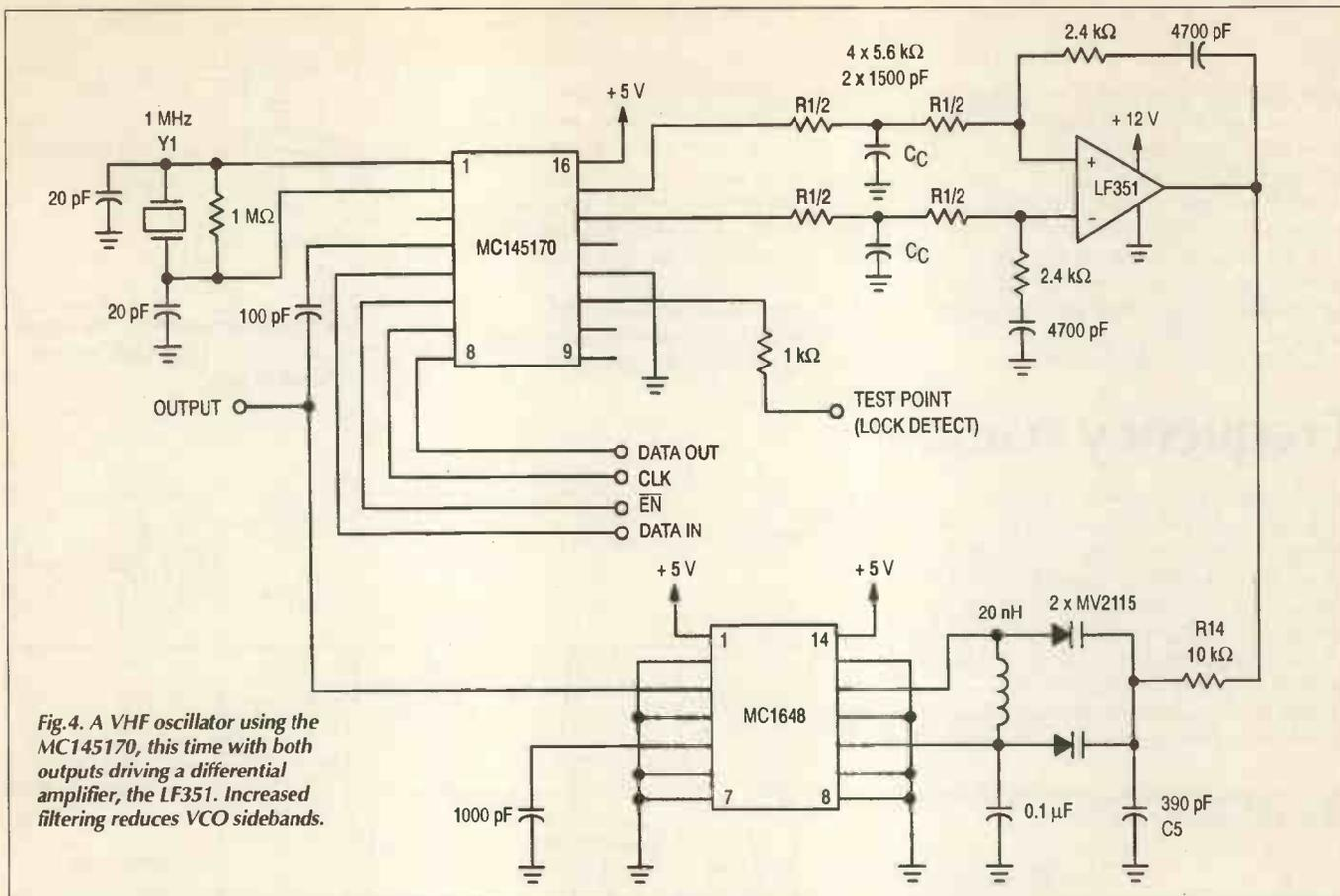
Fig. 4. A VHF oscillator using the MC145170, this time with both outputs driving a differential amplifier, the LF351. Increased filtering reduces VCO sidebands.
