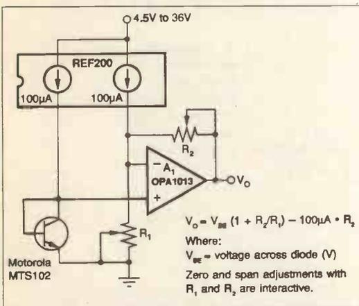
Fig. 1. Half a Burr-Brown OPA1013 dual op-amp, a B-B REF200 current reference and a Motorola MTS102 silicon temperature sensor make up this basic temperature measurement circuit.
