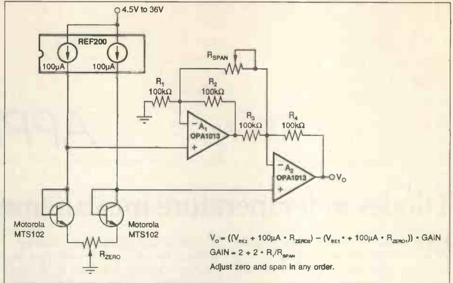
Fig. 5. Differential circuit using both op-amps in the OPA1013.
