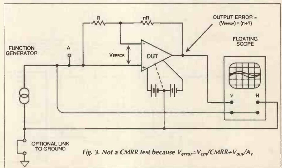
Fig. 3. Not a CMRR test because  $V_{error} = V_{cm}/CMRR + V_{out}/A_v$
