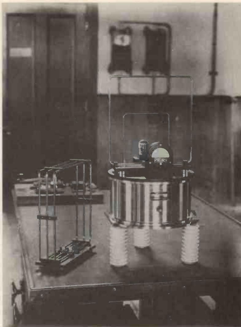
*A standard wave meter, used for checking the transmitted wavelengths.*
