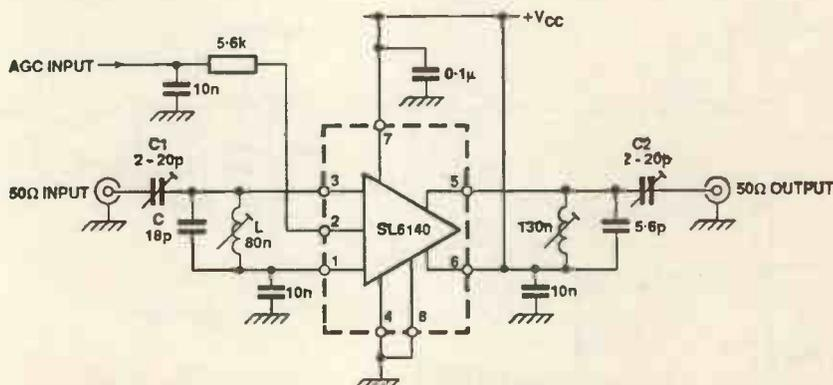
Fig. 1. Tuning input and output of GEC Plessey's SL6140 wide-band amplifier increases its stage gain from 15dB to 35dB, albeit with reduced bandwidth. This is a 100MHz amplifier matched to 50Ω in and out.
