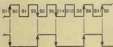
Fig. 1. Input and output waveforms of 2.5 divider. Cycle repeats when starting conditions are repeated.
