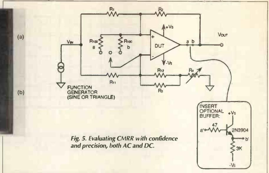
**Fig. 5.** Evaluating CMRR with confidence and precision, both AC and DC.
