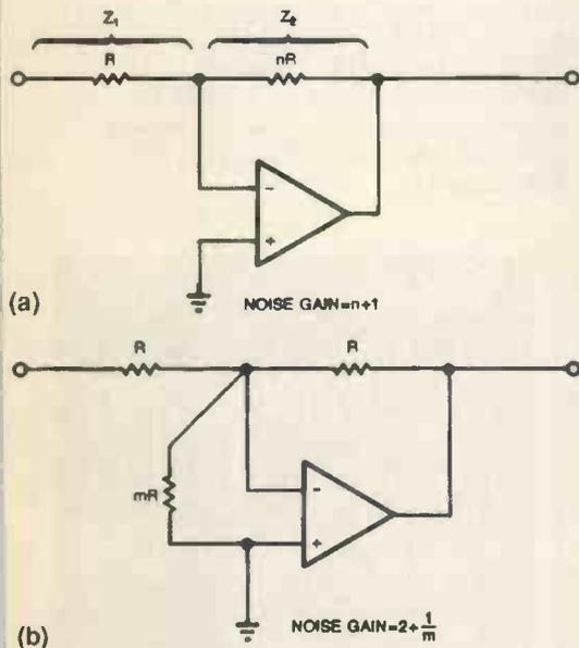
Fig. 8. By adding just a single resistor, the noise gain of a standard integrator can be tailored.
