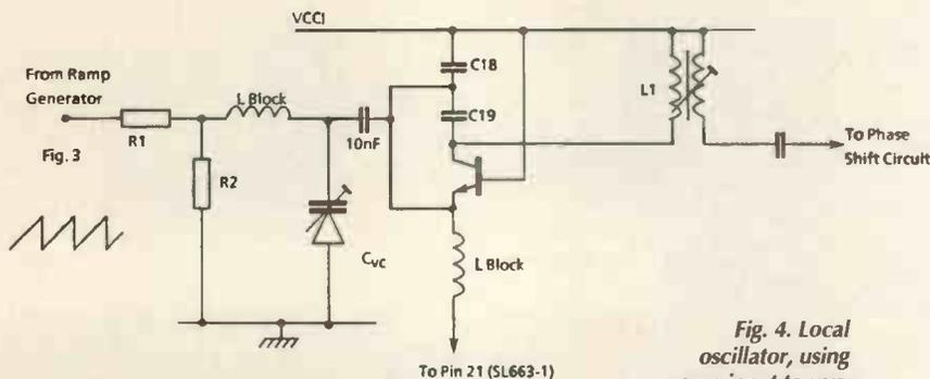
Fig. 4. Local oscillator, using ramp input to vary diode capacitance and therefore tuned frequency.
