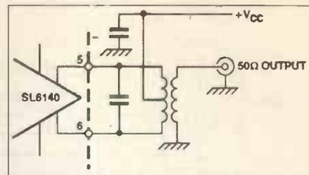
Fig. 2. Using transformer coupling at the output brings the other amplifier output into play and gives another 6dB of gain.
