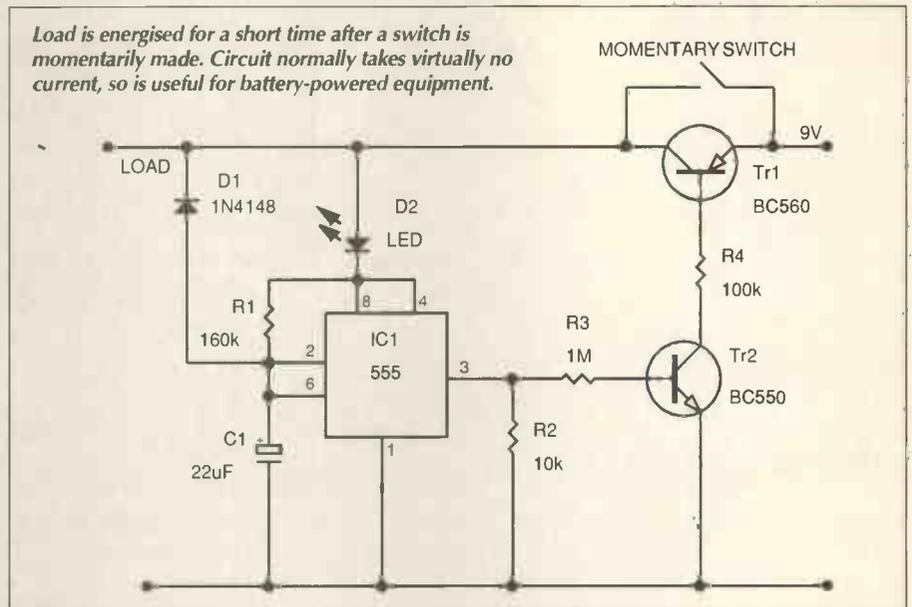
Load is energised for a short time after a switch is momentarily made. Circuit normally takes virtually no current, so is useful for battery-powered equipment.
