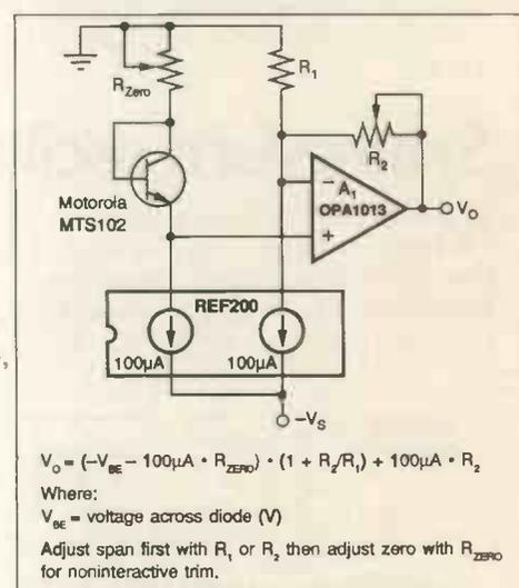
Fig. 3. If temperature-to-voltage inversion is a problem, this arrangement avoids it, but needs a negative power supply line.
