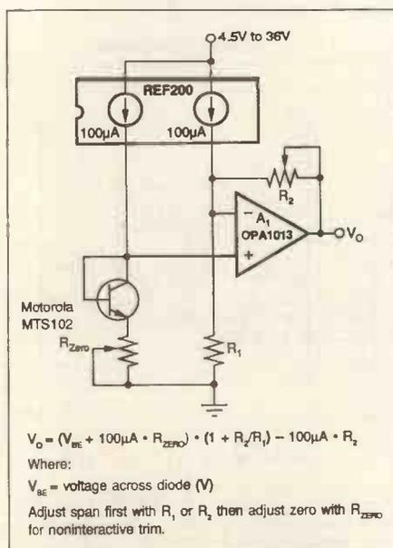
Fig. 2. Addition of  $R_{ZERO}$  avoids interaction of span and zero controls.
