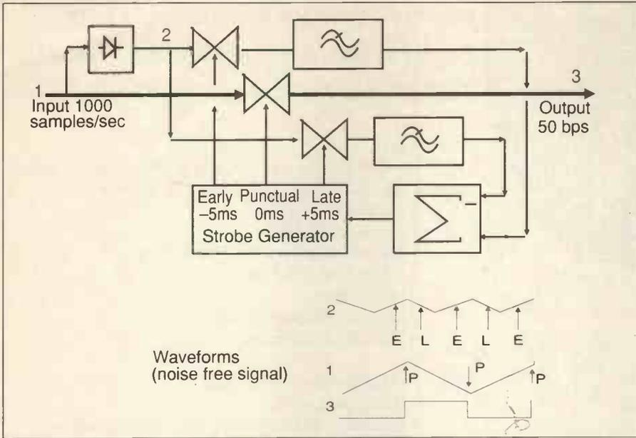
**Fig. 7. Data-bit Extractor.** Data is extracted by detecting the peaks and running a narrow bandwidth PLL to maintain correct sampling. The rectifier removes the data from the tracking channel. Note this is dependent on the integration ramp from the 20ms filter. If the filter were omitted, this would need a differentiator to find edges, which gives very poor noise performance.
