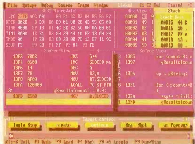
Options displayed under the title "Target Control" when a break point is encountered. Also shown are sections of the two source files, one in the original C and the other in mixed C and assembler.
