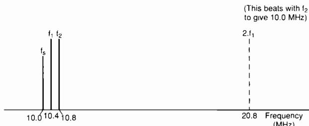
Fig. 6. Close-in third order IMPs that can not be rejected by front-end tuning.
