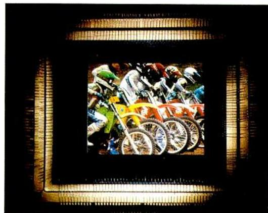
*Microscopic rotatable mirrors fabricated on conventional static ram cells could result in a technology to compete with CRTs. This picture was formed by reflection from the micromirrors.*
