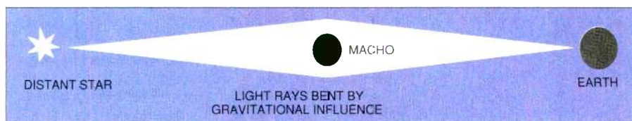
How a macho results in microlensing – and points to the presence of dark matter.
