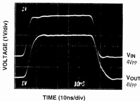
With a differential phase error of 0.01° and a gain error of 0.03%, the MAX405 buffers video up to 180MHz and provides 0.99V/V gain over its full temperature range.
