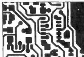
The design, complete with connectivity, can then be translated into the PCB. The connectivity and design rules can be checked automatically to ensure that the PCB matches the schematic.
