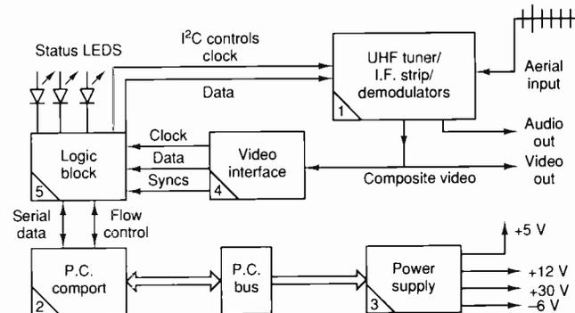
Fig. 1. Essentials of an off-air teletext decoder card for the PC. In addition to feeding teletext data to the PC, the adaptor also makes tv audio and video from the synthesised tuner available. No external power supplies are needed, but some power conditioning is required for comparators and the tuner varicap.
