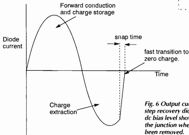
Fig. 6 Output current waveform of the step recovery diode superimposed on a dc bias level showing the snap action of the junction when all the charge has been removed.
