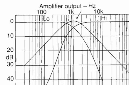
Fig. 4. Output characteristic of final circuit. Amplifier takes part mainly around crossover frequency.
