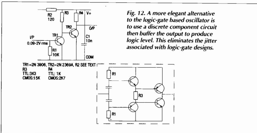
Fig. 12. A more elegant alternative to the logic-gate based oscillator is to use a discrete component circuit then buffer the output to produce logic level. This eliminates the jitter associated with logic-gate designs.
