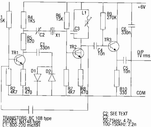
**Fig. 4. At frequencies below 150kHz, equivalent series resistance of a crystal is high so oscillator circuits need to have a high gain.**
