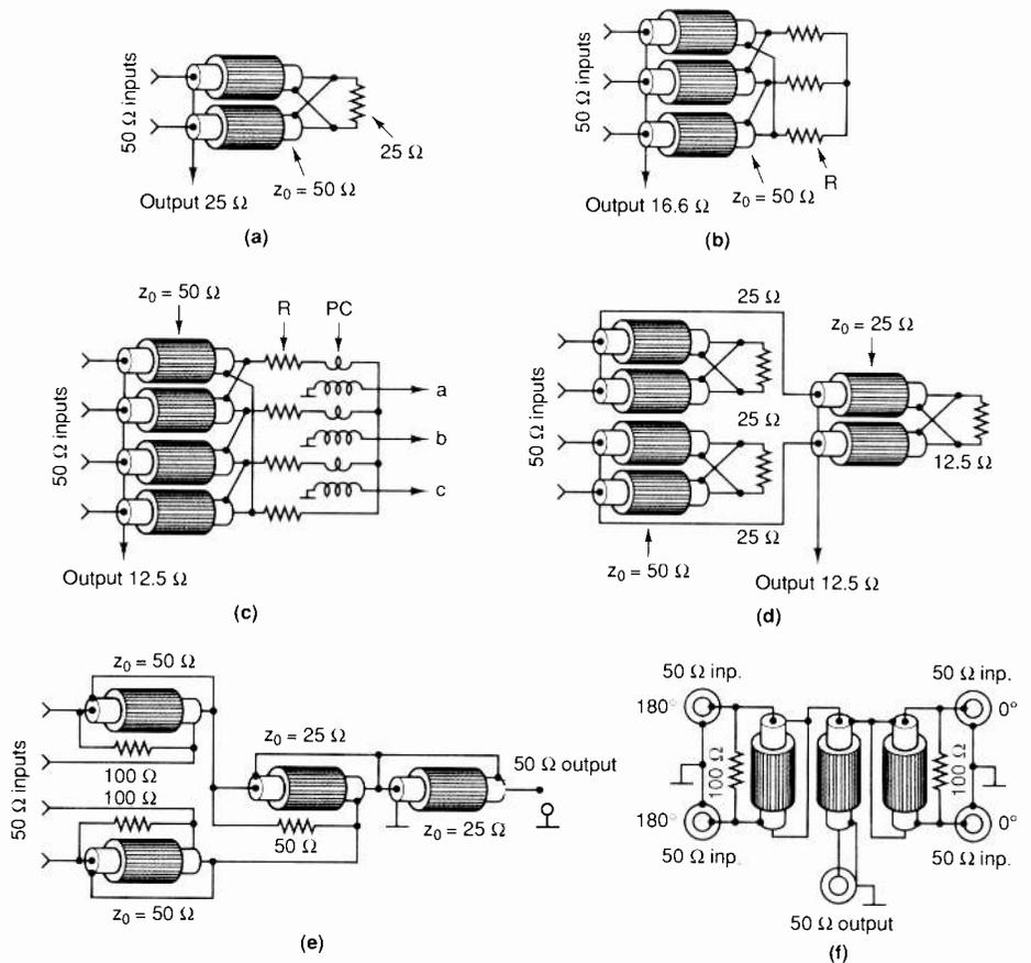
Fig. 1. a), b) and c) represent straight in-phase combiners. Even and odd numbers of input ports are possible with them. d) and e) are staggered or "totem pole" structures, which are adaptable only to even numbers of ports. f) is a 180° combiner that requires no step-up transformer into 50Ω. Note that step-up transformers are not shown for a), b), c) and d).
