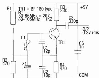
Fig. 8. By driving a crystal into its fifth overtone mode, this oscillator circuit extends useful frequency range to cover 50 to 105MHz.
