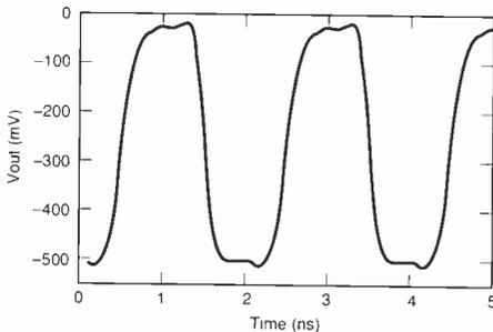
Fig. 9. 12-bit 1GHz digital to analogue converter: output waveform.
