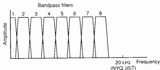
Fig. 4. Spectral segmentation FIR bandpass responses for audio sub-band coding
