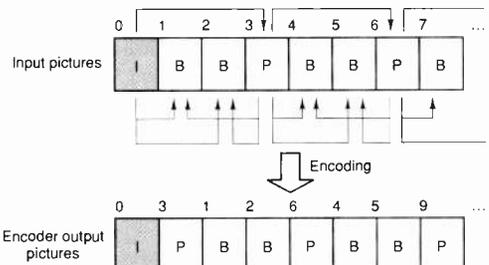
Fig. 12. Video CD picture organisation. Since B frames take longest to encode, output frames are shuffled by the encoder.
