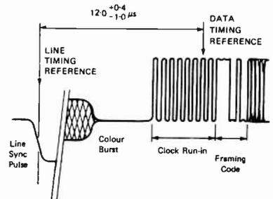
**Fig. 8. Signalling the start of teletext data is a clock synchronisation run in comprising ones and zeroes. Immediately following is framing information that ensures that whatever is decoding the data starts reading it at the first bit of the first byte.**
