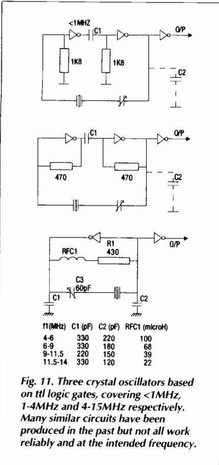
Fig. 11. Three crystal oscillators based on ttl logic gates, covering <math>< 1\text{MHz}</math>, 1-4MHz and 4-15MHz respectively. Many similar circuits have been produced in the past but not all work reliably and at the intended frequency.
