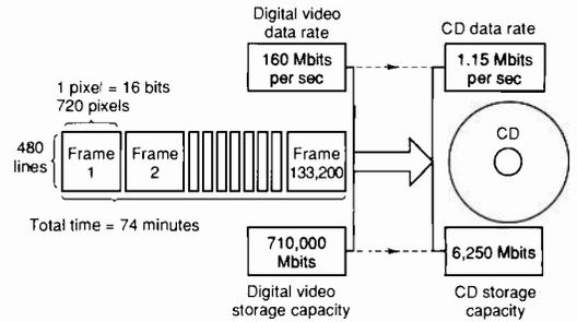
Fig. 2. The video encoding challenge – storing a 710G-bit film on a half-gigabit CD.
