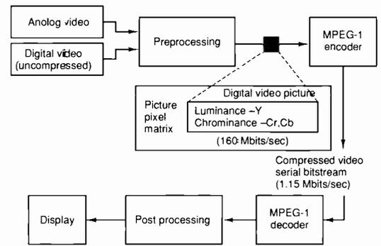
Fig. 3. Video encoding/decoding scheme for the MPEG-1 standard.
