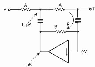
Fig. 3. Resulting lowpass section.
