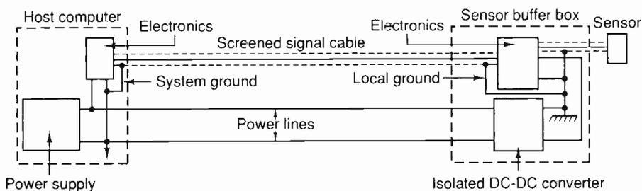
**Fig. 2.** Powering a sensor buffer from a host can cause grounding problems. One solution is to regenerate clean power supplies using isolated dc-to-dc converters within the sensor buffer unit.
