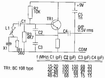
**Fig. 7. Third-overtone crystal oscillator configuration for frequencies from 15 to 63MHz.**
