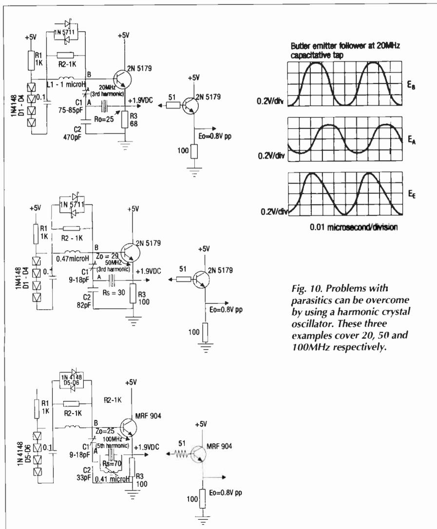
Fig. 10. Problems with parasitics can be overcome by using a harmonic crystal oscillator. These three examples cover 20, 50 and 100MHz respectively.
