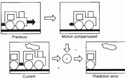
Fig. 10. The image of a moving train need only be stored once, together with a motion vector.
