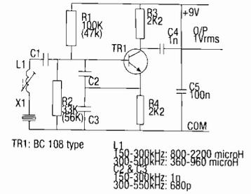
**Fig. 5. Relative to circuitry needed for oscillators working at under 150kHz, this circuit for 150 to 550kHz is much simpler.**
