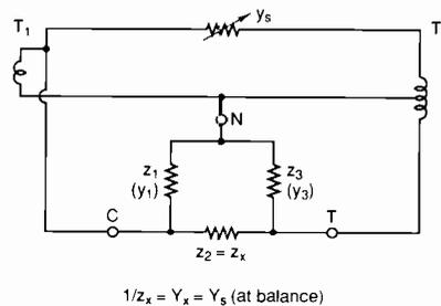
Fig. 3. Circuit showing how a trab is inherently perfectly adapted for three terminal measurements. Admittance  $Y_1$  shunts the source whilst  $Y_3$  shunts the detector ( $T_2$  is a virtual earth). Thus while they may reduce bridge sensitivity slightly, neither affects the accuracy of the measurement of  $Y_2$ .
