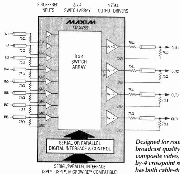
Designed for routing broadcast quality composite video, this 8-by-4 crosspoint switch has both cable-drive buffers and digital control interface.
