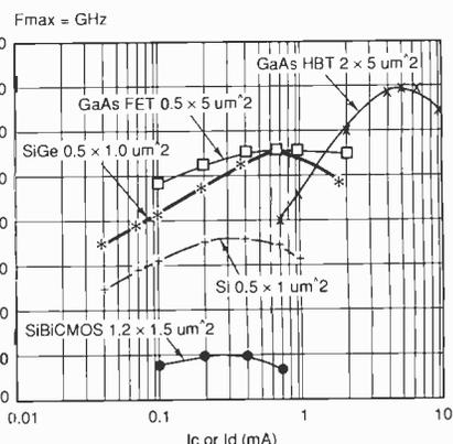
Fig. 4 and 5 show the transition frequency (FT) and maximum oscillation frequency (Fmax) of the SiGe HBTs and compares this to alternative processes.
