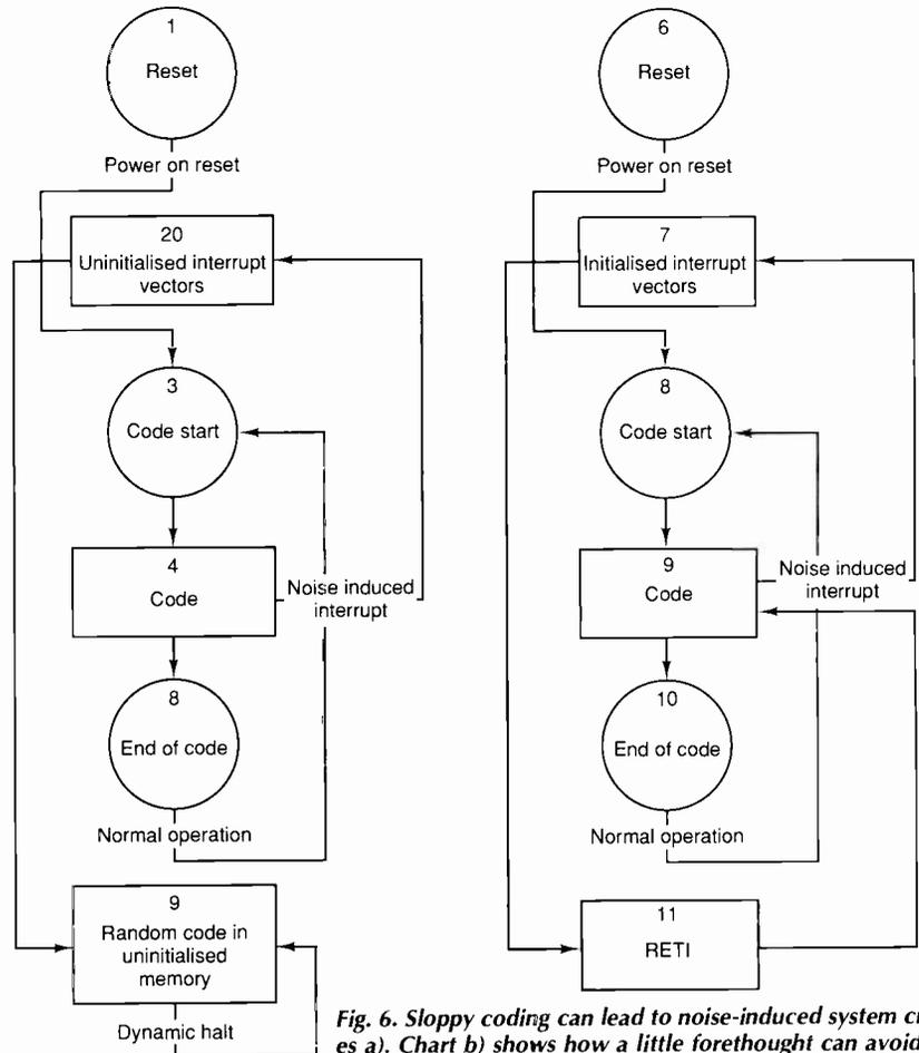
Fig. 6. Sloppy coding can lead to noise-induced system crashes a). Chart b) shows how a little forethought can avoid this problem.
