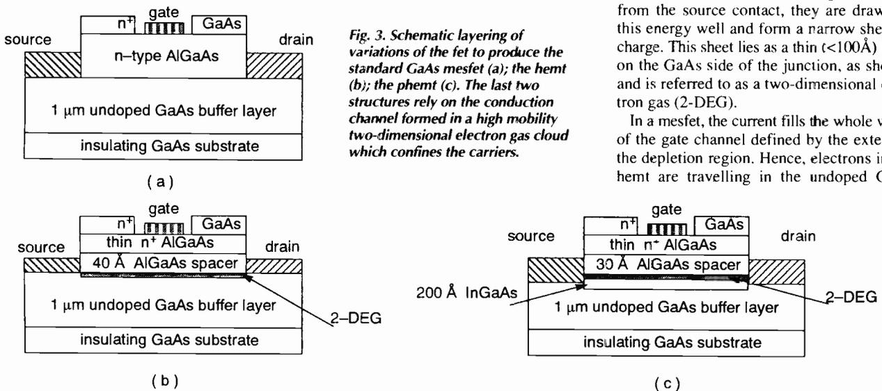
Fig. 3. Schematic layering of variations of the fet to produce the standard GaAs mesfet (a); the hemt (b); the pHEMT (c). The last two structures rely on the conduction channel formed in a high mobility two-dimensional electron gas cloud which confines the carriers.
