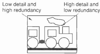
Fig. 4. In video compression, redundancy in individual pictures is exploited.
