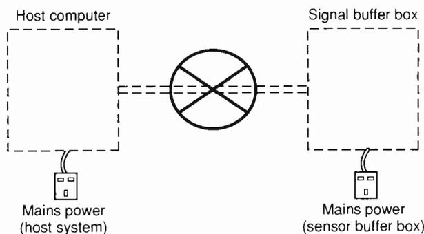
**Fig. 3.** When the host and remote signal buffer have independent mains-derived power supplies, the two are connected via their earths. If the two are also linked by a signal earth ground loops will inevitably cause problems.
