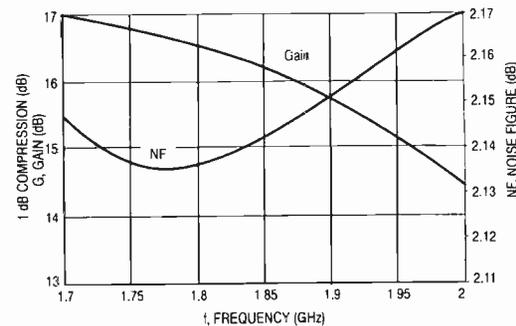
Gain and noise of the 1804 DECT low-noise amplifier versus frequency.
