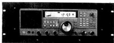
We have taken the synthesised all mode FRG8800 communications receiver and made over 30 modifications to provide a receiver for rebroadcast purposes or checking transmitter performance as well as being suited to communications use and news gathering from international short wave stations.
