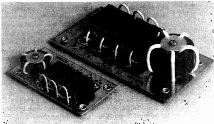
**Fig. 2. Commercial four-port splitter-combiner for use at 1.6-20MHz and power levels up to 1kW. The device is of the type shown in Fig. 1c but the combiner lacks the power pick-up coils. The 50Ω lines are realised by metal tubes with a proper size of insulated conductor threaded through the tube, reducing construction costs. Note the compactness of the units, where the step-up transformer is right next to the combiner structure.**
