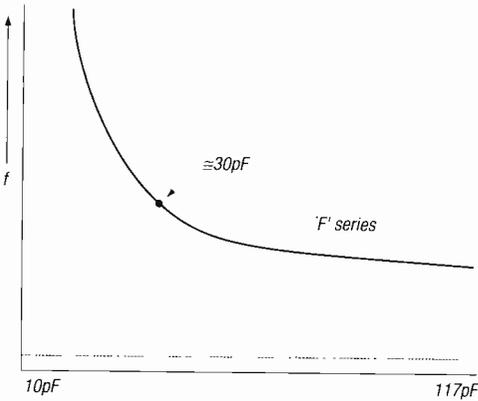
**Fig. 2. Lowering capacitive loading on a crystal increases its output frequency.**
