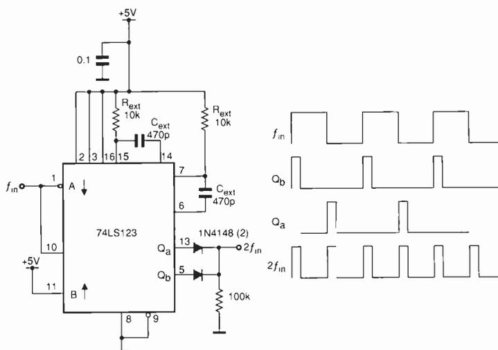
TTL pulse-frequency doubler for operation up to about 2.5MHz with a pulse width of 350ns minimum.
