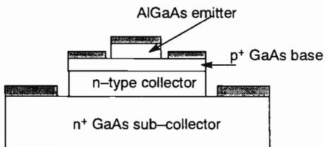
Fig. 4. Structure of the heterojunction bipolar transistor. The key to its high frequency and low noise performance lies in the AlGaAs layer and the high doping possible of the base region.
