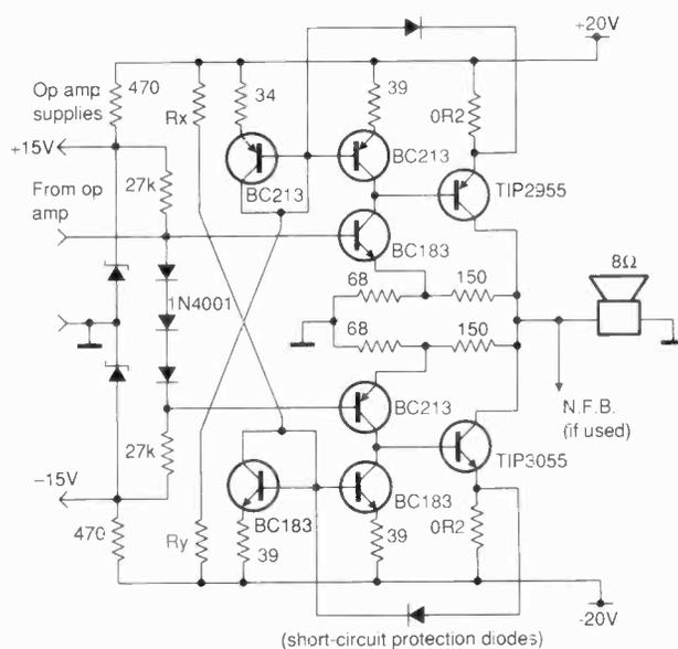
Silicon audio power output stage, using current drive to the output transistors and needing no bias adjustment.
