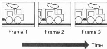
Fig. 5. There is also redundancy in sequences of pictures that can be removed to save memory.
