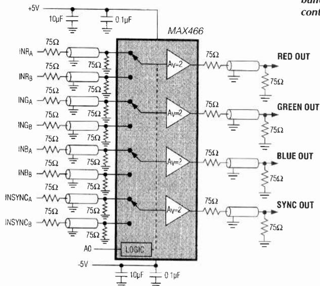
The MAX466, intended for switching between two RGB-plus-sync sources, has 100MHz 6dB buffer amplifiers capable of driving ±2V into a 75Ω load.
