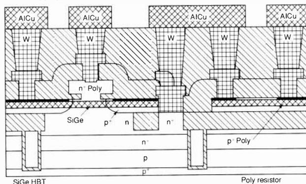
Fig. 3. The structure of an SiGe HBT
