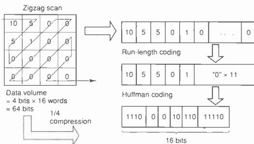
Fig. 8. Variable-length coding involves scanning the pattern in a zig-zag to produce a bit stream.
