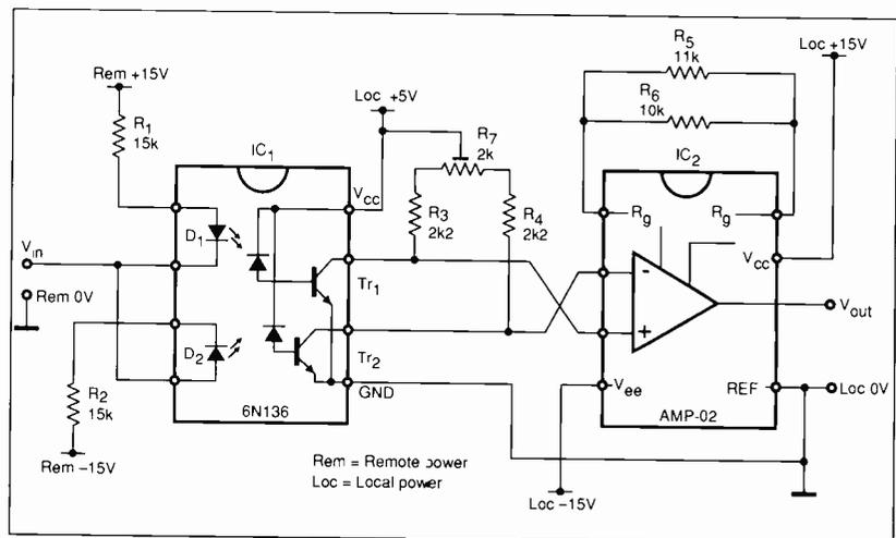
Low-cost, but linear and wide-band, optically isolated amplifier. Running leds differentially cancels out errors.
