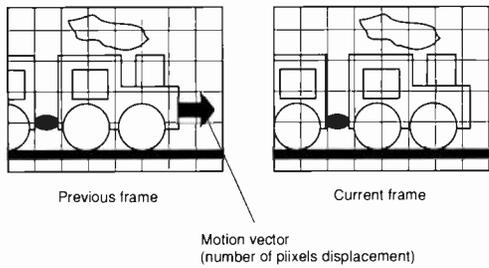
Fig. 9. Further compression is possible by analysing motion over successive frames.
