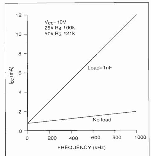
*Current versus frequency for the UCC1570 pwm controller while in operating mode shows that little current is needed to operate the device – even at high switching speeds and with high mosfet gate capacitance.*
