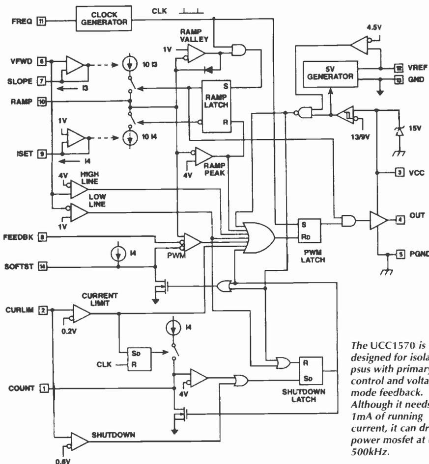
*The UCC1570 is designed for isolated psus with primary-side control and voltage-mode feedback. Although it needs only 1mA of running current, it can drive a power mosfet at up to 500kHz.*
