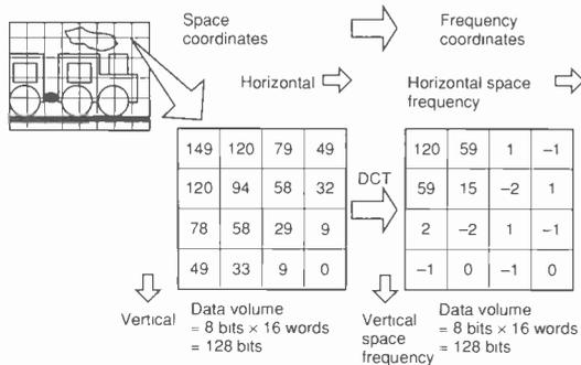
Fig. 6. The process used to sort out redundant data is known as discrete cosine transform, or dct.
