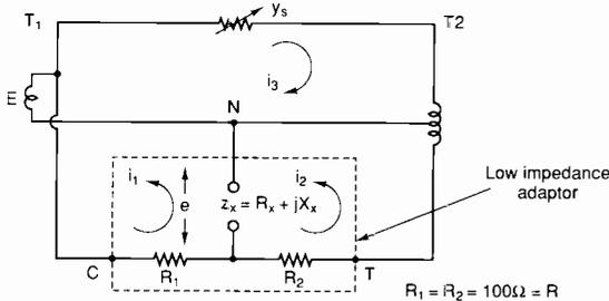
Fig. 4. Showing how a low impedance adaptor not only extends the measurement range of a trab, but also turns conductance into resistance, and capacitive susceptance into inductive reactance and vice versa.
