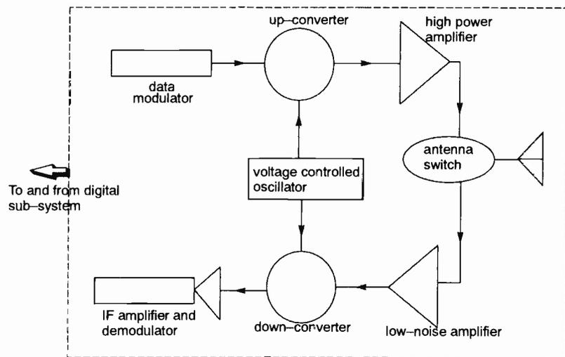
Fig. 2. Typical rf section of a PCS communicator. Different technologies are being used to produce highly optimised devices for each of the major components.
