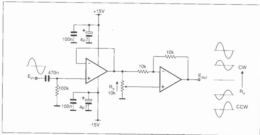
Potentiometer  $R_v$  varies output from inverted to non-inverted version of the input at unity gain.
