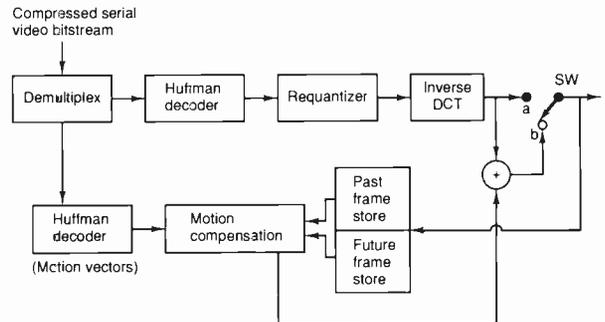
Fig. 14. In the player, a switch routes data depending on whether the disc is audio or video.
