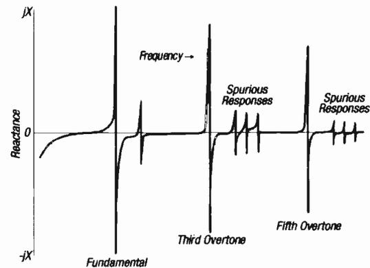
Fig. 1. Operating a crystal at an overtone of its fundamental is tricky. The oscillator circuit needs to be carefully designed to make sure that the spurious response points have no influence on the final output signal.
