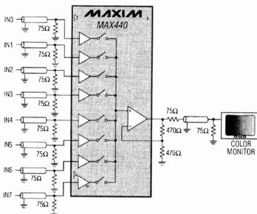
Useful in applications such as selecting surveillance camera sources, the MAX440 eight-way switch has pin-selectable frequency compensation and operates to 160MHz.
