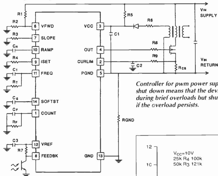
*Controller for pwm power supplies. Fault-counting shut down means that the device stays operational during brief overloads but shuts down completely if the overload persists.*
