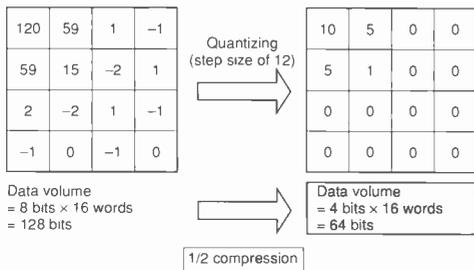
Fig. 7. Here, quantizing the dct components involves scaling down by a factor of 12.
