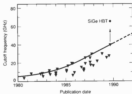
Fig. 1. Trends in cut off frequency. SiGe is a huge leap in speed over the fastest Si transistors reported.
