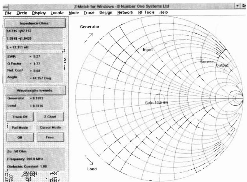
**Fig. 1.** Z-Match for Windows displays its power with a complicated Smith chart, showing stability and gain circles. Note the cross-shaped cursor over the point marked Source; the panel at the left of the screen displays a range of information about the cursor location, including its absolute and normalized impedance. Quick-change buttons control the most used features of the chart.
