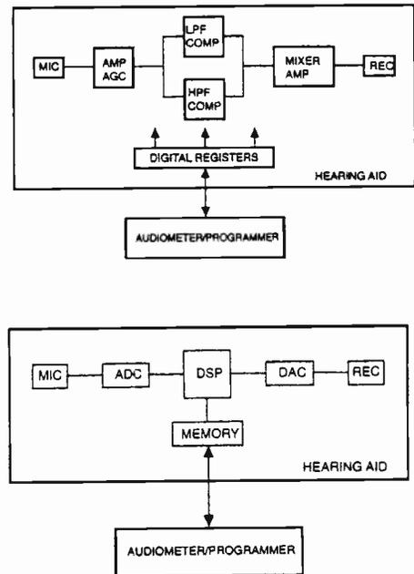
*Top – multichannel hearing aid pushing current hearing aid design to its limits. Bottom – dsp design could open up new possibilities for people with hearing impairments.*
