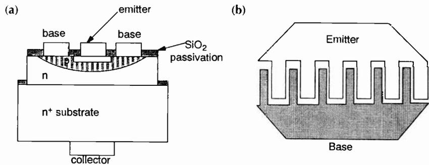
Fig. 1. Basic structure of the silicon bipolar transistor (a) with (b) the general type of interdigitated emitter which allows the current to be increased without a corresponding increase in capacitance.
