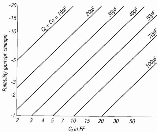
**Fig. 3. When estimating how far a crystal's frequency can be pulled by changing its load capacitance,  $C_L$ , both package shunt capacitance,  $C_0$ , and motional capacitance  $C_1$  need to be taken into account.**
