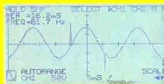
Display of signal shape lets you find faults that DMM can not show.
