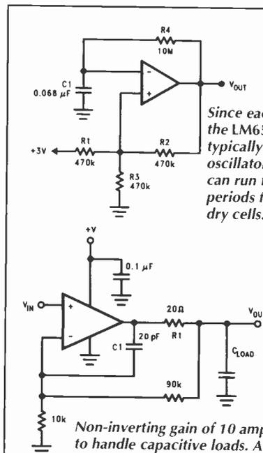
Since each op-amp in the *LM6572* consumes typically 40µA, a 1Hz oscillator such as this can run for long periods from two small dry cells.
