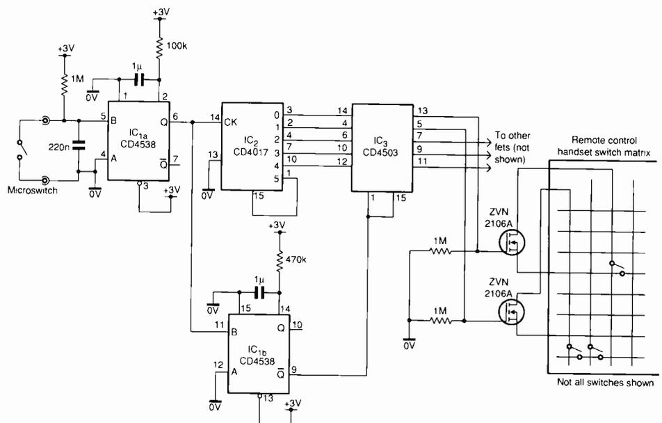
Disabled person's tv controller adaptor, operated by microswitch to step through channels and standby.
