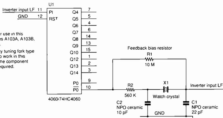
4.194304 MHz at cut timing crystal circuit
