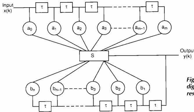
Fig. 3. Elements of a digital finite-impulse response filter.
