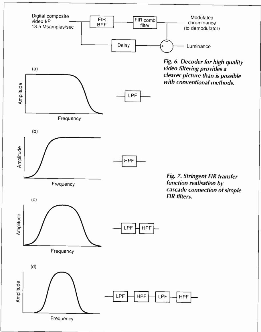
Fig. 6. Decoder for high quality video filtering provides a clearer picture than is possible with conventional methods.
