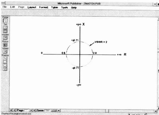
**A) One way to represent all practicable impedances  $R \pm jX$  on two rectangular axes. All combinations of resistance and reactance that have a normalized voltage standing wave ratio of 2.0 will fall on the constant-VSWR circle. To transform this diagram into a Smith chart Figure B, bend the two reactance axes round so that all three "infinity" points meet at the right-hand end of the resistance axis.**
