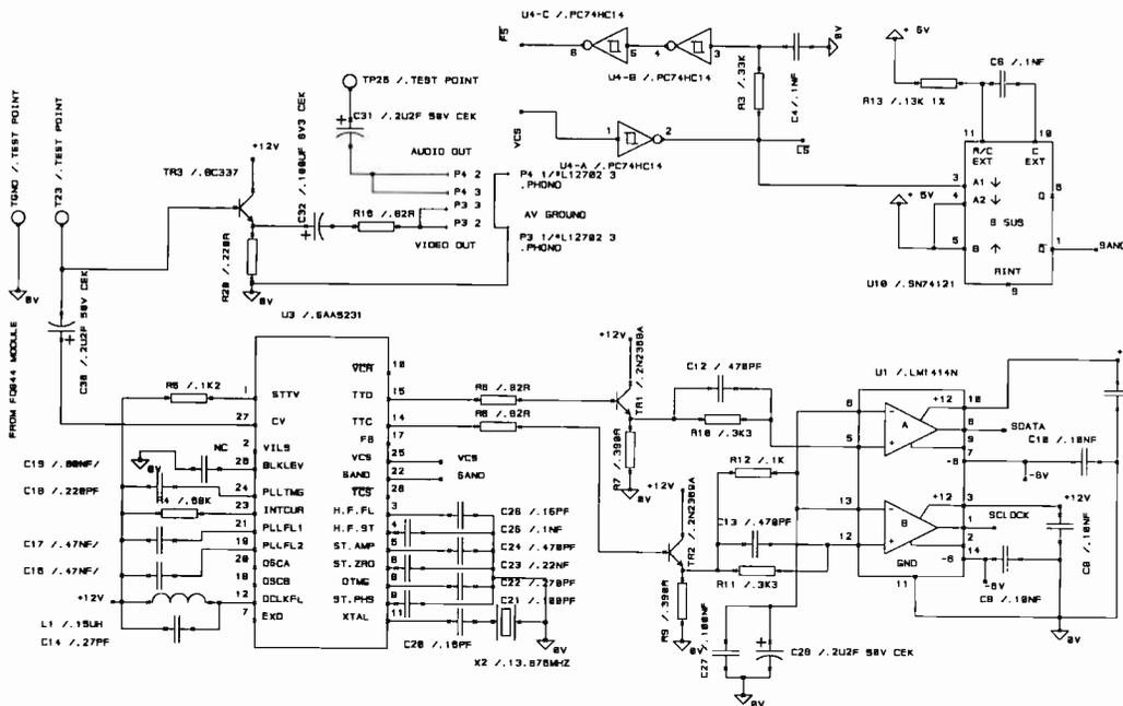
Fig. 3. Teletext information is separated from raw video by an SAA5231 data slicer. Off-air composite video appears at pin 27 while sync pulses are presented at pin 25.
