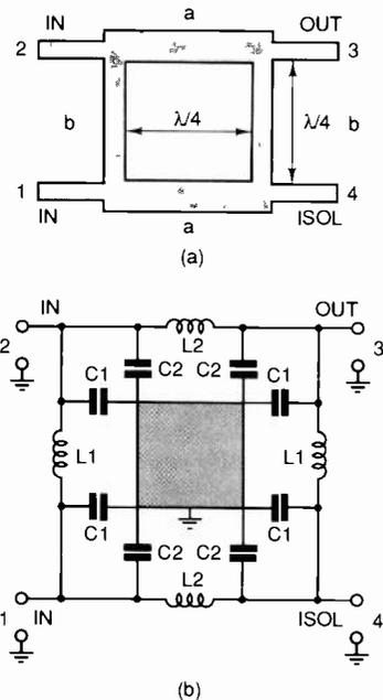
Fig. 5. The branch line hybrid (a) and its lumped equivalent (b). As in the ring hybrid equivalent, the paralleled capacitors (C1 and C2) can be combined into single units.
