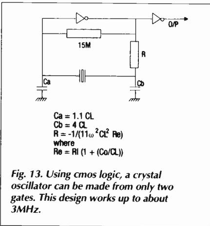
Fig. 13. Using cmos logic, a crystal oscillator can be made from only two gates. This design works up to about 3MHz.
