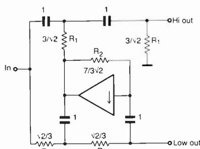
Fig. 1. Low-level crossover circuit with values normalised to  $\omega=1$ , components in ohms and farads.
