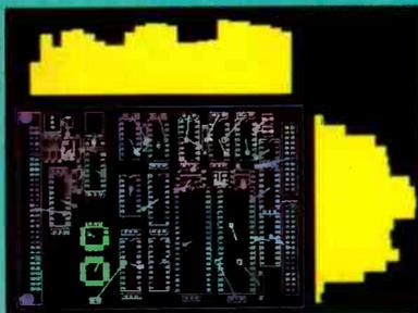
ULTIshell, the integrated user interface, makes sure all your design information is transferred correctly from ULTIcap to ULTIboard. Good manual placement tools are vital to the progress of your design, therefore ULTIboard gives you a powerful suite of REAL-TIME functions such as, FORCE VECTORS, RATS NEST RECONNECT and DENSITY HISTOGRAMS. Pin and gate swapping allows you to further optimise your layout.
