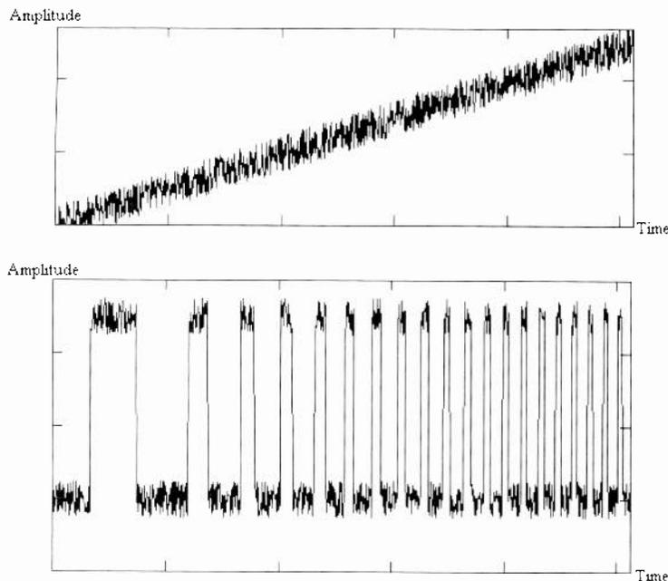
*Fig. 5. In a purely analogue system, the ramp's detail is obscured by noise. Converting the clean ramp to frequency-modulated format reduces the effects of noise.*
