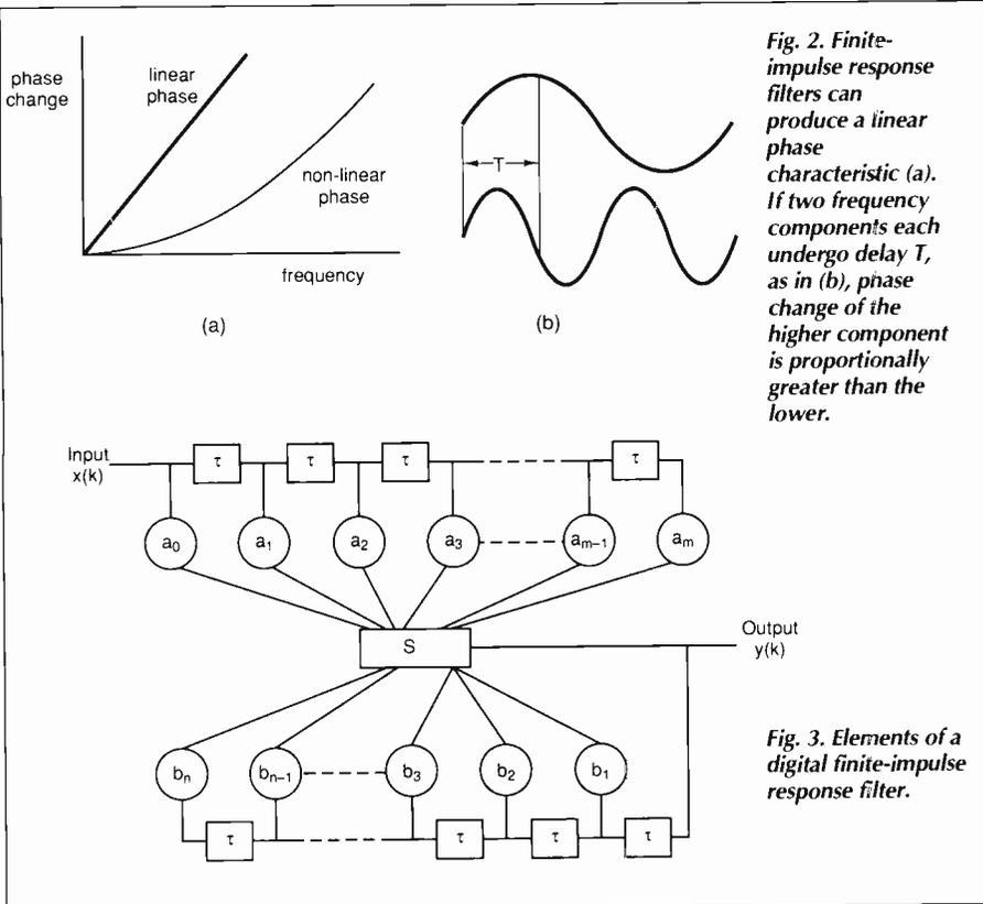
Fig. 2. Finite-impulse response filters can produce a linear phase characteristic (a). If two frequency components each undergo delay T, as in (b), phase change of the higher component is proportionally greater than the lower.
