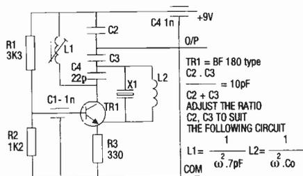
Fig. 9. Above 105MHz, stray capacitances make designing a reliable oscillator difficult. To help prevent oscillation not controlled by the crystal, this circuit uses a small inductor in parallel with the crystal to tune out its static capacitance.
