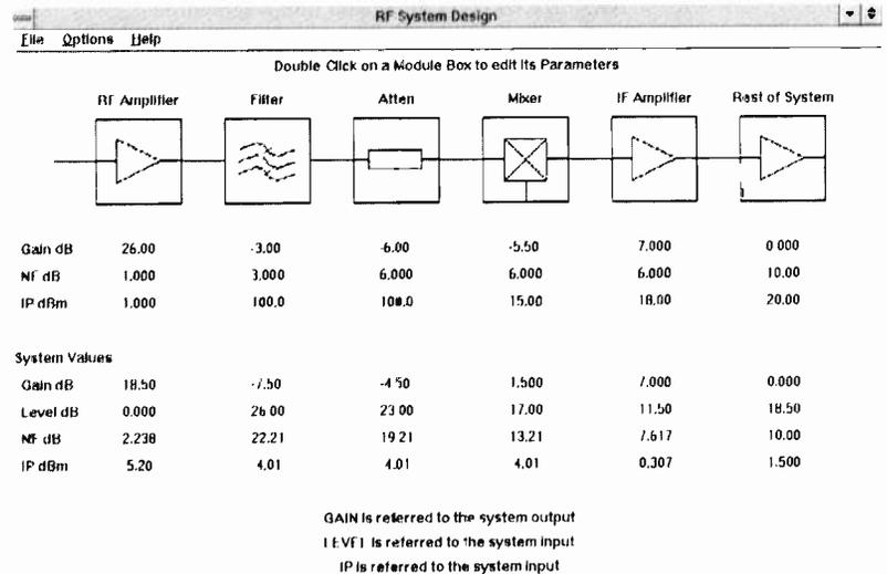
*Fig. 2. The receiver noise figure and intermodulation calculator from the rf Tools menu. The top three rows of data refer to the individual modules in the block diagram drawn above. The bottom four rows show how the cascaded stages interact to produce the overall system performance. Double-click on any module box to alter its data, and the whole display is automatically recalculated.*
