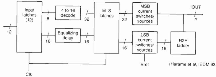
Fig. 8. 12-bit 1GHz digital to analogue converter: block diagram.
