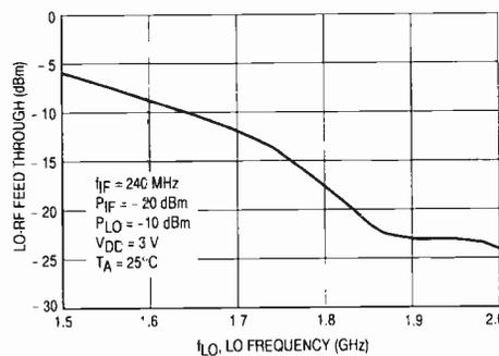
Local oscillator versus rf feedthrough for the 1803 1.8GHz up-converter.
