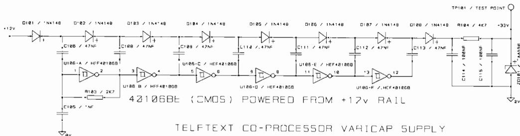
**Fig. 5. Voltage multiplier used to supply the synthesized tuner's varicap. The free-running oscillator on the left feeds the multiplier chain, producing around 50V on the right. Following current limiting, a shunt zener produces a stable 30V varicap feed.**
