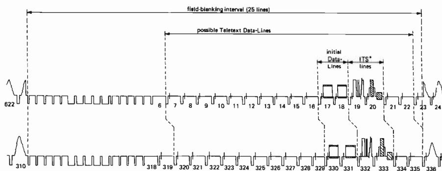
**Fig. 6. Broadcast teletext data streams appear in up to 16 lines per tv frame, all within the blanking period. Data is transmitted at 6.9375Mbit/s.**
