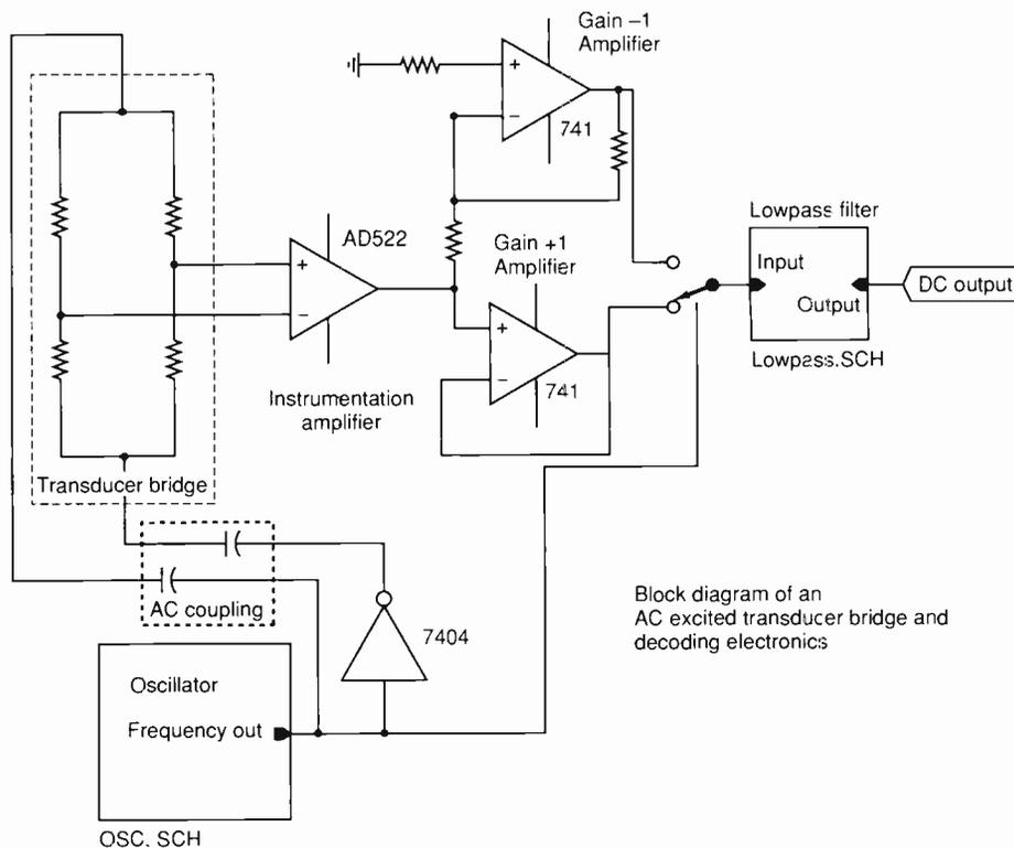
**Fig. 4.** With certain types of transducer, noise problems can be reduced by exciting the sensor with an ac signal. At the receiving end, a frequency-selective amplifier driven by the exciter clock makes sure that unwanted signals are rejected.
