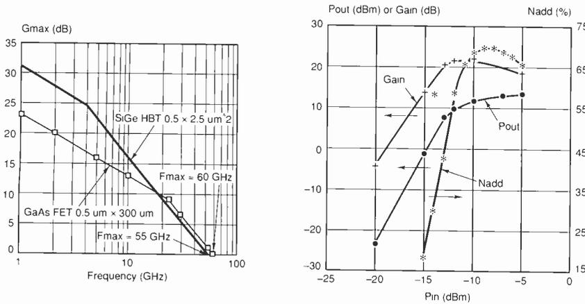
Fig. 6 and 7 show the gain and efficiency of the SiGe HBTs and compares this to alternative processes.
