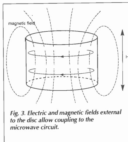
**Fig. 3.** Electric and magnetic fields external to the disc allow coupling to the microwave circuit.
