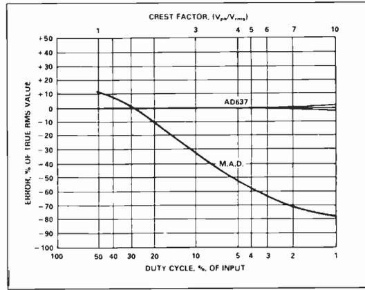
**Fig. 4. Error versus duty cycle for an MAD ac detector and AD637-based converter.**
