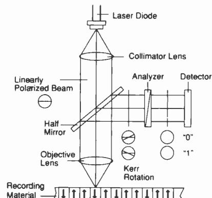
**In a magneto-optical rewritable disk, polarity of the magnetic bit region can only be changed while the area is heated by a laser.**
