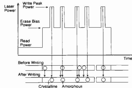
**Similar to worm disks, phase-change rewritable types have amorphous and crystalline areas but the crystalline areas formed by melting can be reversed by heating to just below their melting point.**
