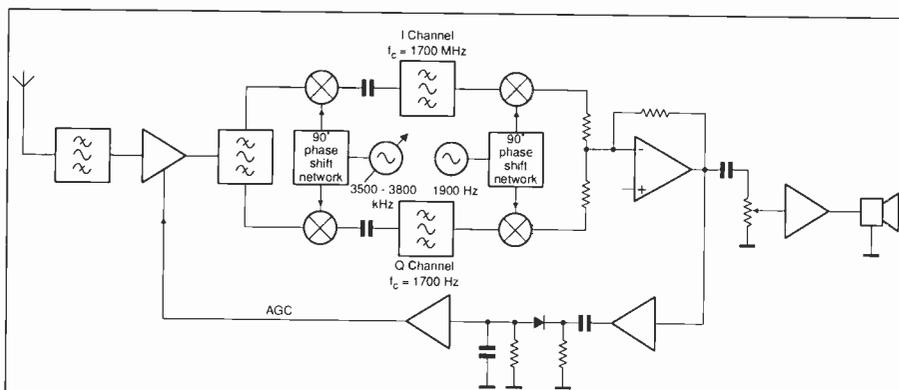
*Receiver block diagram. Most of the circuitry is divided between five separate modules: rf amplifier and dual first mixers; 2-phase rf oscillator; dual 7-pole low-pass filters; dual second mixers, audio amplifier and agc circuit; two-phase second oscillator.*
