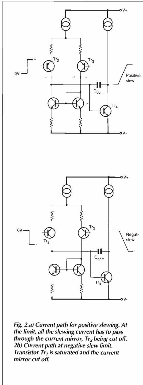
Fig. 2.a) Current path for positive slewing. At the limit, all the slewing current has to pass through the current mirror,  $Tr_2$  being cut off. 2b) Current path at negative slew limit. Transistor  $Tr_1$  is saturated and the current mirror cut off.
