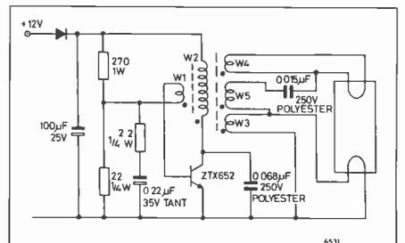
Fig. 3. Inexpensive 8W fluorescent lamp inverter operates efficiently from supplies between 10 and 16.5V.
