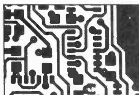
The design, complete with connectivity, can then be translated into the PCB. The connectivity and design rules can be checked automatically to ensure that the PCB matches the schematic.
