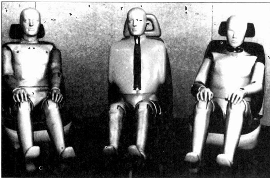
*Dummies with intelligent heads. An element of a new range of crash-test dummies from Vector Research is a new magnetohydrodynamic sensor from Endevco. It measures angular rate to help in the assessment of head injury criteria.*
