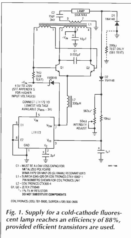
Lamp intensity is continuously and smoothly variable from zero to full intensity. When power is applied, the *LT1172* switching regulator's feedback pin is below the device's internal 1.2V reference. This causes full duty cycle modulation at the  $V_{SW}$  pin. Fig. 2, trace A., Inductor  $L_2$  conducts current, trace B, which flows from  $L_1$ 's centre tap, through the transistors, into  $L_2$ . This inductor's current is deposited in switched fashion to ground by the regulator's action.
