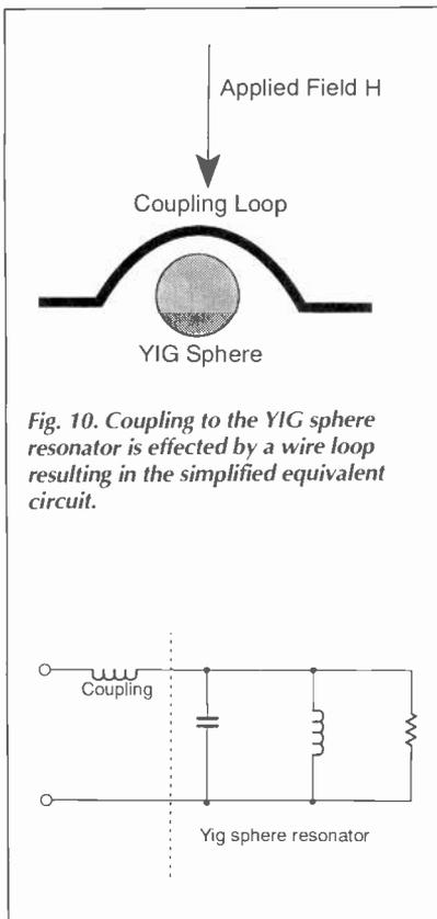
Fig. 10. Coupling to the YIG sphere resonator is effected by a wire loop resulting in the simplified equivalent circuit.
