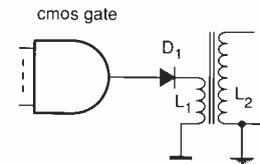
Fig. 2. An alternative to the mosfet switch in Fig. 1.
