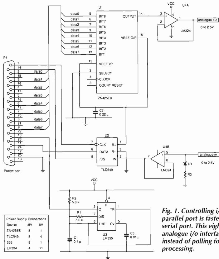
**Fig. 1. Controlling i/o via the PC parallel port is faster than using the serial port. This eight-bit resolution analogue i/o interface uses interrupts instead of polling for more efficient processing.**
