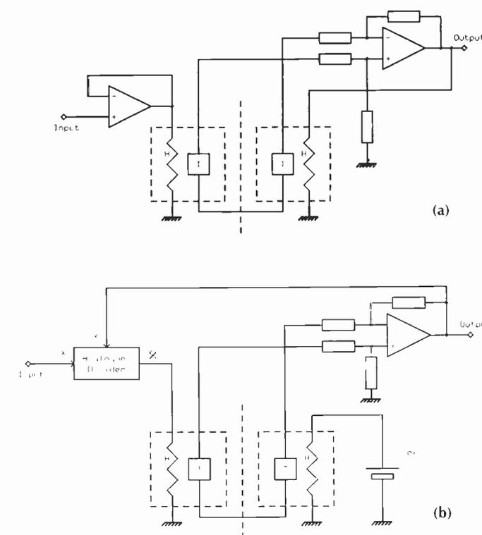
*Fig. 1a). Deriving the rms value of a signal using two heater-sensor combinations. A DC voltage applied to a resistor produces exactly the same amount of heat as its equivalent in rms. b). Dynamic range of the thermal converter is improved by adding analogue divider.*
