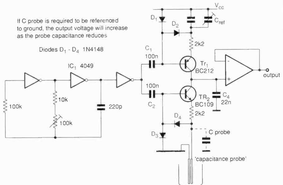
Capacitive level detector provides analogue indication.
