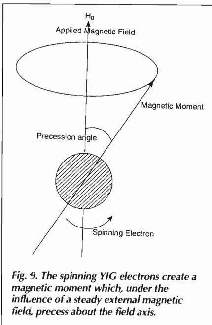
Fig. 9. The spinning YIG electrons create a magnetic moment which, under the influence of a steady external magnetic field, precess about the field axis.
