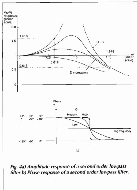
Fig. 4a) Amplitude response of a second order lowpass filter b) Phase response of a second order lowpass filter.
