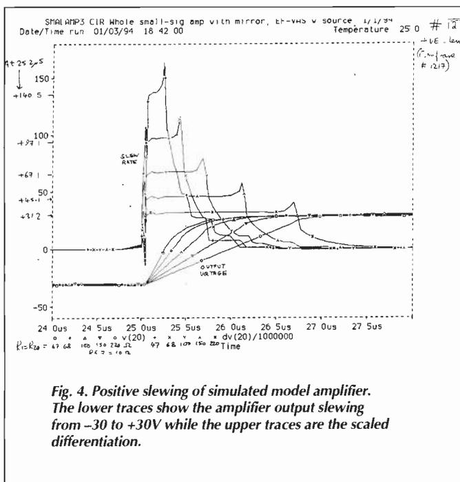
**Fig. 4. Positive slewing of simulated model amplifier.** The lower traces show the amplifier output slewing from -30 to +30V while the upper traces are the scaled differentiation.
