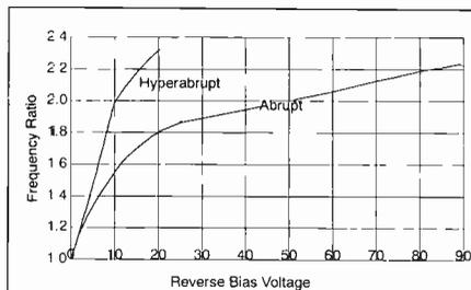
Fig. 8. Tuning curves of theoretical frequency ratio for a hyperabrupt and abrupt junction varactor
