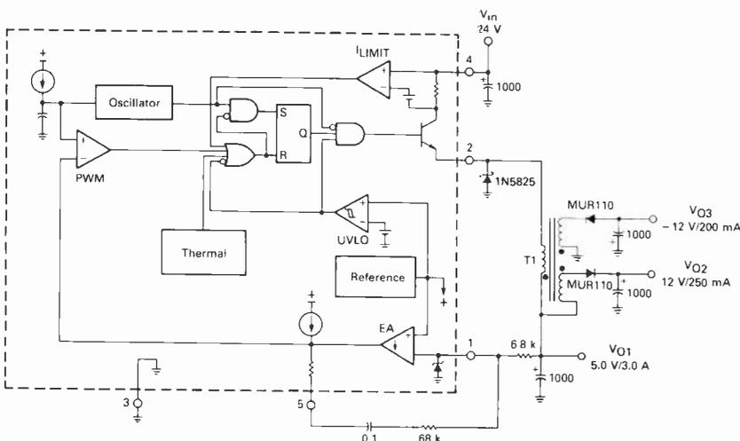
*Triple-output converter. Multiple auxiliary outputs are easily derived by winding secondaries on the main output inductor. These must be connected so that the energy is delivered to the auxiliary outputs when the switch output turns off. During the off time, voltage across the primary is regulated by the feedback loop, yielding a constant volts/turn ratio. The number of turns for any given secondary voltage can be calculated by:*
