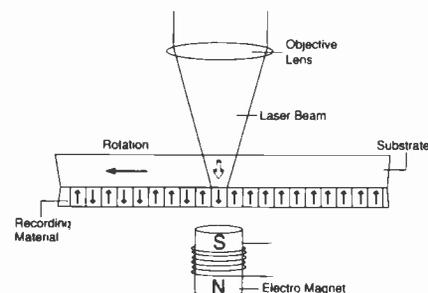
temperature however, polarity of a magnetic domain can be easily changed by an external magnetic field. Wherever a data bit is to be recorded, a high powered laser beam is used to heat the material above this temperature, allowing this reversal to take place.
