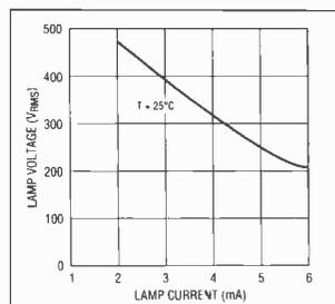
Fig. 8. Current versus voltage for a lamp in its operating region.
