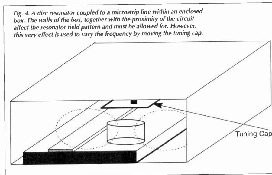
**Fig. 4.** A disc resonator coupled to a microstrip line within an enclosed box. The walls of the box, together with the proximity of the circuit affect the resonator field pattern and must be allowed for. However, this very effect is used to vary the frequency by moving the tuning cap.
