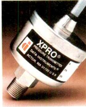
**Pressure sensor.** Pressure sensors in Control Transducers's *XPRO* range are moisture-proof, water-resistant, in a stainless-steel body with invulnerability to shock and vibration. Built-in amplifiers give a conditioned output of 5V or 4-20mA, driving controls or indicators without extra amplification. Accuracy is better than 1% due to all causes and the range includes 1bar-13.8bar in absolute scaling and in sealed gauge up to 490bar. Control Transducers. Tel., 0234 217704; fax, 0234 217083.
