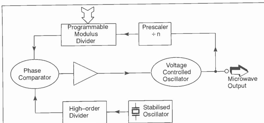
**Fig. 1.** A practical form of microwave frequency synthesiser uses a fundamental VCO in a phase locked loop. The loop incorporates high frequency dividers, one having a programmable modulus.
