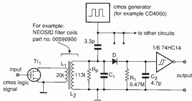
Fig. 1. While providing effective logic isolation, this inductive circuit consumes about 2000 $\times$  less power than an opto-isolator.
