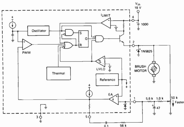
This variable motor speed controller incorporates emf feedback sensing. For any supply from 12 to 24V, line regulation is 1% measured at 1760rev/min, and 6% at 3260rev/min.
