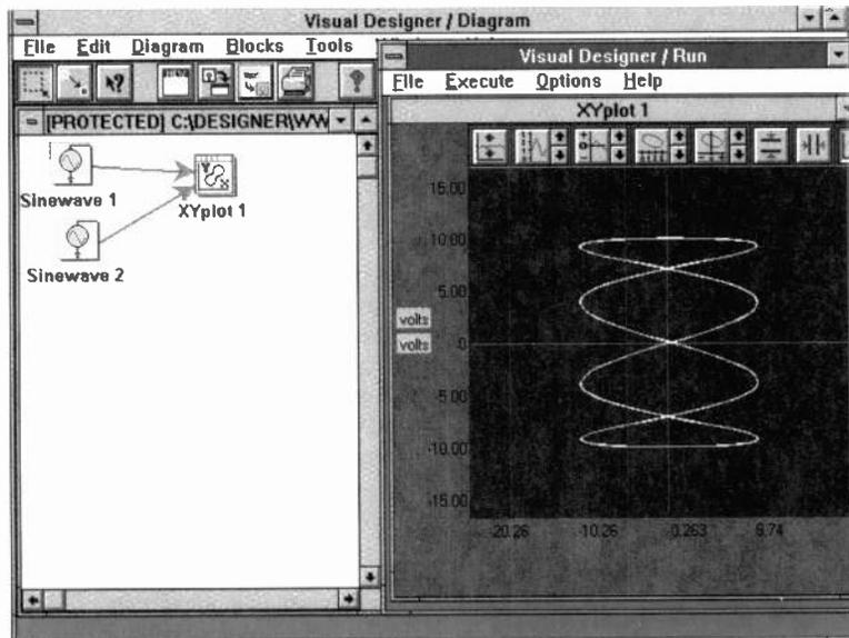
Fig. 4. Illustration of the XYPlot block and display.
