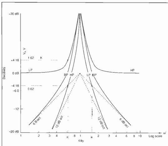
Fig. 5. Amplitude response (on a logarithmic scale) versus frequency (on a logarithmic scale) for low-pass and high-pass filters, showing how the gain is  $K'$ ,  $1$  or  $K$  at frequency  $K'$  or  $K$ , according to type. Since  $K \times K'=1$ , these three points on the logarithmic frequency axis are equally spaced.  $K$  and  $K'$  on the amplitude scale correspond to  $\pm 4.179$  dB. Note that the bandpass curve always lies between the other two.
