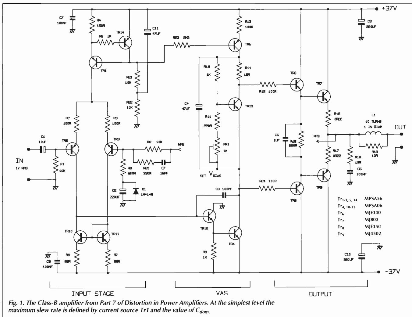
Fig. 1. The Class-B amplifier from Part 7 of *Distortion in Power Amplifiers*. At the simplest level the maximum slew rate is defined by current source  $Tr_1$  and the value of  $C_{dom}$ .
