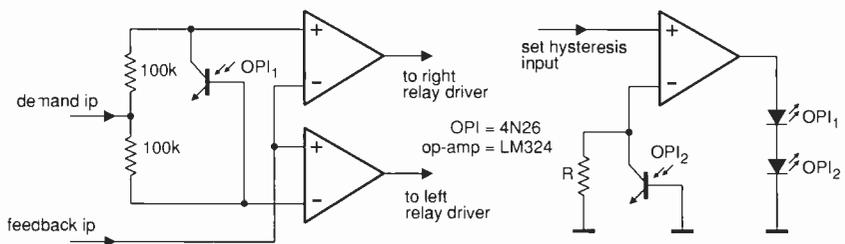
*Servo, originally used to control steering on a small vehicle, uses opto-isolators to provide a floating hysteresis voltage to define dead zone.*
