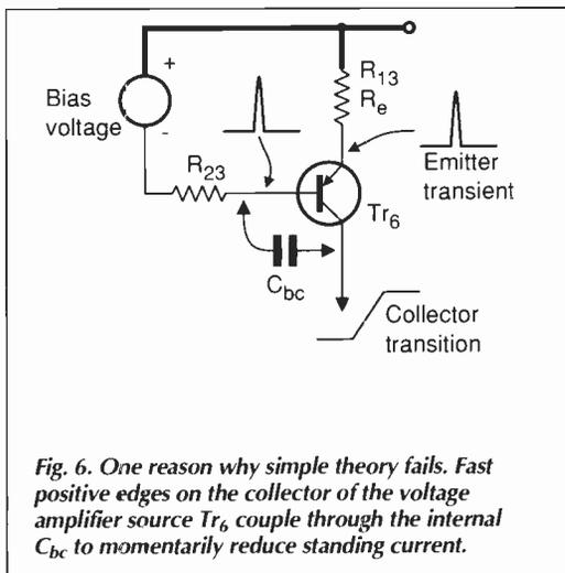
**Fig. 6. One reason why simple theory fails.** Fast positive edges on the collector of the voltage amplifier source  $Tr_6$  couple through the internal  $C_{bc}$  to momentarily reduce standing current.
