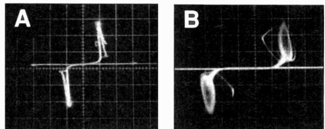
Fig. 10. Negative resistance characteristic for dual cold-cathode fluorescent lamps. The 'snap-back' effects show clearly as oscillation in b). These characteristics complicate power supply design.
