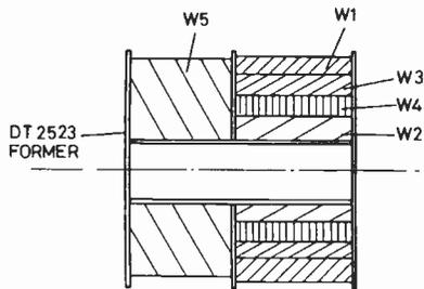
**Fig. 4. Winding format for the 8W fluorescent lamp inverter.**
