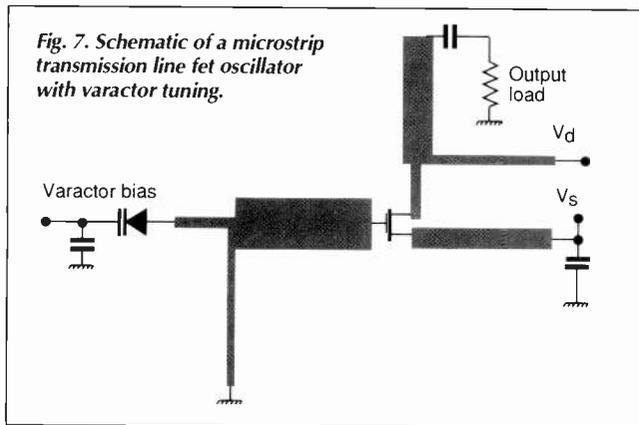
Fig. 7. Schematic of a microstrip transmission line fet oscillator with varactor tuning.
