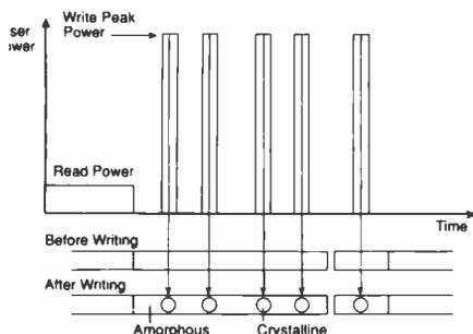
**Unrecorded, the active layer in worm media is amorphous and absorbs light. Recording involves changing the phase of a data area by crystallising it using heat from a laser. This results in light absorbing and reflecting areas: each represents a logic level.**
