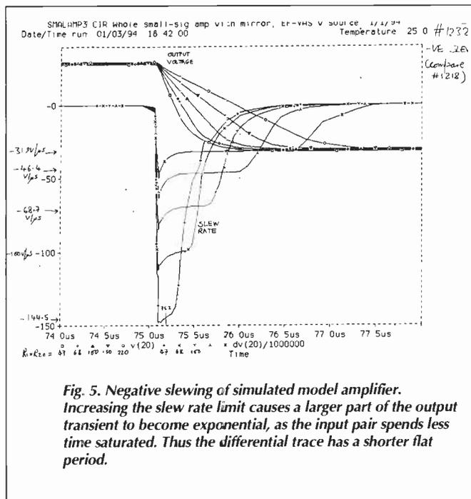
**Fig. 5. Negative slewing of simulated model amplifier.** Increasing the slew rate limit causes a larger part of the output transient to become exponential, as the input pair spends less time saturated. Thus the differential trace has a shorter flat period.
