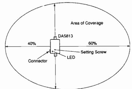
*Because it is unlikely that the Doppler radar module will be mounted exactly in the middle of the car, its effective area is asymmetrical. Although proportions of the area covered are fixed, the size of the area is adjustable by simply turning a screw.*
