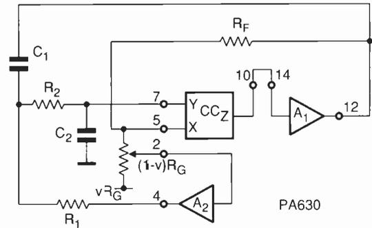
Fig. 1. Current-feedback amplifier circuit allows independent control of amplitude and frequency.
