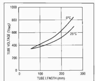
Fig. 9. Running voltage against lamp length at two temperatures. Start-up voltages are usually 50 to 200% higher over temperature.
