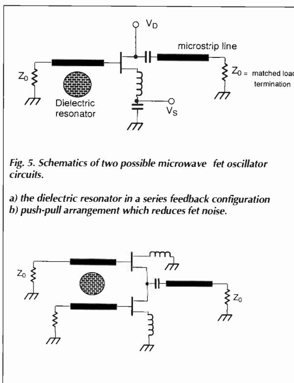
Fig. 5. Schematics of two possible microwave fet oscillator circuits.
