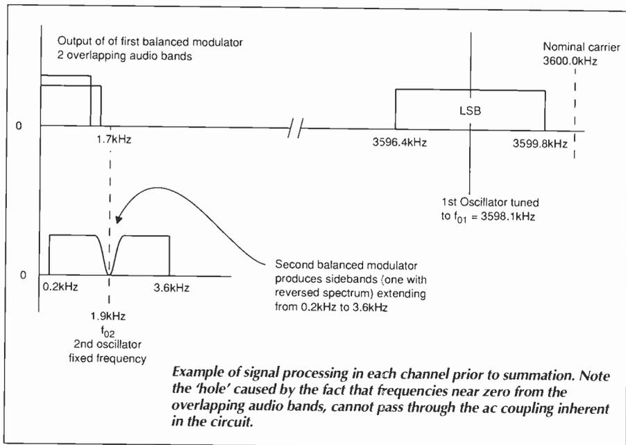
*Example of signal processing in each channel prior to summation. Note the 'hole' caused by the fact that frequencies near zero from the overlapping audio bands, cannot pass through the ac coupling inherent in the circuit.*
