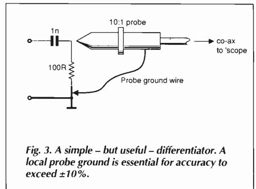
Fig. 3. A simple – but useful – differentiator. A local probe ground is essential for accuracy to exceed  $\pm 10\%$ .
