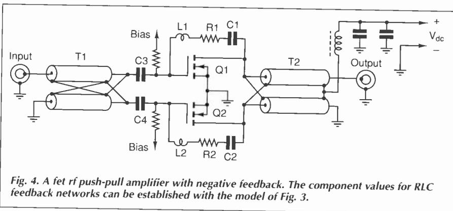
Fig. 4. A fet rf push-pull amplifier with negative feedback. The component values for RLC feedback networks can be established with the model of Fig. 3.
