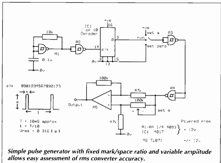
Simple pulse generator with fixed mark/space ratio and variable amplitude allows easy assessment of rms converter accuracy.
