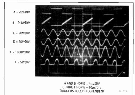
Fig. 2. Waveforms for the cold-cathode fluorescent lamp supply. Triggering is independent on traces A and B, and C through F.
