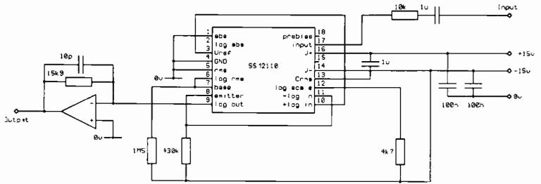
Fig. 9. Versatile converter chip configured for log of rms conversion. This configuration is useful for audio decibel metering.
