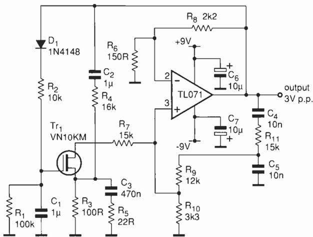
*Spot-frequency Wien-bridge oscillator uses a mosfet instead of a thermistor for amplitude control, while retaining a THD of about 0.02%.*
