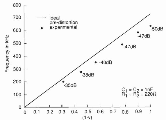
Fig. 2. Results of testing agree closely with predicted characteristics. Output frequency is shown plotted against
