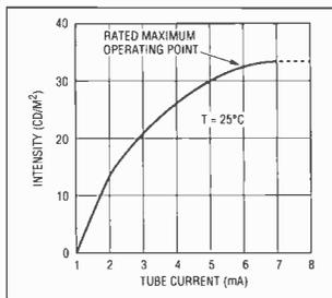
Fig. 6. Emissivity for a typical 6mA fluorescent lamp. Curve clearly flattens badly above about 6mA.
