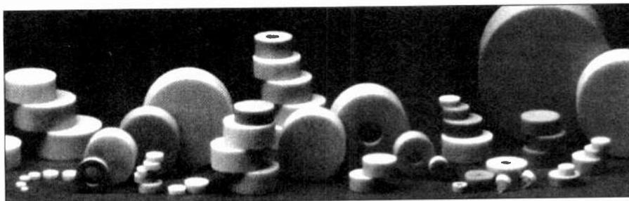
**Fig. 2.** Assorted sizes and shapes of ceramic discs suitable for high Q dielectric resonators. Diameter ranges from a few millimetres to several centimetres. An optimum diameter to height ratio would be 2:1.
