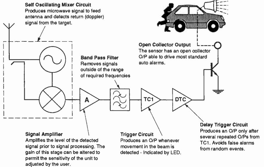
*This Doppler radar module, built into a bolt-on box, provides an output compatible with existing alarm systems and is easily retrofitted.*
