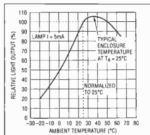
Fig. 7. Ambient temperature effects on emissivity of a typical 5mA lamp. Lamp and lamp enclosure must come to thermal steady state before measurements are made.
