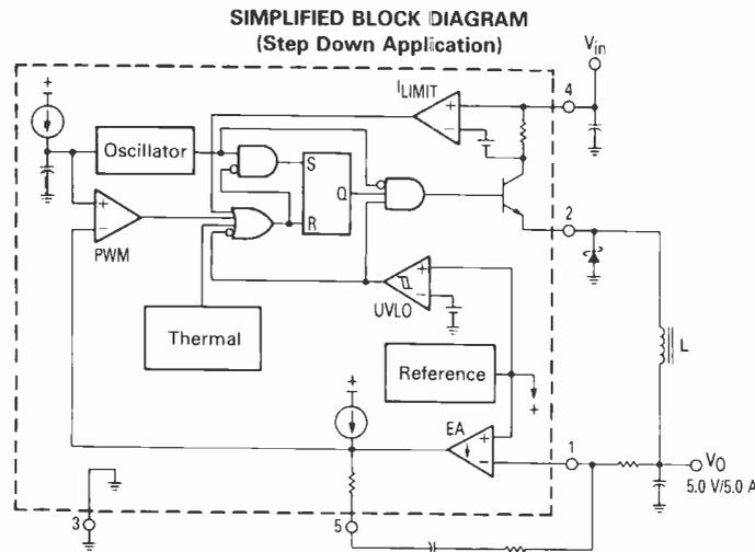
*Housed in a five-pinned flat pack, the MC34167 switching regulator needs few external components yet can be configured for a wide range of DC converter topologies. It delivers more than 5A switch current and operates from inputs to 40V.*
