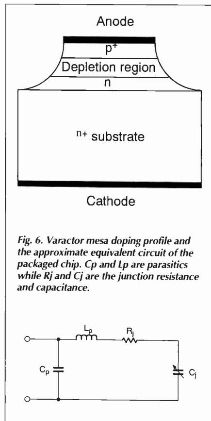
Fig. 6. Varactor mesa doping profile and the approximate equivalent circuit of the packaged chip.  $C_p$  and  $L_p$  are parasitics while  $R_j$  and  $C_j$  are the junction resistance and capacitance.
