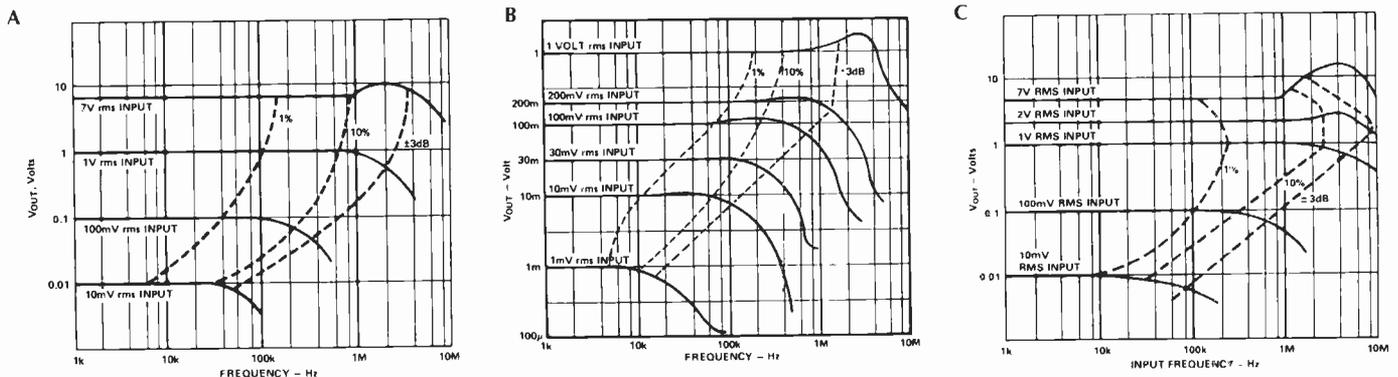
**Fig. 5. High frequency response for the three converters – AD536A at a), AD636 at b) and AD637 at c).**
