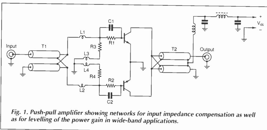
Fig. 1. Push-pull amplifier showing networks for input impedance compensation as well as for levelling of the power gain in wide-band applications.
