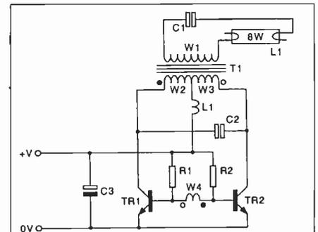
**Fig. 5. Emergency fluorescent lamp controller runs from 2.4 or 4V. Low operating voltage results in fewer power cells, reduced volume and lower cost.**
