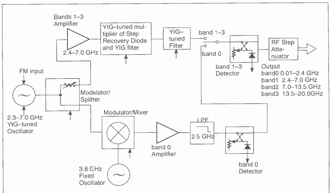
Fig. 12. This plug-in for a H-P signal generator provides an excellent example of using several technologies to produce signals over an 11-octave range.
