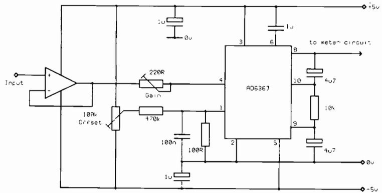
Fig. 8. Dedicated rms converter chips can reduce component count and improve accuracy.
