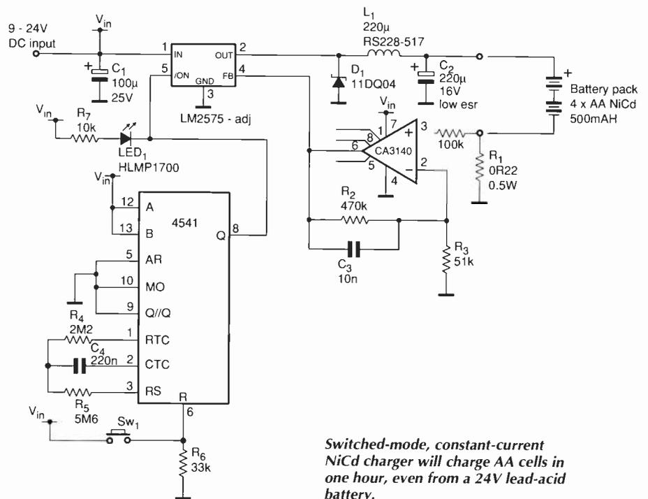
Switched-mode, constant-current NiCd charger will charge AA cells in one hour, even from a 24V lead-acid battery.
