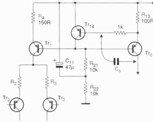
Fig. 7. A modified biasing system that makes  $Tr_6$  current the controlled variable, and reduces the feedthrough effect.
