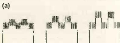
Fig. B(a). Tangential sensitivity of a diode, taken when output is as in middle case. Tangential sensitivity can be improved by applying a small forward bias current to the detector diode, as shown at (b) for various diodes. Optimum value of bias and the improvement that results depends upon frequency, as illustrated at (c) for a particular diode. ((b) and (c) reproduced by courtesy of Hewlett-Packard Ltd, from H-P Application Note 923.)
