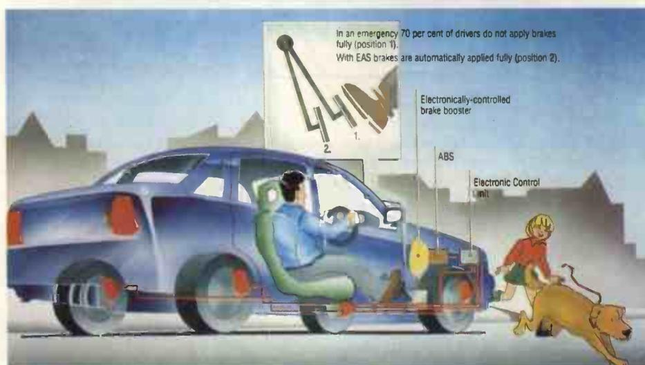
*Fig. 8. One of the problems with ABS is that often, drivers only press the brake pedal hard enough to invoke ABS when it's too late. Lucas' new brake assistance system senses when the brake is pressed more rapidly than usual, and applies the brakes harder than would be the case if the pedal were depressed normally.*
