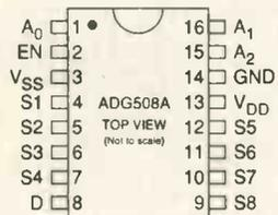
Fig. 3. One-of-eight switching is provided by this eight-way analogue multiplexer.
