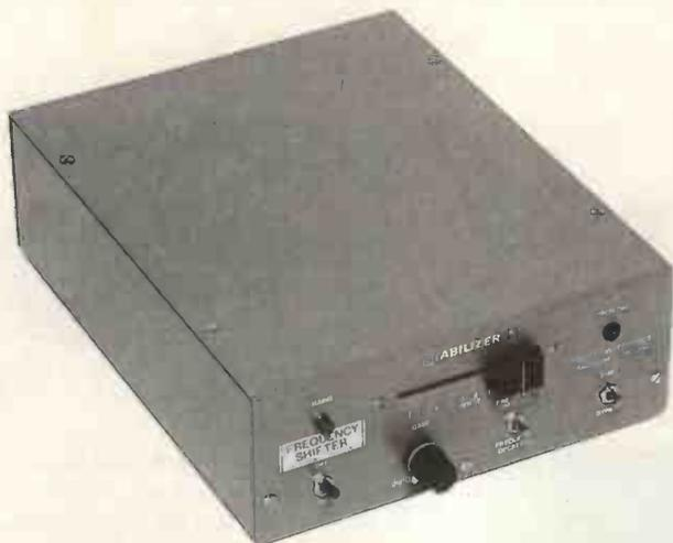
In any public address system where microphones and loudspeakers are in the same vicinity, acoustic feedback (howlround) occurs if the amplification exceeds a critical value. By shifting the audio spectrum fed to the speakers by a few Hertz, the tendency to howl at room resonance frequencies is destroyed and increased gain is available before the onset of feedback.
