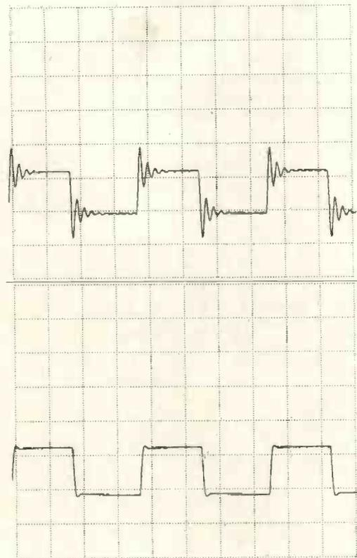
Fig. 7a). Output of the TLE2161 when the photodiode is receiving square wave on/off modulated light, Cf not in circuit. b) as a), but Cf (reduced to 0.9pF) in circuit.
