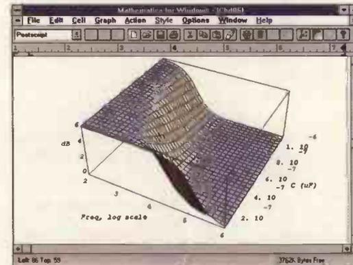
Fig. 12. The 3-D plot shows the sensitivity of the filter to variation in the value of capacitance C in Fig 11. Plotting ranges are easily changed to investigate sensitivity at other frequencies and with larger or smaller capacitances.
