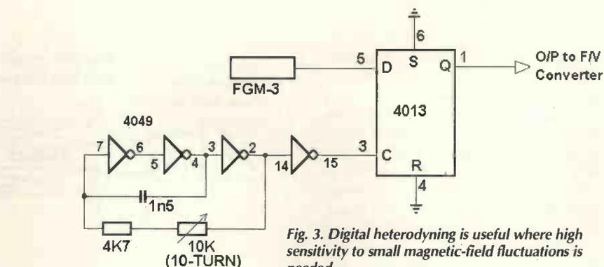
Fig. 3. Digital heterodyning is useful where high sensitivity to small magnetic-field fluctuations is needed.
