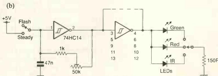
Fig.5a). Experimental photodiode circuit. b) Square wave flashing light circuit used to illuminate the photodiode.
