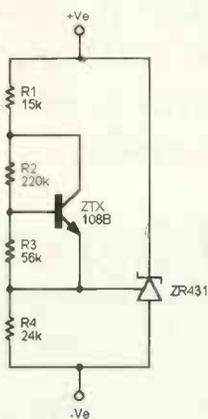
Fig. 7. When charging a lead-acid cell, terminal voltage must not be exceeded. This circuit tracks the large change in terminal with temperature..
