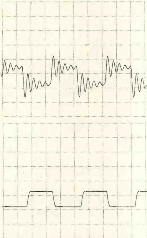
Fig. 6a). Output of the op-amp when the photodiode is receiving square wave on/off modulated light, Cf not in circuit. b) As a), but Cf in circuit.
