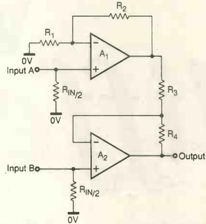
Fig. 3. Output from this circuit is zero when common mode signals are applied. This option has a gain of  $(R_1+R_2)/R_2$  for differential signals. Matched pairs of resistors are required.
