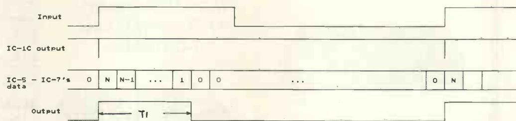
Programmed in 1% steps from zero to 99%, this duty-cycle controller is totally insensitive to frequency.
