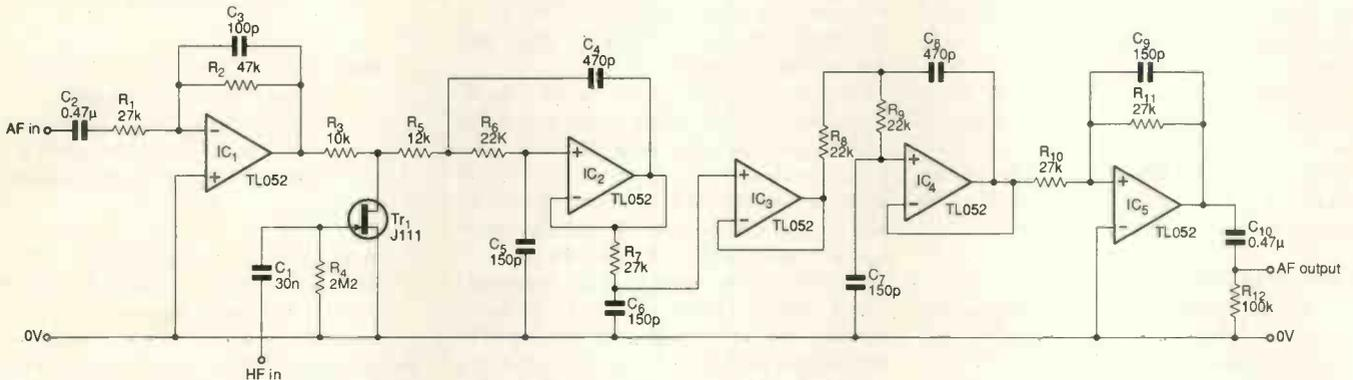
**Fig. 3. Audio dynamic range controller incorporating a switched attenuator. The jfet provides the attenuation, under control of square waves from oscillator, Fig. 4.**
