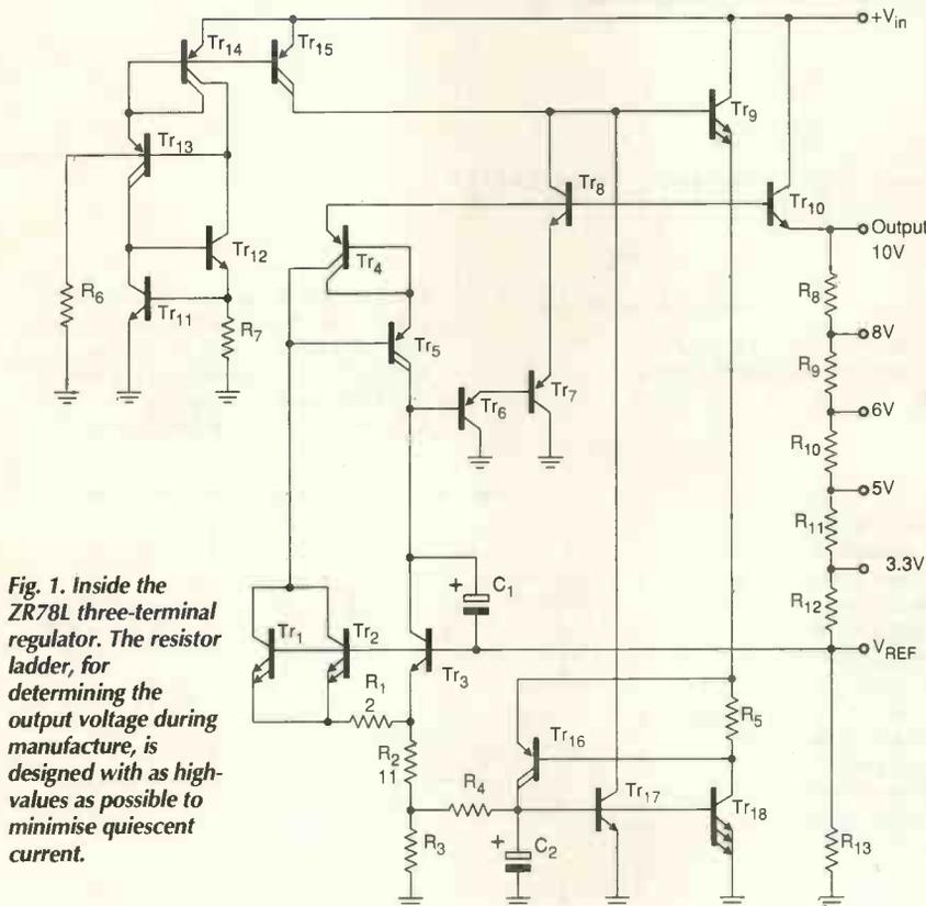
**Fig. 1.** Inside the ZR78L three-terminal regulator. The resistor ladder, for determining the output voltage during manufacture, is designed with as high-values as possible to minimise quiescent current.
