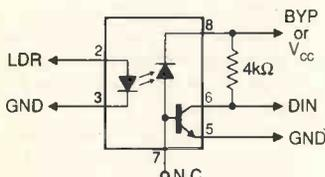
**Fig. 4.** High speed *6N136* couplers improve speed, but their pin-out is different.
