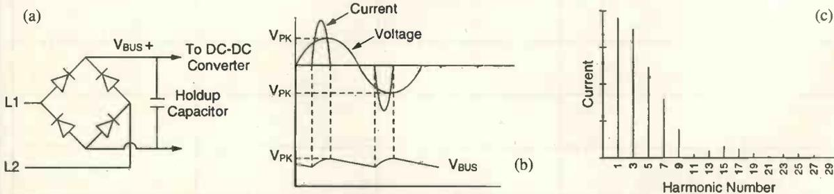
Fig. 2a). off-line power supply with a ac-dc front end consisting of a bridge rectifier and large filter capacitor. 2b) Current is drawn from the line only when peak voltage on the line exceeds voltage on the filter capacitor c) Typical input current spectrum of an electronic load. The odd harmonics are generated as a result of poor power factor occurring in electronic loads.
