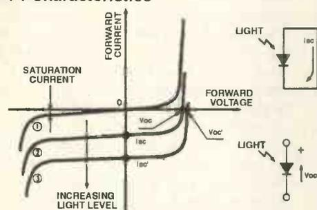
Fig. 3a). How the normal diode characteristic of a photodiode is shifted when light falls upon it.
