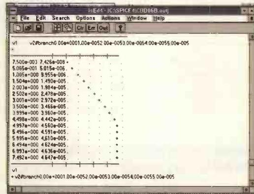
Fig. 4. With a low-value load resistor in circuit, current through the load rises as supply voltage is ramped from 0-7.5V, stabilising between 4.6µA and 4.7µA.
