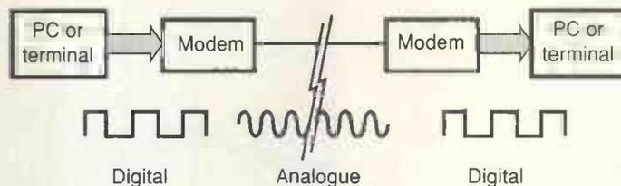
In order for digital data to pass over a normal telephone line, it needs to be converted to analogue form at the sending end and back to digital at the receiver. Ones and zeros travelling over the line are usually represented by two tones.
