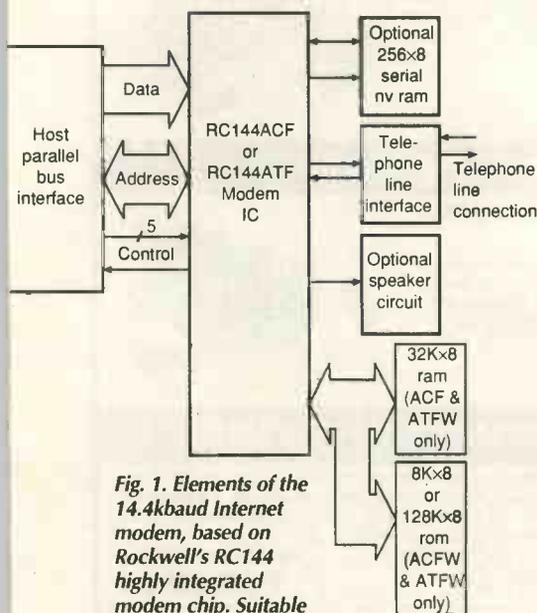
Fig. 1. Elements of the 14.4kbaud Internet modem, based on Rockwell's RC144 highly integrated modem chip. Suitable for fax or data, this version interfaces to the pc via an expansion card slot.
