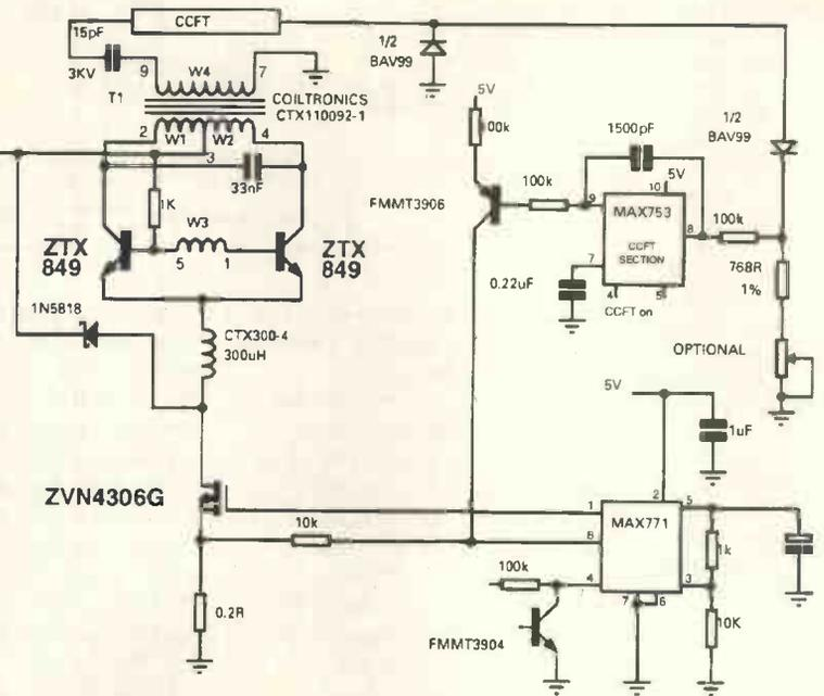
current. Using the primary current method allows the tube to be fully floating with low high-voltage loss.
