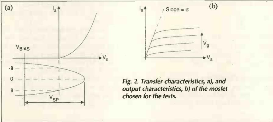
Fig. 2. Transfer characteristics, a), and output characteristics, b) of the mosfet chosen for the tests.
