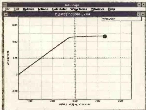
Fig. 2. IntuScope postprocessor software produces an oscilloscope-like display of the dc sweep of the zener stabiliser circuit. The zener, nominally 4.7V, produces a stabilised output at approximately 4.65V.
