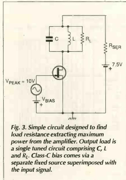
Fig. 3. Simple circuit designed to find load resistance extracting maximum power from the amplifier. Output load is a single tuned circuit comprising C, L and  $R_L$ . Class-C bias comes via a separate fixed source superimposed with the input signal.
