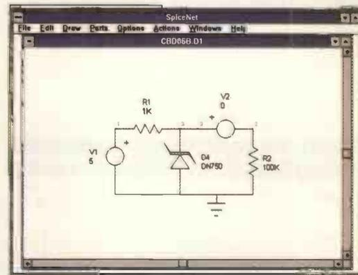
Fig. 3. Load resistor and dummy voltage source, added to stabiliser Fig. 1. Source V2 has zero output, but is included so that the load current can be measured.
