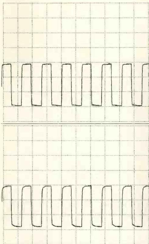
Fig. 8a) Output of the the circuit of Figure 5 a) (using the TLE2061) when illuminated by light from a green led (3mm ultra-bright green, 590-345). b) As a) but receiving light from an infra red led, T.I. GaAlAs IR diode TIL901. Note the delayed contribution from carriers released in the bulk material, outside the depletion region.
