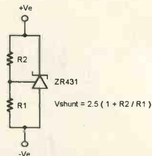
**Fig. 5. In battery applications, where the generic 431 three-terminal shunt regulator may consume too much power, this high-performance alternative is useful. Its quiescent current is 50µA and the reference input current just 120mA.**
