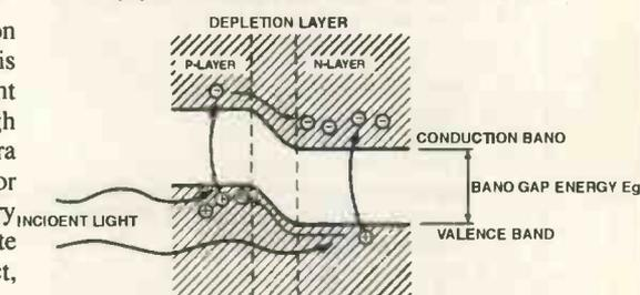
Fig. 2a). Diagrammatic cross-section of a typical planar diffused silicon photodiode. b) Bandgap diagram for a).\*
