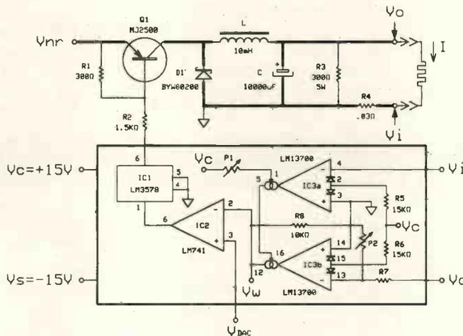
Switching power supply is programmed for power instead of voltage or current, giving up to 100W from 40V input.
