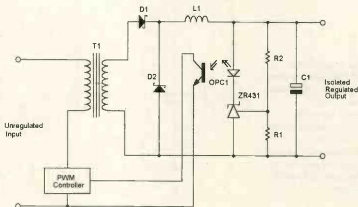
pin of the device is not directly wired to the sense divider. Instead it has the led of an optocoupler in series which feeds error signals to the pulse width modulator of the power supply across the isolation barrier.
