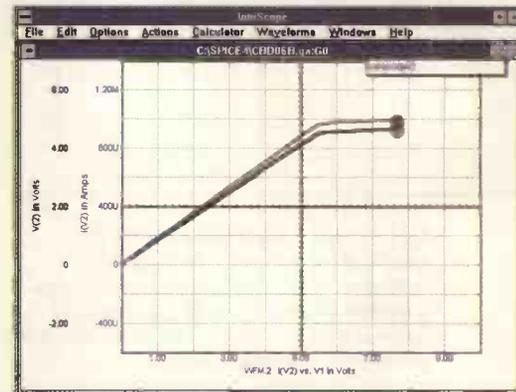
Fig. 5. An *Intuscope* plot shows how V(2), the output voltage at node 2 (curve 1), and I(V2) the output current through source V2 (curve 2), vary as supply current V1 is swept up from 0-7.5V.
