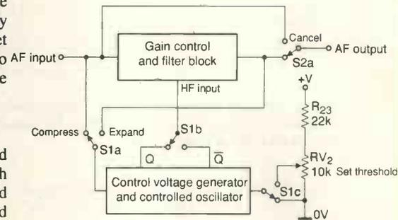
**Fig. 2. Audio compression and expansion system based on a low-distortion switched attenuator.**
