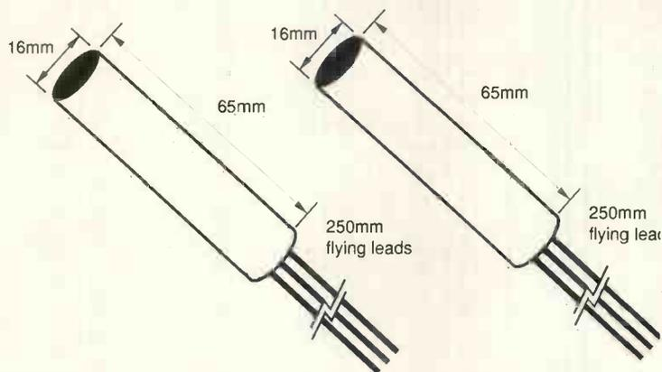
The FGM-3 outputs a frequency between 50kHz and 120kHz whose period represents magnetic fields in the range  $\pm 50\mu\text{T}$  and is highly stable with temperature.
