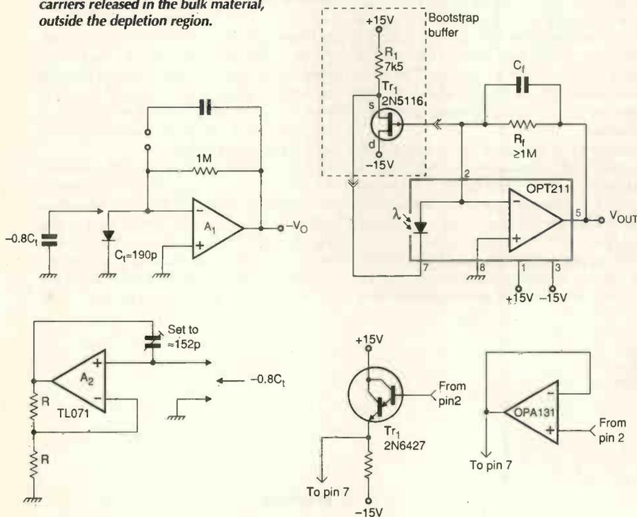
Fig. 9.a) Increasing the bandwidth by connecting negative capacitance in parallel with the photodiode. b) Increasing the bandwidth by bootstrapping, applied to an OPT211 integrated photodiode/op-amp type.<sup>†</sup>
