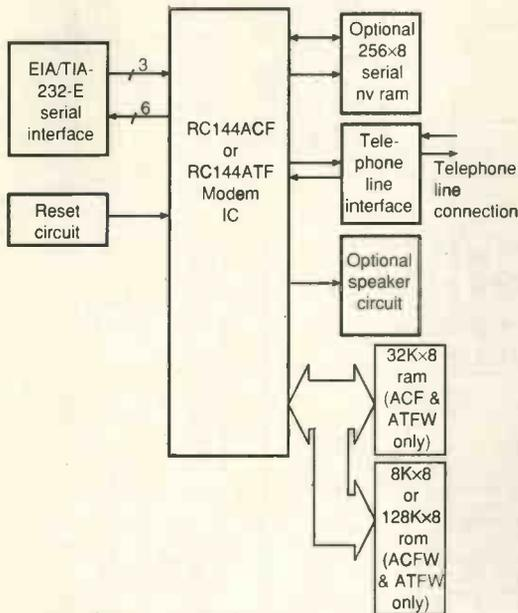
Fig. 2. Options of the RC144 fax/data modem chip allow interfacing to a pc COM port via a standard serial interface.
