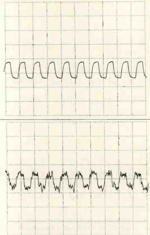
12b) Output of  $A_1$  at a range of 2m from 3000mcd red led. c) simulated output of  $A_2$  at a range of 200m.
