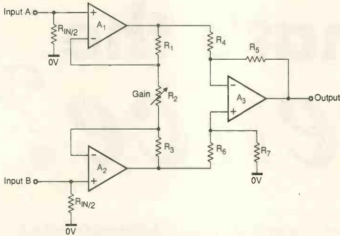
Fig. 2. This amplifier has the correct input impedance, rejects common-mode signals and has its gain set by a single resistor. This method of gain adjustment makes the design ideal for instrumentation amplifiers.
