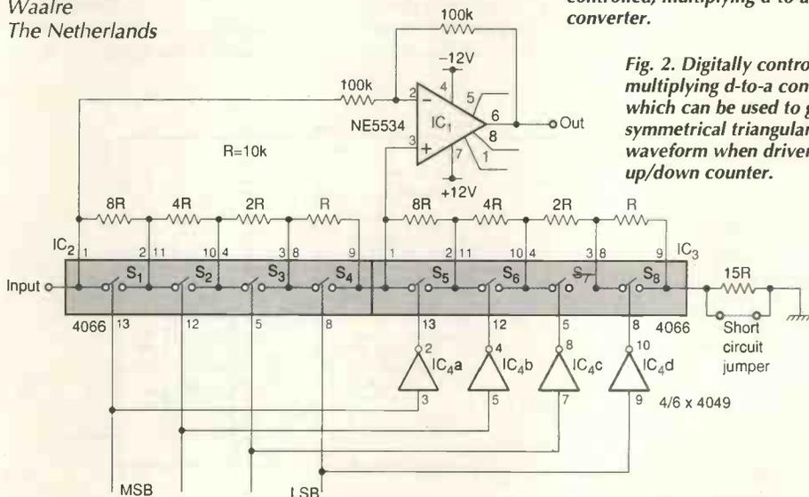
Fig. 2. Digitally controlled, multiplying d-to-a converter, which can be used to give a symmetrical triangular output waveform when driven by an up/down counter.
