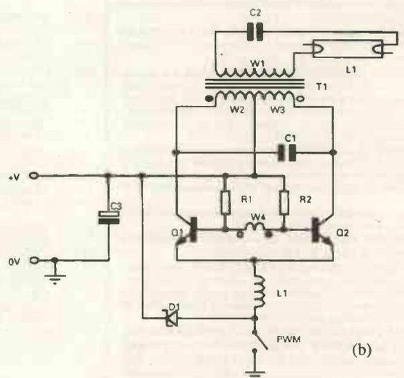
Fig. 3a). Linear Technology lcd backlight converter for a fluorescent lamp. Based on the Buck converter current fed Royer scheme of 2b), the circuit has a stated electrical conversion efficiency of 88%. b) Maxim lcd backlight converter.
