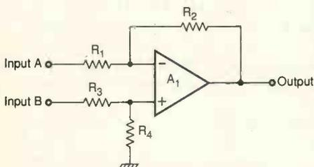
Fig. 1. This circuit has equal impedance into input A and B for common mode signals – but not for differential signals. Consequently, transmission lines may be unbalanced.
