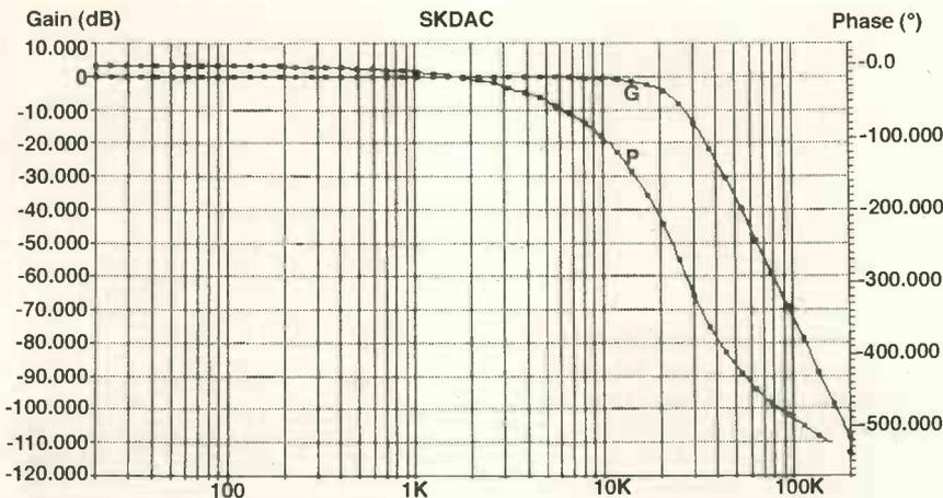
Fig. 5. Frequency response of two consecutive third-order Sallen and Key low-pass filter stages between the chopper stage and af output. The circuit gives about 90dB rejection of the switching waveform in the af output.
