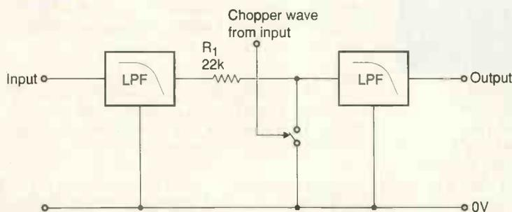
Fig. 1. Low-distortion, gain-controlled block based on a high-speed electronic switch. Over most of the audio range, distortion is just 0.005%. On and off durations of the switch are determined by an externally applied dc voltage.
