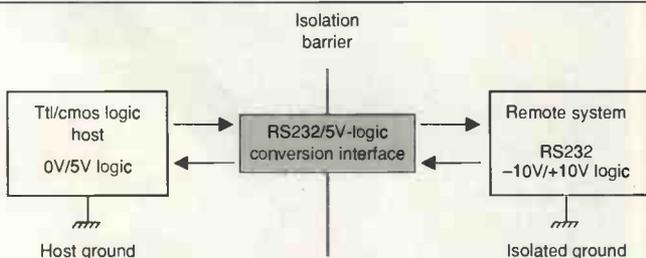
Fig. 1. Distinction between 'cable' ground at the remote end of an isolated RS-232 system, and the logic system ground, which will typically be the 0V potential of a pc.
