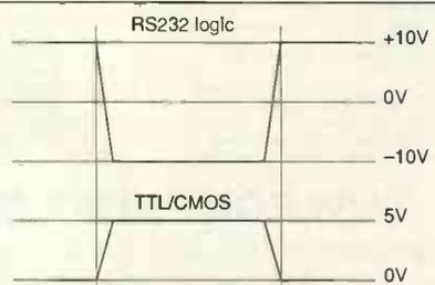
Fig. 2. RS-232 isolation systems usually involve both RS-232 and standard cmos/ttl logic levels.
