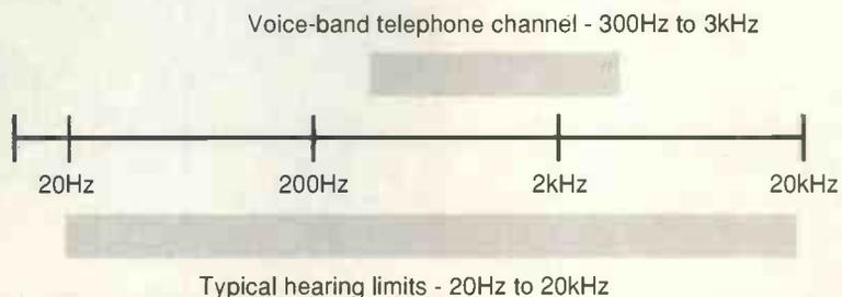
When communicating data over the public switched network, data rate is usually limited by the bandwidth of the telephone line, which is only designed to carry part of the voice spectrum. But data compression and error correction can provide significant benefits.
