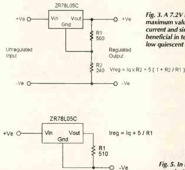
**Fig. 4. Removing Fig. 1's resistor to ground produces a precision current source.**
