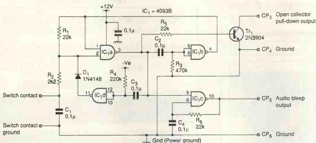
Switch debouncer, originally for a Morse key, has been used for many other applications, introducing no extra delay and producing a beep when contacts are made.
