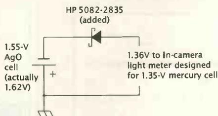
Instead of junking older photometers using banned mercury cells, use a Schottky and a silver oxide cell.
