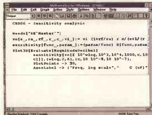
Fig. 10. This Mathematica-based sensitivity analysis of the filter in Fig 11 is adaptable to a wide range of circuits.
