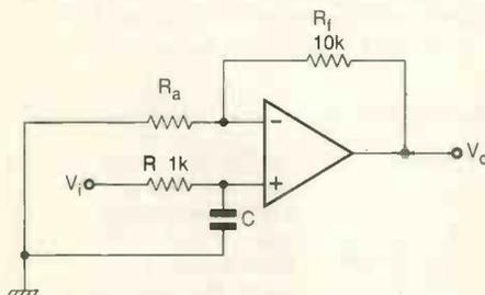
Fig. 11. Low-pass active filter circuit used to demonstrate sensitivity analysis.
