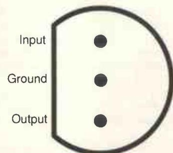
**Fig. 2.** Pinout of the ZR78L05C three-terminal, 5V regulator.
