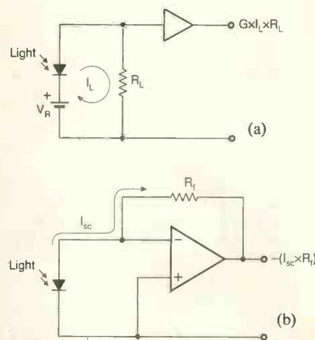
(Above) Fig. 4a). Circuit for photodiode operation with reverse bias. b) Circuit for operation where  $R_L$  is short circuit.\*
