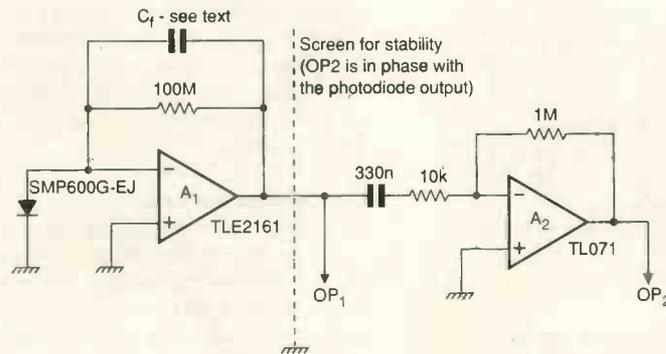
Fig. 12a) Receiving end of a long range optical data link.
