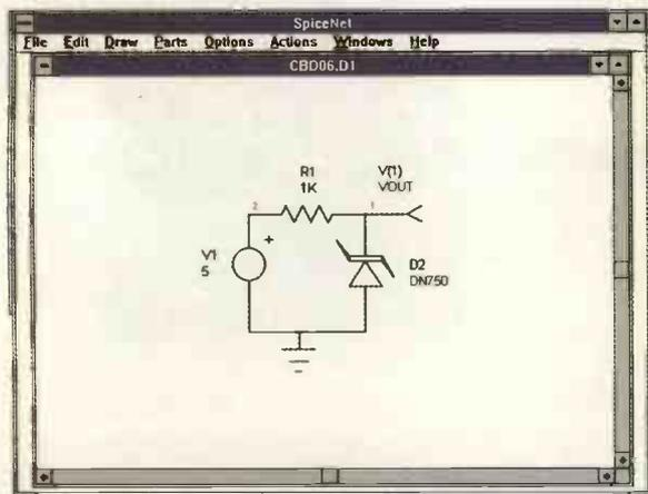
Fig. 1. This schematic of a zener diode stabiliser was produced using the SpiceNet software. Node numbers are displayed (in red), except for the ground line, which is node 0. The Y-shaped symbol is an optional way of indicating a test point.
