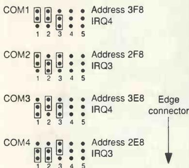
Table 3. On the modem card, jumpers are provided for non-standard address and IRQ selections.
