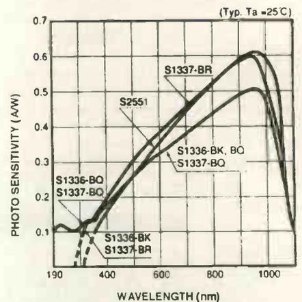
Fig. 1. Sensitivity of typical silicon photodiodes as a function of wavelength.\*
