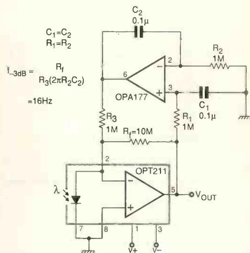
Fig. 10. Circuit to reject ambient light while providing high sensitivity to wanted signals.<sup>†</sup>
