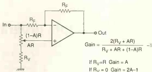
Fig. 1. Principle of the digitally controlled, multiplying d-to-a converter.
