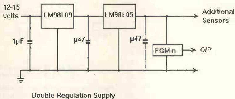
**Fig. 1. The three-terminal sensor is very stable with temperature, but it needs a doubly regulated supply for best performance.**
