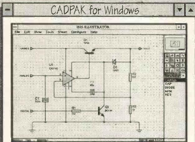
CADPAK is especially suited to educational, hobby and small scale schematic and PCB design. CADPAK includes both schematic drawing and 32-bit PCB drafting tools but as an entry level product, there is no netlist link between them.
