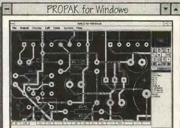
PROPAK has all of the features in CAPAK plus netlist based integration, automatic power plane generation and a powerful auto-router. PROPAK includes enough schematic capture and PCB design functionality for all but the most demanding applications.
