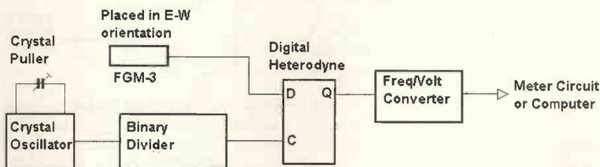
Fig. 4. Digital heterodyning is a useful building block for a magnetometer capable of measuring the Earth's magnetic field, but the oscillator needs to be stable.
