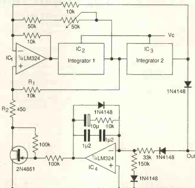
Fig. 2. Complete oscillator circuit, in which frequency is determined by  $RC$  in Fig. 1 and  $Q$  by the ratio of  $R_1$  and  $R_2$ .
