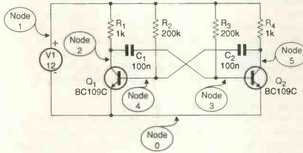
Fig. 8. An astable circuit such as this has a symmetrical operating point in a dc analysis, Table 5.
