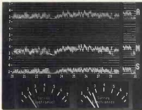
PPM10 In-Vision PPM and Chart Recorder generates a display emulating the well known coaxial TWIN movements for monitoring stereo audio levels and mono compatibility. Also: TWIN TWIN PPM comprising two PPM9 boards, featuring inherent stability with law under micro-processor control, the unit gives simultaneous monitoring of A/B on red/green and M/S on white/yellow pointers. Manufactured under licence from the BBC.
