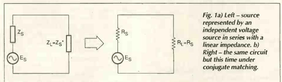
**Fig. 1a) Left – source represented by an independent voltage source in series with a linear impedance. b) Right – the same circuit but this time under conjugate matching.**
