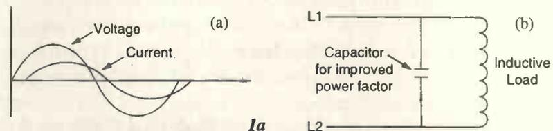
Fig. 1a). Traditional poor power factor – the current either leads or lags the voltage. b) An easy way to correct this type of poor power factor is to add a reactive component of opposite sign in parallel with the load.
