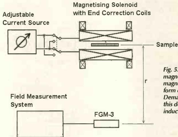
Fig. 5. At the heart of this materials magnetometer is a controllable magnetising arrangement in the form of an air-cored solenoid. Demagnetising field measured by this device relates to magnetic induction in the specimen.
