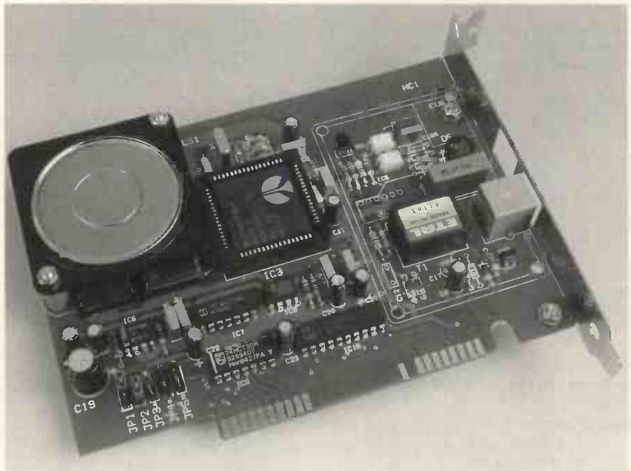
PC interfacing 14.4kbit/s modem includes error correction and compression to achieve sustained data throughput of 57kbit/s.
