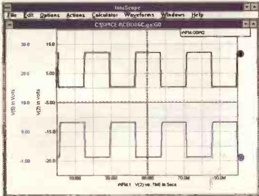
Fig. 9. Outputs (collector voltages) of the astable after it has been stimulated into oscillation by one of the techniques described in the text. After a 1ms settling period, V(2) becomes a square-wave, upper curve. V(5) is in antiphase to V(2), lower curve.
