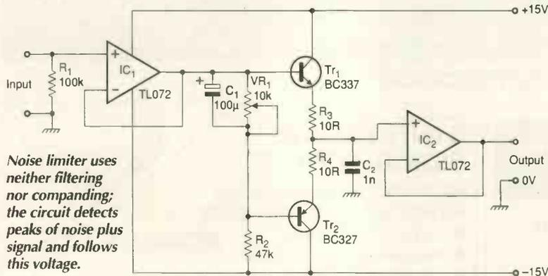
Noise limiter uses neither filtering nor companding; the circuit detects peaks of noise plus signal and follows this voltage.
