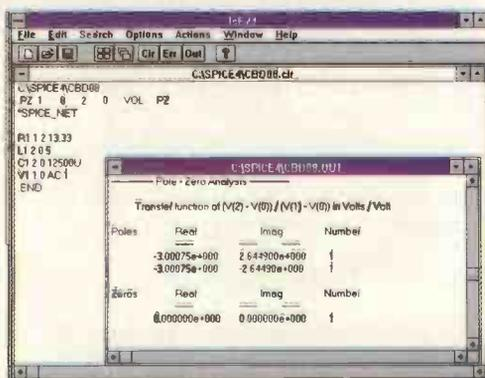
Fig. 13. The netlist of Fig. 9, with the pole-zero analysis seen in the Output file. The circuit has two complex poles, q and  $\omega_0$  having been given the values that produced Fig. 12.
