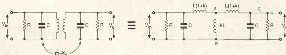
But, how can any phase-shift exist between the primary and secondary of a transformer if the flux closely couples both coils? The answer is – in the Foster-Seeley circuit it does not.
