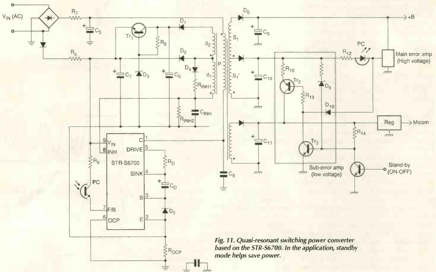
Fig. 11. Quasi-resonant switching power converter based on the STR-S6700. In the application, standby mode helps save power.
