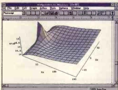
Fig. 8. A three-dimensional plot of the noise figure of the attenuator helps the engineer to see how noise is related to source resistance and impedance.
