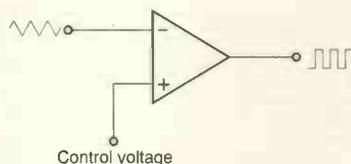
*Replacing an integrator and comparator sawtooth generator with a simple relaxation oscillator still provides a linear relationship between control and output square-wave width in this cheaper pulse-width modulator.*
