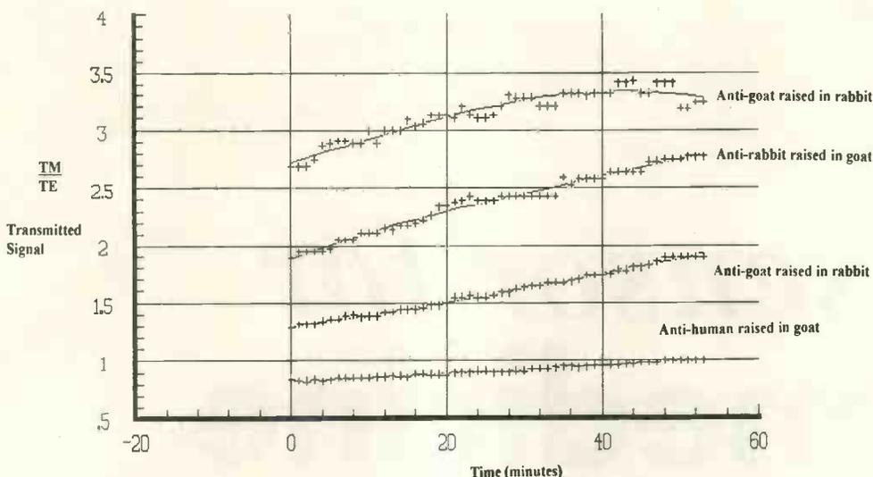
Fig. 2. Transmitted output power of the waveguide (TM/TE) is recorded as a function of time for the following sequence of antibodies bound to the waveguide – a) anti-human raised in goat, b) anti-goat raised in rabbit, c) anti-rabbit raised in goat and d) anti-goat raised in rabbit. As each subsequent layer binds to the preceding layer the transmitted output power is observed to rise in each case.
