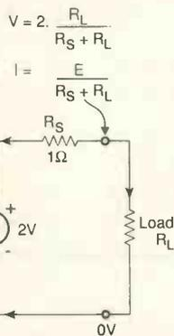
Fig. 1a). Normalised source and load, illustrating the maximum power theorem.
