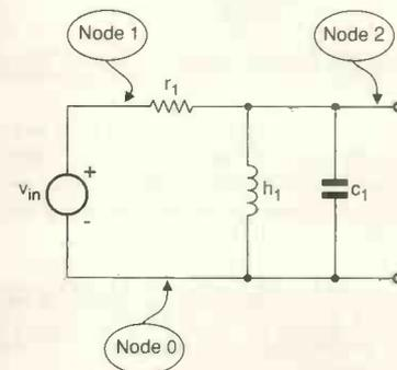
Fig. 9. Poles and zeros of this band-pass filter are analysed by a Nodal routine in Fig. 10.
