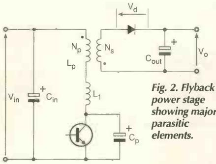
Fig. 2. Flyback power stage showing major parasitic elements.
