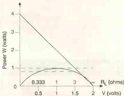
Fig. 1b). Power in the load resistor  $R_L$  as a function of its value, when  $R_S$  equals the design system impedance of 1Ω (curve) and total power supplied by the generator (sloping line).
