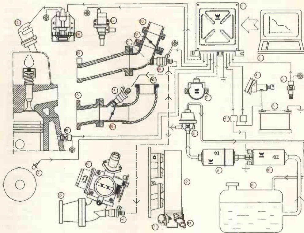
*Weber's engine-management system takes into account a wide variety of engine parameters from fuel flow to water temperature. The result is faster engine response, more efficient combustion and fewer noxious emissions.*
