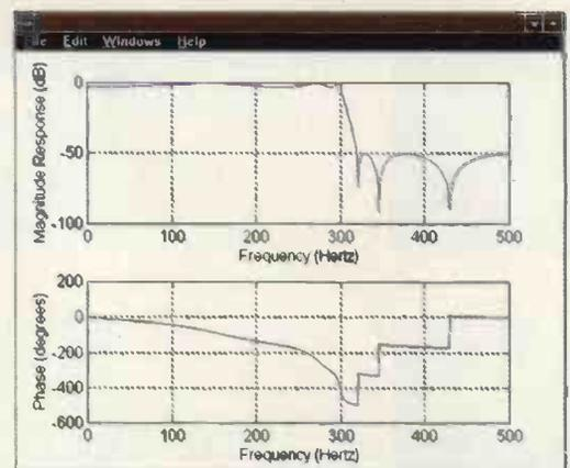
**Fig. 2.** Transfer function generated graphically in the digital z domain.
