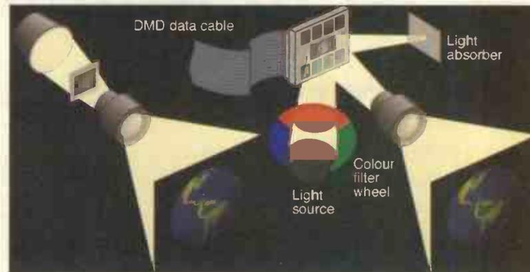
Conventional projector, left, and a projection system incorporating the digital micromirror device, right. In the DMD system, light from the source passes through a colour wheel and is reflected to both the projection lens and to the light absorber on the right. Picture courtesy Texas Instruments.
