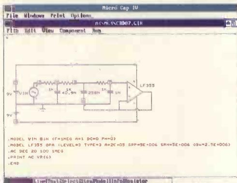
Fig. 1. Typical schematic drawn with Micro-Cap IV includes definitions of models and optional command statements for the analysis.
