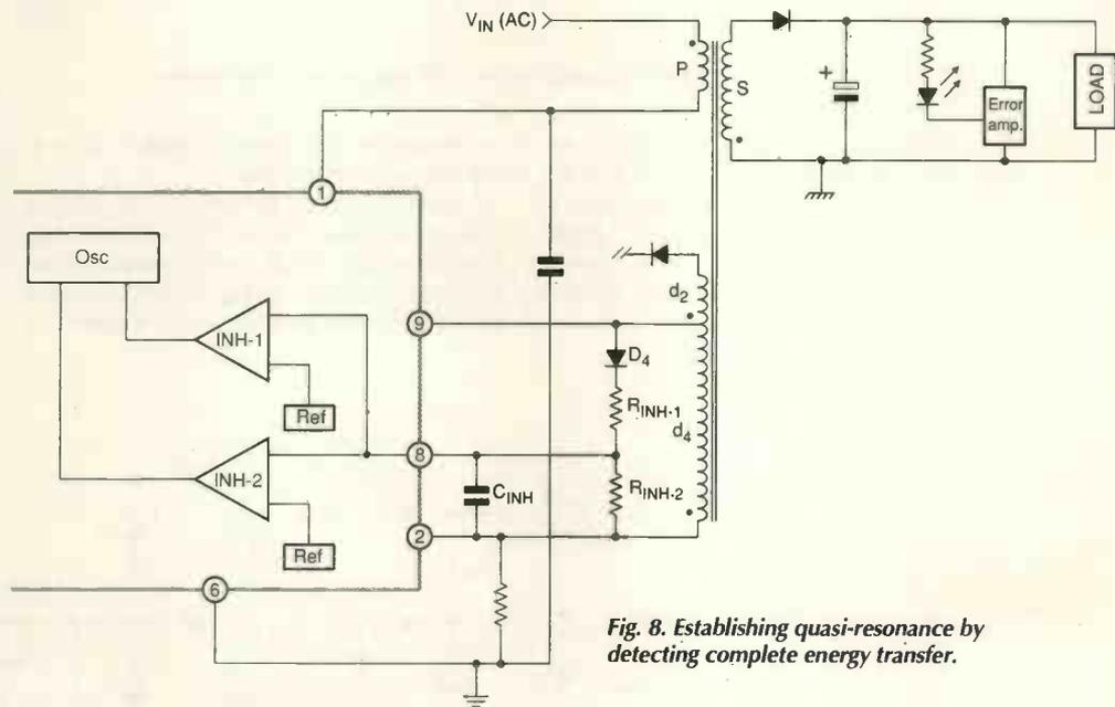
Fig. 8. Establishing quasi-resonance by detecting complete energy transfer.
