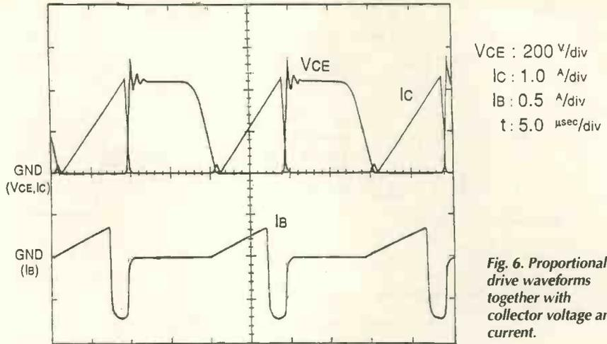
Fig. 6. Proportional drive waveforms together with collector voltage and current.
