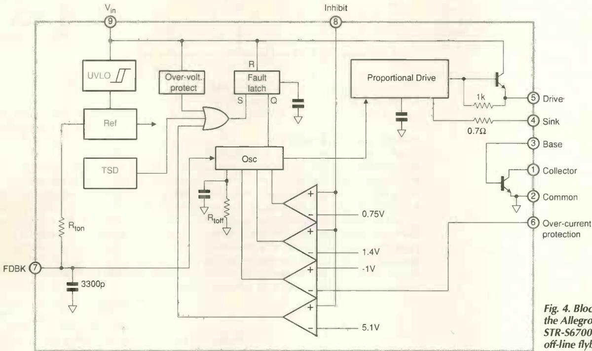
Fig. 4. Block schematic of the Allegro Microsystems STR-S6700 quasi-resonant off-line flyback converter.
