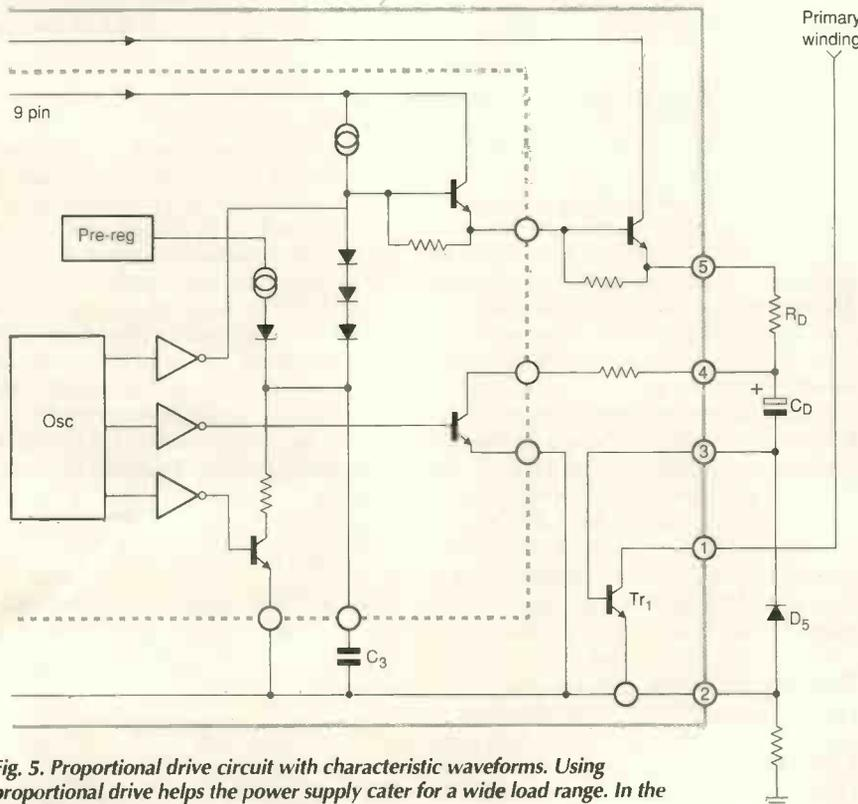
Fig. 5. Proportional drive circuit with characteristic waveforms. Using proportional drive helps the power supply cater for a wide load range. In the upper waveform diagram,  $I_{B1(peak)} = (V_{9pin} - 3) / R_D$
