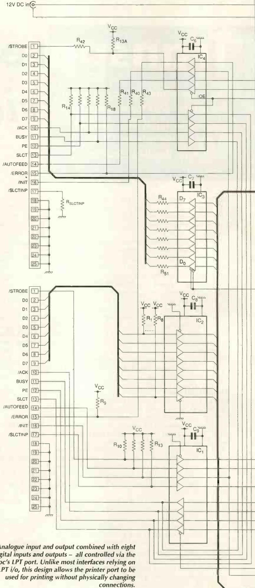
*Analogue input and output combined with eight digital inputs and outputs – all controlled via the pc's LPT port. Unlike most interfaces relying on LPT i/o, this design allows the printer port to be used for printing without physically changing connections.*
