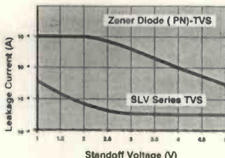
Leakage current and capacitance of the pnp enhanced punch-through diode are orders of magnitude lower than typical pn zener diodes.
