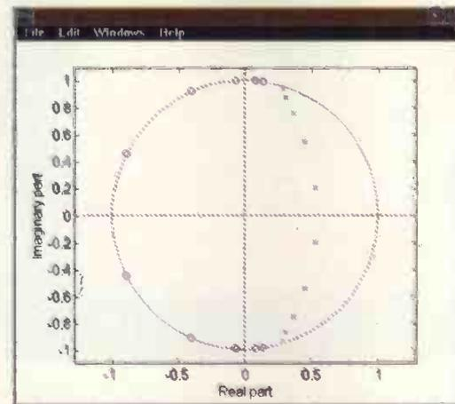
Fig. 4. Determining the positions of the poles and zeros in the z-plane unit circle gives information on possible problems that may occur for poles lying close to the perimeter. If through quantisation effects they should stray outside the unit circle the system becomes unstable.
