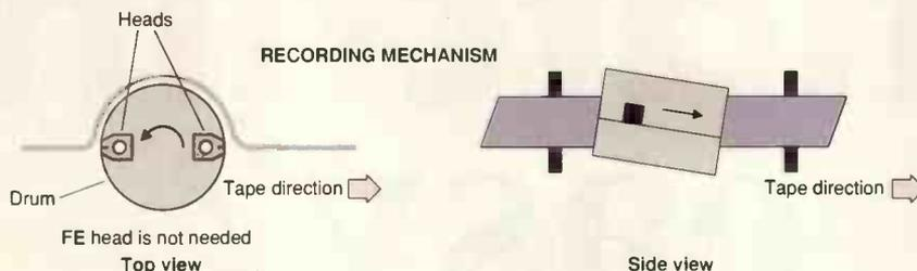
DVCPRO differs in using more robust metal particle tape, which is run at double speed to increase track pitch to 18µm, and the addition of a control track and cue channel. The HD version uses metal-evaporated ME tape run at double speed to record twenty 10µm tracks per frame. Horizontal resolution is about 500 lines for SD – 25% greater than Hi8/S-VHS – and 600 lines for HD, with double the vertical resolution.
