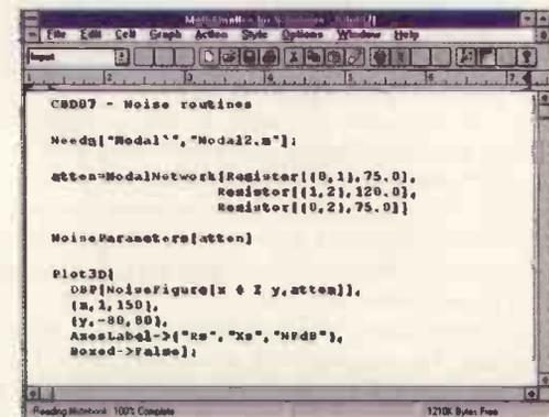
Fig. 6. Nodal routines are used for calculating noise parameters of circuits such as the attenuator network of Fig. 7.
