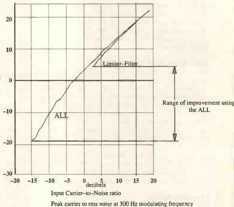
Fig. 5. Comparison between a limiter-filter and an amplitude-locked loop demodulator showing that the amplitude-locked loop is capable of extracting a phase coherent carrier well down into noise levels.
