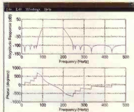
Fig. 5. Graphical results from the design of a digital filter using the instructions in Table 1. This example shows that Elliptical filters are unsuitable for systems which require linear phase response.
