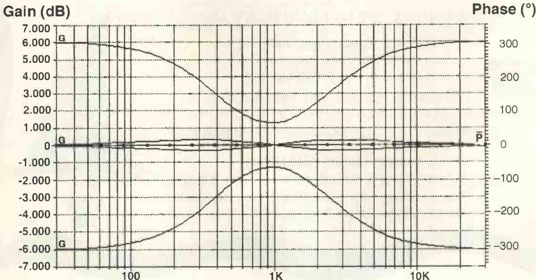
Simulation of boost and cut curves with the preamplifier's tone controls set flat and at maximum and minimum. Centre curves show phase shift. Measured results tally.
