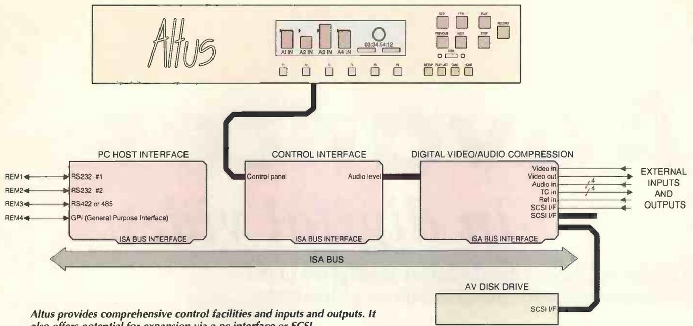
*Altus provides comprehensive control facilities and inputs and outputs. It also offers potential for expansion via a pc interface or SCSI.*
