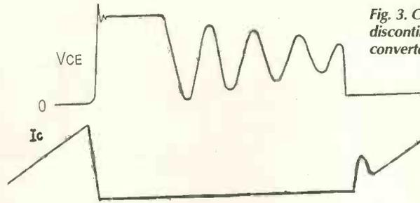
Fig. 3. Characteristic discontinuous flyback converter waveforms.
