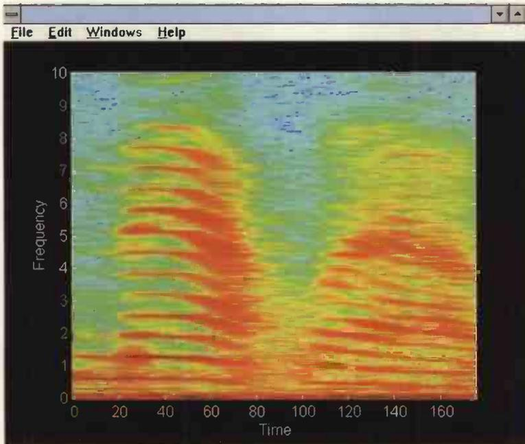
Fig. 6. Spectrogram of the word *matlab*. The function *specgram* can be used with great effect to analyse speech signals.
