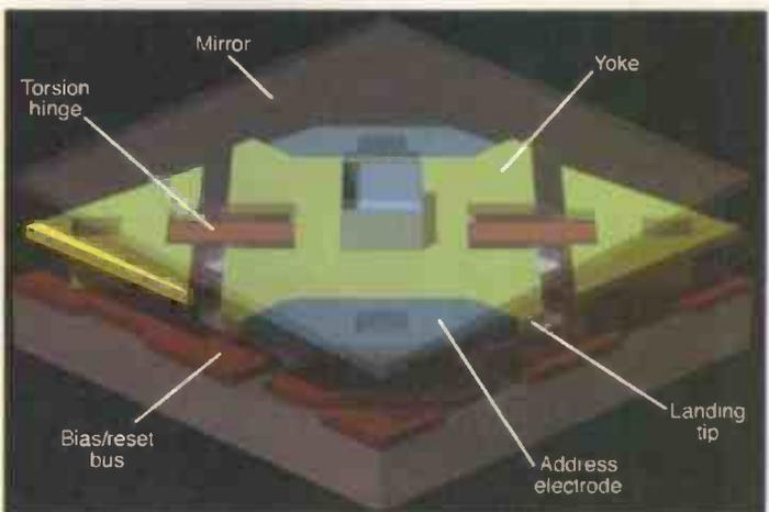
Details of the digital micromirror device. 500,000 mirrors – each hinged and capable of rotating independently under digital control – make up a display measuring just 1.5 by 1cm. Pictures courtesy TI.
