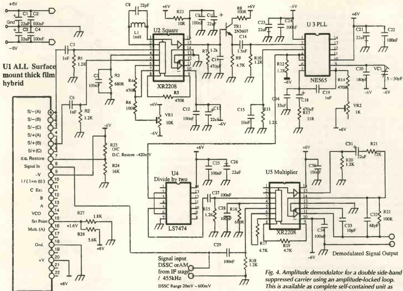
Fig. 4. Amplitude demodulator for a double side-band suppressed carrier using an amplitude-locked loop. This is available as complete self-contained unit as shown in U1. ICs U2-5 comprise a standard synchronous demodulator.
