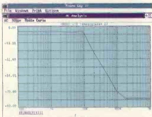
Fig. 3. AC response of the circuit of Fig. 1 shows the typical response of Chebyshev low-pass filter.
