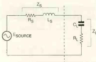
Fig. 1c). In the ac case, source and load reactance must be taken into account. Source to the left of the dotted line, load to the right.
