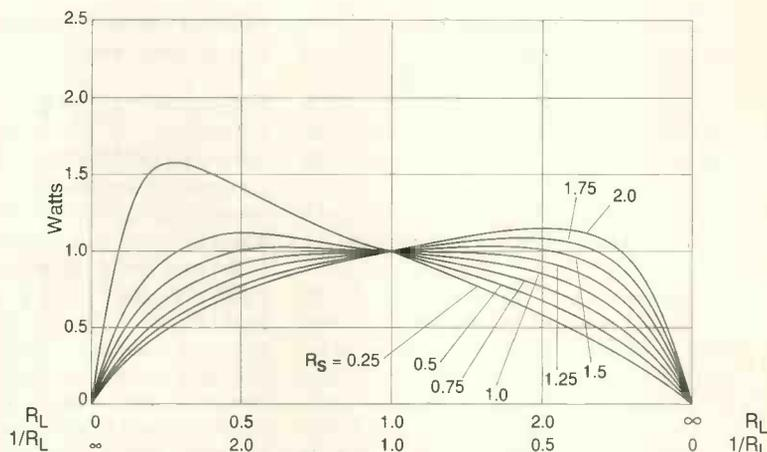
Fig. 3. Power in the load resistor  $R_L$  as a function of its value, showing curves for several different values of  $R_S$ . Source emf  $E_{SOURCE}$  adjusted to give 1W into a  $1\Omega$  load resistor  $R_L$  for each value of  $R_S$ .
