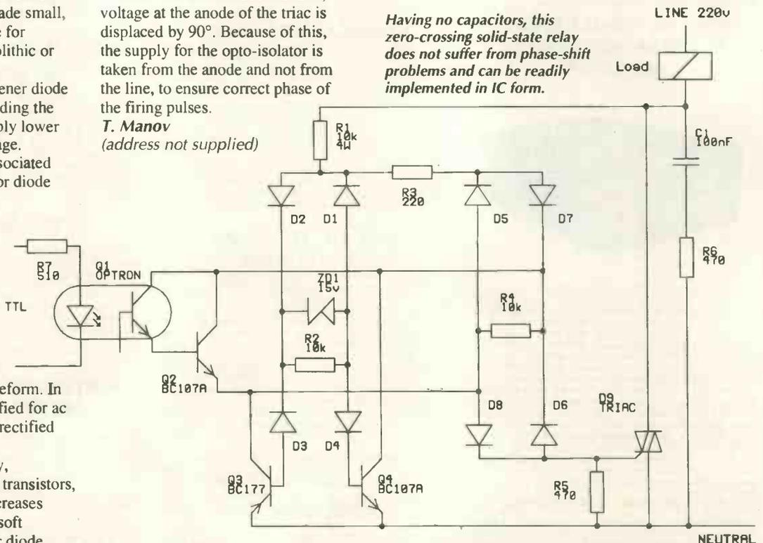
Having no capacitors, this zero-crossing solid-state relay does not suffer from phase-shift problems and can be readily implemented in IC form.
