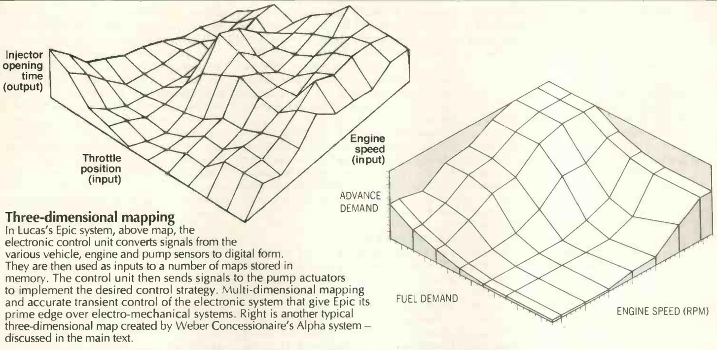
engineer runs the engine at a series of set speeds and tunes ignition timing and fuel injection using Weber Concessionaires' own software to store settings in a portable computer. These settings are logged against throttle positions and engine speeds.
