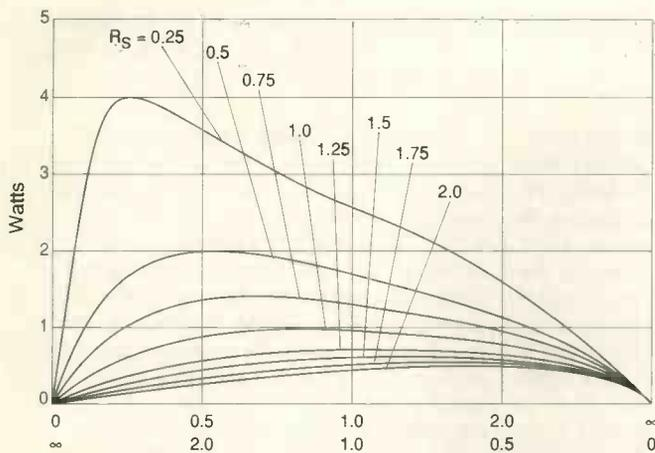
Fig. 2. Power in load resistor  $R_L$  as a function of its value, showing curves for several different values of  $R_S$ . Source emf  $E_{SOURCE}$  is as in Fig. 1a).
