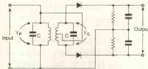
Foster-Seeley discriminator – it is still common to see descriptions of this referring to a 90° phase-shift between the primary and secondary of the tuned transformer.
