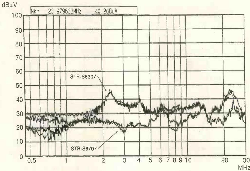
Fig. 10. Comparison of conducted EMI – ringing choke versus quasi-resonant techniques.
