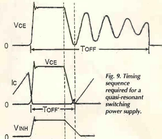
Fig. 9. Timing sequence required for a quasi-resonant switching power supply.
