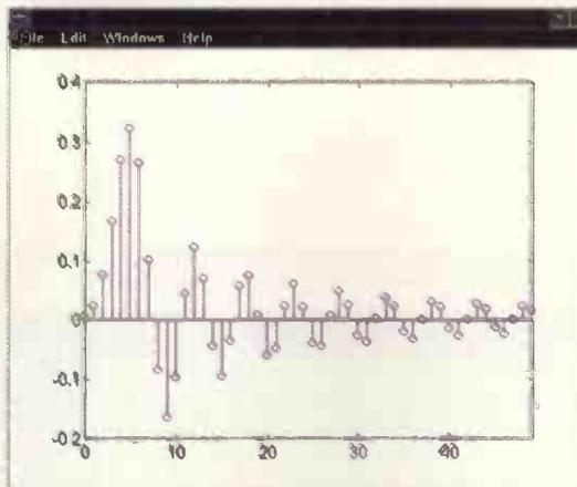
Fig. 3. When subjected to a single impulse, the impz function allows the response of the system to be visualised with ease.
