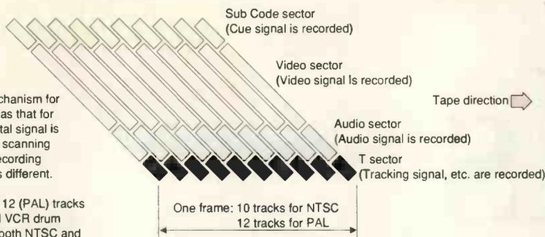
The basic recording mechanism for digital VCR is the same as that for analogue VCR. The digital signal is recorded using a helical scanning system. However, the recording pattern for digital VCR is different.
