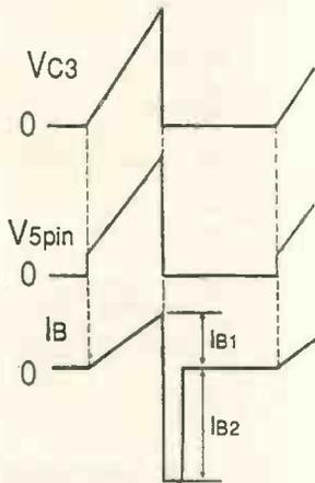
conventional pwm flyback converters – leakage inductance causes overvoltage, and primary capacitance causes overcurrent.
