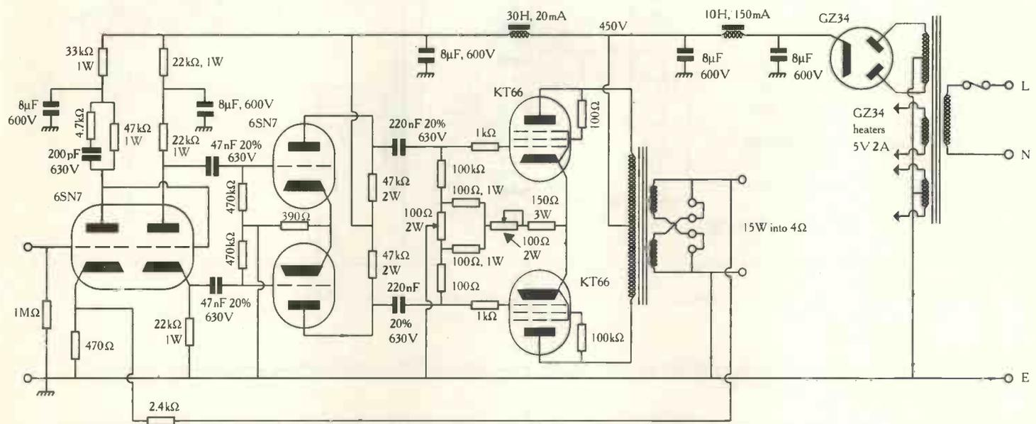
Fig. 1. Williamson's amplifier set a standard of performance that was years ahead of its time.
