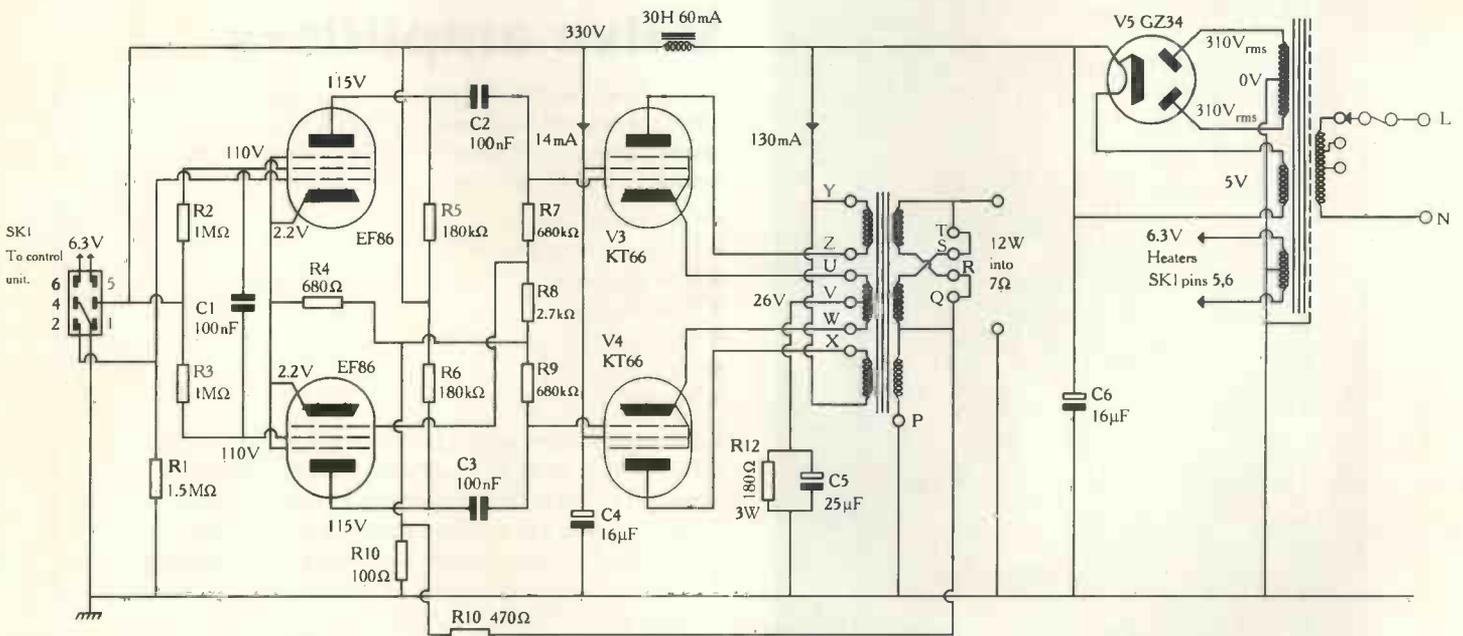
Fig. 4. The Quad II is different. Not only is the phase splitter combined with the driver, but it is also combined with the input stage. Circuit courtesy Quad Electroacoustics.
