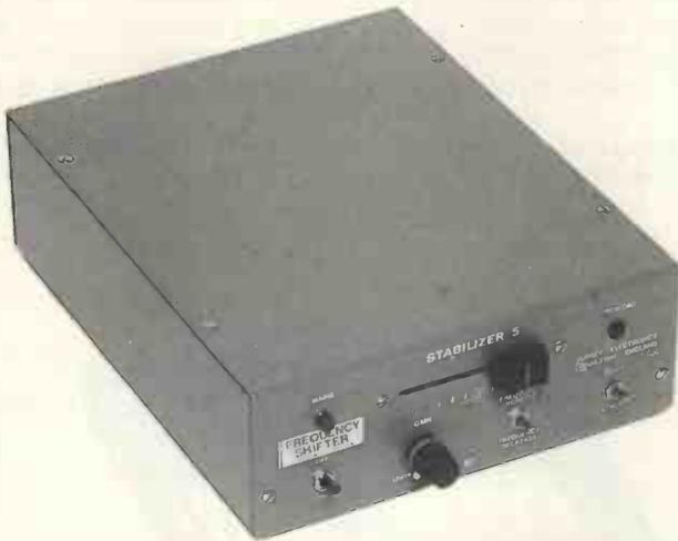
In any public address system where microphones and loudspeakers are in the same vicinity, acoustic feedback (howlround) occurs if the amplification exceeds a critical value. By shifting the audio spectrum fed to the speakers by a few Hertz, the tendency to howl at room resonance frequencies is destroyed and increased gain is available before the onset of feedback.
