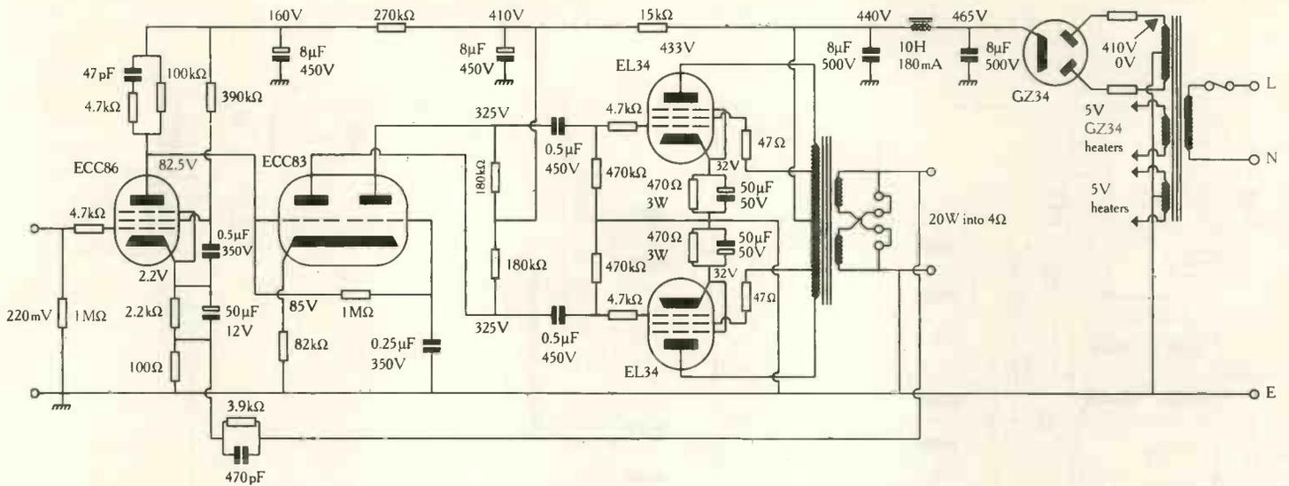
Fig. 2. Mullard's 5-20 was an ultra-linear design with high sensitivity but poor noise performance due to the input being pentode, rather than triode, based. Circuit courtesy Philips Components Ltd.
