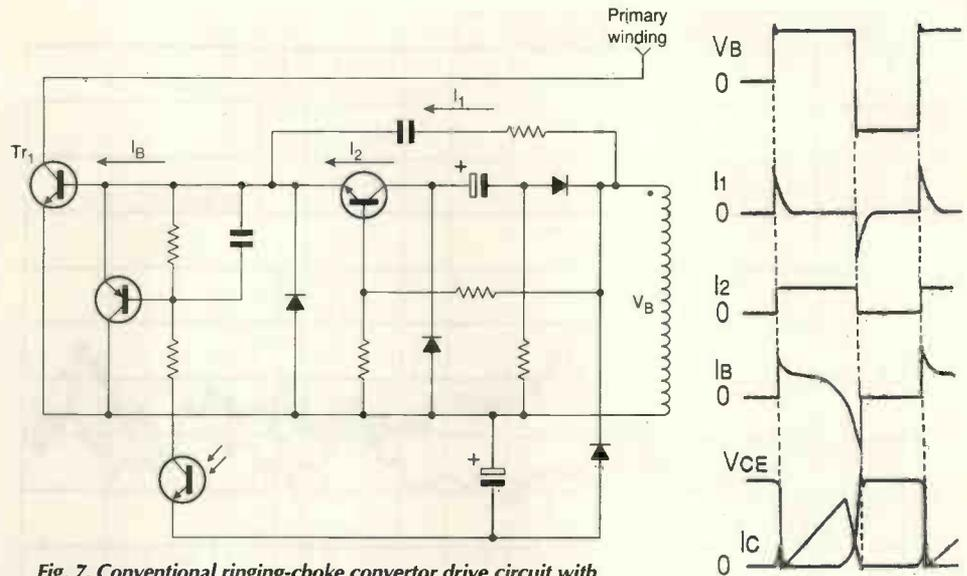
Fig. 7. Conventional ringing-choke convertor drive circuit with waveforms.
