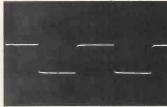
Response of the preamplifier subjected to a 5kHz squarewave at 6V pk-pk amplitude. Output loading was the quasi-standard of 50kΩ.
