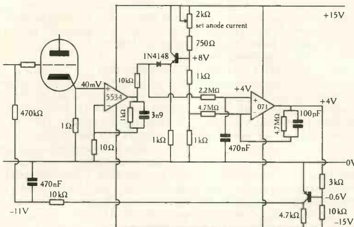
Fig. 3. Principles of the output bias servo. Although this circuit was designed to provide -11V bias, it can easily be changed by returning the transistor's collector load to a more negative supply, as necessary.
