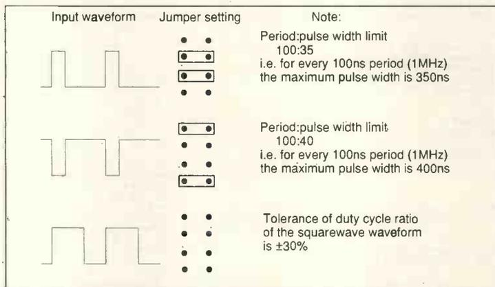
This jumper function diagram applies to both the ttl and ecl-output isolators.
