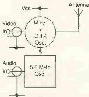
Only two transistors are needed to transmit both audio and video on vhf channel 4.
