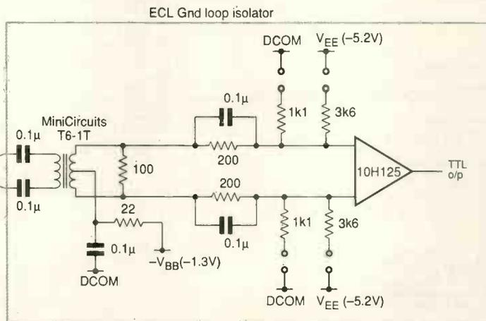
Circuits to isolate or break the path between instruments and host computer to avoid ground currents interfering with analogue equipment.
