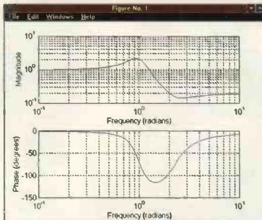
**Fig. 1.** Using the signal processing toolbox, a transfer function in the Laplace S domain can be easily realised in a plot.
